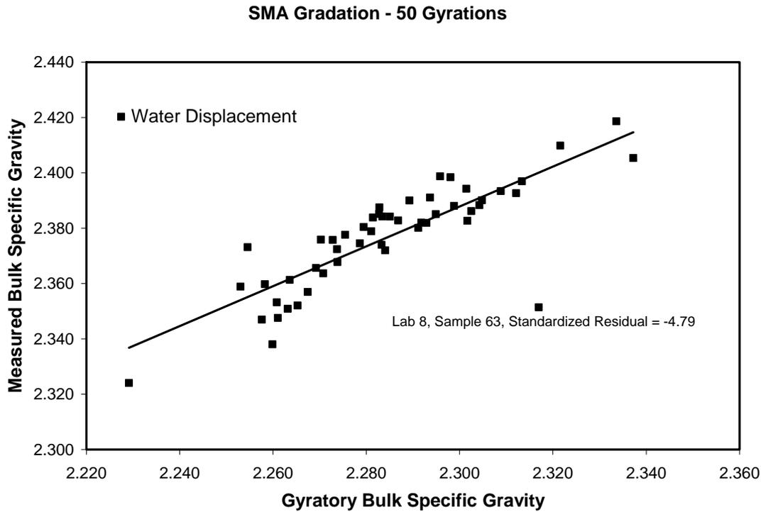
**Figure 19. Outlier Identification for Water Displacement Results SMA- 50 Gyration**
