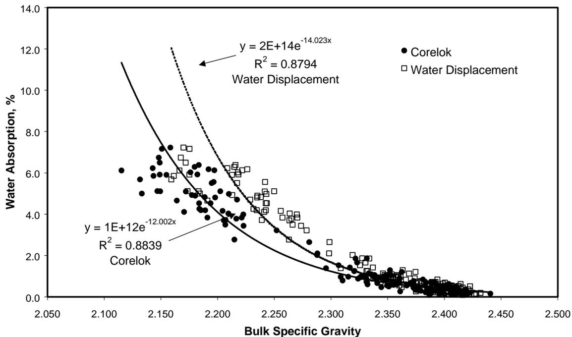
**Figure 22. Relationship Between Water Absorption and  $G_{mb}$  for Coarse Mixes**
