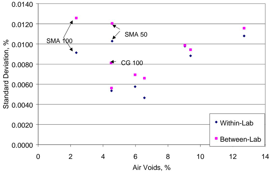
**Figure G3. Corelok Within and Between Laboratory Standard Deviations with Outliers Removed Versus Air Voids**
