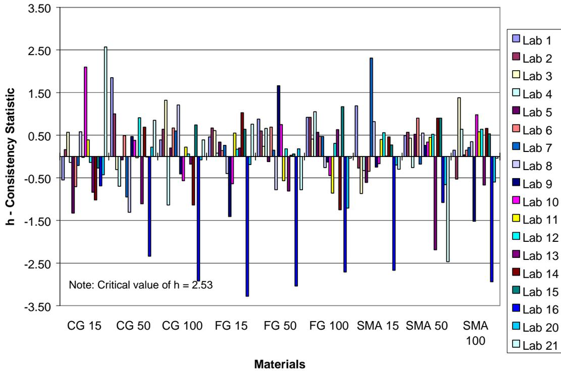
Figure 11. Corelok *h*-Consistency (Average) Factors by Material
