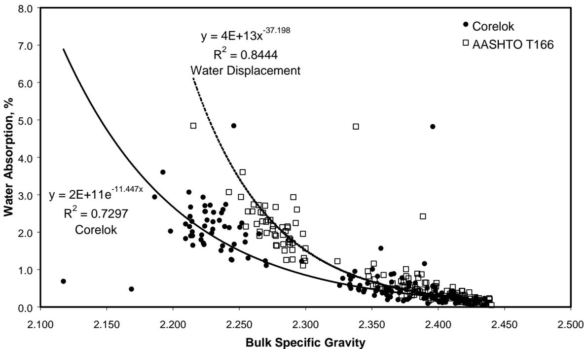
**Figure 25. Relationship Between Water Absorption and  $G_{mb}$  for SMA Mixes**
