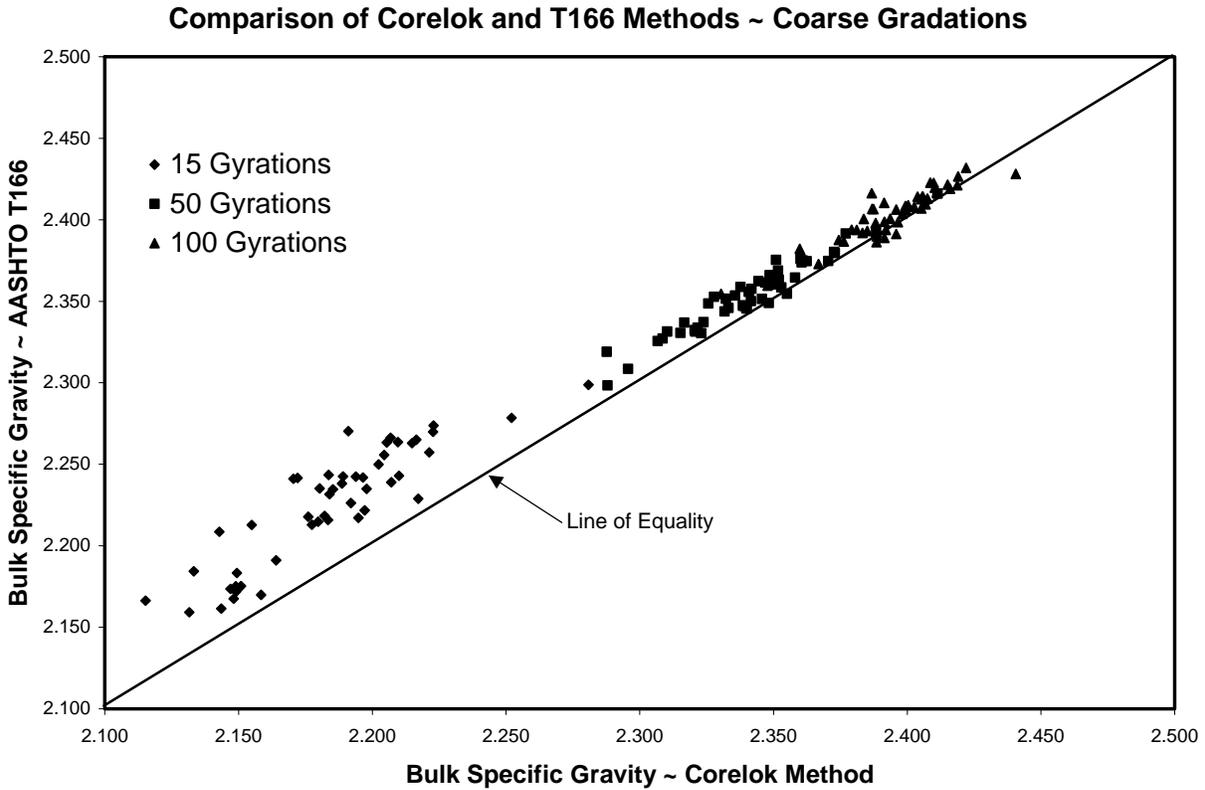
**Figure 21. Relationship Between Two Methods in Measurement for Coarse Gradation**
