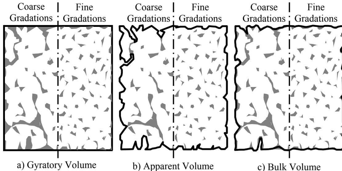
**Figure 3. Volumes Associated with Compacted HMA**
