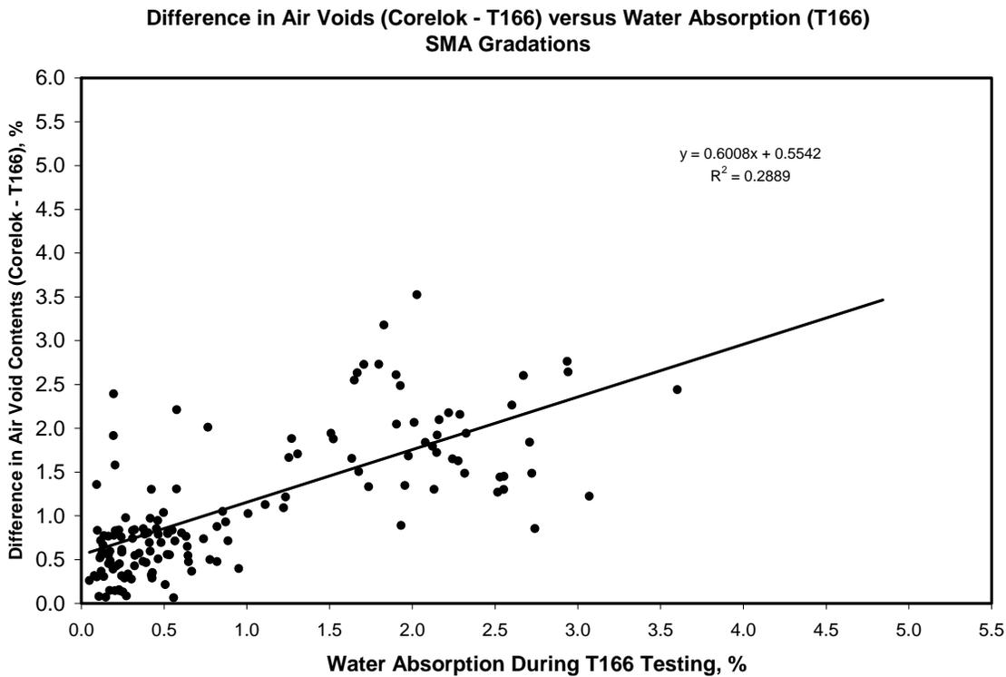
**Figure 26. Difference in Air Void Content Based Upon Water Absorption (SMA Mixes)**
