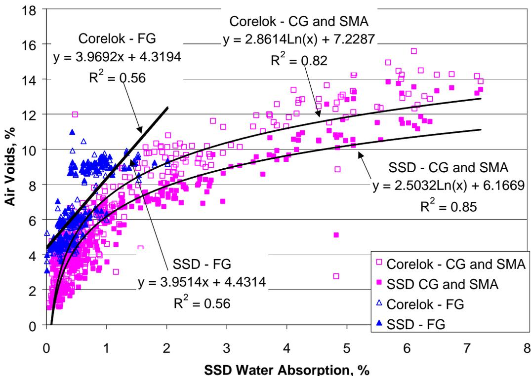
**Figure 27. Relationship Between Air Void Content and Water Absorption for All Mixes**
