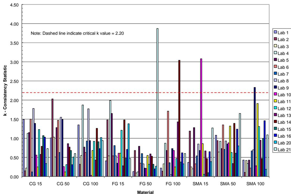
**Figure 9. AASHTO T166 *k*-Consistency (Variability) Factors by Material**
