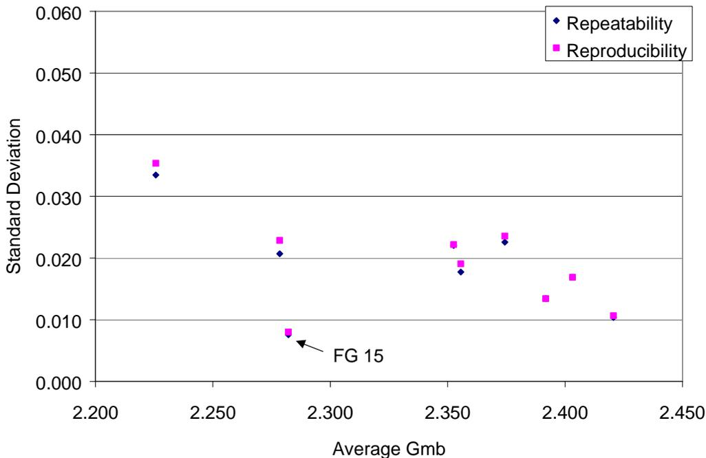
**Figure 14. Standard Deviation (1s) versus Average  $G_{mb}$  for AASHTO T166 Results**
