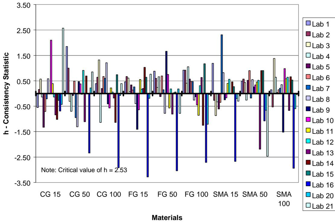
Figure 7. AASHTO T166  $h$ -Consistency (Average) Factors by Material
