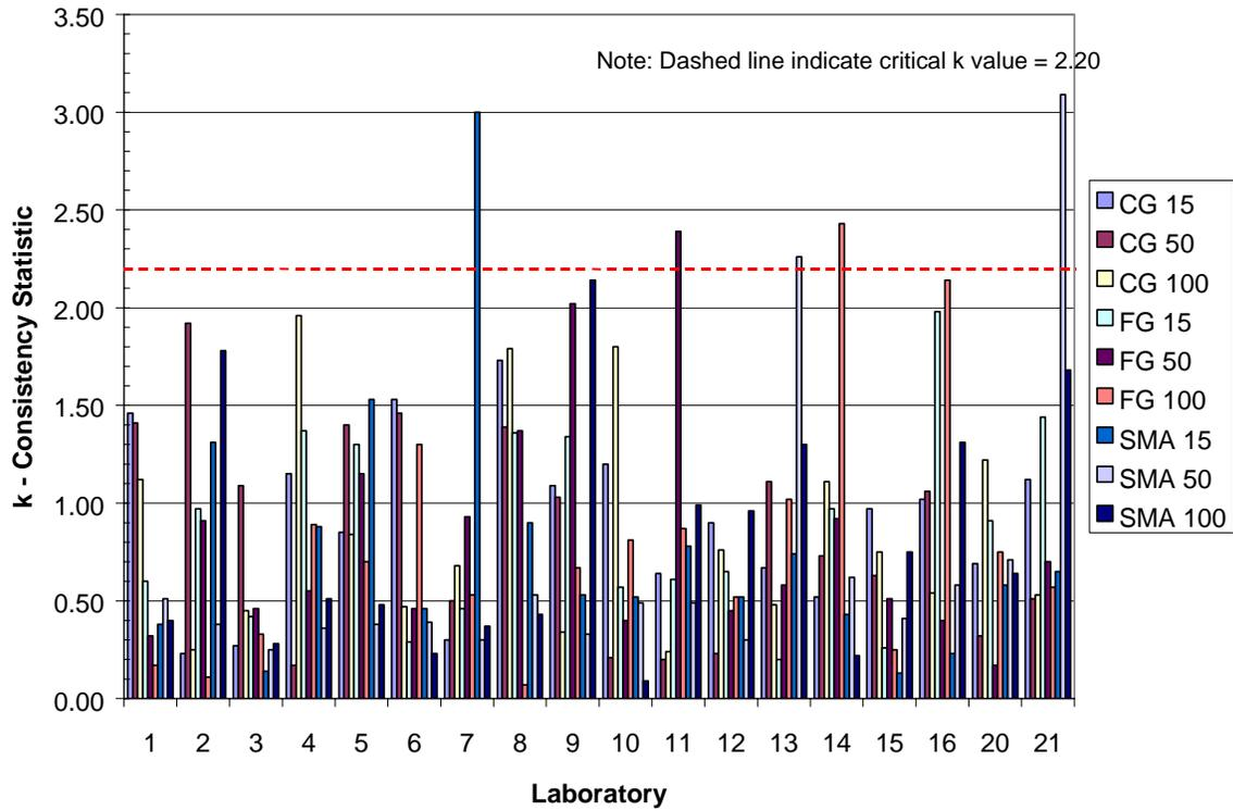
Figure 12. Corelok  $k$ -Consistency (Variability) Factors by Laboratory
