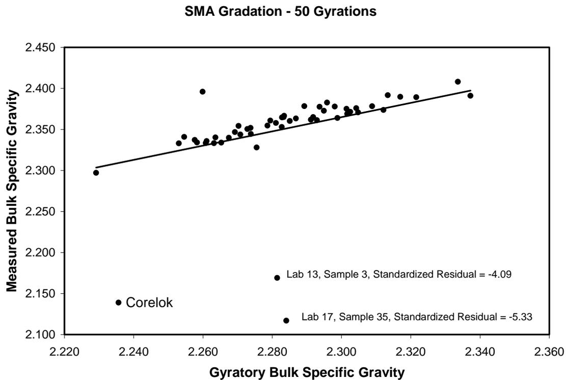
**Figure 18. Outlier Identification for Corelok Results SMA- 50 Gyration**
