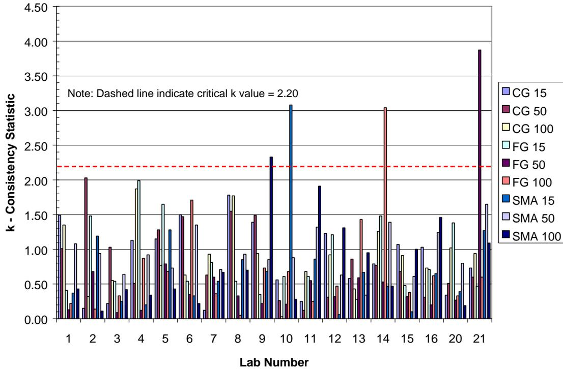
Figure 8. AASHTO T166  $k$ -Consistency (Variability) Factors by Laboratory
