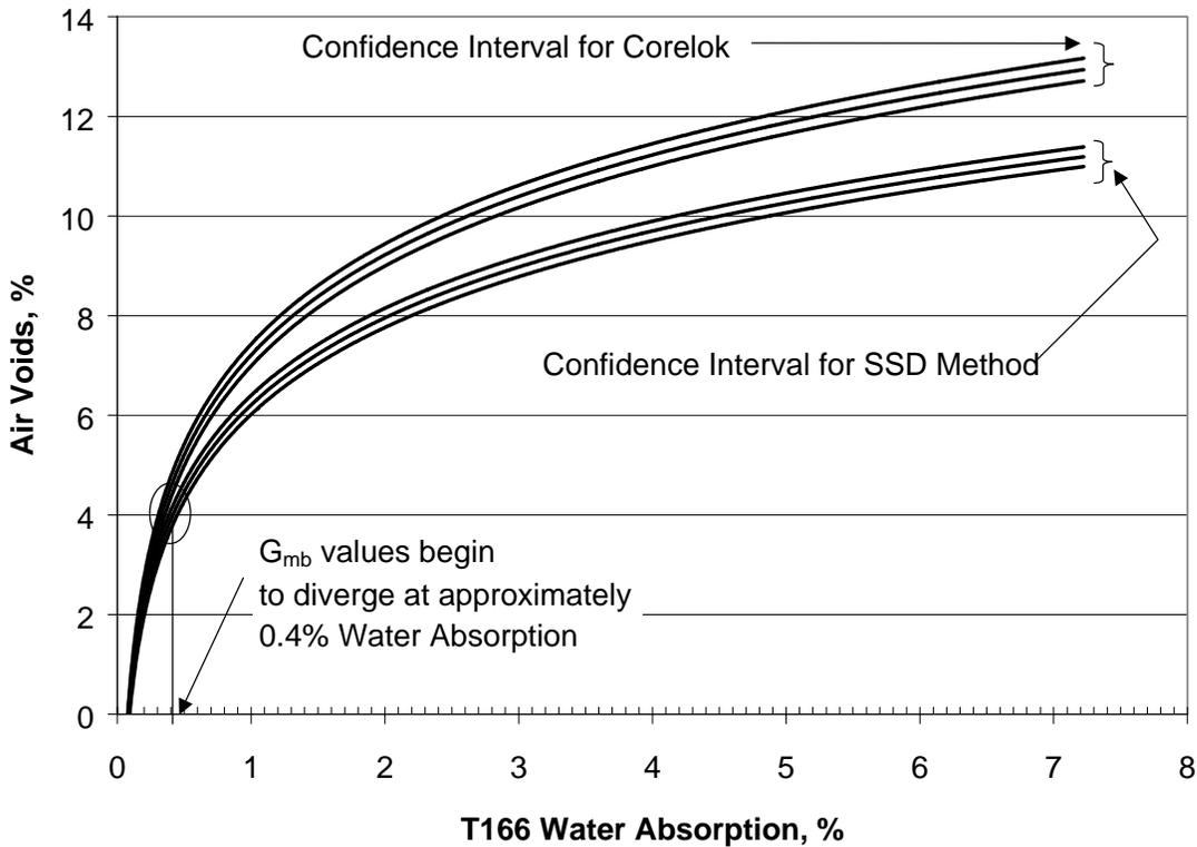
**Figure 28. Divergence in Air Voids for the Two Methods**
