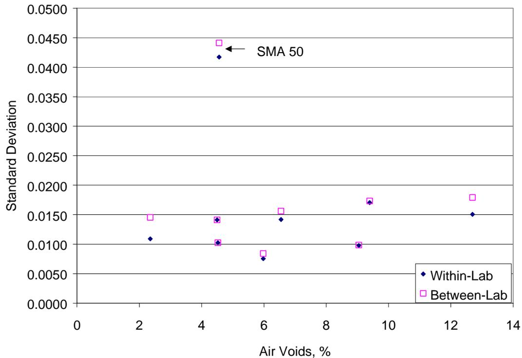
**Figure 17. Corelok Standard Deviation Including Outliers Based on Difference Analysis Versus Average Air Voids**
