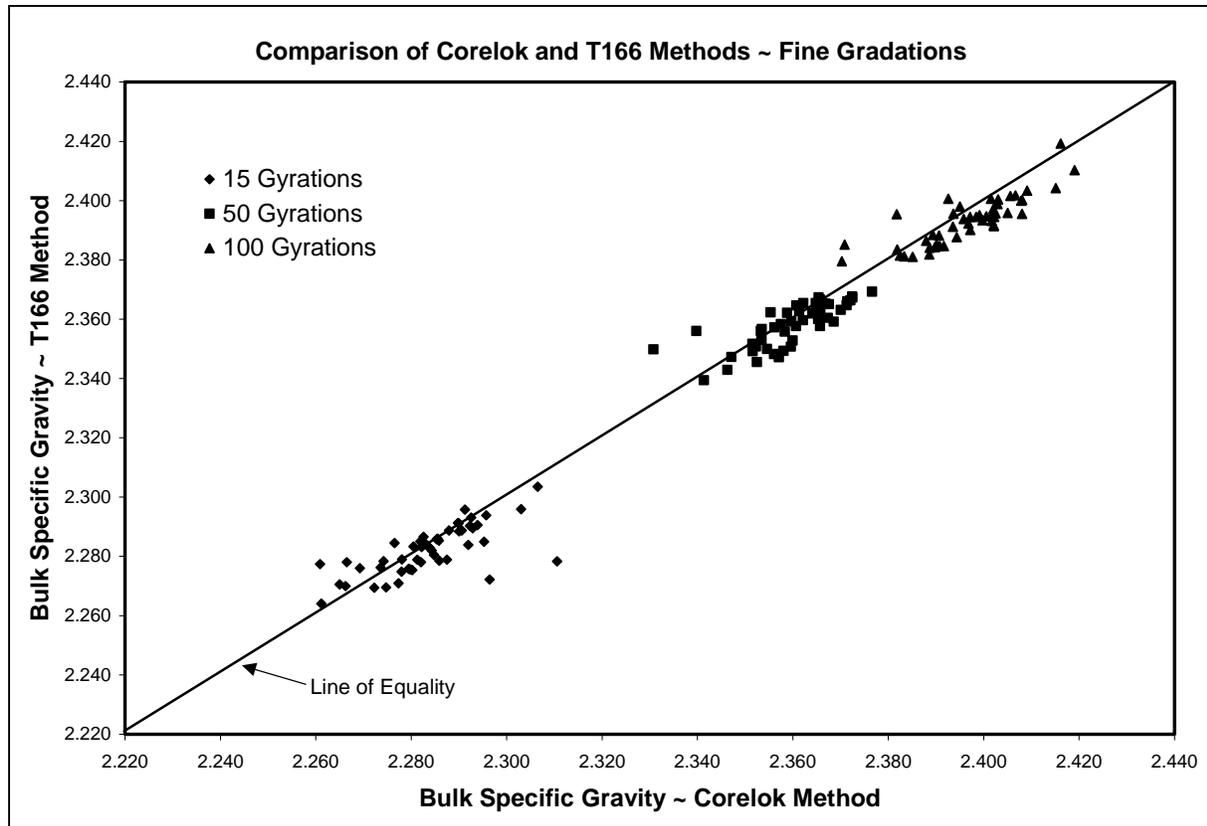
**Figure 20. Relationship Between  $G_{mb}$  Measurements for Fine Gradation Materials**
