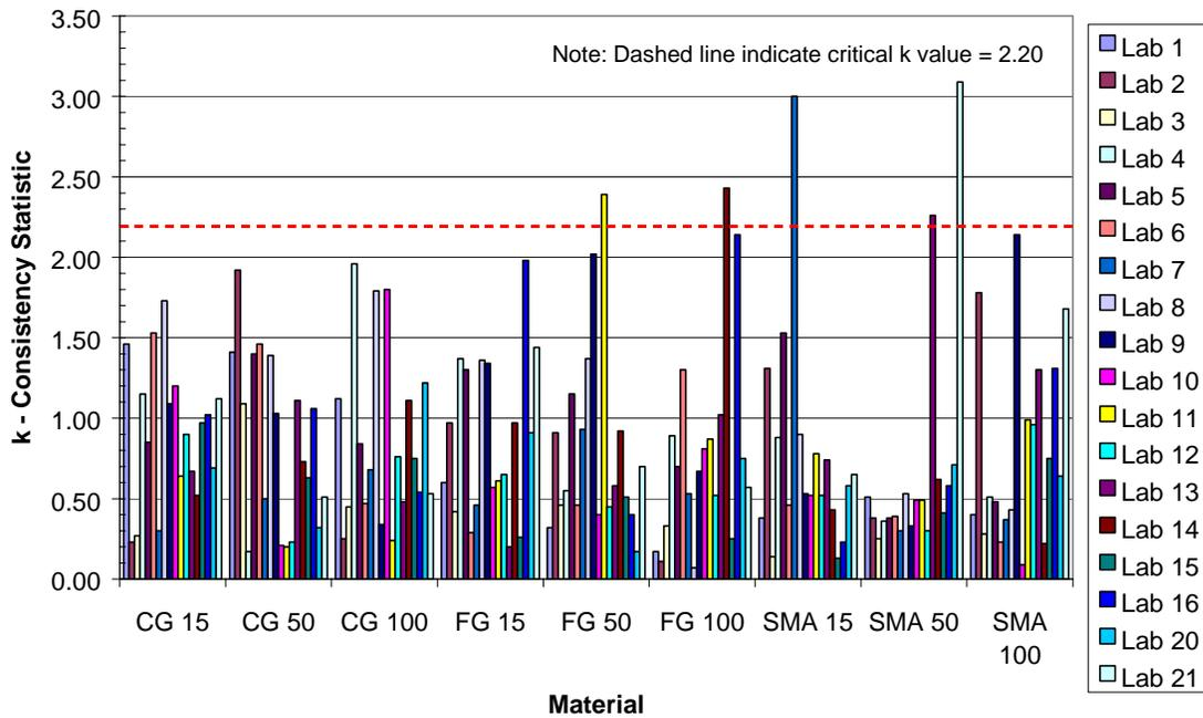
Figure 13. Corelok  $k$ -Consistency (Variability) Factors by Material
