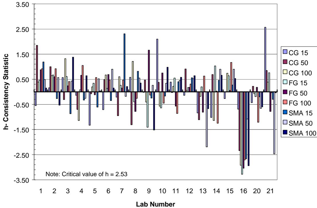
**Figure 6. AASHTO T166  $h$ -Consistency (Average) Factors by Laboratory**
