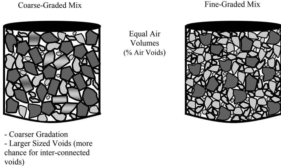
**Figure 1. Differences in Internal Void Structure for Coarse- and Fine-Graded Mixes**
