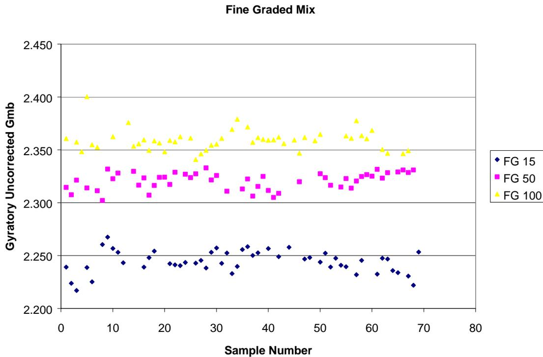
**Figure 16. Uncorrected Gyratory  $G_{mb}$  for Fine Graded Mixes**
