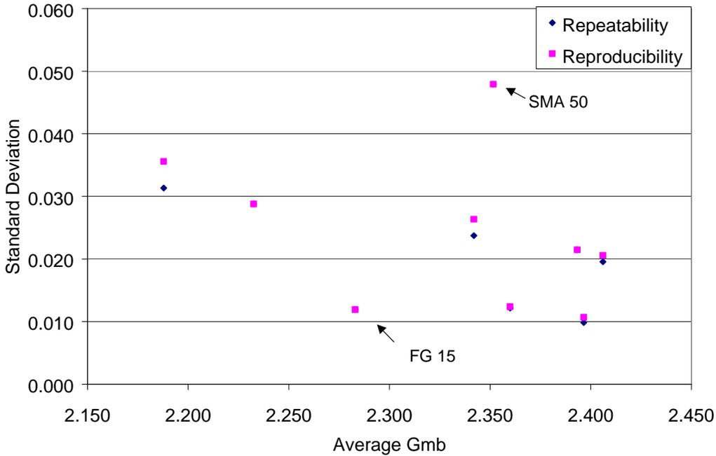
**Figure 15. Standard Deviation (1s) versus Average G<sub>mb</sub> for Corelok Results**
