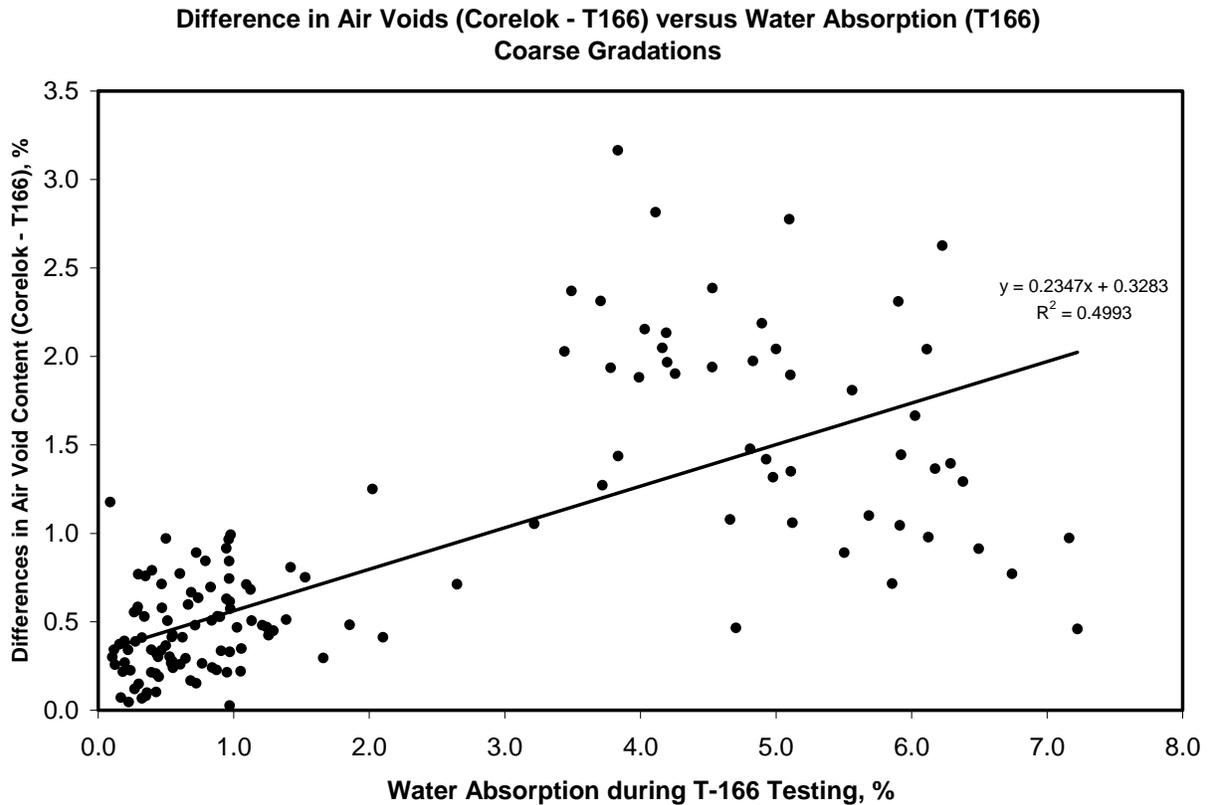
**Figure 23. Difference in Air Void Contents Based Upon Water Absorption (Coarse Mixes)**
