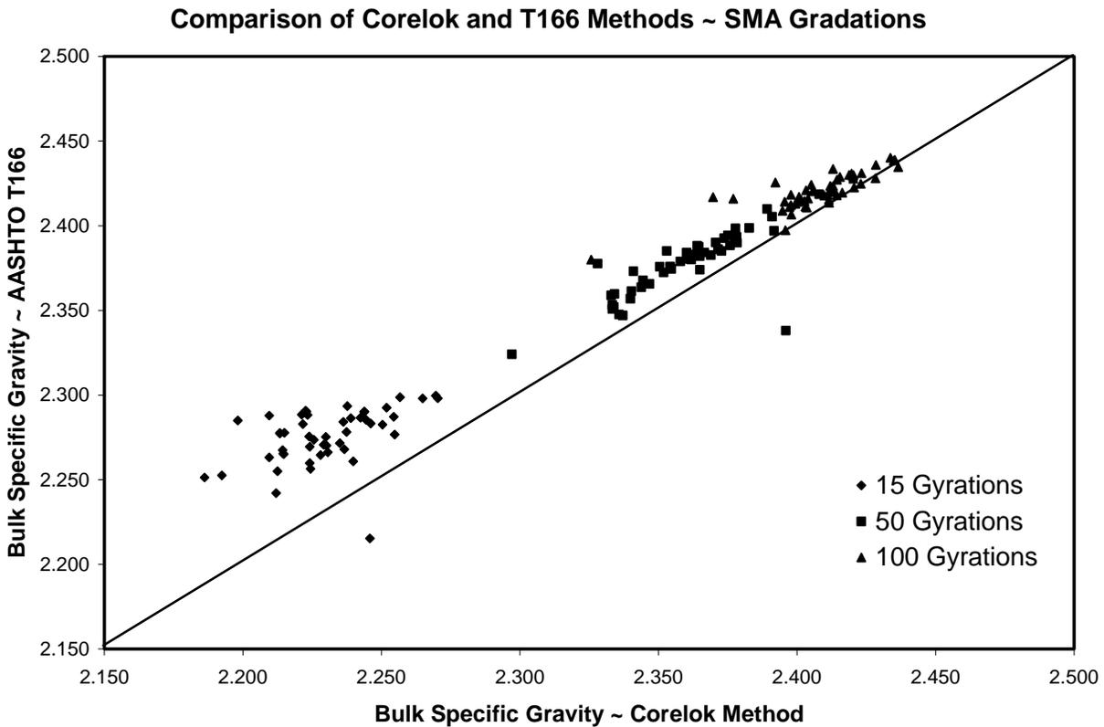
**Figure 24. Relationship Between Two Methods of Measurement for SMA Gradations**
