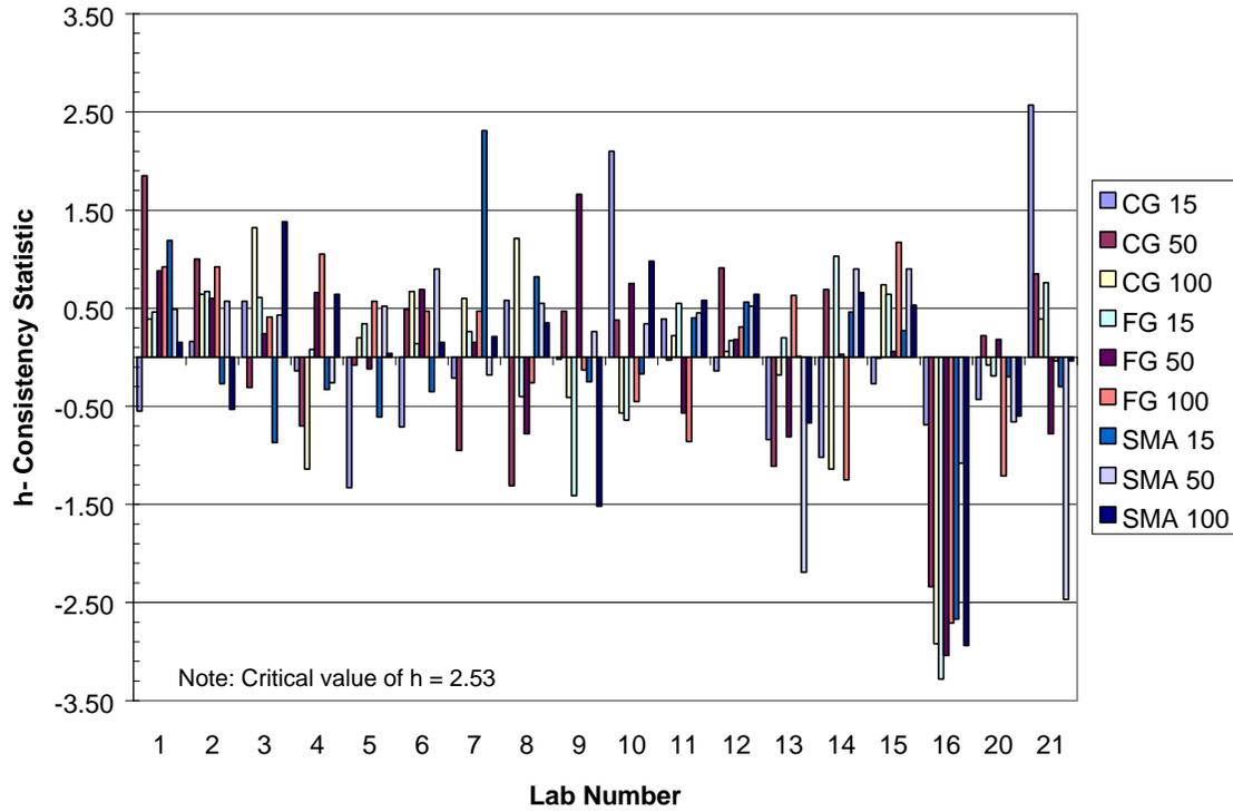
Figure 10. Corelok *h*-Consistency (Average) Factors by Laboratory
