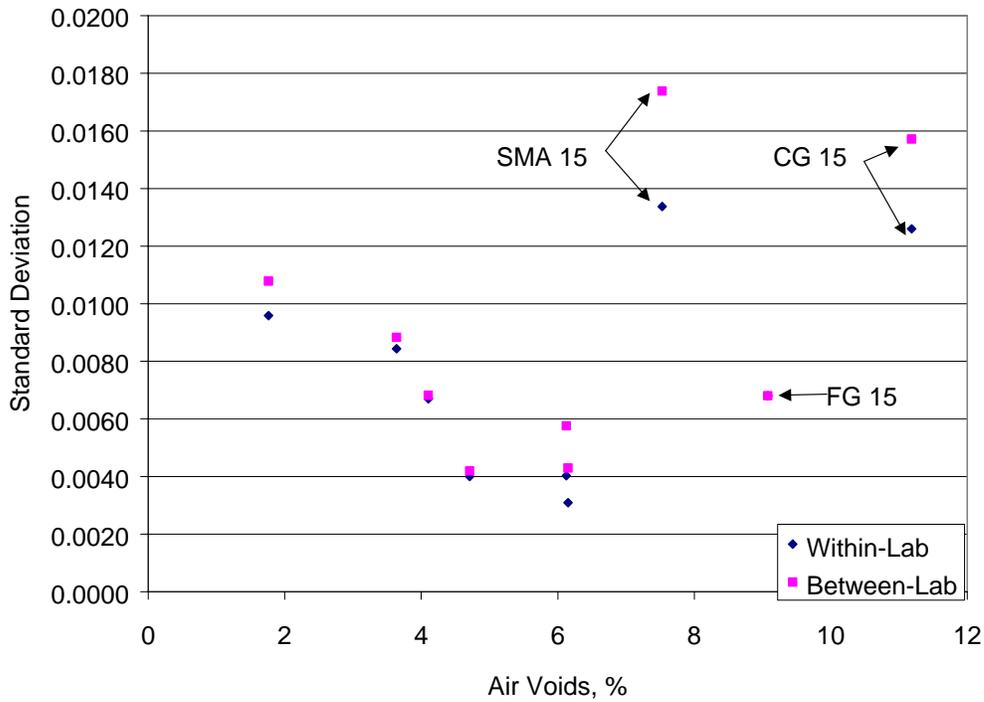
**Figure G2. SSD Within and Between Laboratory Standard Deviations with Outliers Removed Versus Air Voids**
