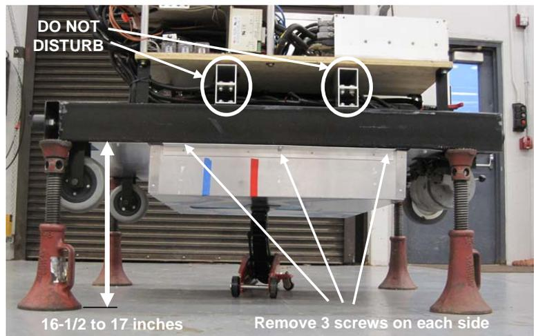
Figure D.3. The benchmark profiler supported on four post jacks with the battery jack lightly supporting the center floor panel
