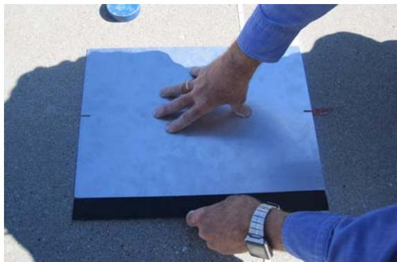
c. Secure the transfer plate in position and transfer the marker plate to the opposite edge of the transfer plate.
