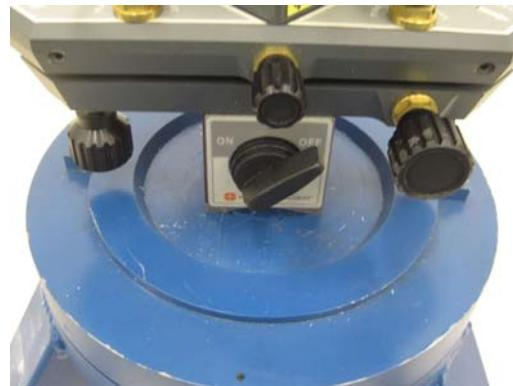
**b. The L-740 improperly mounted: the magnetic base is not against the edge of the dished surface and the magnet switch is off.**
