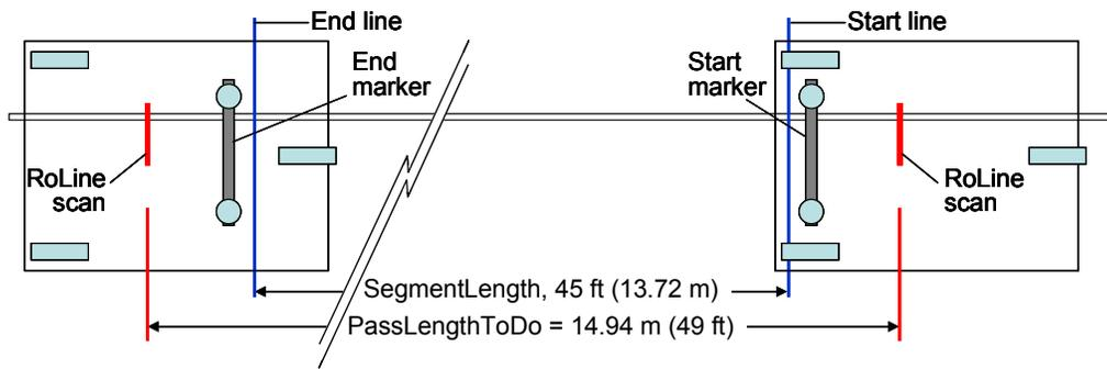
**Figure 2.9. The segment length and pass length for the standard-length test segment**
