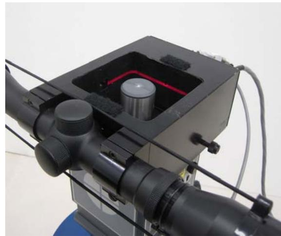
b. Rear quarter view showing the laser beam sweeping across the window into the circuit chamber
