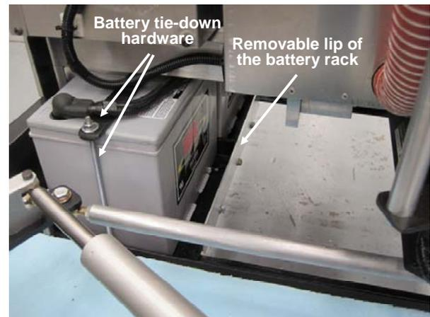
**Figure D.4. View of the batteries on the right side (8-in., 12-volt system) looking from the front**
