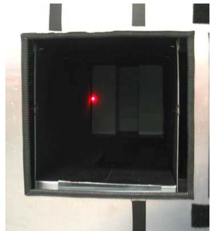
c. Laser dot on the far left edge of the near laser target
