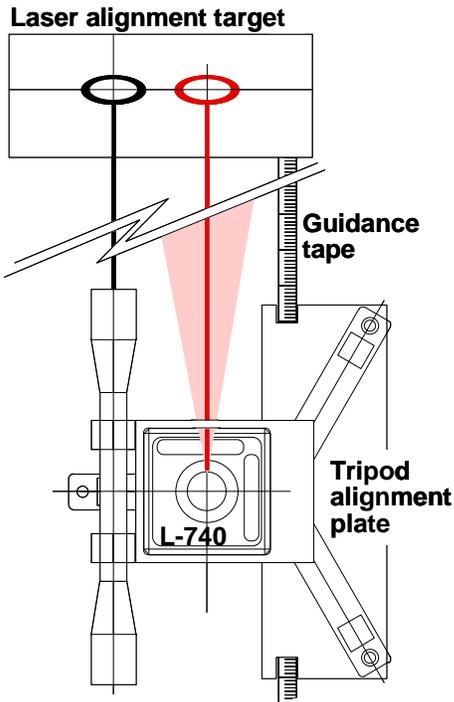
Figure 3.7. A schematic diagram of the lateral and yaw alignment of the spinning laser
