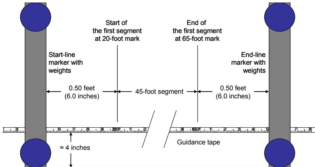
Figure 4.7. Placement of the start-line and end-line marker strips for the first segment (not to scale)
