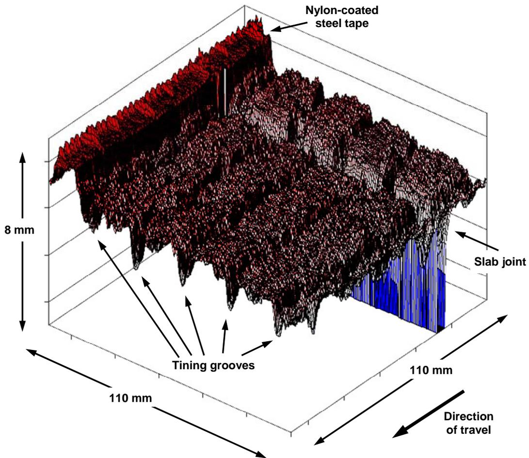
Figure 1.7. Surface plot of RoLine measurements of a new, longitudinally-tined road surface
