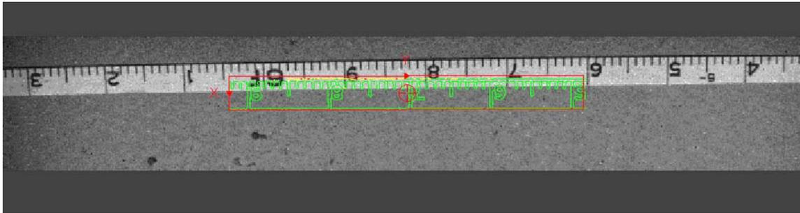
**Figure E.6. Initial image with the tape poorly aligned longitudinally, laterally and angularly**
