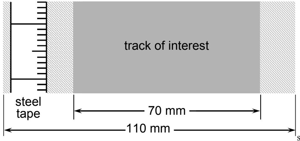
Figure 1.6. Layout within the RoLine footprint
