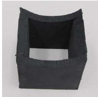
Figure A.15. Sun shade for laser bubble-levels
