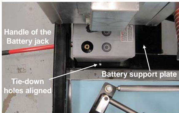
**a. Position the battery jack with the support plate adjacent to the battery to be removed.**
