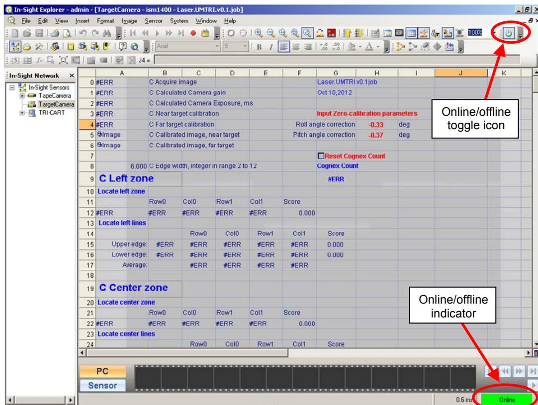
Figure I.1. *In-Sight Explorer* screen with TargetCamera connected (Spreadsheet view)
