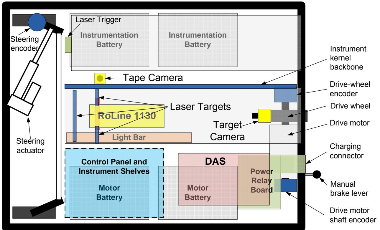
Figure 1.3. A schematic diagram of the major elements of the benchmark profiler in plan view
