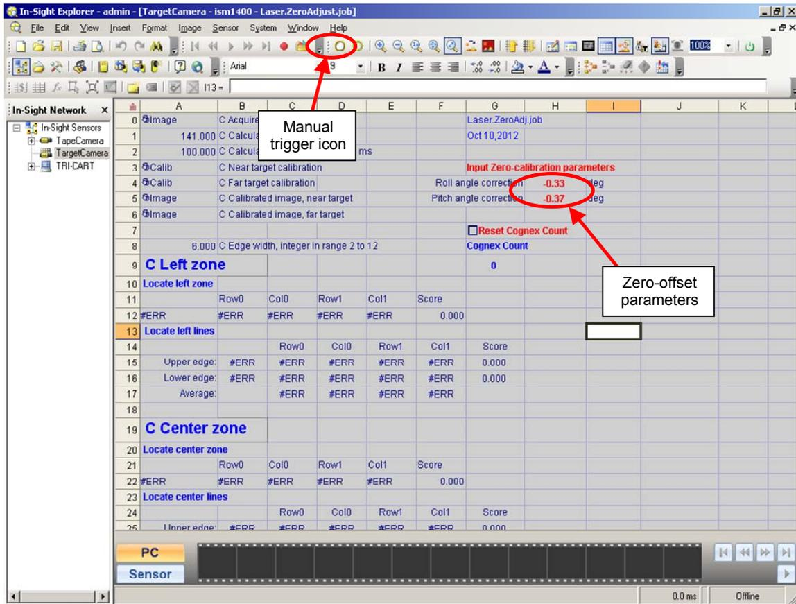
Figure I.2. In-Sight Explorer screen with Laser.ZeroAdj.job loaded (Spreadsheet view)
