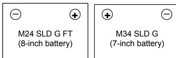
**Figure D.1. Terminal positions differ on the two types of batteries used on the benchmark profiler**
