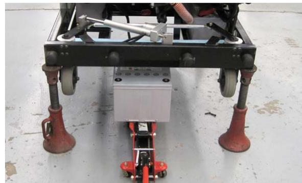
**d. Rotate the jack 90 degrees and remove it and the battery toward the front of the profiler.**
