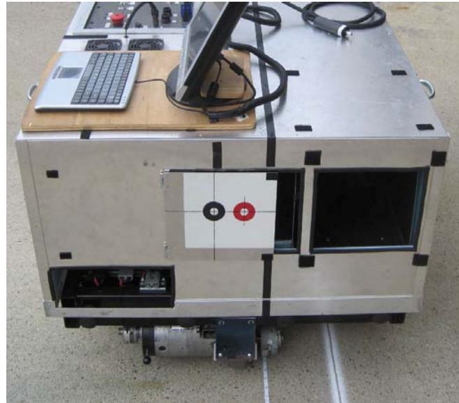
Figure 3.8. The laser alignment target, in the display position, on the rear of the benchmark profiler
