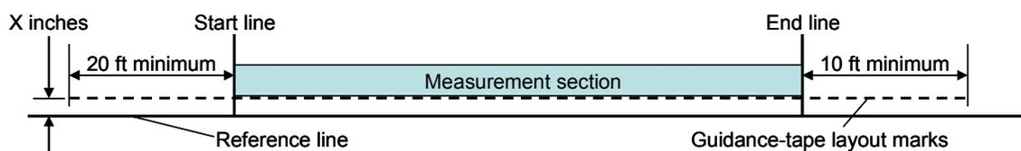
Figure 4.1. A schematic diagram of site preparation for the benchmark profiler (not to scale)
