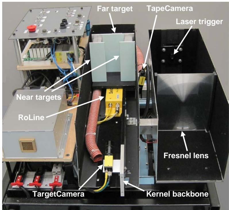
**Figure 1.4. Features of the instrument kernel and the laser trigger**
