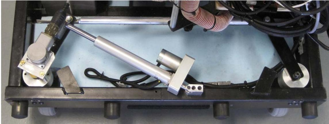
**Figure 1.10. Top view of the steering system showing actuator, linkage, and encoder**
