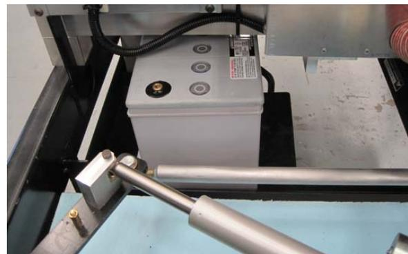
**b. Slide the battery onto the support plate.**
