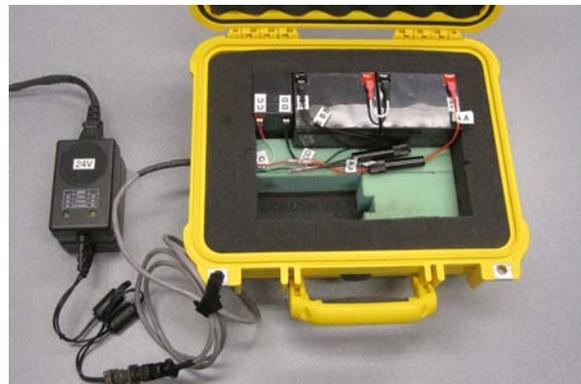
b. The chargers removed for charging the batteries
