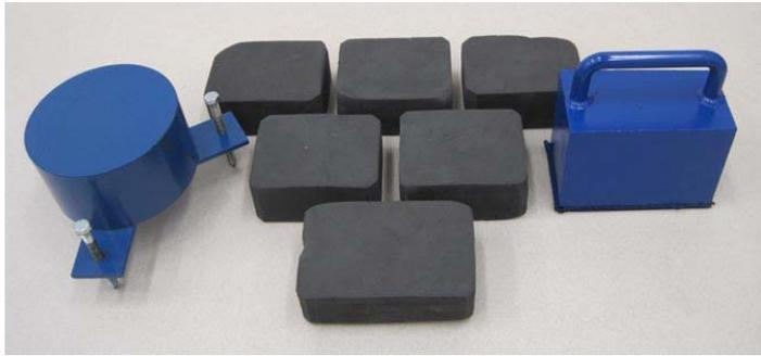
Anchor, tripod    Foam block weights    Anchor, block
