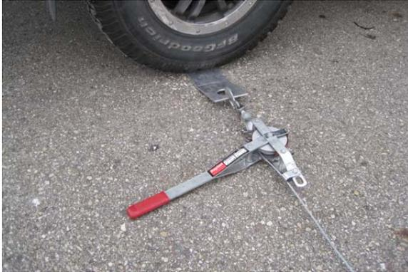
**a. The come-along attached to one vehicle anchor plate**
