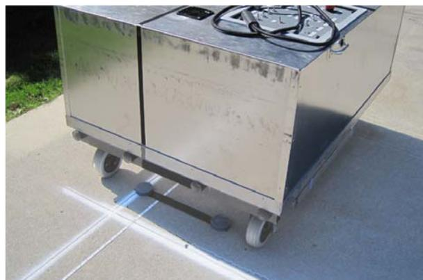
**Figure 2.11. The benchmark profiler in position to start the measurement of a segment**
