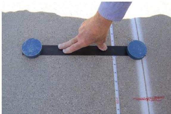
a. Secure the end-line marker plate in position.
