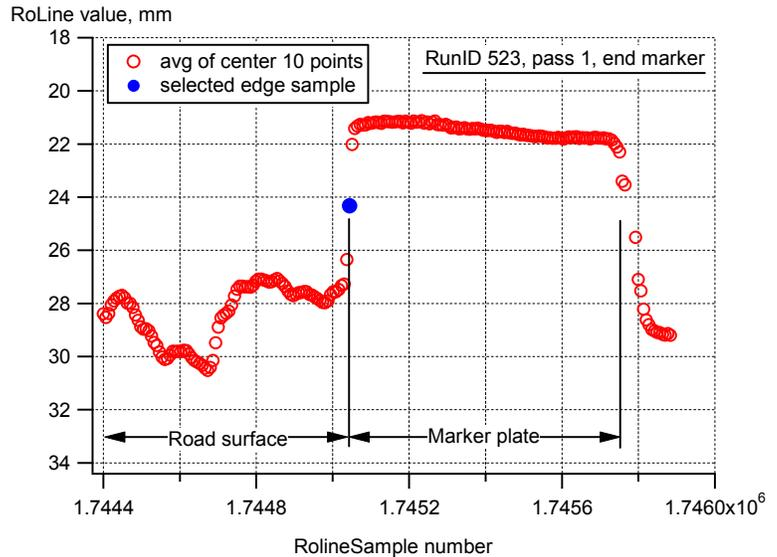
**Figure 5.2. An example of processed RoLine data in the vicinity of an end-marker plate**
