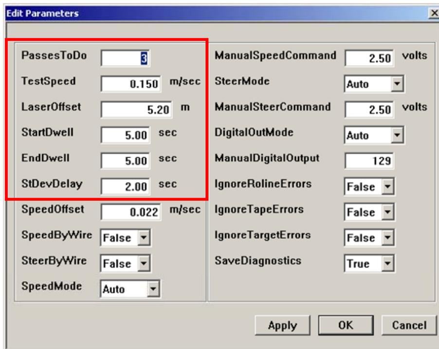
Figure 2.6. The *Edit Parameters* dialog with standard values shown and the five parameters subject to change highlighted
