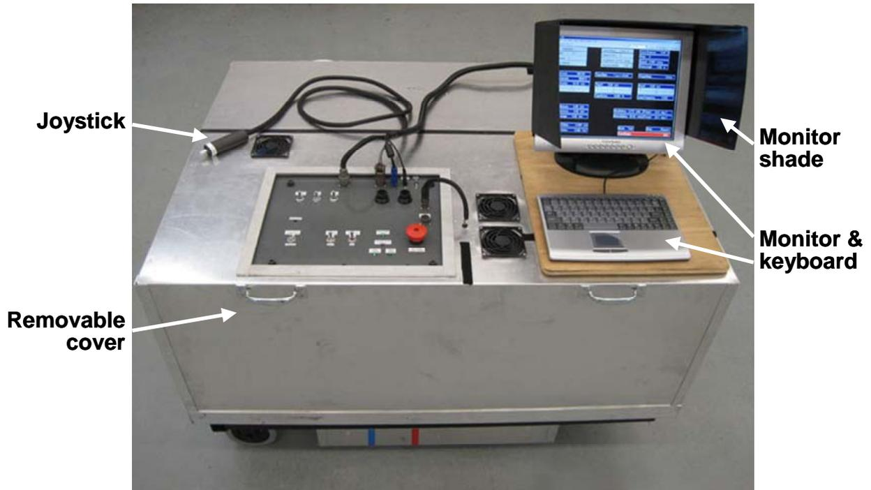
a. With cover, joystick, monitor & keyboard, and monitor sun shade
