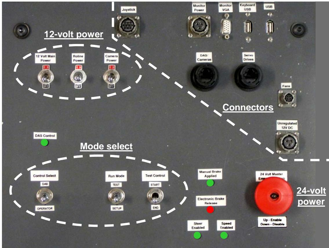
**Figure 2.2. The benchmark profiler’s control panel (with group indications added)**
