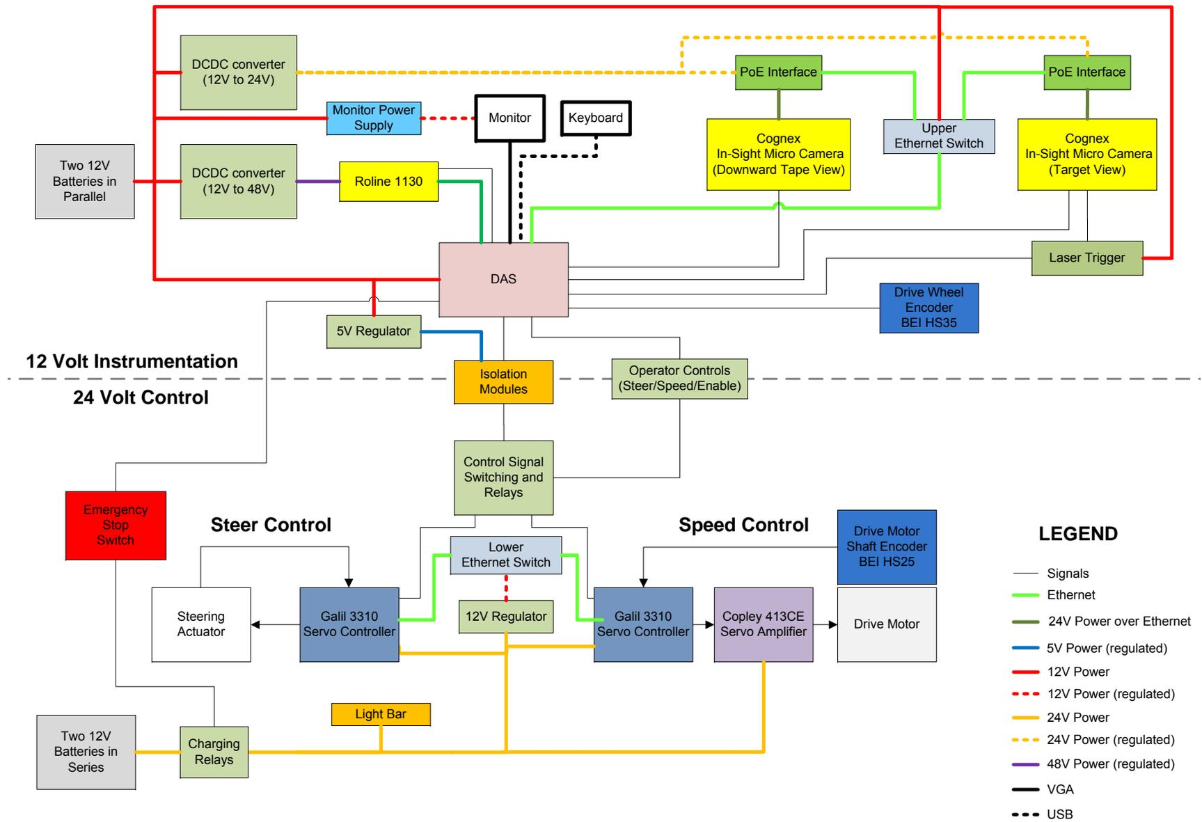
Figure F.2. Block diagram of the electrical systems
