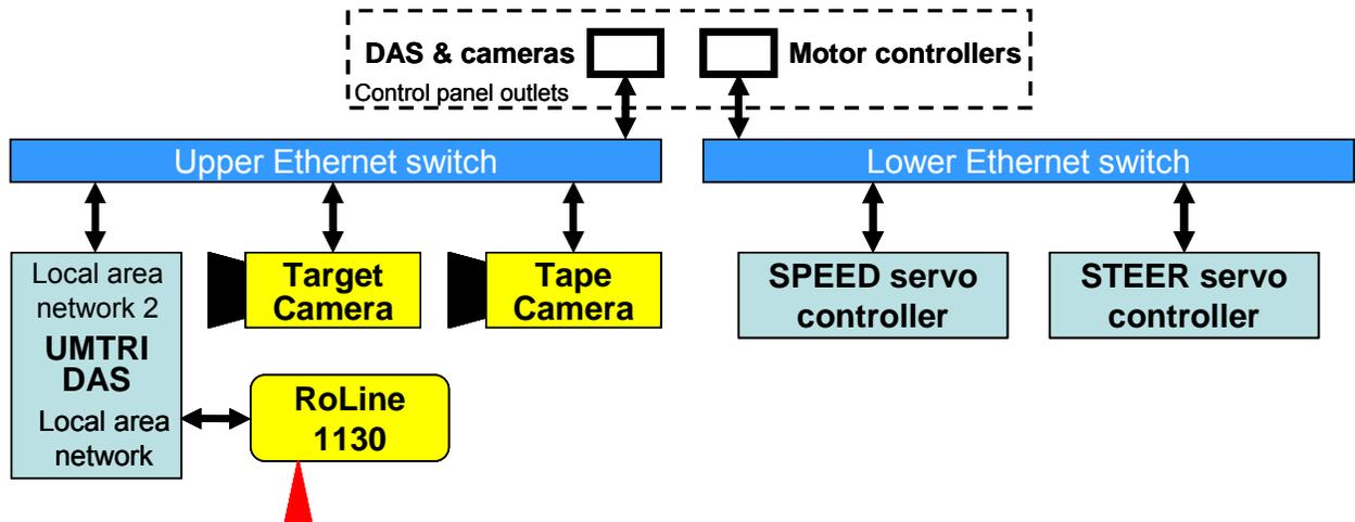
Figure B.1. Schematic diagram of the Ethernet connections of the benchmark profiler
