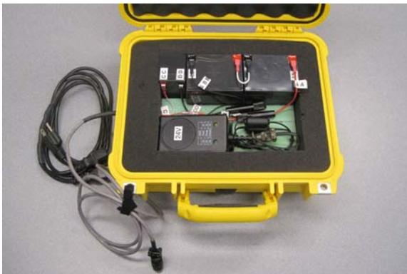
a. The battery pack with chargers and three batteries
