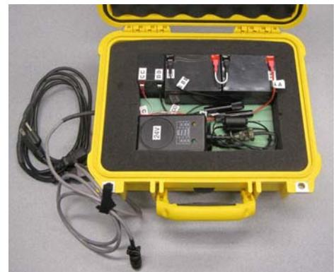
b. Open showing batteries and chargers
