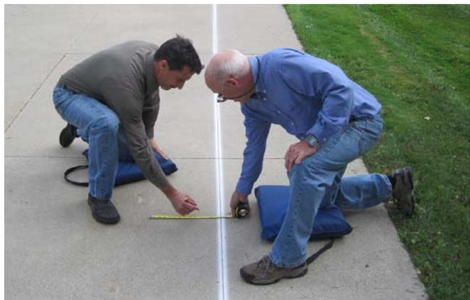
**Figure 4.3. Two people marking the guidance tape position relative to the reference line**
