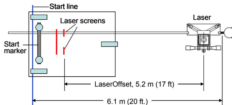
**Figure 2.7. The initial laser offset for the standard test setup is 5.2 m.**
