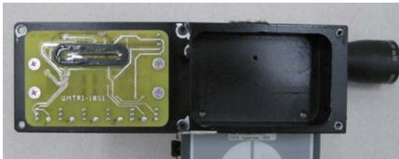
d. Side view with the circuit chamber open and the laser-beam window and the photo diode visible
