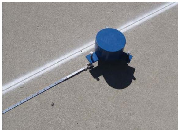
b. The start of the guidance tape anchored with the weighted tripod.
