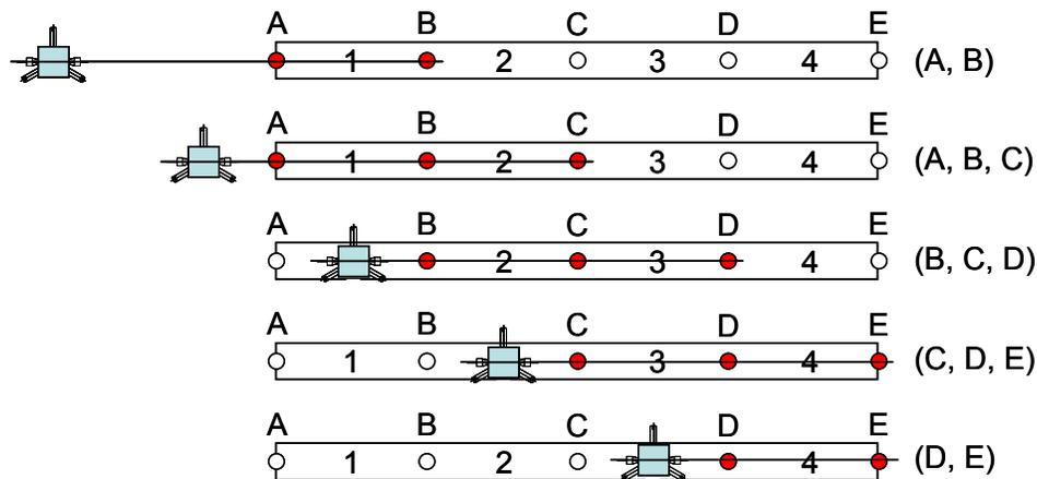
**Figure 4.14. A scheme for surveying a measurement section with four segments (1 through 4) and five segment endpoints (A through E)**
