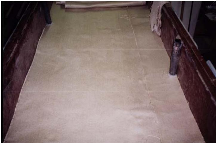
**Figure 14.** Separator of GCBD after placement on the subgrade. Note overlap of the geotextile towards the right side of the box.
