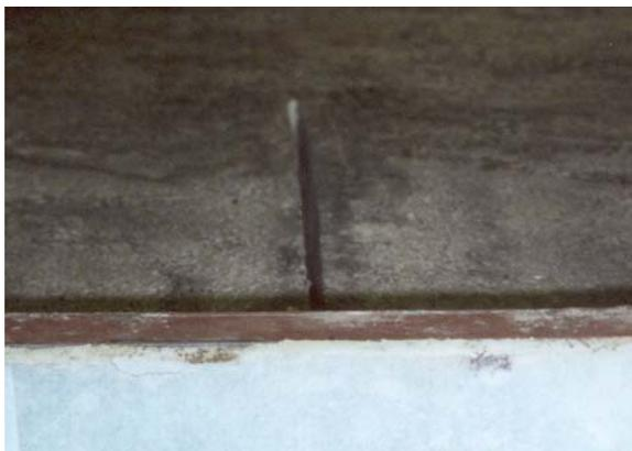
**Figure 11.** Photograph of crack sawn into the asphalt. The crack is 6 mm wide.
