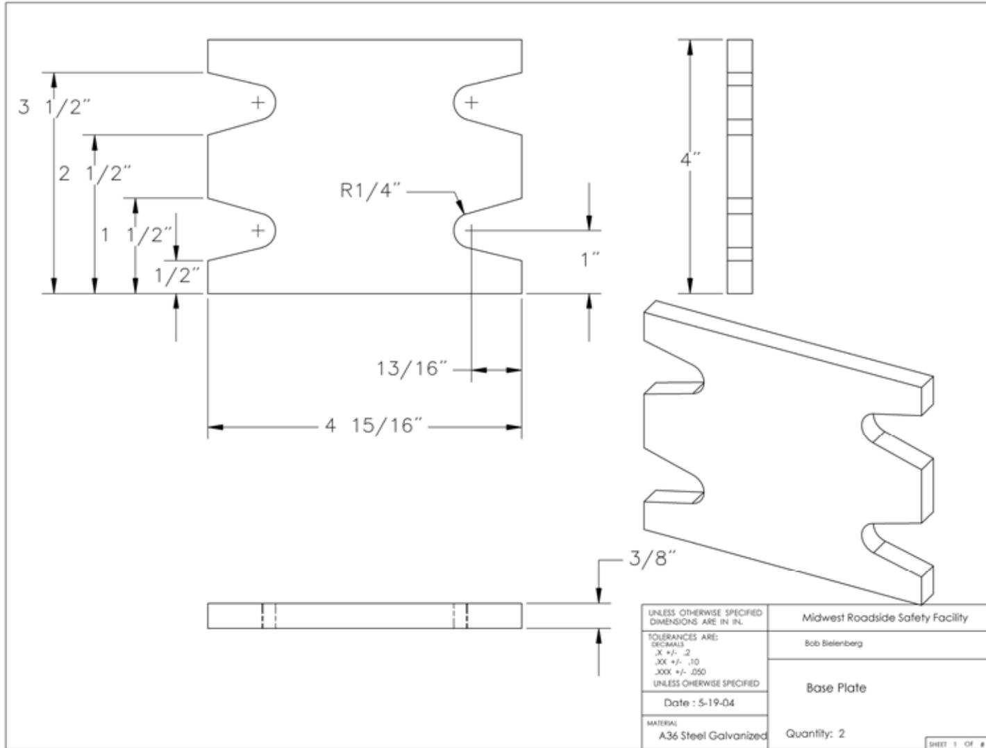
Figure 7. Modified NY Cable Anchorage Details
