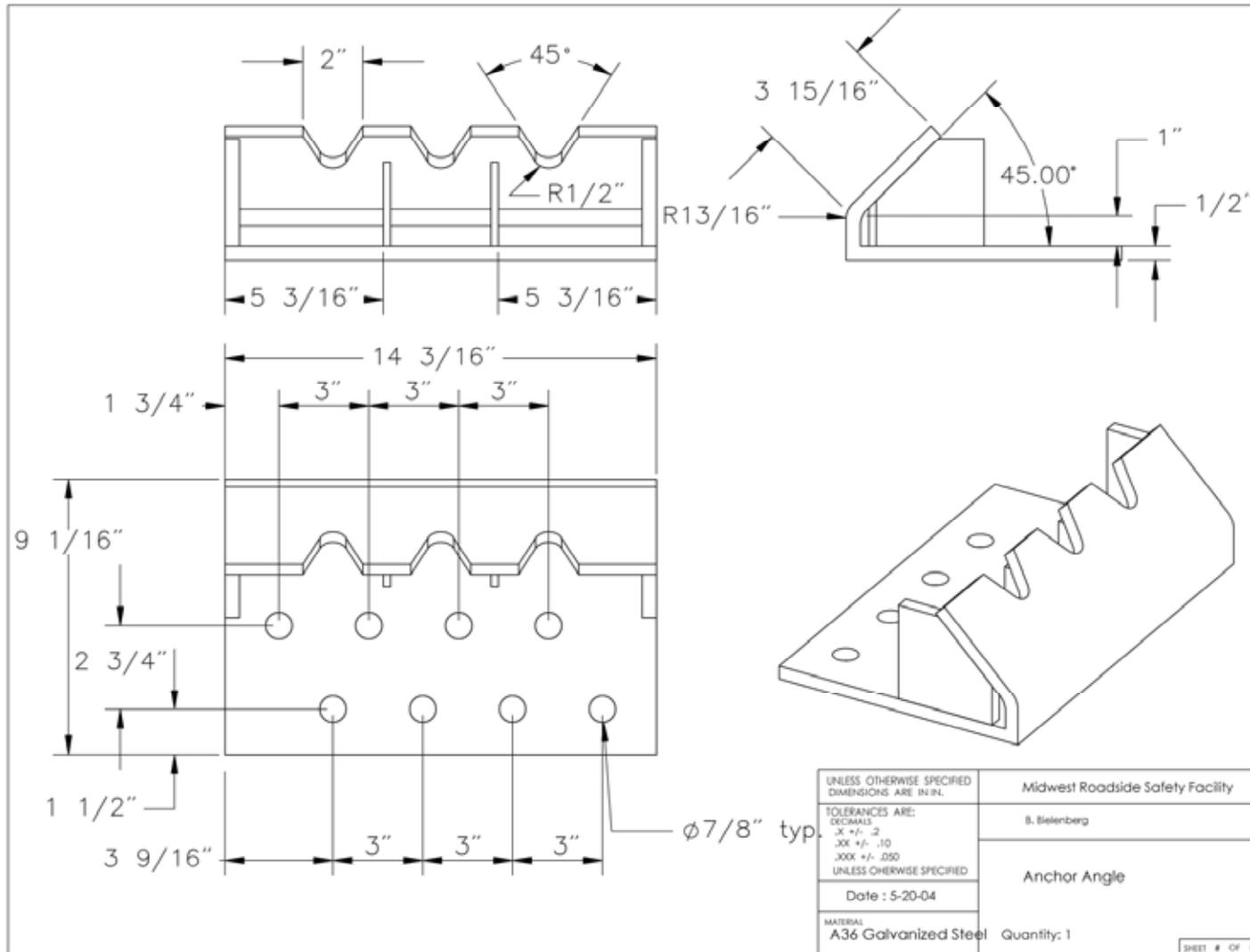
Figure 11. Modified NY Cable Anchorage Details
