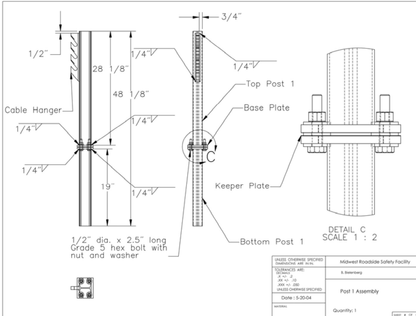
Figure 3. Modified NY Cable Anchorage Details
