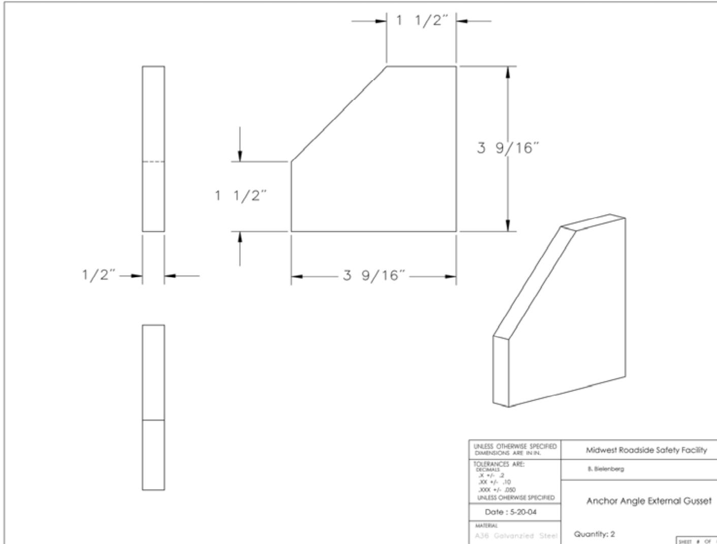
Figure 12. Modified NY Cable Anchorage Details
