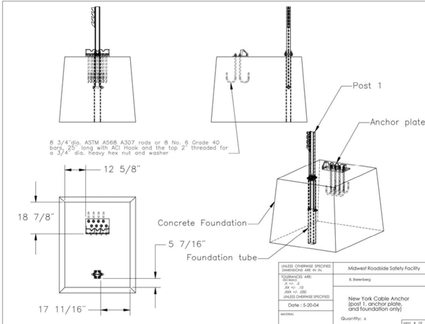
Figure 2. Modified NY Cable Anchorage Details
