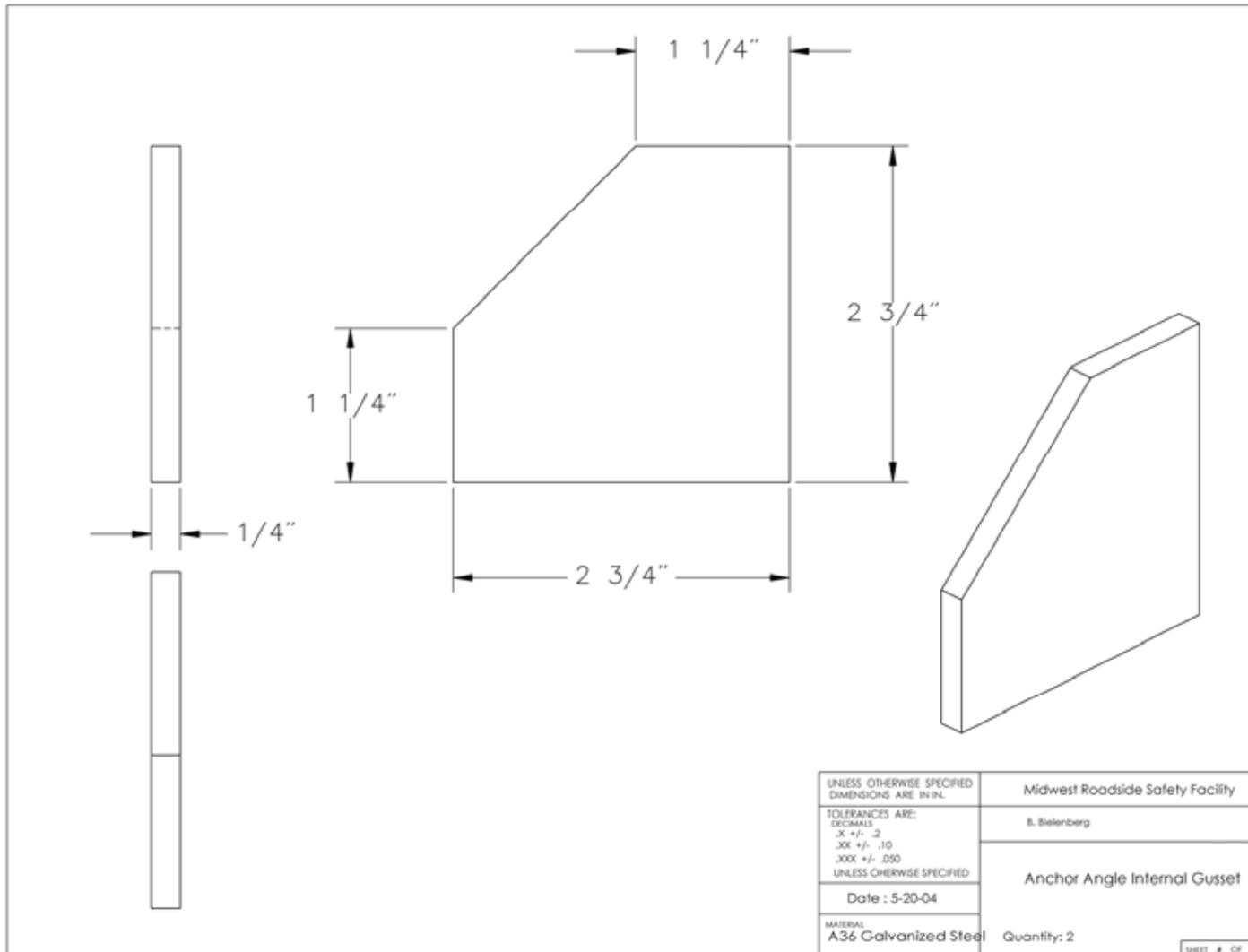
Figure 13. Modified NY Cable Anchorage Details
