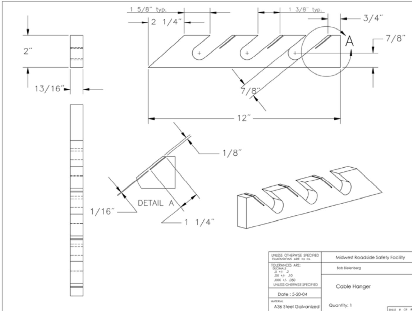
Figure 9. Modified NY Cable Anchorage Details
