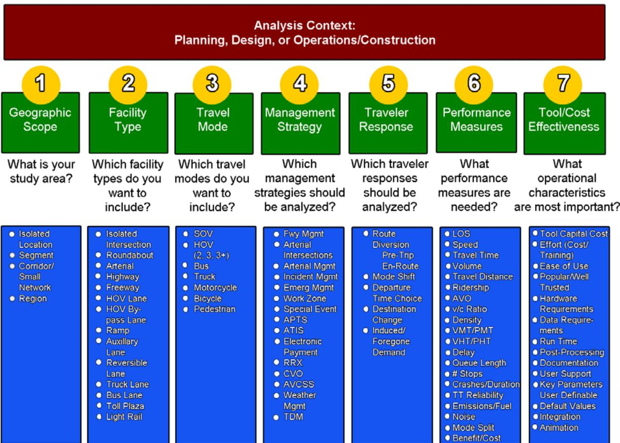
**Figure 9. Flowchart. Overview of analysis factors to be considered in selecting an analysis methodology/tool.<sup>(6)</sup>**
