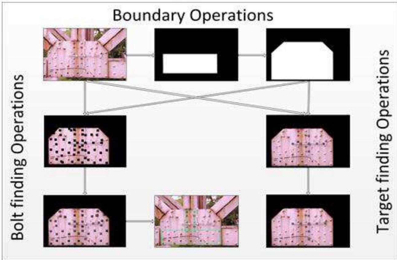
Figure 1. Process for image processing of gusset plate.
