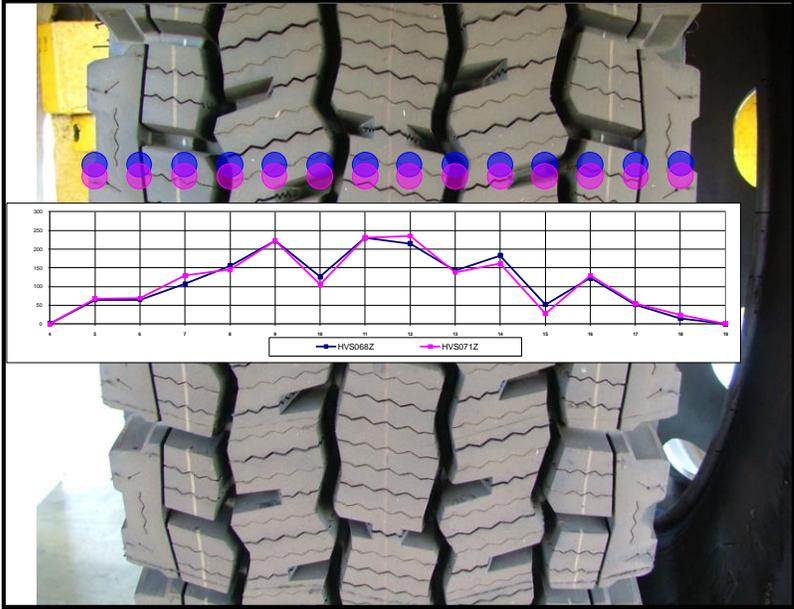
**Figure 3. Sample approximate lateral position of the tire over the instrumented pins.**
