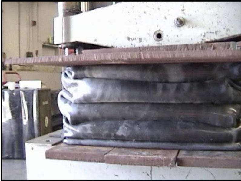
**Figure 6-10 Fully Compressed Module, About 10" Deep**
