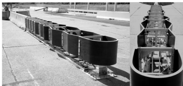
Figure 4-12 Hybrid Energy Absorbing Reusable Terminal (HEART™) System
