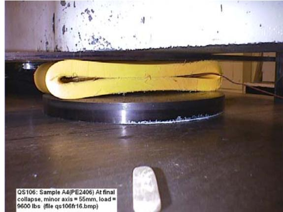
**Figure 6-8 Sample at Near Flat State**
