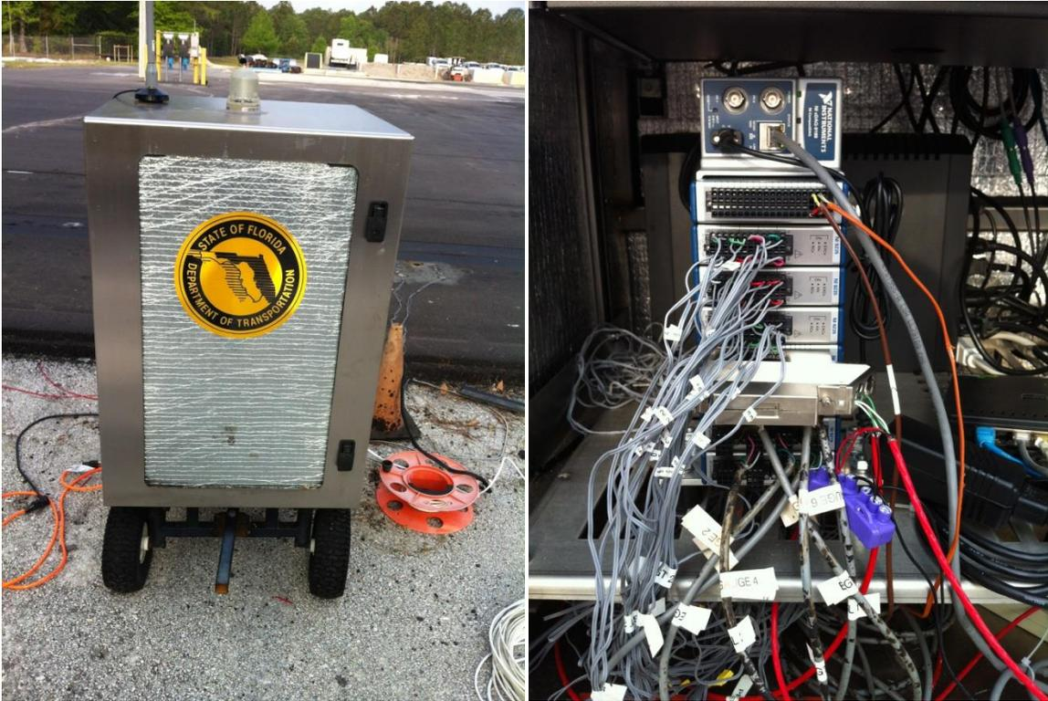
**Figure 48. Mobile DAQ system**
