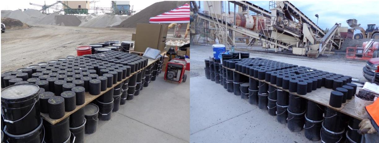
**Figure 37. Compacted samples of intermediate and surface layers**
