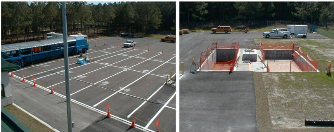
**Figure 43. HVS Test tracks and test pits**
