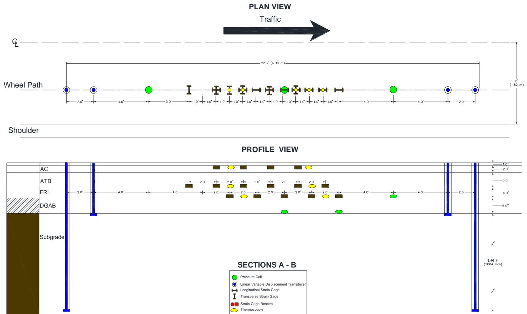
**Figure 20. Pavement structure and instrumentation of Sections A and B (13-in thick)**
