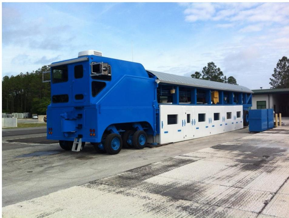
**Figure 44. Insulated panels on HVS**
