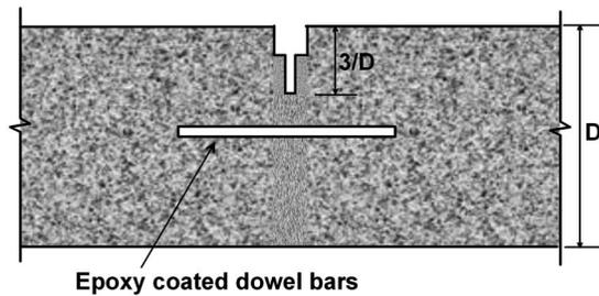
Fig. 3. Cross section of the joints in pavement
