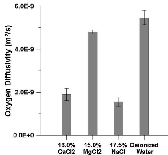
Figure 5: Oxygen diffusivity results
