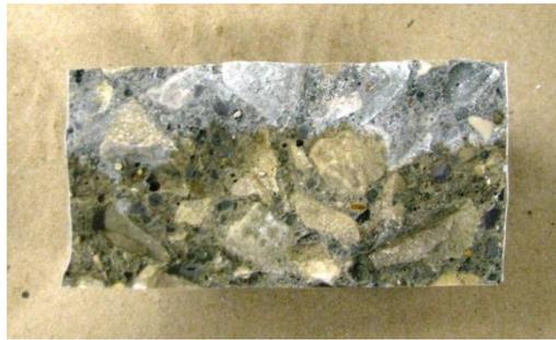
**Figure 4 – A Sample from the Rapid Chloride Migration (RCM) test that was split after and sprayed with Silver Nitrate (AgNO<sub>3</sub>). The white portion of the sample at the top represents the chloride penetration while the brown area represents the portion of the concrete that has not received substantial chloride penetration. The sample is 101 mm (4 in wide) and 50 mm (2 in tall).**
