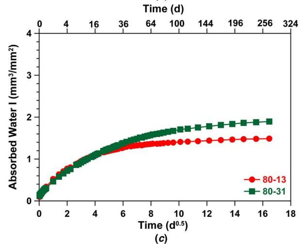
**Fig. 8.** Effect of air content and initial moisture on water absorbed: (a) 50% RH; (b) 65% RH; (c) 80% RH
