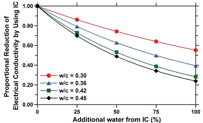
**Fig. 9.** Proportional reduction of electrical conductivity of 1-year-old saturated, internally cured samples
