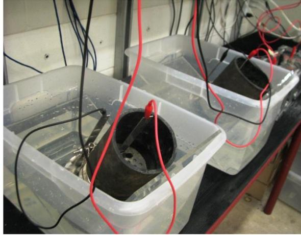
**Figure 3 – Rapid Chloride Migration (RCM) experimental set up.**
