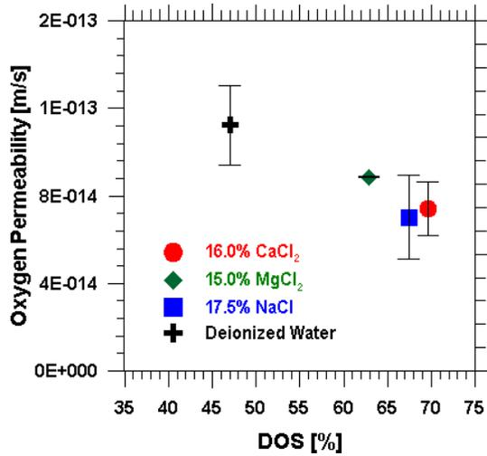
Figure 6: Oxygen permeability versus degree of saturation (DOS)
