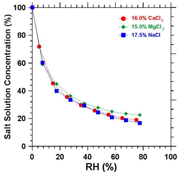
Figure 10: Salt solution concentration as a function of drying
