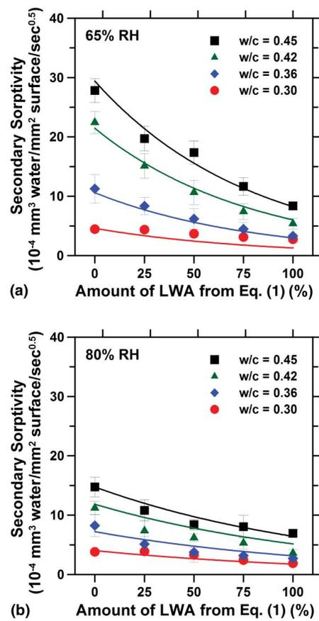
**Fig. 5.** Secondary sorptivity as a function of the  $w/c$  and the amount of LWA for samples conditioned at (a) 65% RH, (b) 80% RH; error bars represent standard deviation of 3 samples; continuous lines represent empirical equations described subsequently
