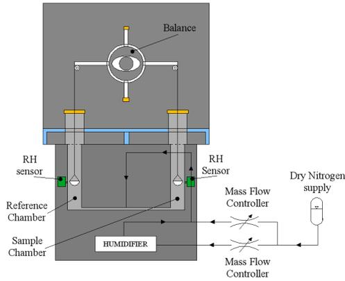
Figure 3: Schematic of automatic sorption/desorption analyzer
