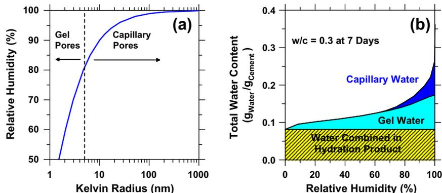
Fig. 1. Relation between relative humidity and partially empty pores in cement paste.
