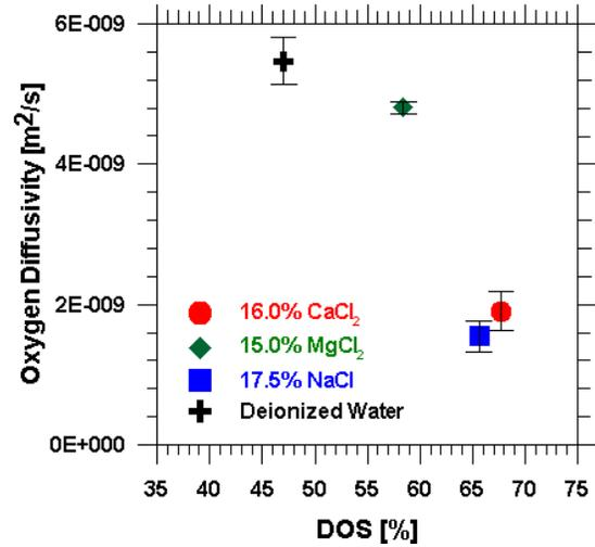
Figure 7: Oxygen diffusivity versus degree of saturation (DOS)
