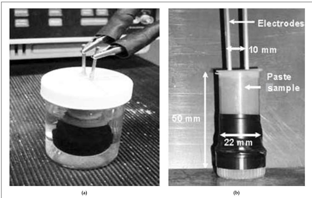
**Figure 1. An illustration of the apparatus used for the measurement of electrical conductivity of cement pastes (a) The conductivity cell for cement pastes immersed in a water bath (b) The vial with embedded electrodes for paste and pore solution conductivity assessment**
