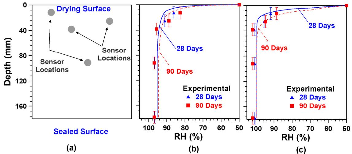
Figure 5: Comparison of the experimentally measured relative humidity and numerically obtained relative humidity profile, (a) illustration of location of the sensors and boundary conditions of the slab, (b) plain mortar, (c) mortar with 5% shrinkage reducing admixture (SRA)
