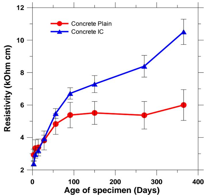
Figure 10 – Electrical resistivity if the plain and an internally cured concrete samples kept in lime water during the testing period.
