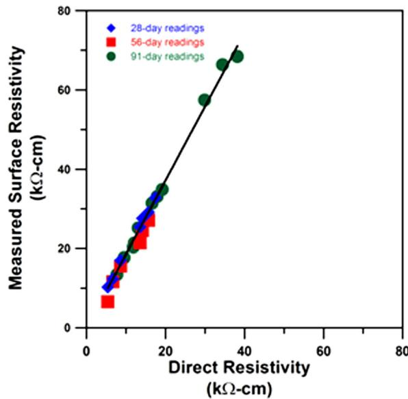
FIG. 4—Correlation of measured SR and BR of samples of differing ages; each data point represents the average of three samples.
