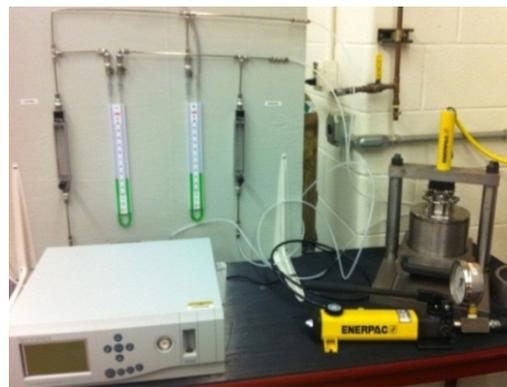
Figure 2: Oxygen diffusivity test device
