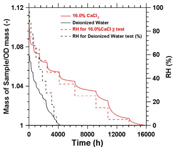
Figure 9: Mass change during each RH step for samples submerged in 16% calcium chloride and deionized water. Solid lines show the change in mass, while dashed lines show the RH steps.
