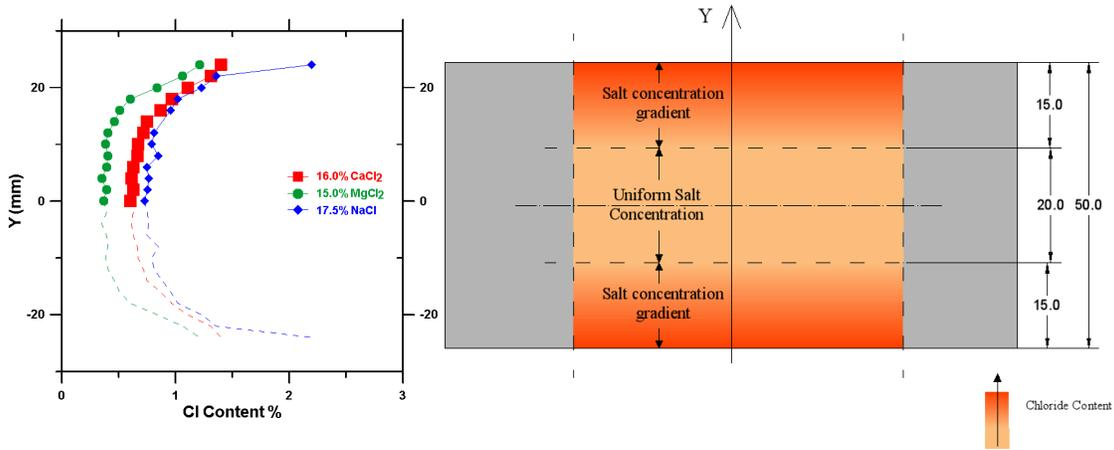
Figure 11: Chloride Profiles in Oxygen Diffusivity Sample
