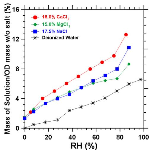
Figure 8: Desorption curves for mortar samples submerged in salt water solutions
