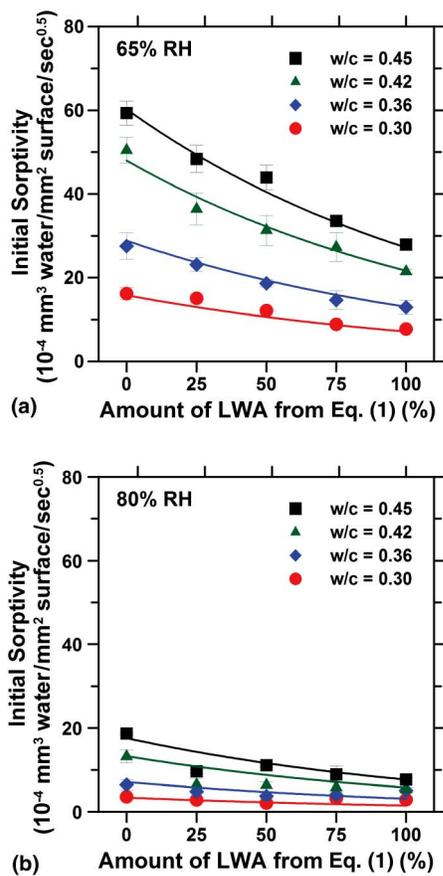
**Fig. 4.** Initial sorptivity as a function of  $w/c$  and the amount of LWA for samples conditioned at (a) 65% RH, (b) 80% RH; error bars represent standard deviation of 3 samples; continuous lines represent empirical equations described subsequently
