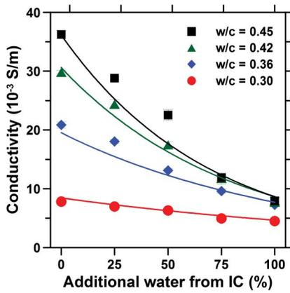
**Fig. 7.** Electrical conductivity of vacuum-saturated samples at 365 days; error bars represent the standard deviation of 3 samples; continuous lines represent empirical relations described subsequently
