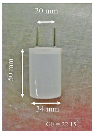
Fig. 2. Mold used for continuous electrical conductivity measurements
