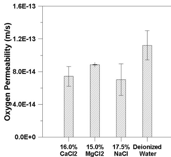
Figure 4: Oxygen permeability results
