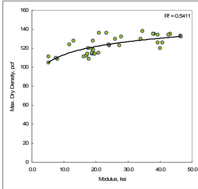
Figure 15. Maximum dry density versus subgrade modulus of coarse-grained soils (1 ksi = 6.89 MPa; 1 pcf = 1 kg/m<sup>3</sup>)
