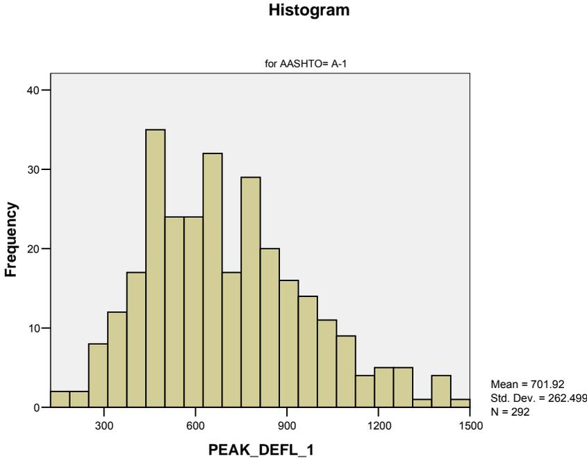
Figure 3. Histogram for deflection (PEAK\_DEFL\_1) data for A-1 soils (deflection in µm)
