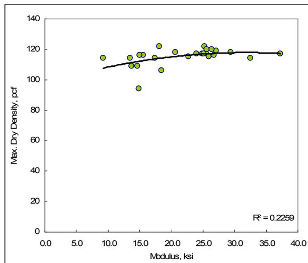
Figure 16. Maximum dry density versus subgrade modulus of fine-grained soils (1 ksi = 6.89 MPa; 1 pcf = 1 kg/m<sup>3</sup>)
