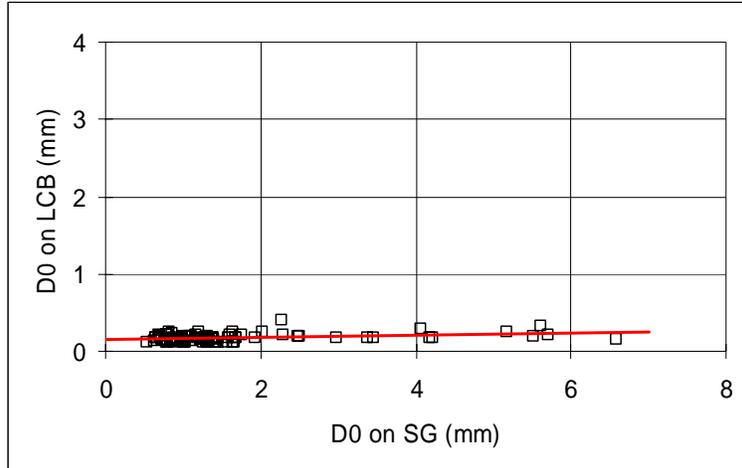
Figure 18. Lean Concrete Base Deflection Comparison (1 mm = 39.37 mil)
