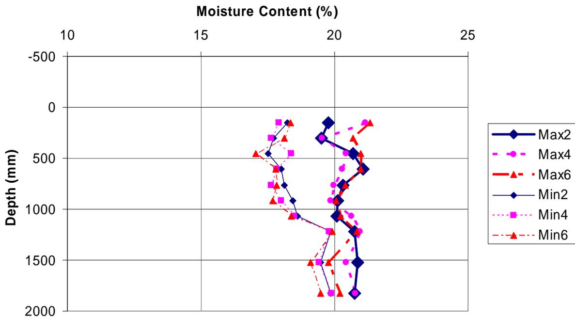
Figure 3. Range of Moisture Content Variation and Max/Min Moisture Content as a Function of Depth (Ohio Section 390104 ATB) (100 mm = 3.94 in)
