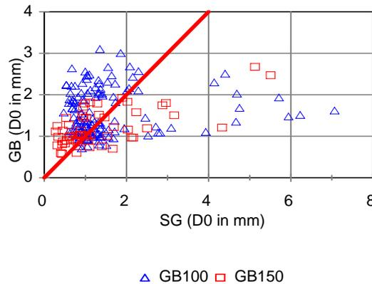
Figure 15. Thin Granular Base Deflection Comparison (1 mm = 39.37 mil)
