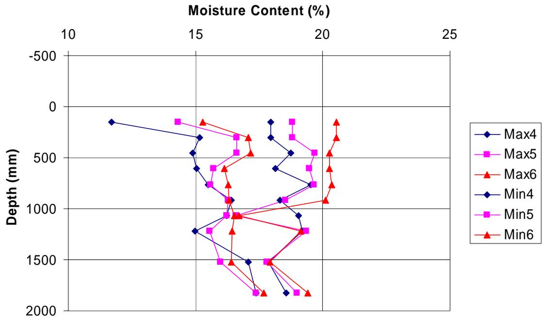
Figure 4. Range of Moisture Content Variation and Max/Min Moisture Content as a Function of Depth (Ohio Section 390208 LCB) (100 mm = 3.94 in)
