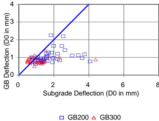
Figure 16. Thick Granular Base Deflection Comparison (1 mm = 39.37 mil)
