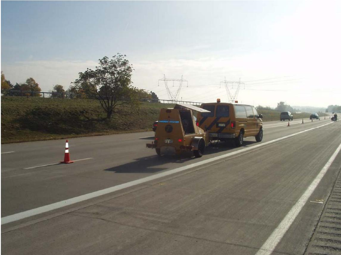
Figure 17. Falling Weight Deflectometer attached to a van
