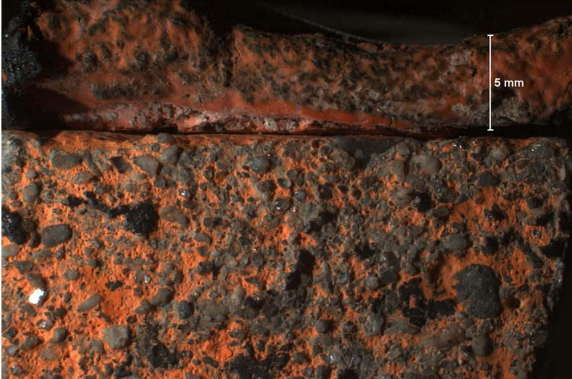
SAMPLE ID: D DESCRIPTION: Mortar-eroded top surface mostly cleaned of orange marking paint.
