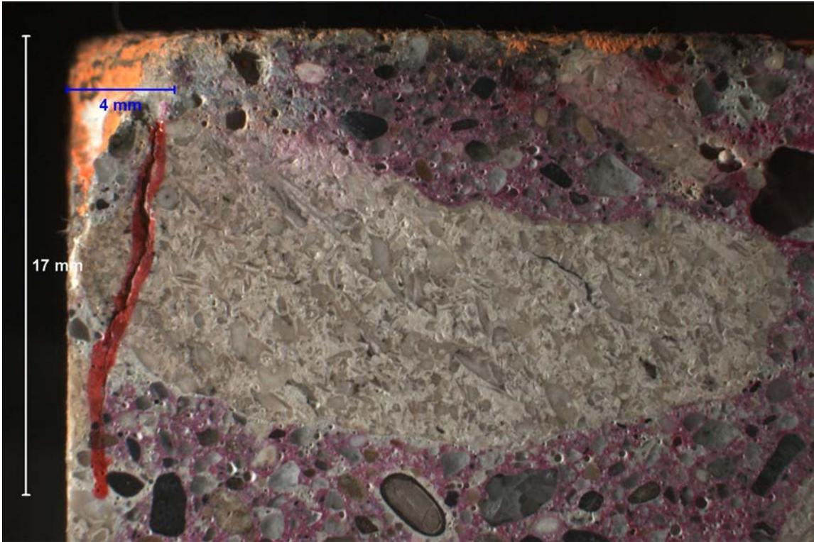
SAMPLE ID: D DESCRIPTION: Incipient sliver spalling in sawcut and lapped cross section of concrete at joint (left).
