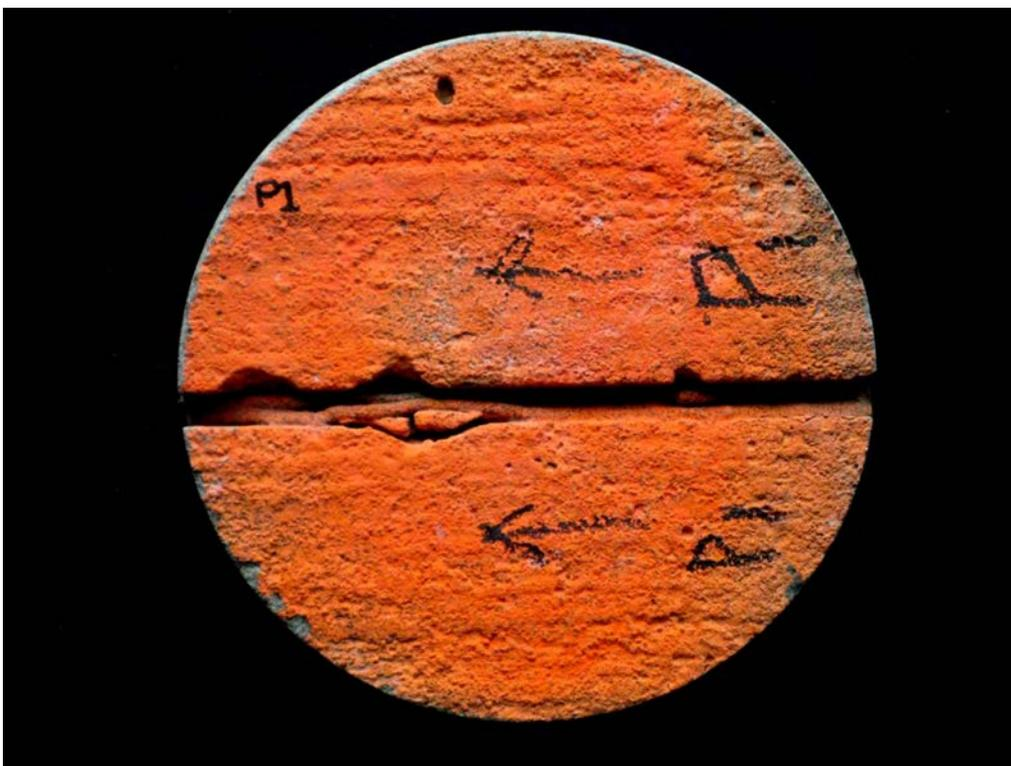
SAMPLE ID: P1 DESCRIPTION: Top surface of the core as received; covered by orange marking paint. Note core was taken through a sawcut control joint; which exhibits intermittent “sliver spalling”. The joint was filled with hot-pour joint sealant.
