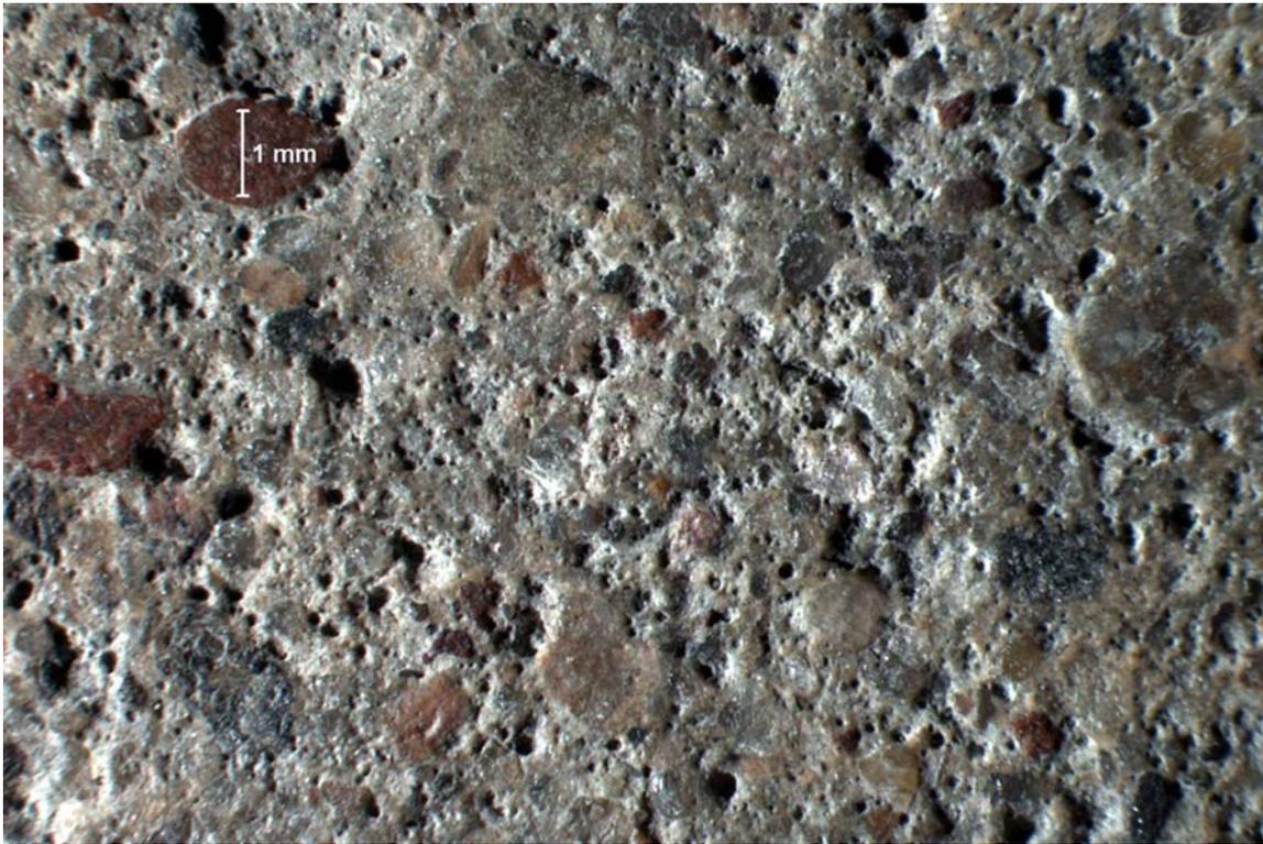
SAMPLE ID: FG3 DESCRIPTION: Traffic-worn top surface of the concrete under magnification
