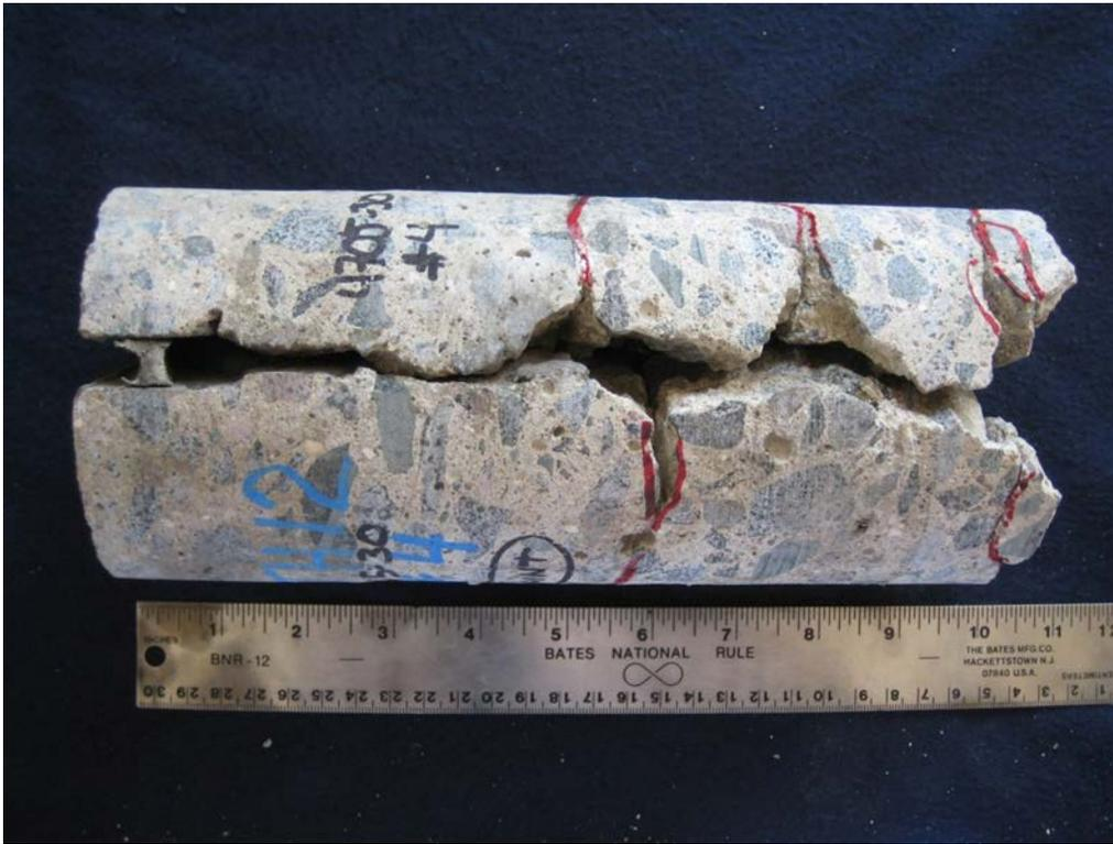
SAMPLE ID: 4, 4705-30 DESCRIPTION: Core sample taken directly through a pavement joint, as received. Top surface is left. Existing fractures are mapped in red ink.
