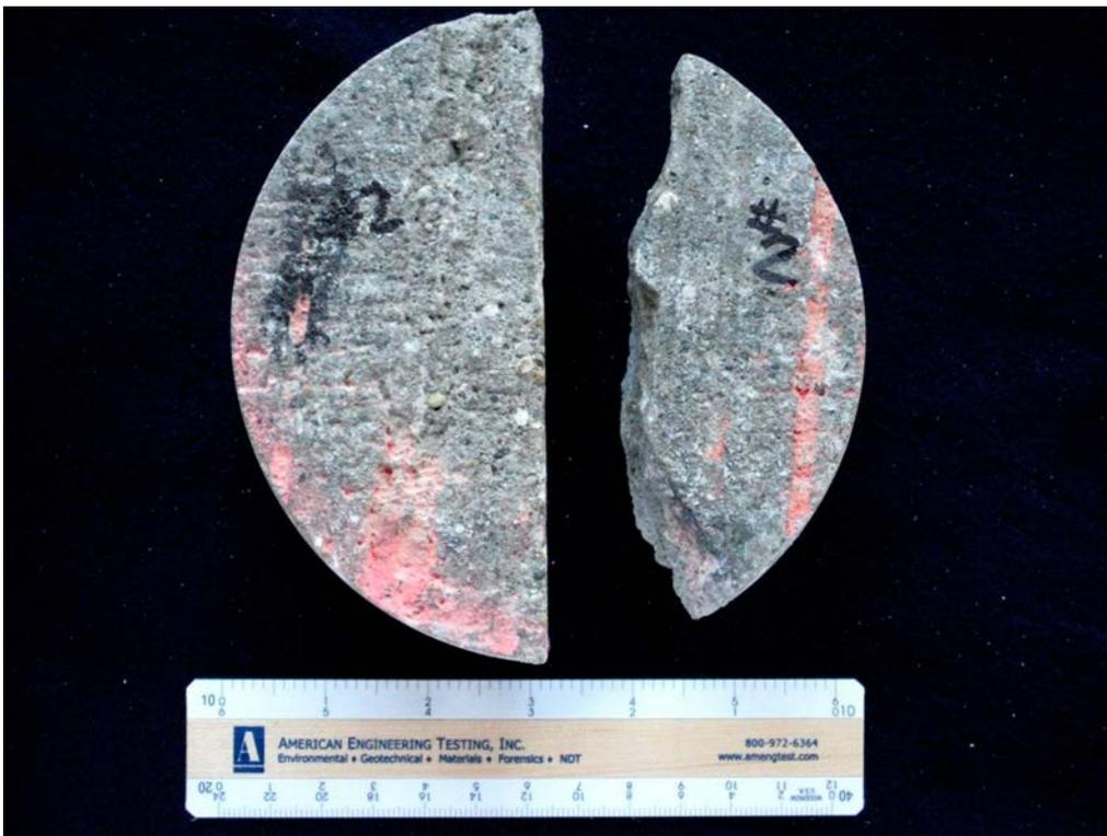
SAMPLE ID: #2 DESCRIPTION: The top surface of the core sample, taken directly through a joint, as received.
