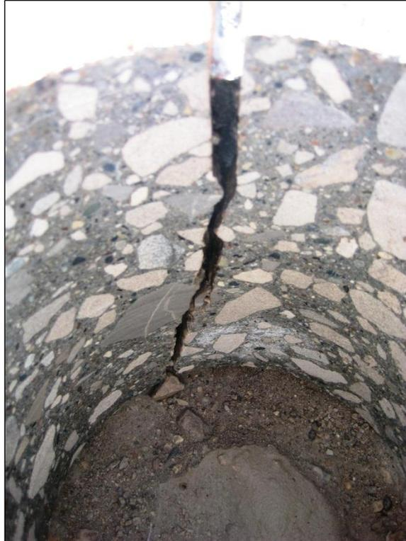
**Figure 3. Faulting and loss of aggregate interlock**
