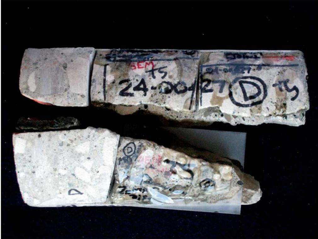
SAMPLE ID: D DESCRIPTION: Locations of the thin section produced for analysis.
