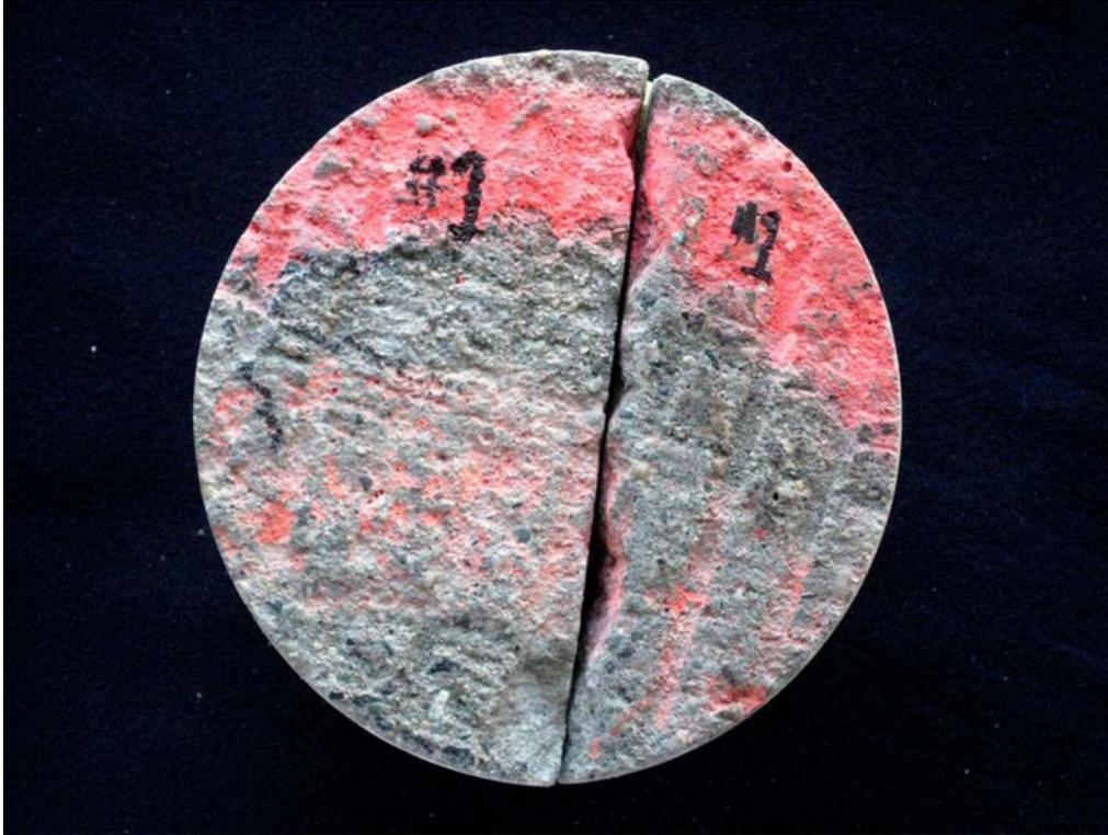
SAMPLE ID: #1 DESCRIPTION: Top surface of the core sample, taken directly through a joint, as received.
