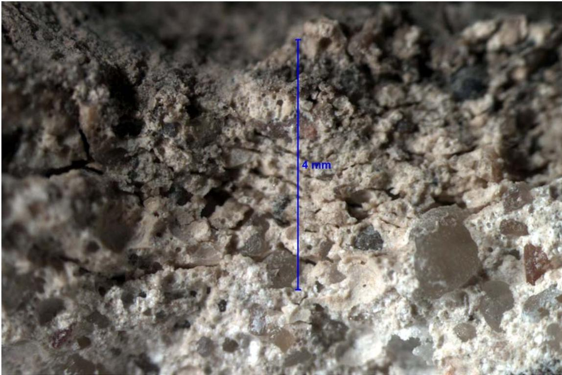
SAMPLE ID: FG1 DESCRIPTION: Highly concentrated anastomosing microcracking in carbonated paste directly adjacent to distressed joint plane (top of image); in freshly fractured cross sectional surface of core.
