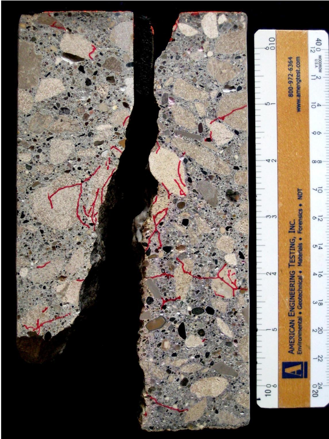
**SAMPLE ID:** D    **DESCRIPTION:** Sawcut and lapped cross section of core taken through joint. Microcracking is mapped in red ink. Note mass lost along the joint crack and cracking within coarse aggregate particles.
