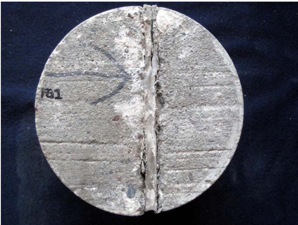
SAMPLE ID: FG1 DESCRIPTION: Top surface of the core as received. Note core was taken through a sawcut and silicone sealed control joint.
