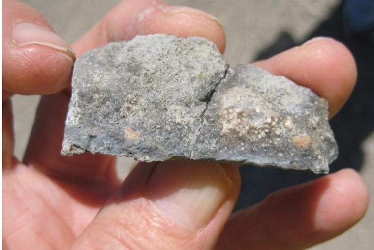
**Figure 2. Sample removed piece showing that material between the free surface and the new crack is reasonably sound with coarse aggregate particles free of paste**
