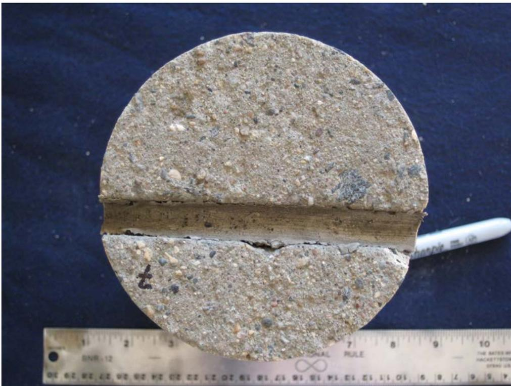
SAMPLE ID: 7, 4705-30 DESCRIPTION: Top surface of the core as received. Note core was taken through a sawcut and silicone sealed control joint.
