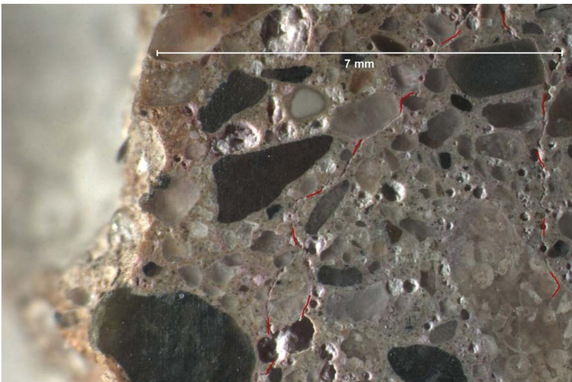
SAMPLE ID: D DESCRIPTION: The great majority of fine spherical entrained air voidspaces at 98mm depth in the core and directly adjacent to the distressed joint (left) are filled with secondary ettringite. Microcracking, oriented sub-parallel to the distressed joint plane, is marked in red dashed line.
