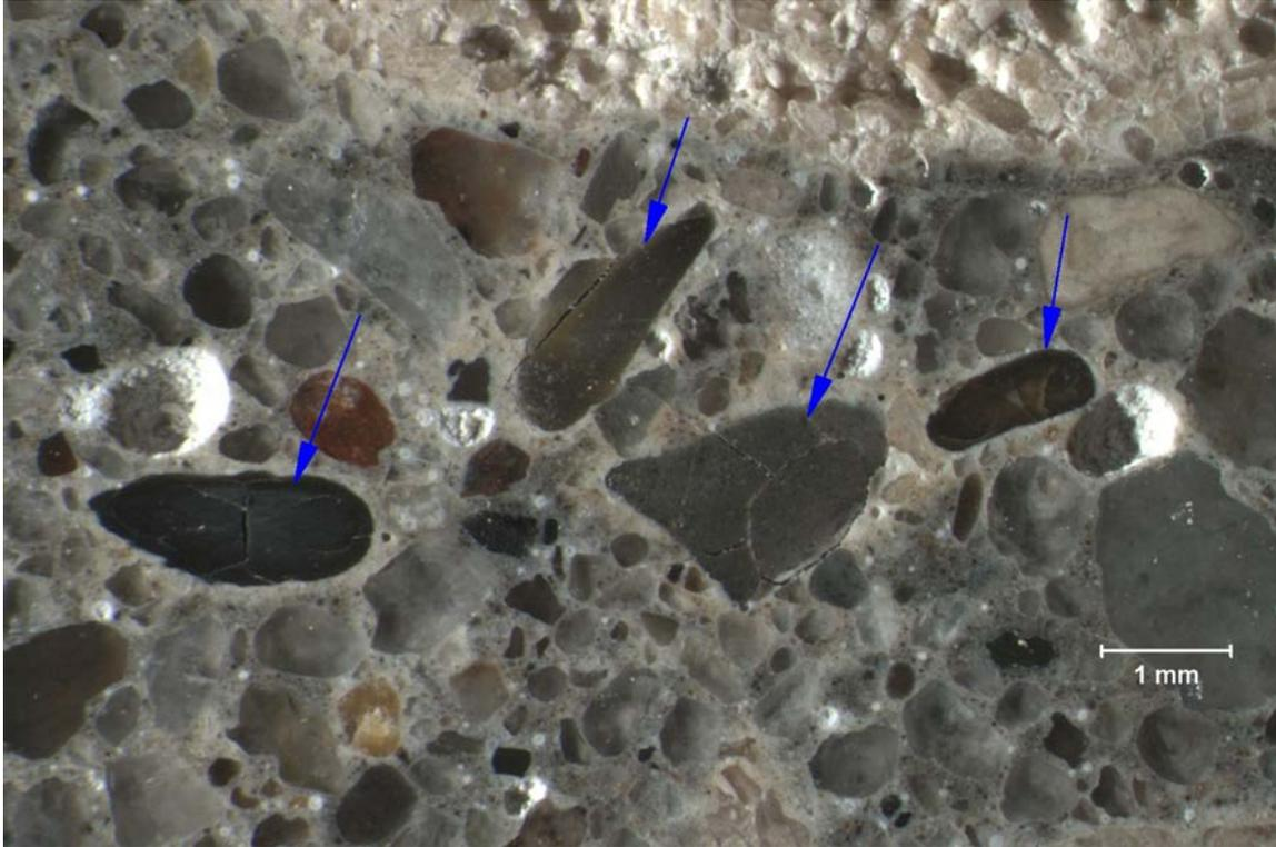
SAMPLE ID: P1 DESCRIPTION: Abundant reactive shale particles at depth in the core.
