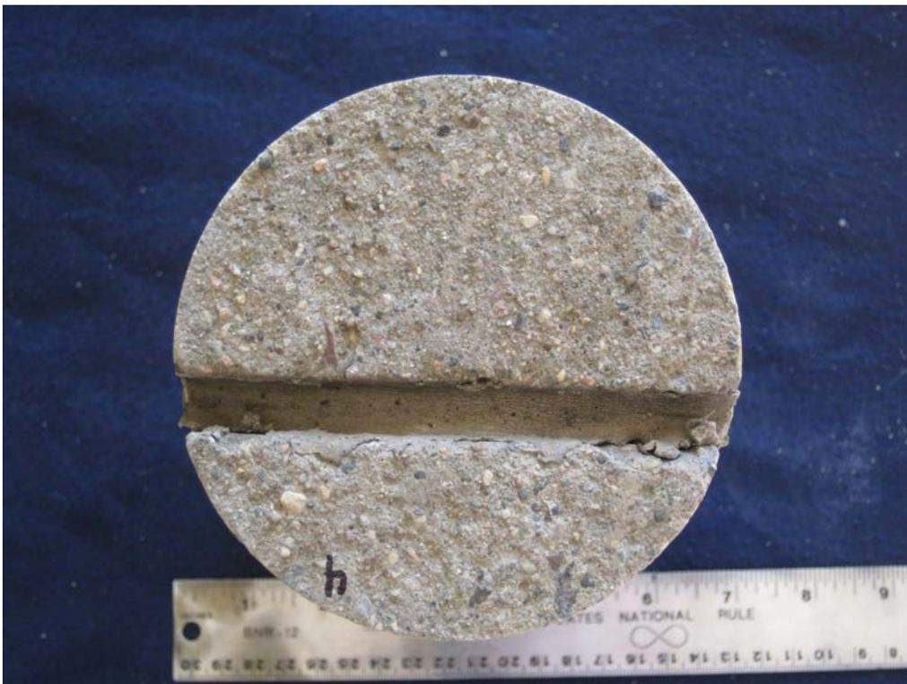
SAMPLE ID: 4, 4705-30 DESCRIPTION: Top surface of the core as received. Note core was taken through a sawcut and silicone sealed control joint.
