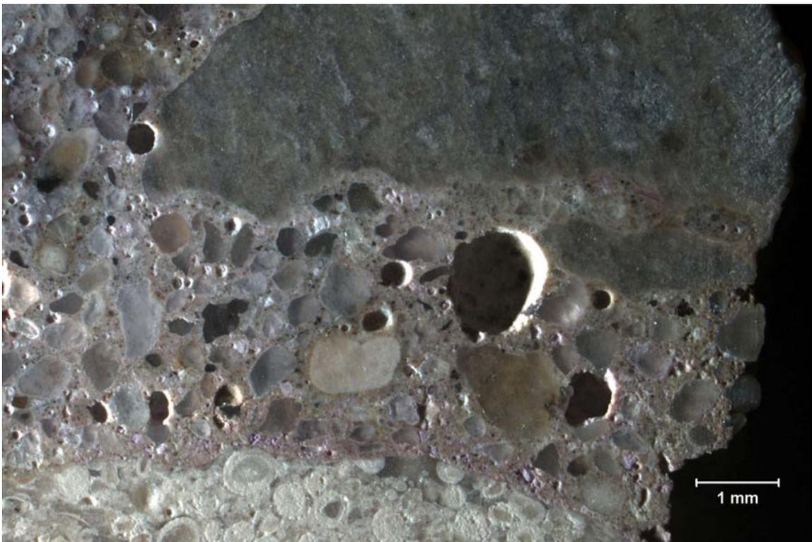
SAMPLE ID: #1 DESCRIPTION: Much of the air voids proximate to the joint and at 140mm depth from the top surface are filled with secondary ettringite.
