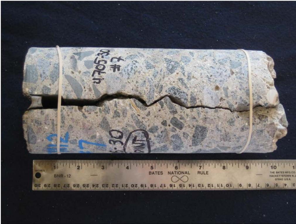
SAMPLE ID: 7, 4705-30 DESCRIPTION: Core sample taken directly through a pavement joint, as received. Top surface is left.
