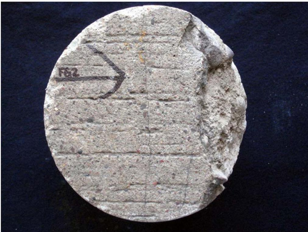
SAMPLE ID: FG2 DESCRIPTION: Top surface of the core as received. Note core was taken in distress apparently directly adjacent to a control joint..
