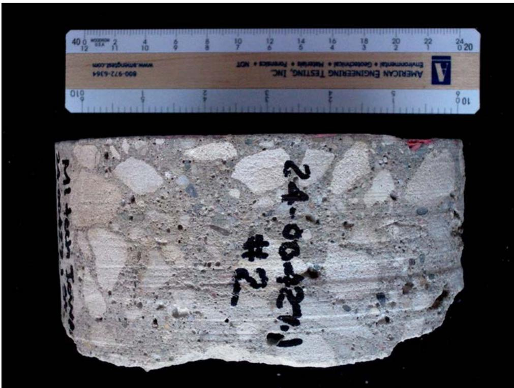
SAMPLE ID: #2 DESCRIPTION: The 75mm long core sample as received.
