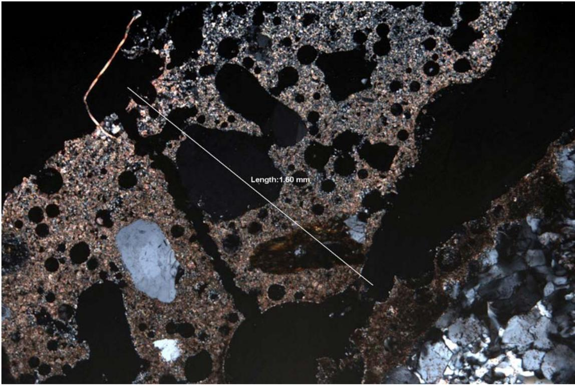
SAMPLE ID: FG2 DESCRIPTION: Brightly colored, carbonated paste directly adjacent to the distressed joint plane (upper left); in thin section under cross polarized light.
