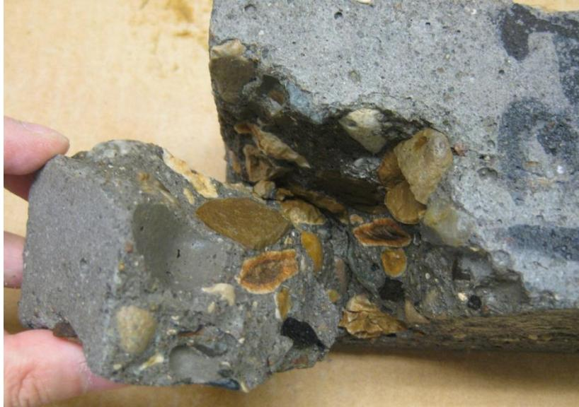
**Figure 11. Laboratory observation of distress incurred during freezing and thawing**
