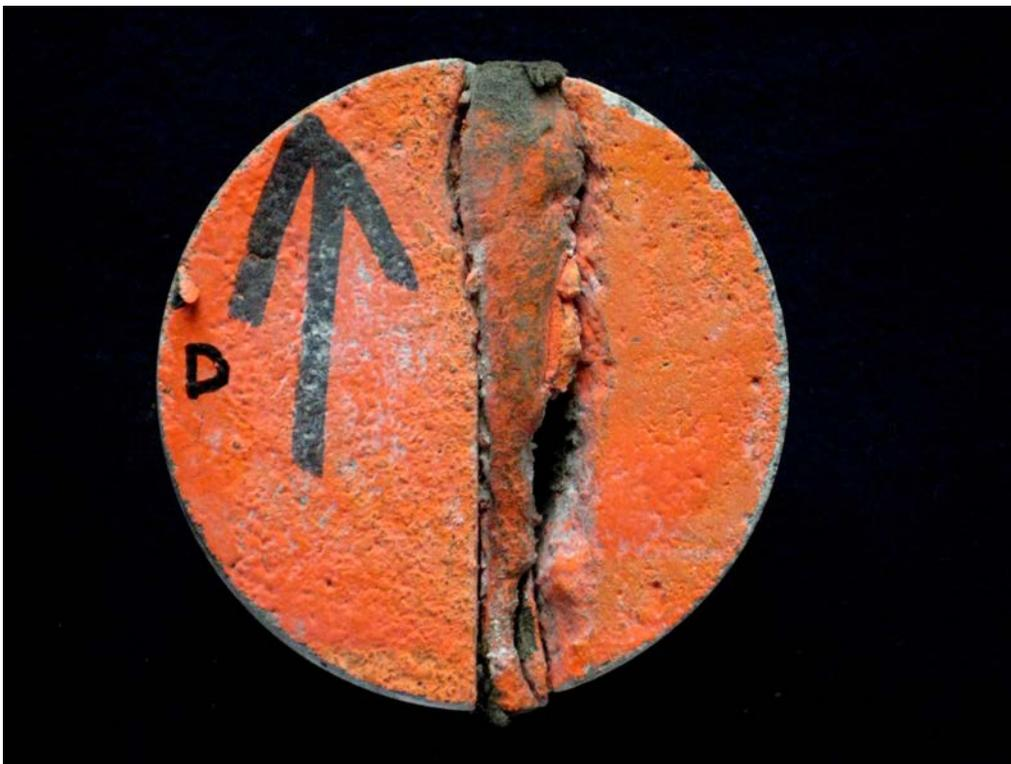
SAMPLE ID: D DESCRIPTION: Top surface of the core as received; covered by orange marking paint. Note core was taken through sawcut control joint; which subsequently "sliver spalled" and was filled with hot-pour joint sealant (now de-bonded).
