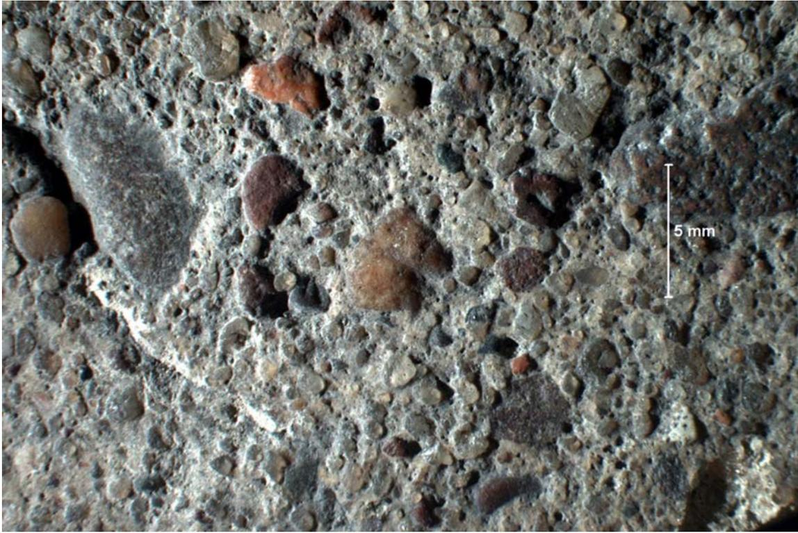
SAMPLE ID: FG4 DESCRIPTION: Traffic-worn and mortar eroded top surface of the core under magnification.
