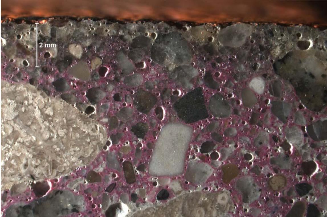
SAMPLE ID: D DESCRIPTION: Carbonation (unstained paste) to 2mm depth from the top surface, in this view.
