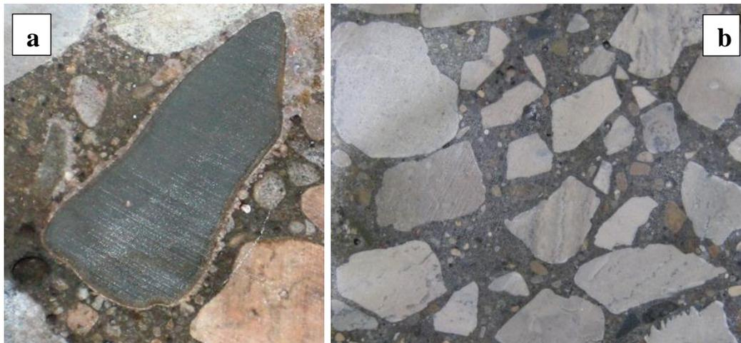
**Figure 10. Samples tested in salt, cut, then treated with silver nitrate to highlight presence of chlorides (a) 0.5 - 0%SF - gravel (b) 0.4 - 5%SF - limestone**
