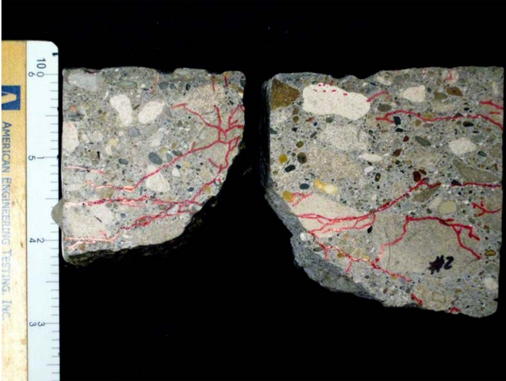
SAMPLE ID: #2 DESCRIPTION: Sawcut and lapped cross section of core taken through a distressed joint. Microcracking is mapped in red ink. Note some concentration within coarse aggregate particles.
