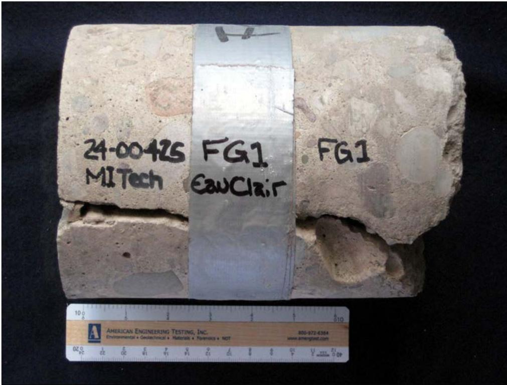
SAMPLE ID: FG1 DESCRIPTION: Core sample taken directly through a joint as received. Top surface is left.
