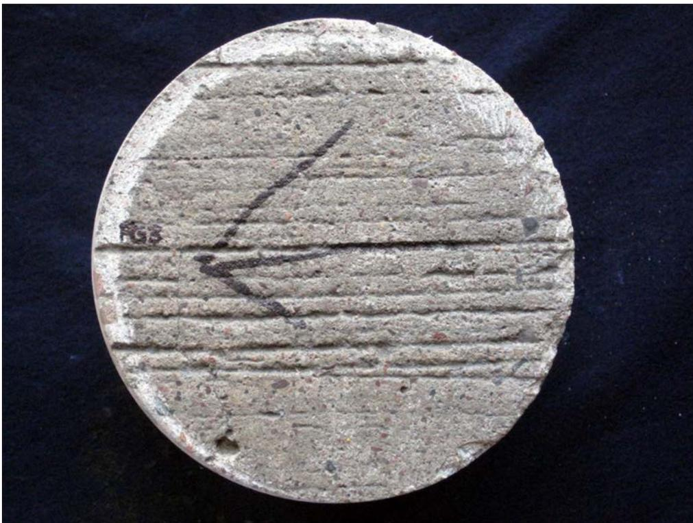
SAMPLE ID: FG3 DESCRIPTION: Screeded, tined and traffic worn top surface of the core as received.
