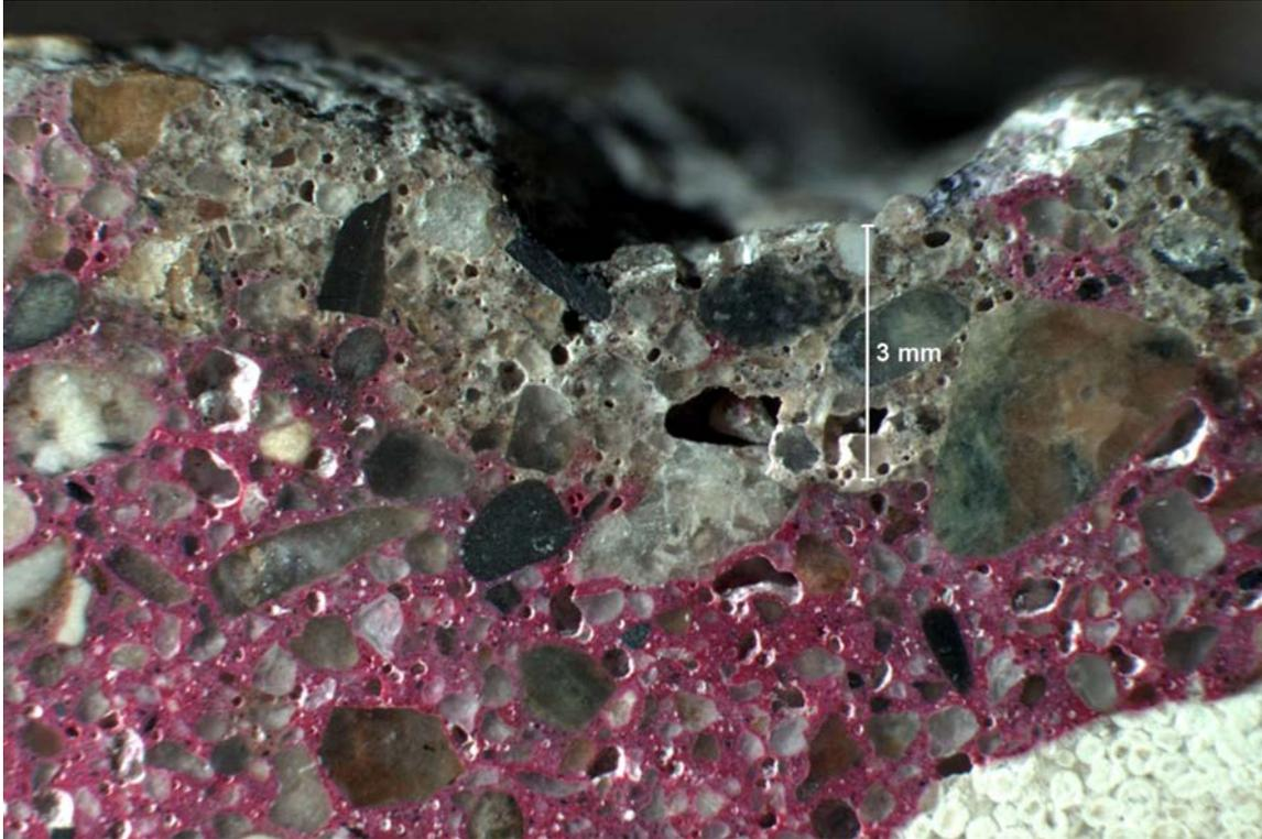
SAMPLE ID: #2 DESCRIPTION: Carbonation (unstained paste) ranges from negligible to 3mm depth from the top surface of the core. In freshly sawcut and lapped cross section of core exposed to phenolphthalein pH indicator.
