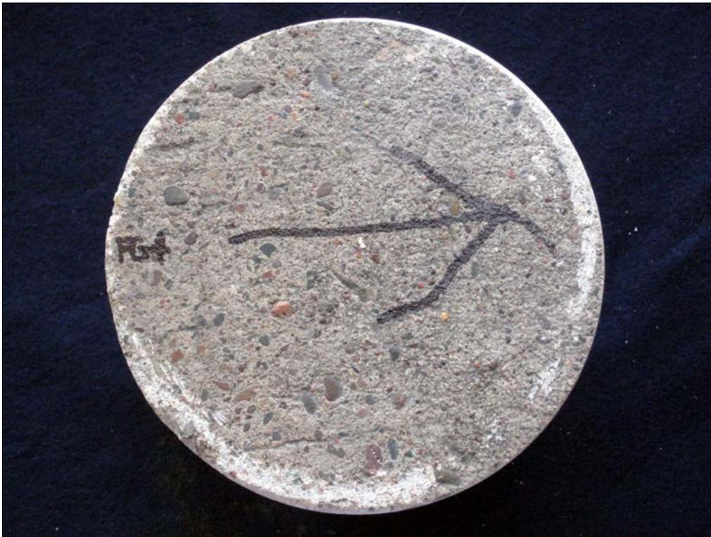
SAMPLE ID: FG4 DESCRIPTION: Mortar eroded top surface of the core as received.
