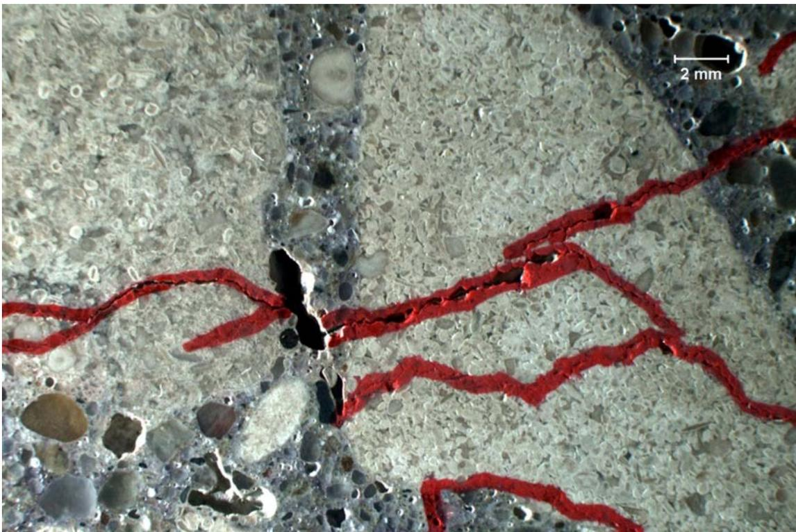
SAMPLE ID: #1 DESCRIPTION: Microcracking, proceeding through coarse aggregates at depth in the core, is mapped in red ink.
