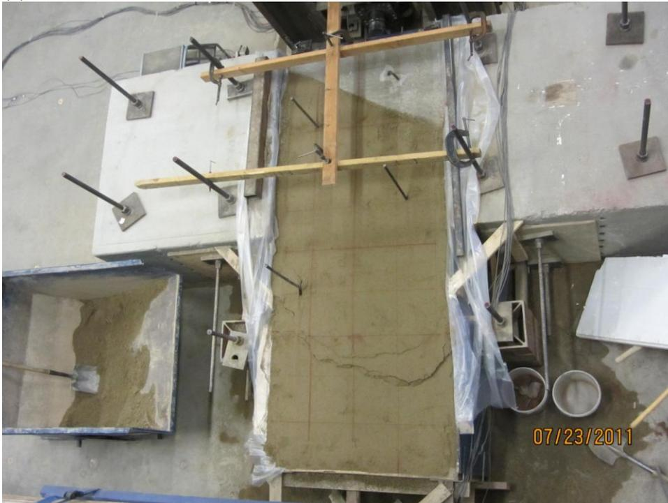
**Fig. 10: Photos of failure surface geometry at the ground surface for (a) no skew and (b) 30 degree skew tests.**
