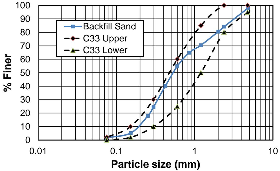
Fig. 3: Gradation for backfill sand relative to concrete sand gradation.
