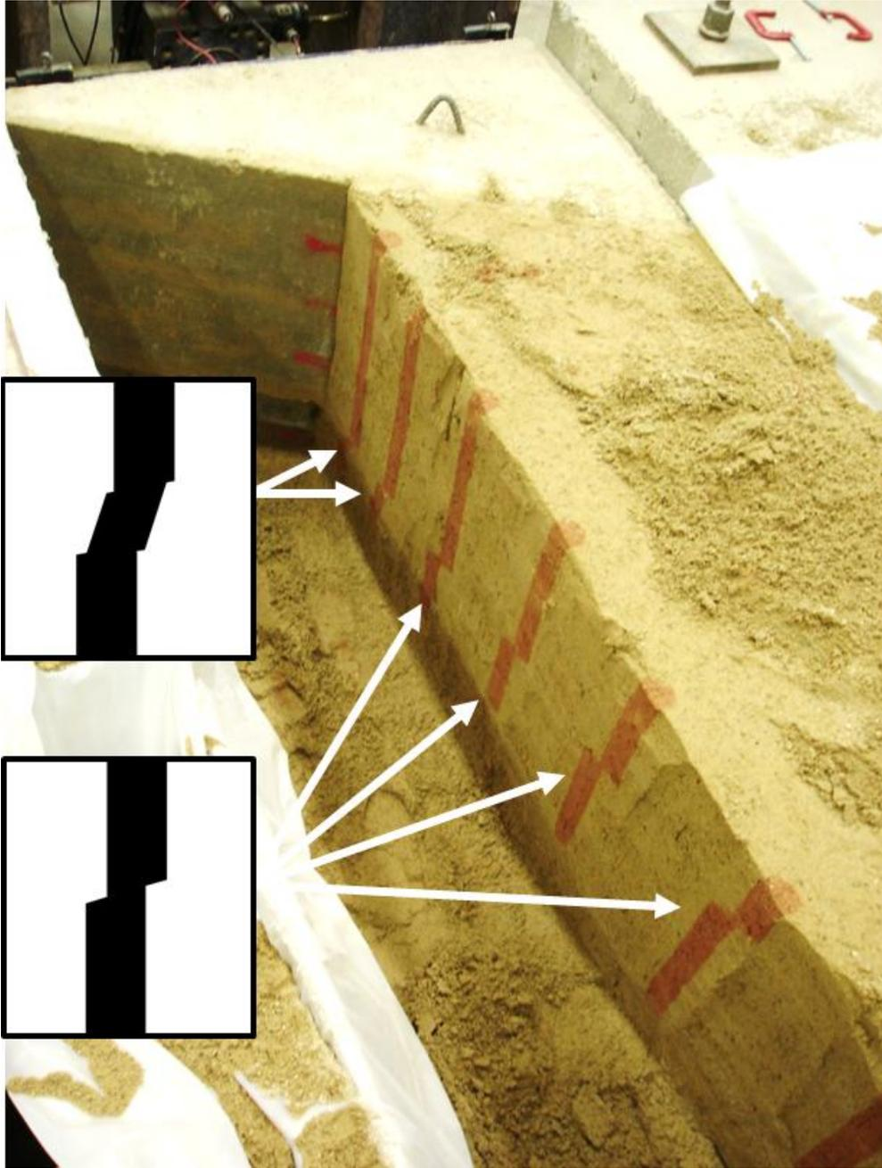
**Fig. 11: Photograph showing failure surface geometry determination within sand based on offset in red sand columns for 30 degree skew test.**
