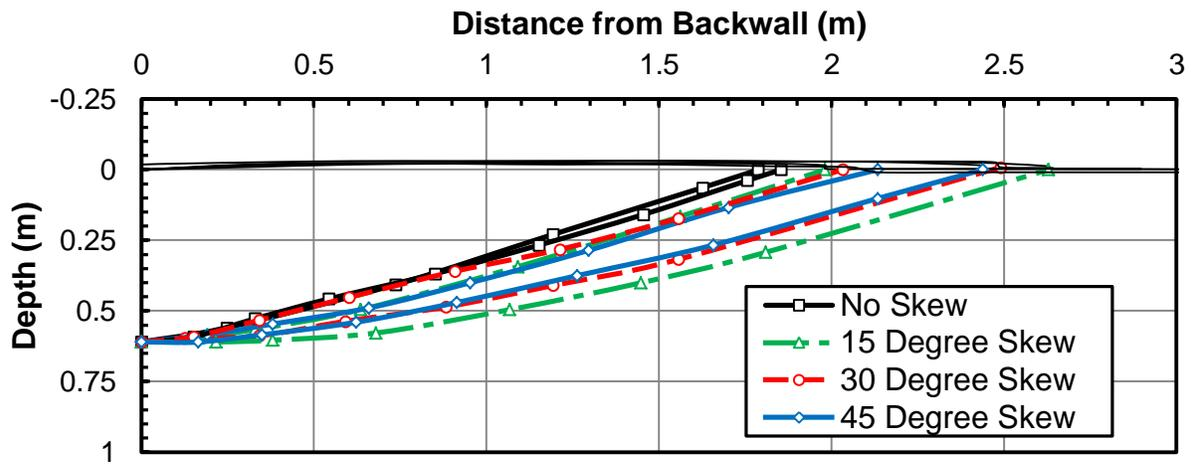
**Fig 12: Failure surface geometry and ground surface heave as a function of distance behind the wall for tests at various skew angles.**
