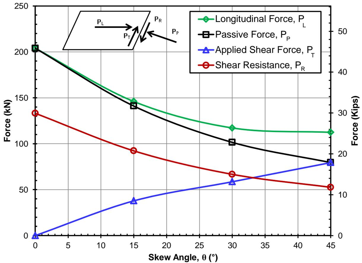
**Fig. 9: Plot of longitudinal force ( $P_L$ ), passive force ( $P_P$ ), transverse shear resistance ( $P_R$ ) and applied shear force ( $P_T$ ) as a function of skew angle ( $\theta$ ).**
