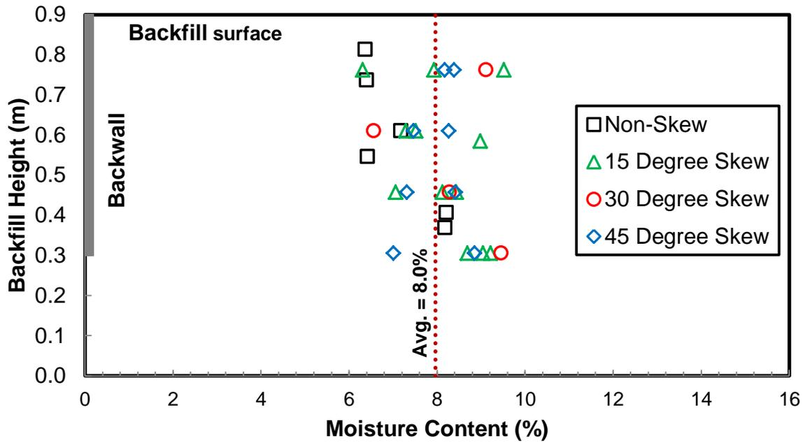
**Fig. 5: Plot of moisture content versus depth for the various skew tests based on samples obtained immediately after tests.**
