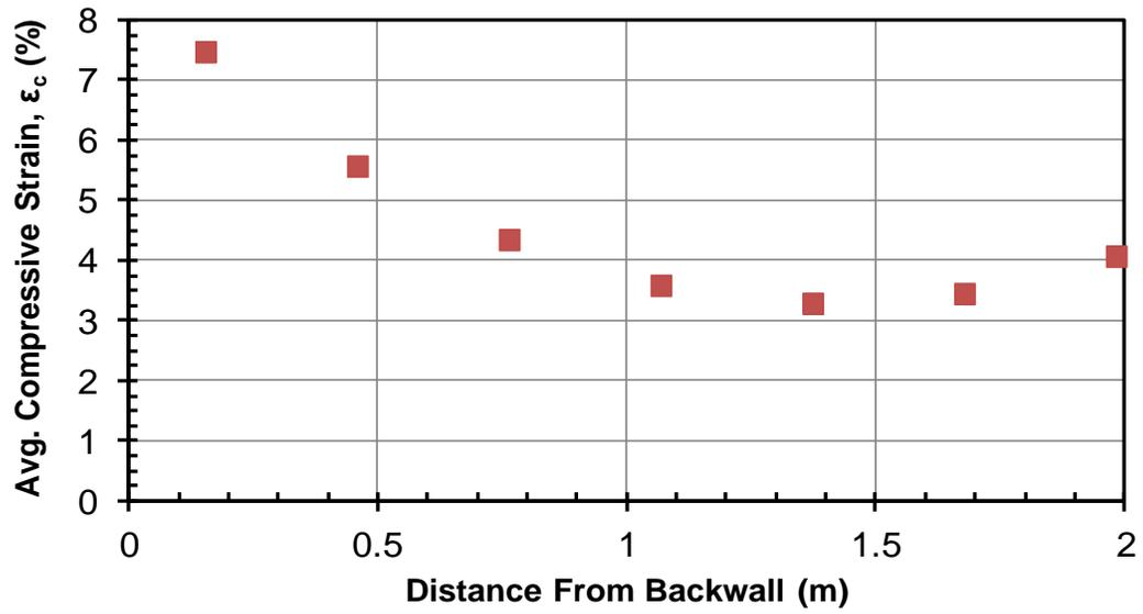
**Fig. 14: Average compressive strain as a function of distance behind the wall based on ground surface displacement measurements for all tests.**
