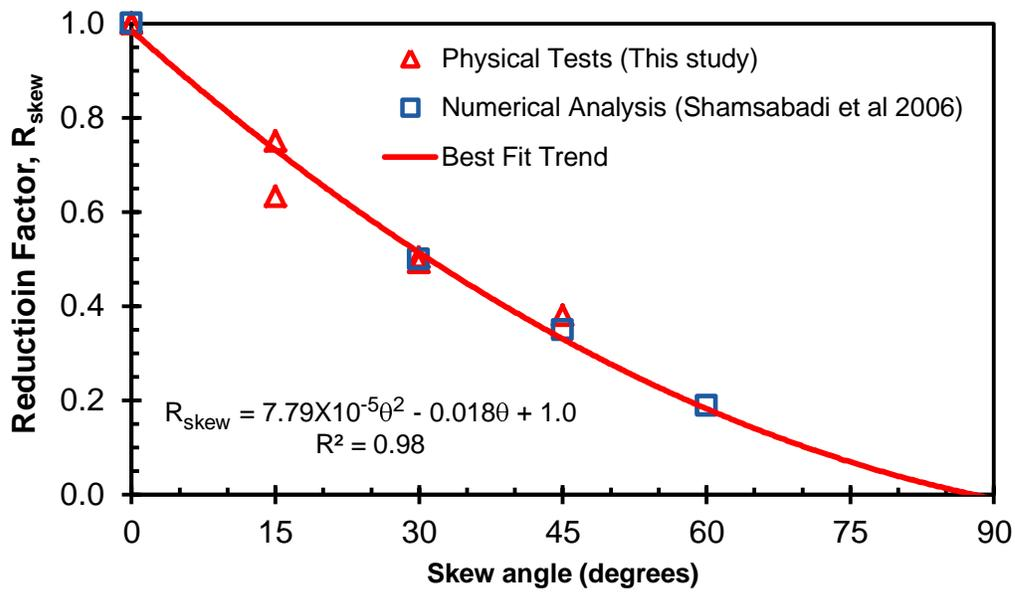
**Fig. 7: Provisional reduction Factor,  $R_{skew}$ , (passive force for a given skew angle normalized by passive force with no skew) plotted versus skew angle based on physical test results and numerical analyses.**
