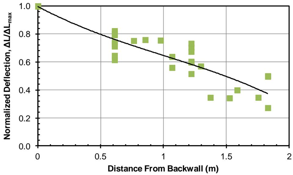
**Fig. 13: Plots of longitudinal ground surface displacement as a function of distance behind the wall for various skew angles.**
