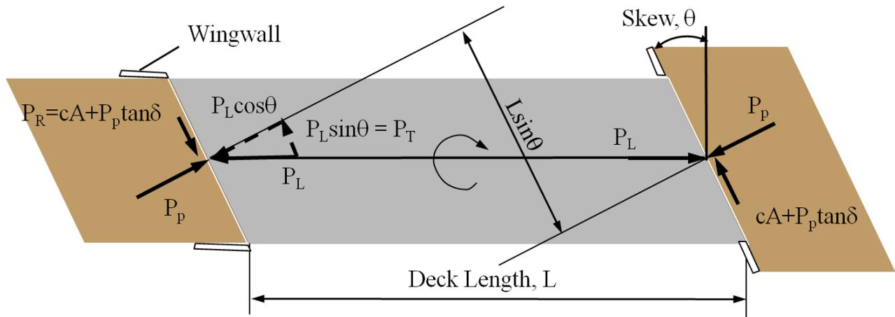
**Fig. 1: Typical distribution of forces on a bridge with a skewed abutment.**
