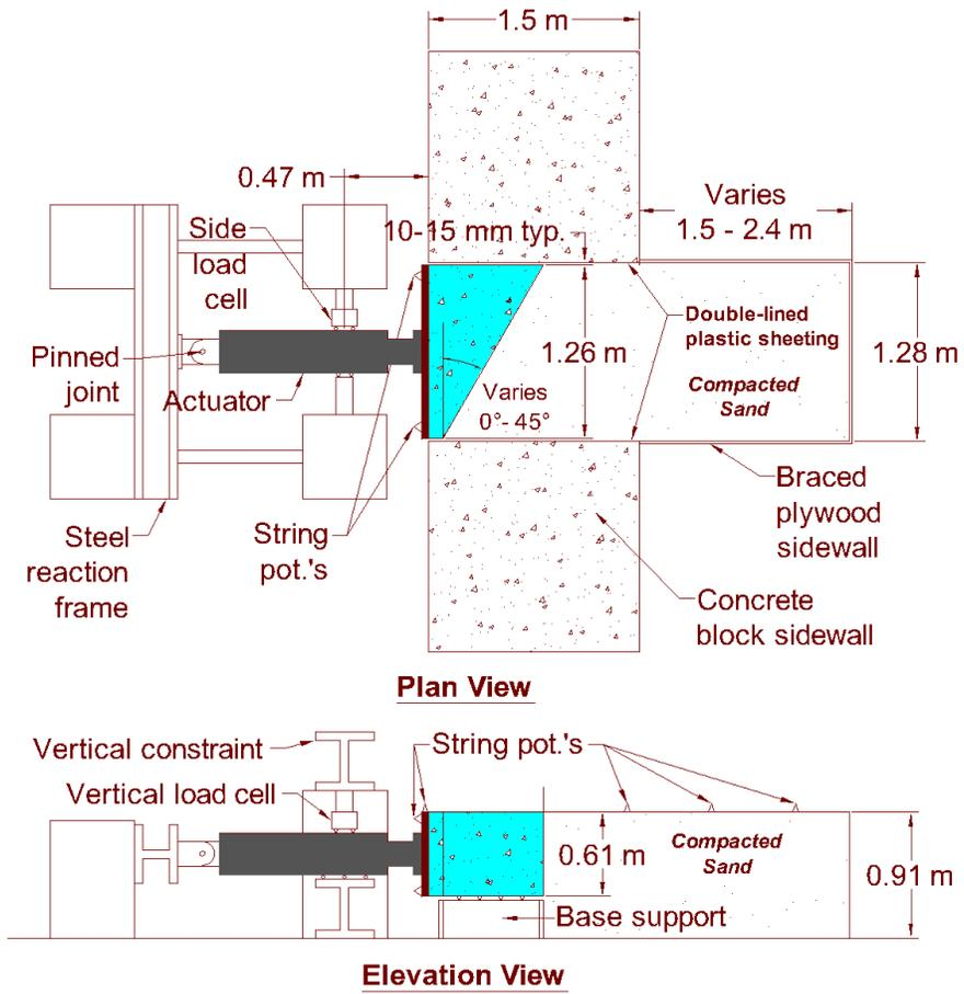
**Fig. 2: Schematic plan and elevation view drawings of the test layout for the skewed passive force deflection tests.**
