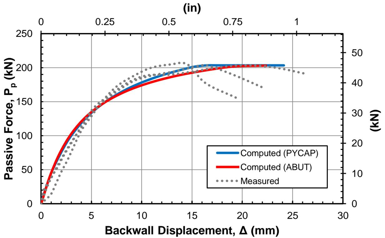
**Fig. 15: Comparison of measured and computed passive force versus longitudinal deflection curves for the no skew case.**
