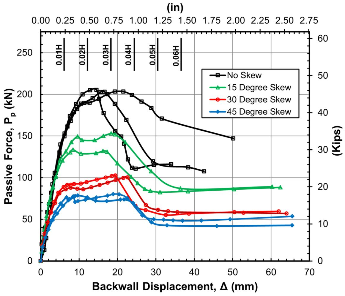
Fig. 6: Passive force versus longitudinal deflection curves for all the tests at various skew angles.
