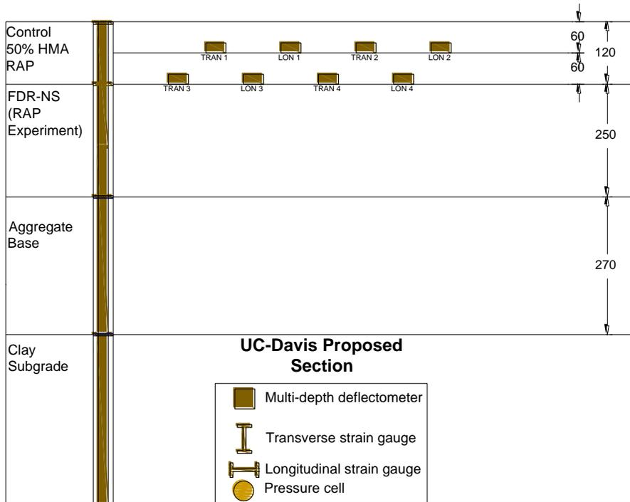
**Figure A-2. Plan and profile view of pavement structure and instrumentation for the 50%-RAP-HMA test section at UC-Davis**
