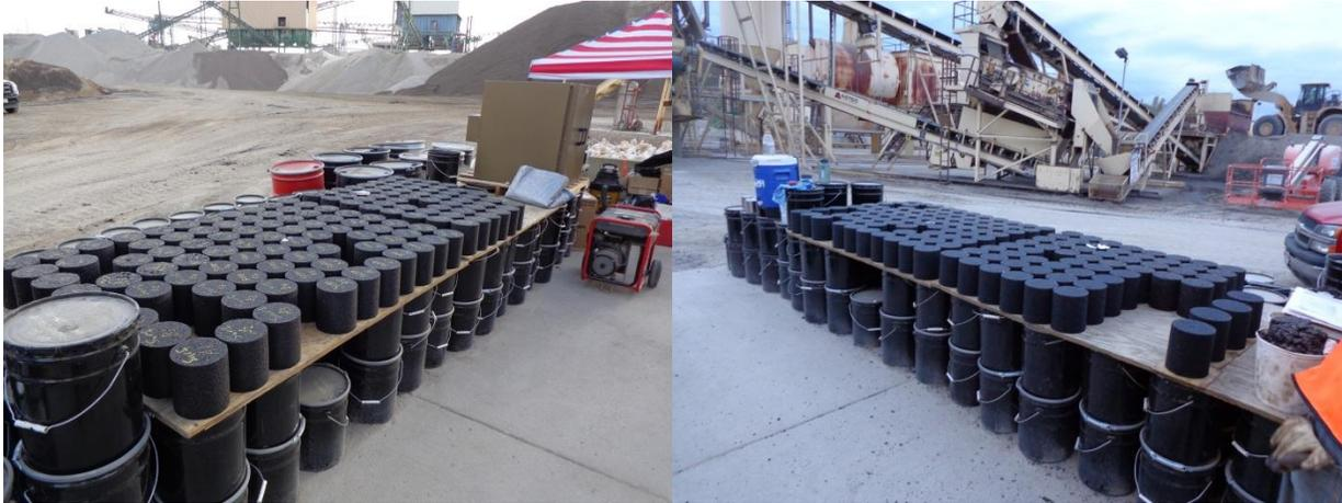
**Figure C-12. Compacted samples of Intermediate and Surface layer**
