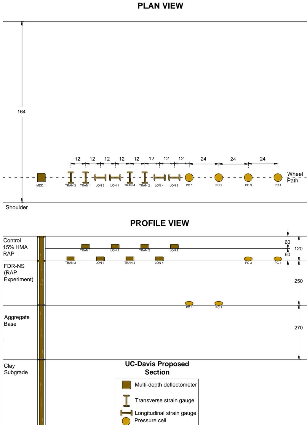
**Figure A-1. Plan and profile view of pavement structure and instrumentation for the 15%-RAP-HMA test section at UC-Davis**
