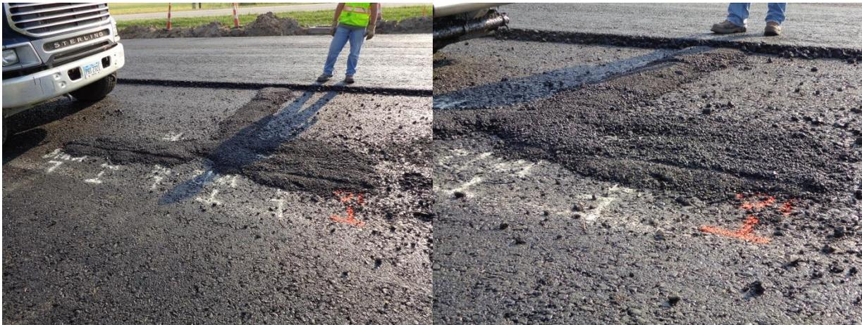
**FigureC-9. Possible misalignment of sensors after truck passes**
