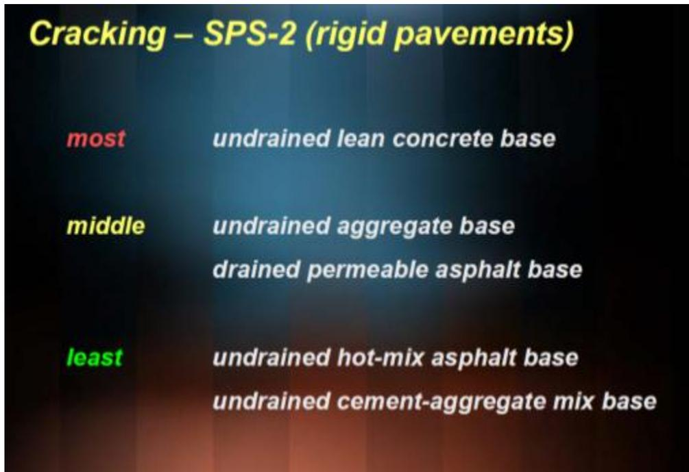
Figure 5-3 SPS-2 Crack Levels as a Function of Base Type (3)
