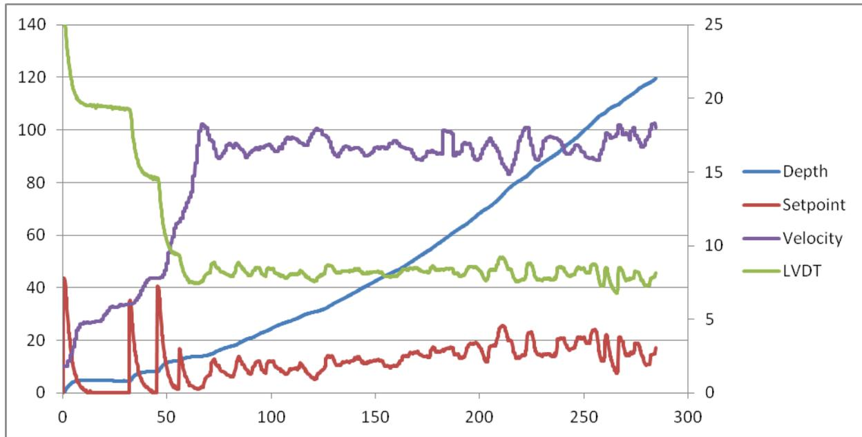
**Figure 9 Controlled motion of the ISTD showing the depth of the device, setpoint of the control system, LVDT reading, and velocity of the movement**
