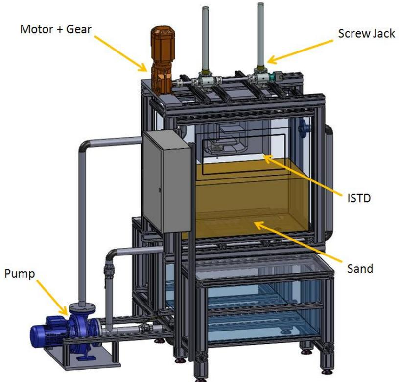
Figure 6: Solid Works drawing of the demonstration apparatus
