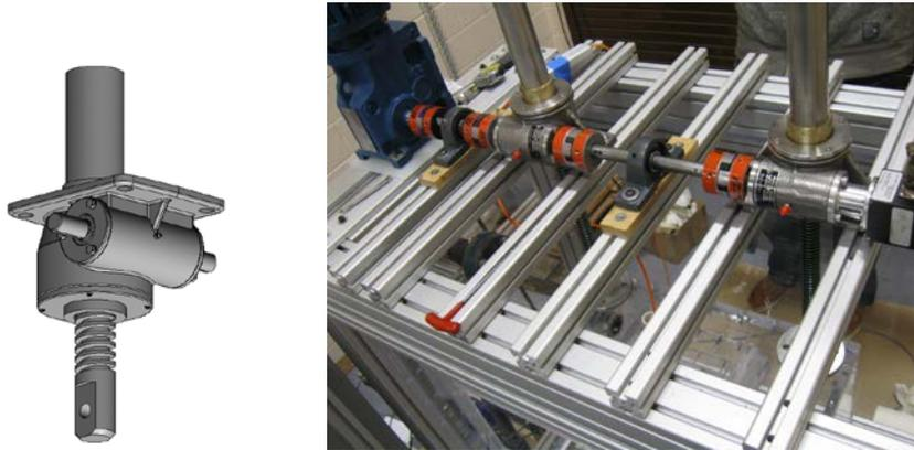
**Figure 3 Screw jack driving system**
