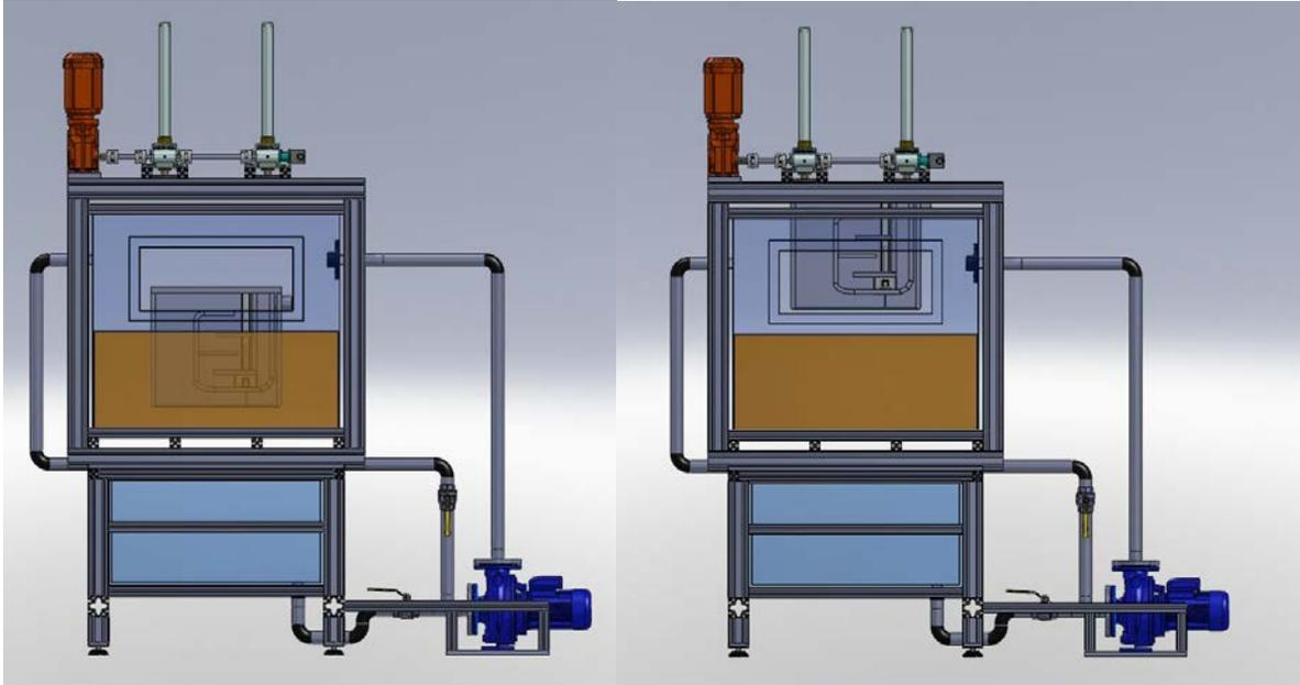
**Figure 7 The ISTD lowers into the sand bed**
