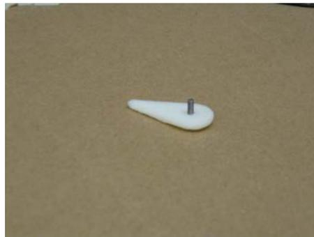
**Figure 4 Foot plate of the LVDT**
