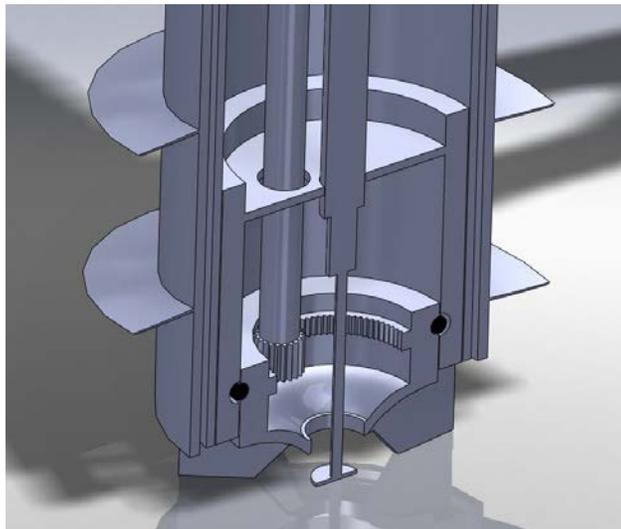
**Figure 11 Close-up view of the erosion head of the worm design**
