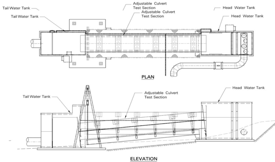
**Figure 1. Test Bed for Evaluation of Passage of Juvenile Salmon through Culverts Designed by Montgomery Watson Harza for the Pacific Northwest National Laboratory and the Washington State Department of Transportation.**
