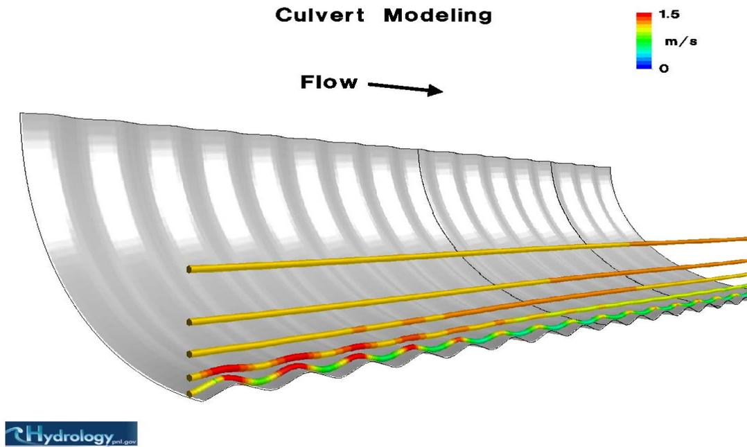
**Figure 2. An Example Visualization of Output from a Computational Fluid Dynamics Model for Water Flow in a Corrugated Steel Culvert.**
