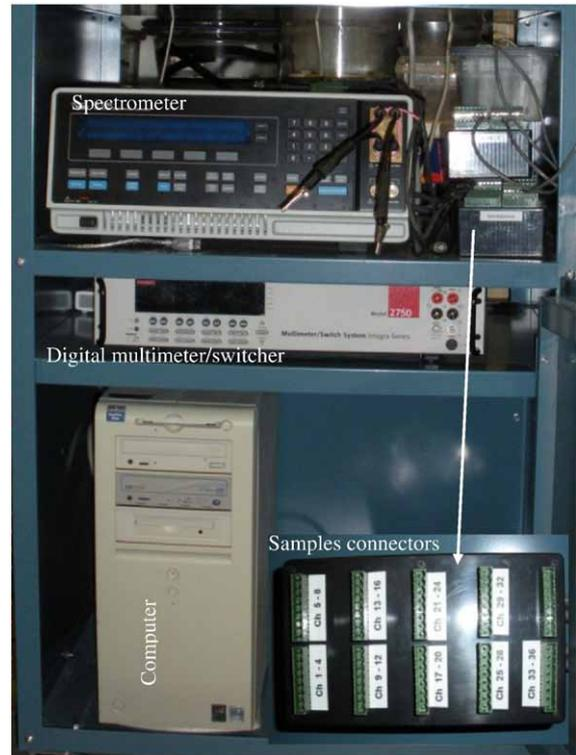
Fig. 2. Components of the system.
