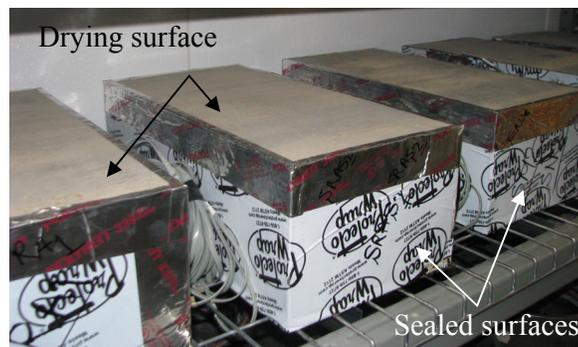
Figure 2: Slab geometry with one-sided drying
