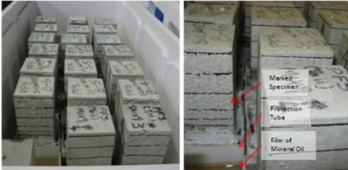
**Figure 14 USBR half immersed specimens in the container**
