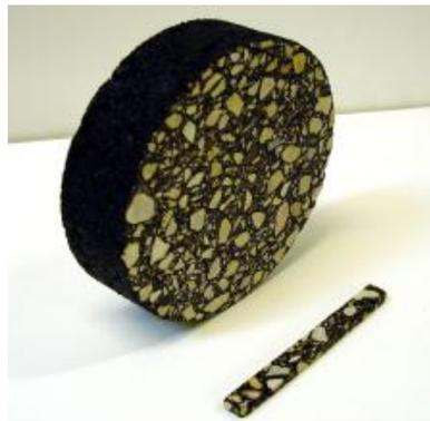
**Figure 32. IDT and BBR test specimens**
