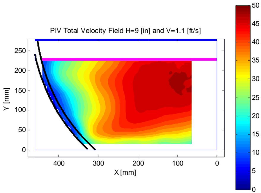
Fig. 25 PIV results for the 2<sup>nd</sup> CMP section with water height=9 [in] and average velocity= 1.1 [fts]
