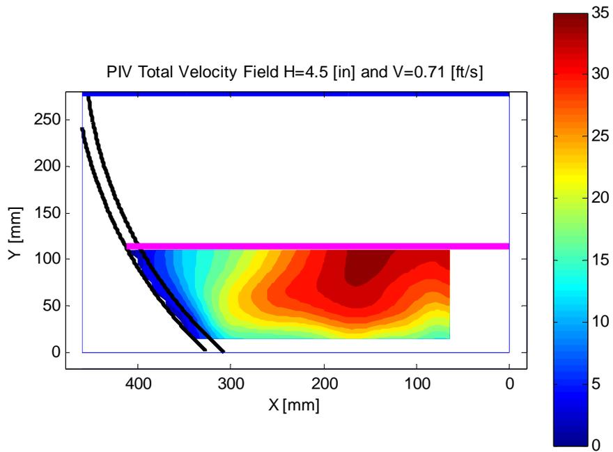
Fig. 15 PIV results for the 2<sup>nd</sup> CMP section with water height=4.5 [in] and average velocity= 1.1 [fts]
