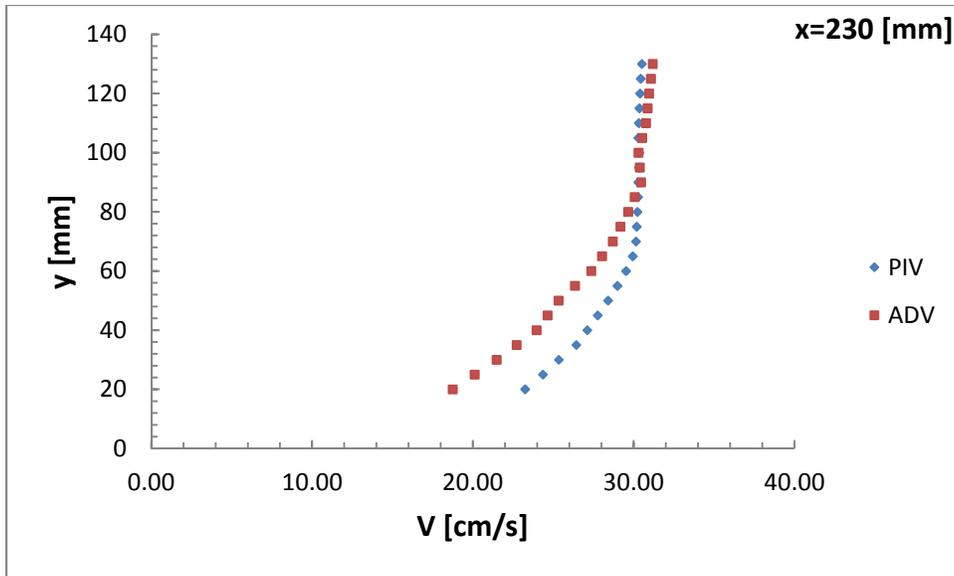
Fig. 9. PIV and ADV comparison for x=230 [mm] station with roughness
