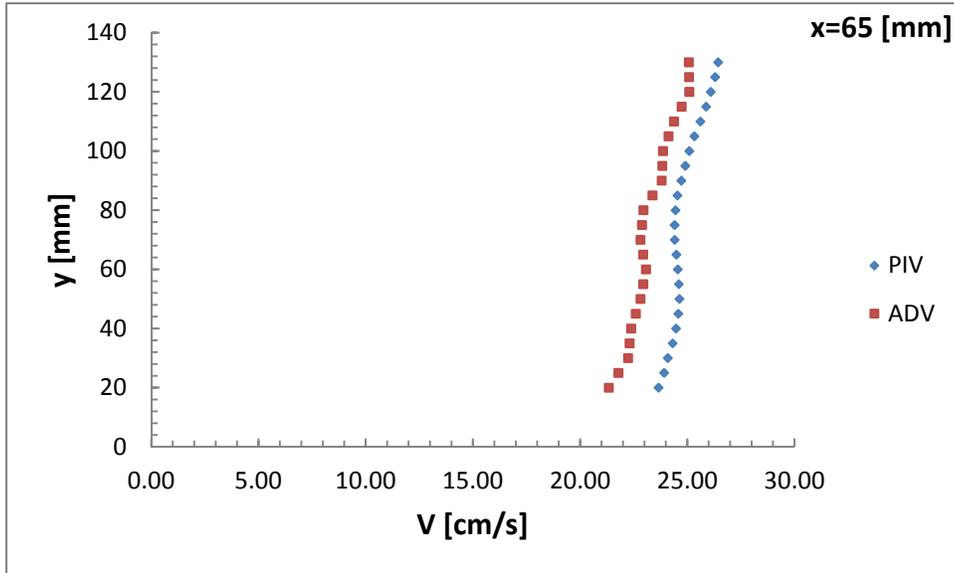
Fig. 5. PIV and ADV comparison for x=65 [mm] station without roughness
