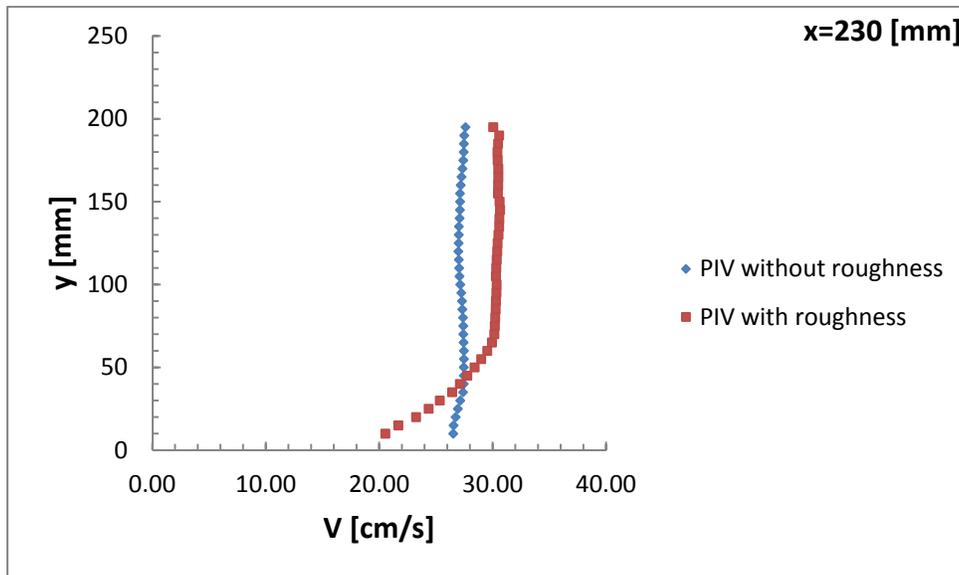
Fig. 12. PIV comparison for  $x=230$  [mm] station for bed both with and without roughness
