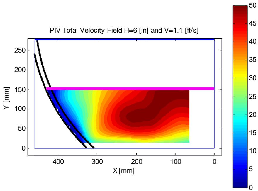
Fig. 21 PIV results for the 2<sup>nd</sup> CMP section with water height=6 [in] and average velocity= 1.1 [fts]
