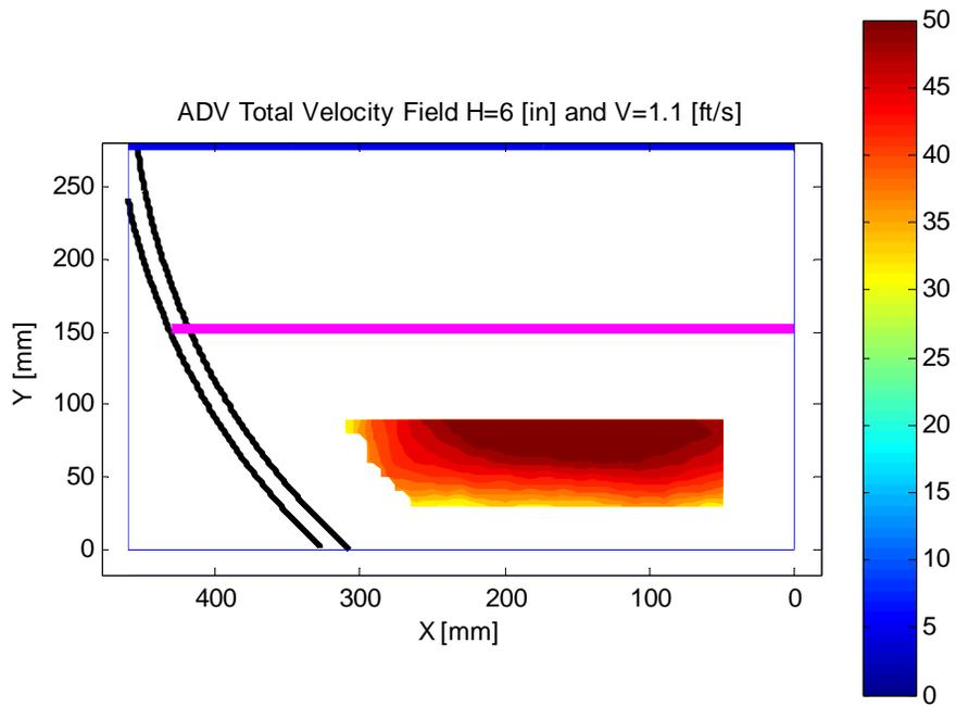
Fig. 20 ADV results for the 2<sup>nd</sup> CMP section with water height=6 [in] and average velocity= 1.1 [fts]
