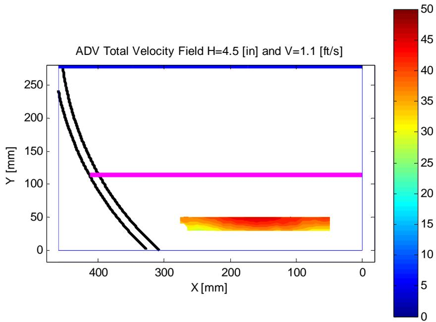
Fig. 16 ADV results for the 2<sup>nd</sup> CMP section with water height=4.5 [in] and average velocity= 1.1 [fts]
