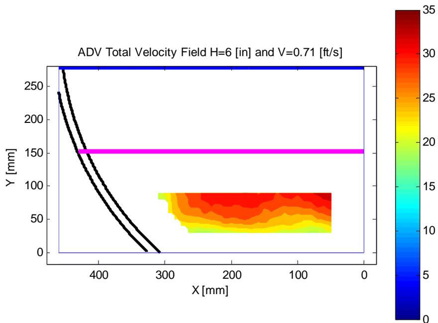
Fig. 18 ADV results for the 2<sup>nd</sup> CMP section with water height=6 [in] and average velocity= 0.71 [fts]
