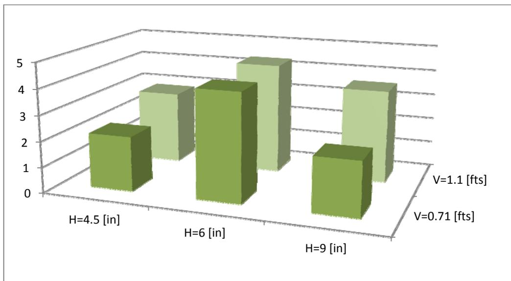
Fig. 26 RMSE between PIV and CFD for the 2<sup>nd</sup> CMP section
