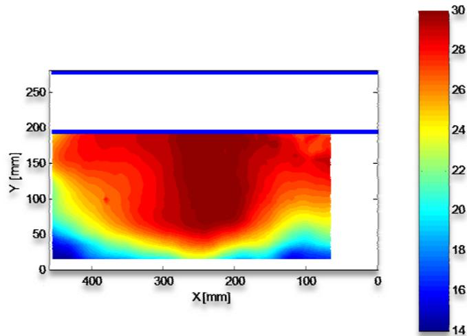
Fig. 4. PIV total velocity for a rectangular section with roughness
