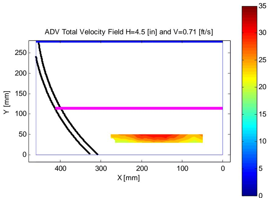
Fig. 14 ADV results for the 2<sup>nd</sup> CMP section with water height=4.5 [in] and average velocity= 0.71 [fts]
