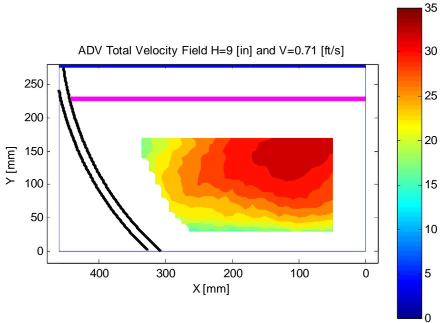
Fig. 22 ADV results for the 2<sup>nd</sup> CMP section with water height=9 [in] and average velocity= 0.71 [fts]
