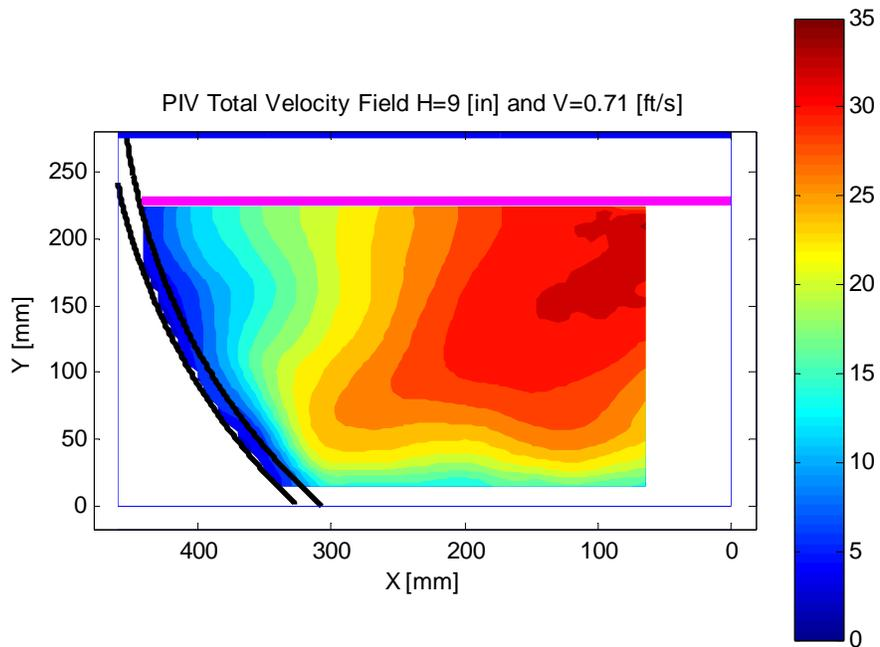
Fig. 23 PIV results for the 2<sup>nd</sup> CMP section with water height=9 [in] and average velocity= 1.1 [fts]
