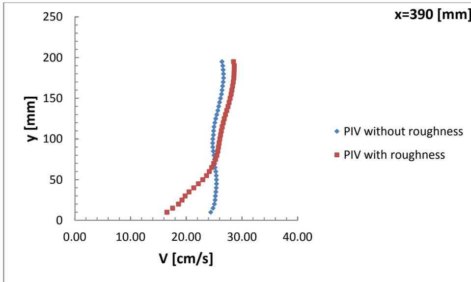
Fig. 13 .PIV comparison for x=390 [mm] station for bed both with and without roughness
