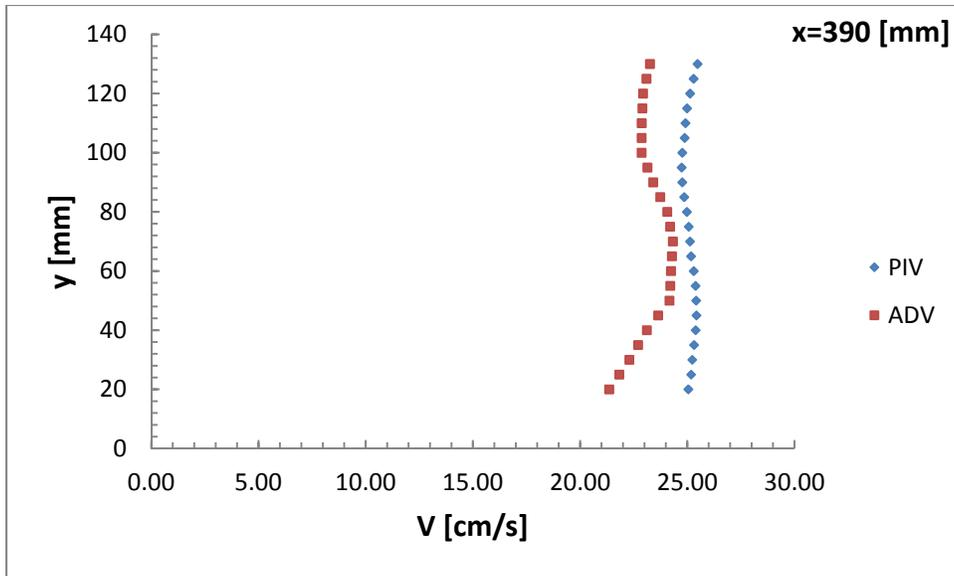
Fig. 7. PIV and ADV comparison for x=390 [mm] station without roughness
