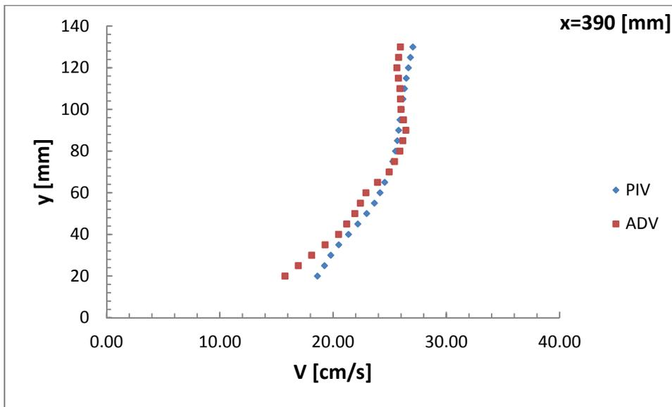
Fig. 10. PIV and ADV comparison for x=390 [mm] station with roughness
