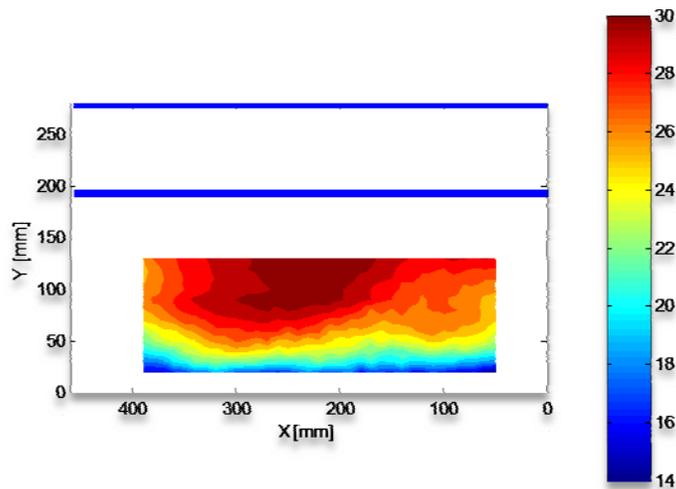
Fig. 3. ADV Total velocity for a rectangular section with roughness
