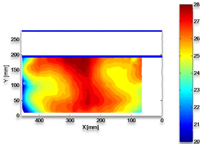
Fig. 2. PIV total velocity for a rectangular section without roughness
