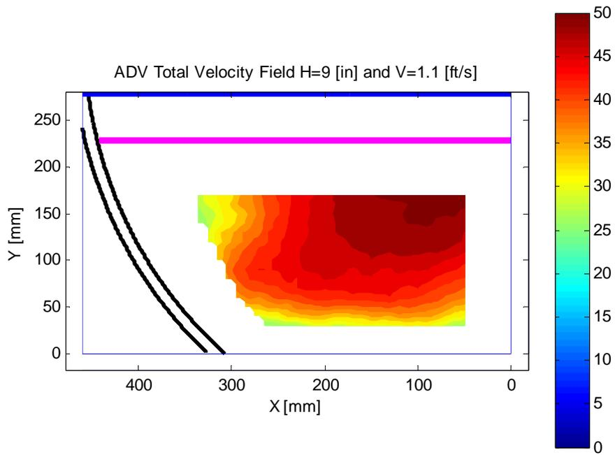
Fig. 24 ADV results for the 2<sup>nd</sup> CMP section with water height=9 [in] and average velocity= 1.1 [fts]
