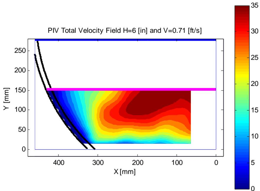
Fig. 19 PIV results for the 2<sup>nd</sup> CMP section with water height=6 [in] and average velocity= 1.1 [fts]
