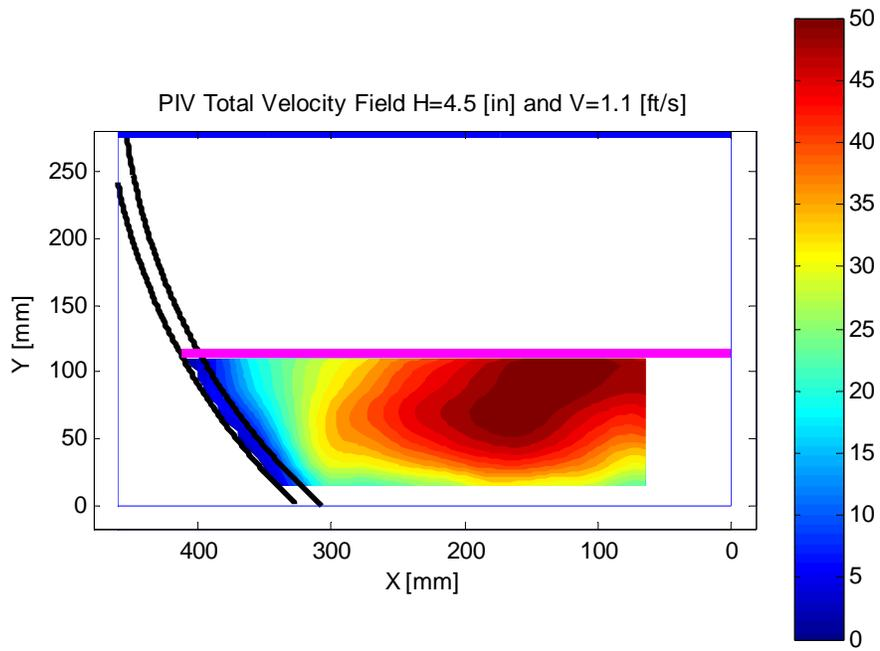
Fig. 17 PIV results for the 2<sup>nd</sup> CMP section with water height=4.5 [in] and average velocity= 1.1 [fts]
