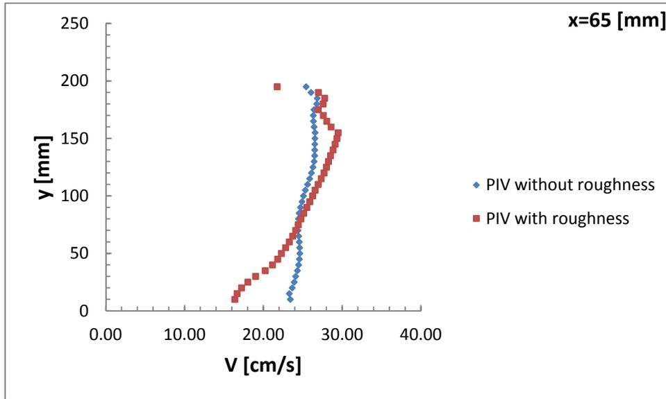
Fig. 11. PIV comparison for  $x=65$  [mm] station for bed both with and without roughness
