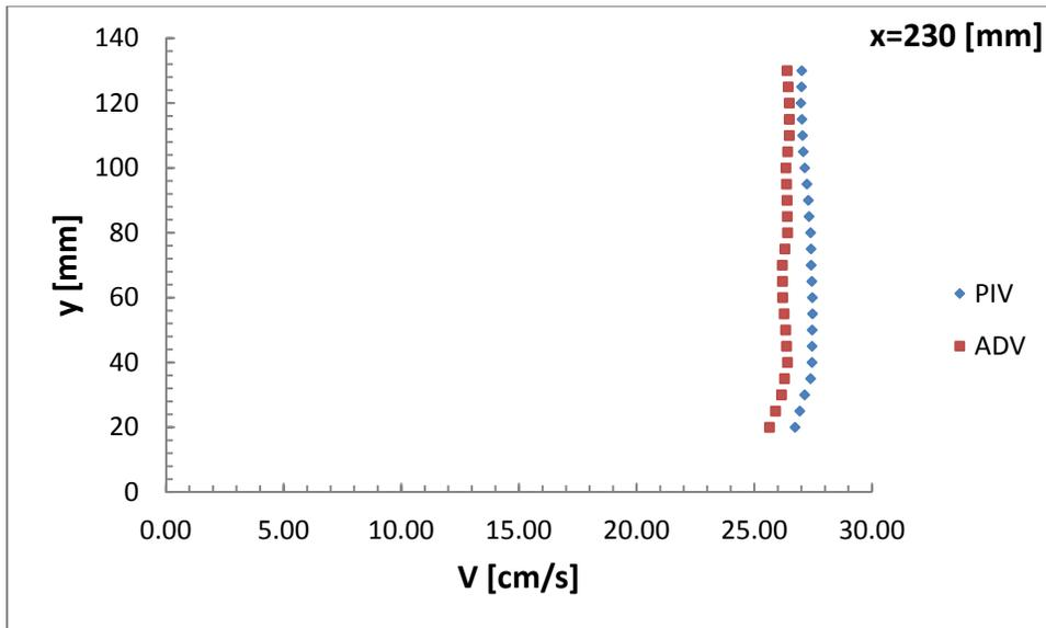
Fig. 6. PIV and ADV comparison for x=230 [mm] station without roughness
