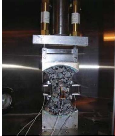
**Figure 4: Dog-bone direct tension test prototype (27)**
