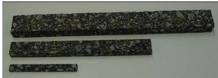
**Figure 2: 1x, 2x, and 3x asphalt mixture beam specimens. (17)**
