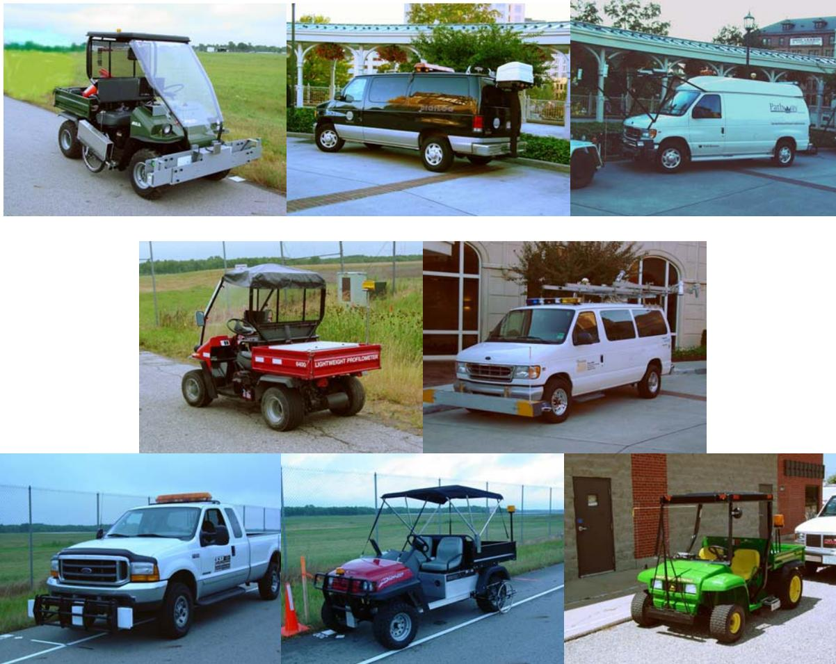
Profilers use state-of-the-art technology, accelerometers, lasers, distance measurement instruments, and they can provide International Roughness Index (IRI) values. But, they may not give the same measurements on the same roads. **Pooled Fund Study TPF-5 (063) "Improving the Quality of Profiler Measurement"** could change that.
