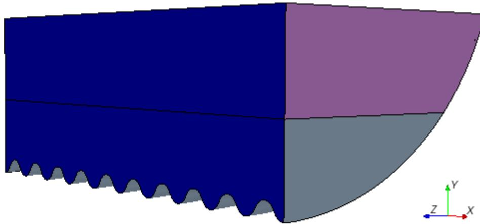
Figure 2.12 Increased section of the culvert (nearly three times bigger than the reduced section) used for porous media modeling
