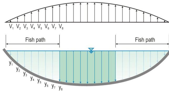
**Figure 2.3: Flow path for the selected fish design criteria of velocity and depth**
