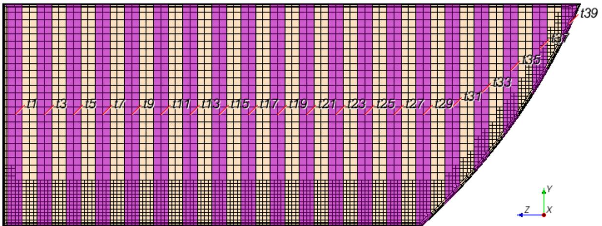
Figure 2.19 Representation of odd numbered Uniform strips of 1 cm width created along the fluid section
