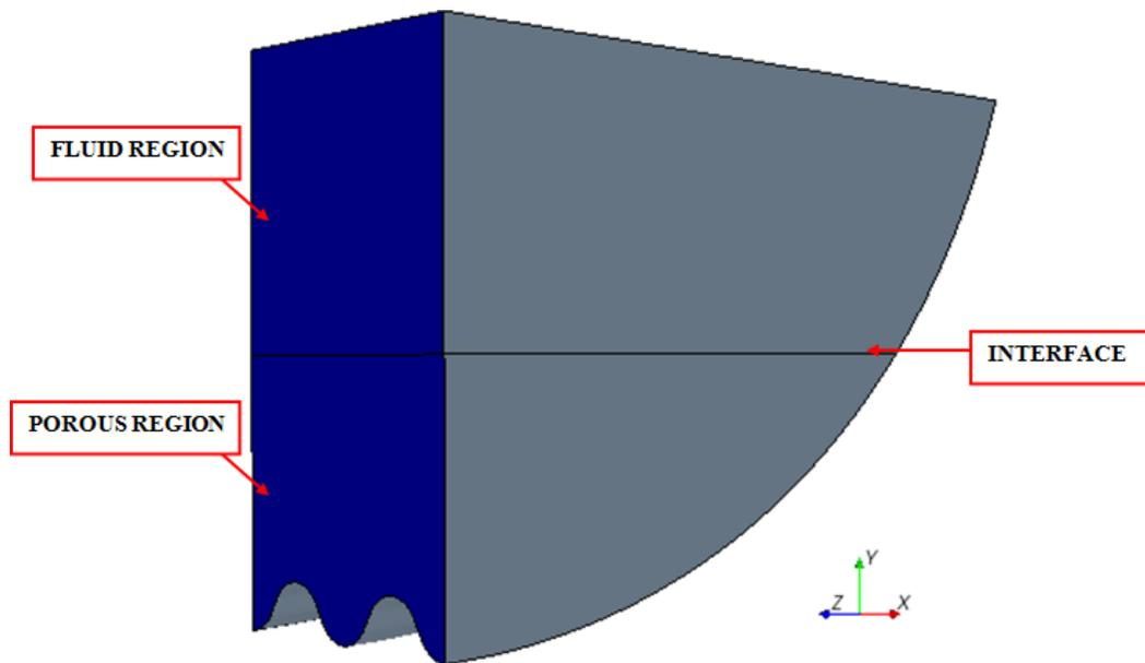
Figure 2.9 CAD model representing the computational domain used for porous media modeling
