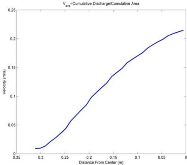
Figure 2.8: average velocity curve in a cross-section of 6 inch water depth with symmetry boundary
