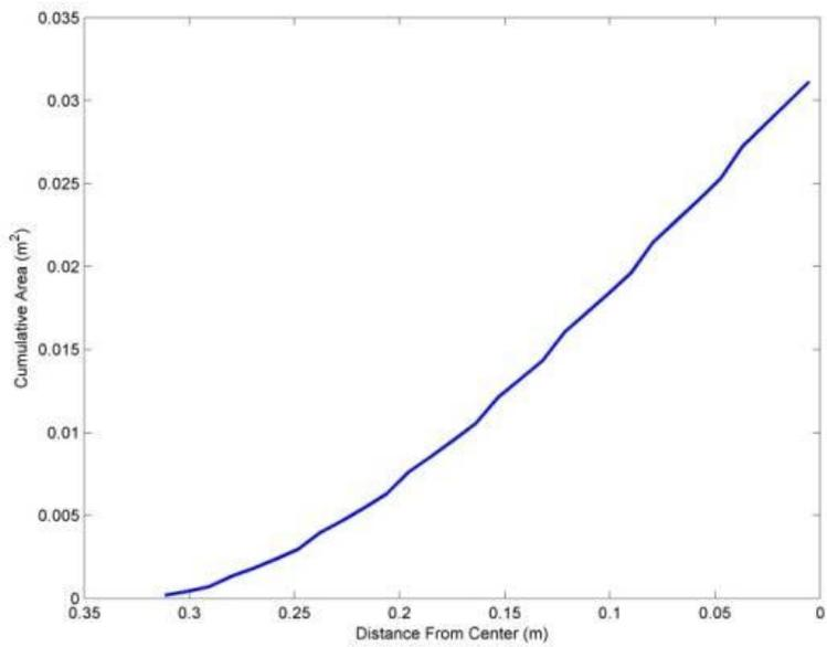
Figure 2.7: Cumulative area from the wall to the centerline in a cross-section of 6 inch water depth with symmetry boundary
