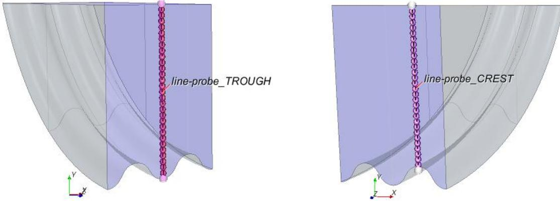
Figure 2.14 Image depicting the line probes created at a trough and a crest for a reduced section
