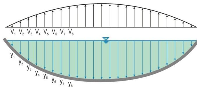
Figure 2.1: Variation of flow velocity and depth in a cross-section of a corrugated metal pipe
