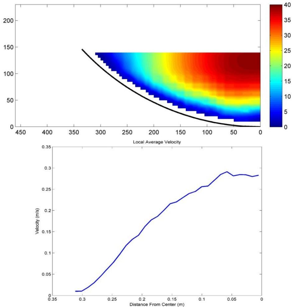
Figure 2.2: Depth-averaged velocity curve development in a cross-section of 6 inch water depth with symmetry boundary
