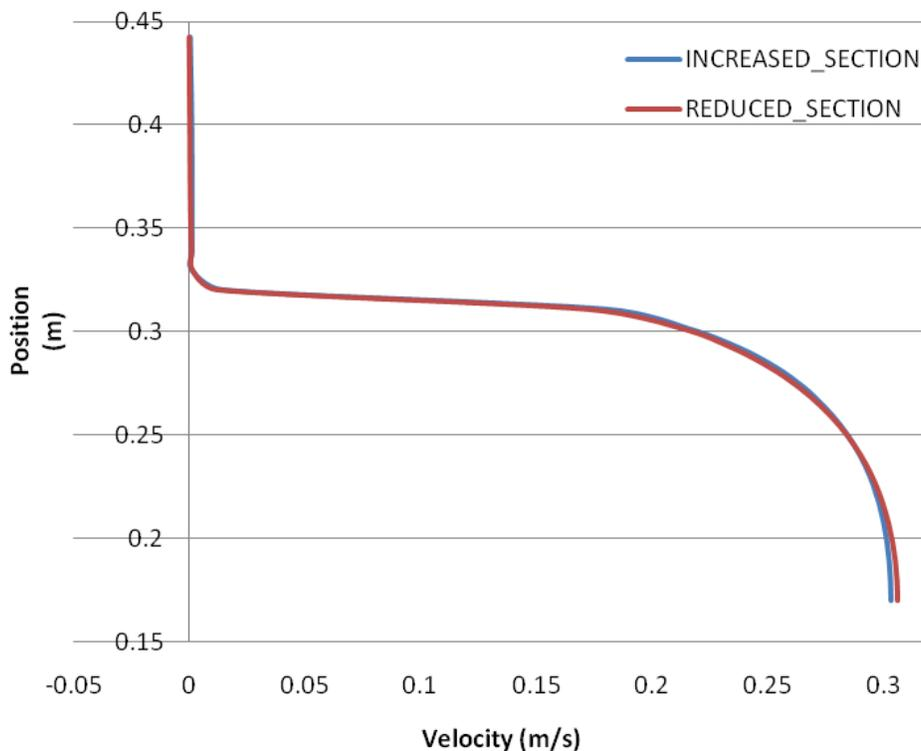
Figure 2.16 Velocity profiles for both reduced and increased sections at a crest
