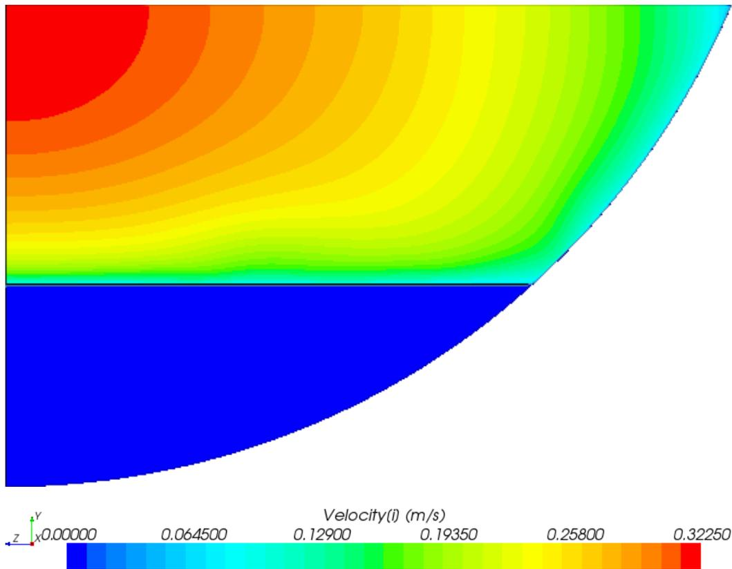
Figure 2.21: Velocity distribution over cross section at a crest showing the variation above the porous media gravel bed
