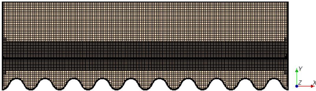
Figure 2.13 Cross sectional view of mesh scene along on a plane taken along the length of the increased section
