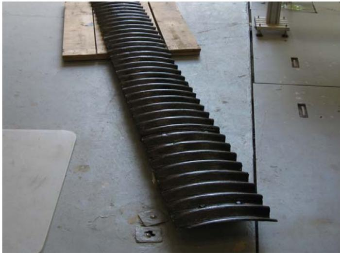
Figure 10. 2nd CMP pipe after applying tar
