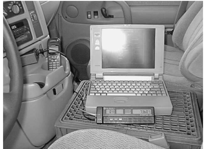
FIGURE 5 DMI instrumentation in test vehicle.
