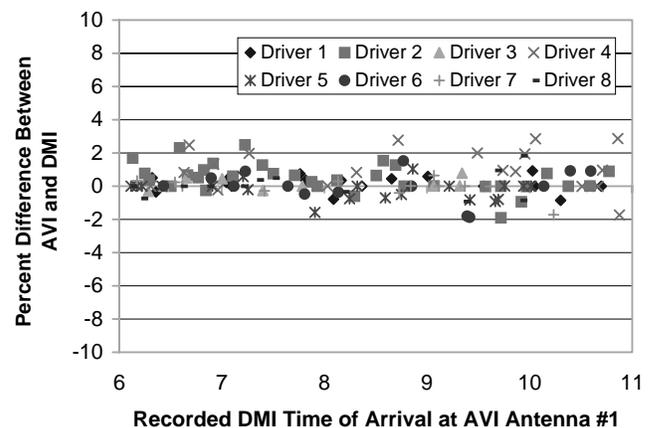
FIGURE 7 Percent difference between AVI and test vehicle (DMI) travel-time estimates by driver for entire corridor.
