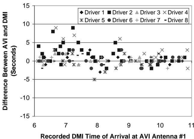
FIGURE 6 Difference between AVI and test vehicle (DMI) travel-time estimates by driver for entire corridor.
