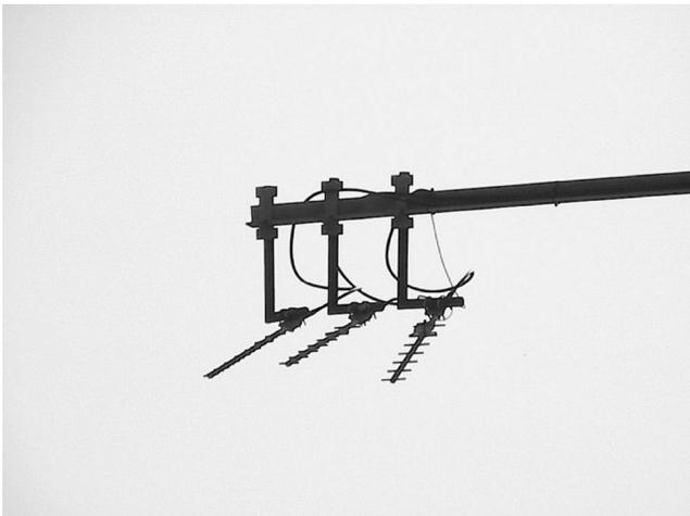
FIGURE 4 AVI antenna configuration.
