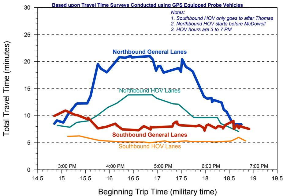
Fig. 2.3: Example of a Travel Time Profile for the Study Corridor
