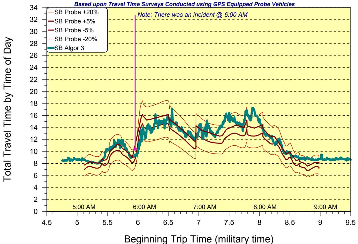
**Fig. 2.13: Comparison of the Results of the Predictive Travel Time Algorithm with Comparable Observed Travel Times for the Southbound General-Purpose Lanes Results**
