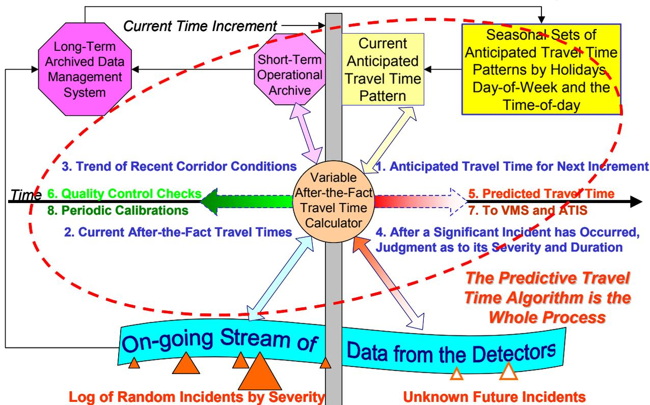
Fig. 2.12: Basic Components of the Predictive Travel Time Algorithm
