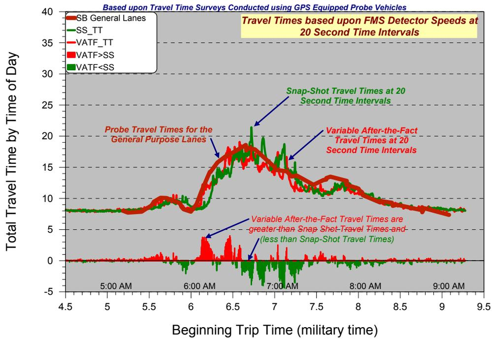
**Fig. 2.8: Example of Comparison of Snap Shot Travel Time to After the Fact Travel Time**
