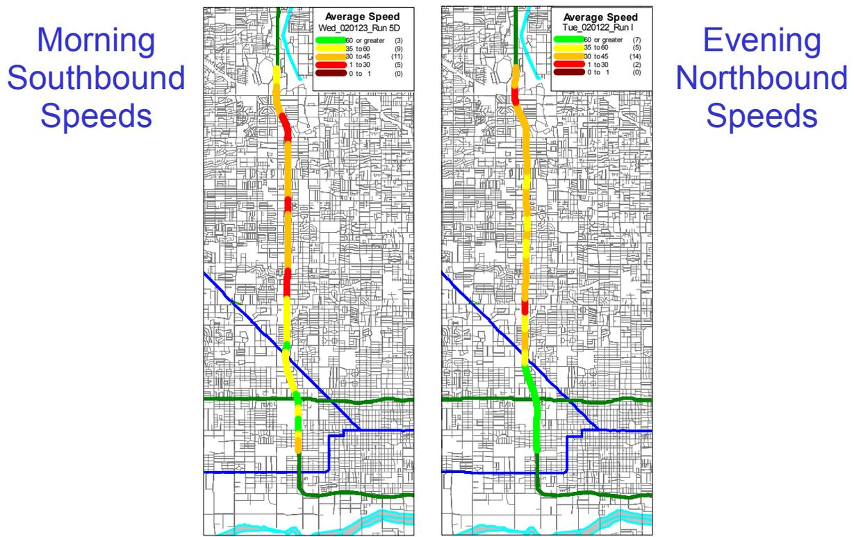
Fig. 2.2: Avg. Speed Between Detectors based on GPS Data
