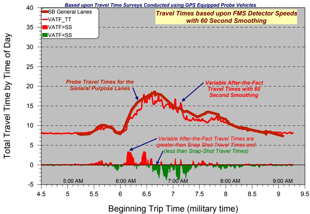
**Fig. 2.9: Snap Shot Travel Time Versus After the Fact Travel Time with Smoothing**
