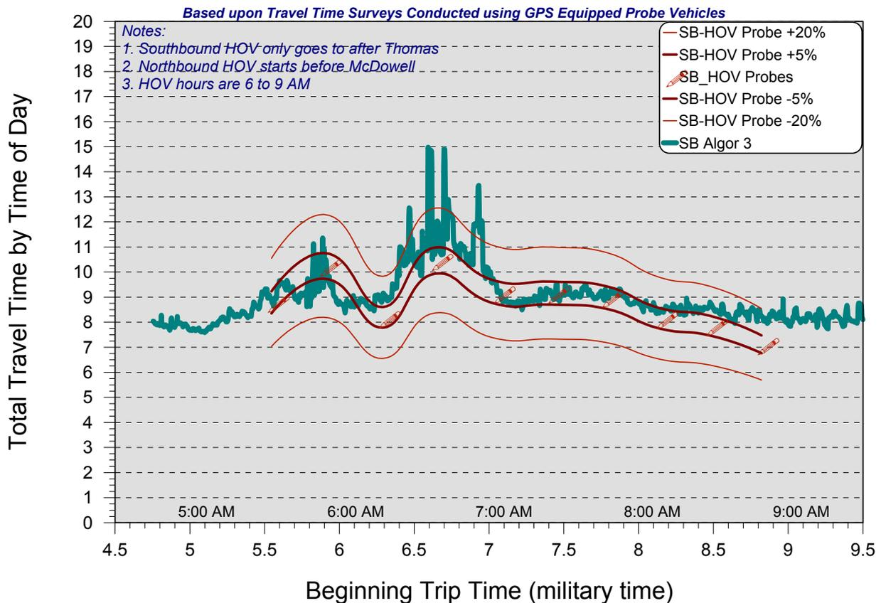
**Fig. 2.14: Comparison of the Results of the Predictive Travel Time Algorithm with Comparable Observed Travel Times for Southbound HOV Lanes**
