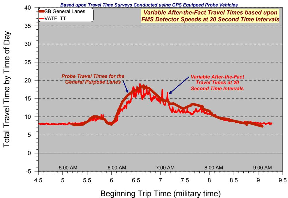
Fig. 2.7: Example of After-the-Fact Travel Time Compared to Observed Probe Travel Time
