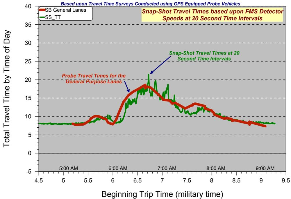
Fig. 2.6: Example of Snap Shot Travel Compared to Observed Probe Travel Time
