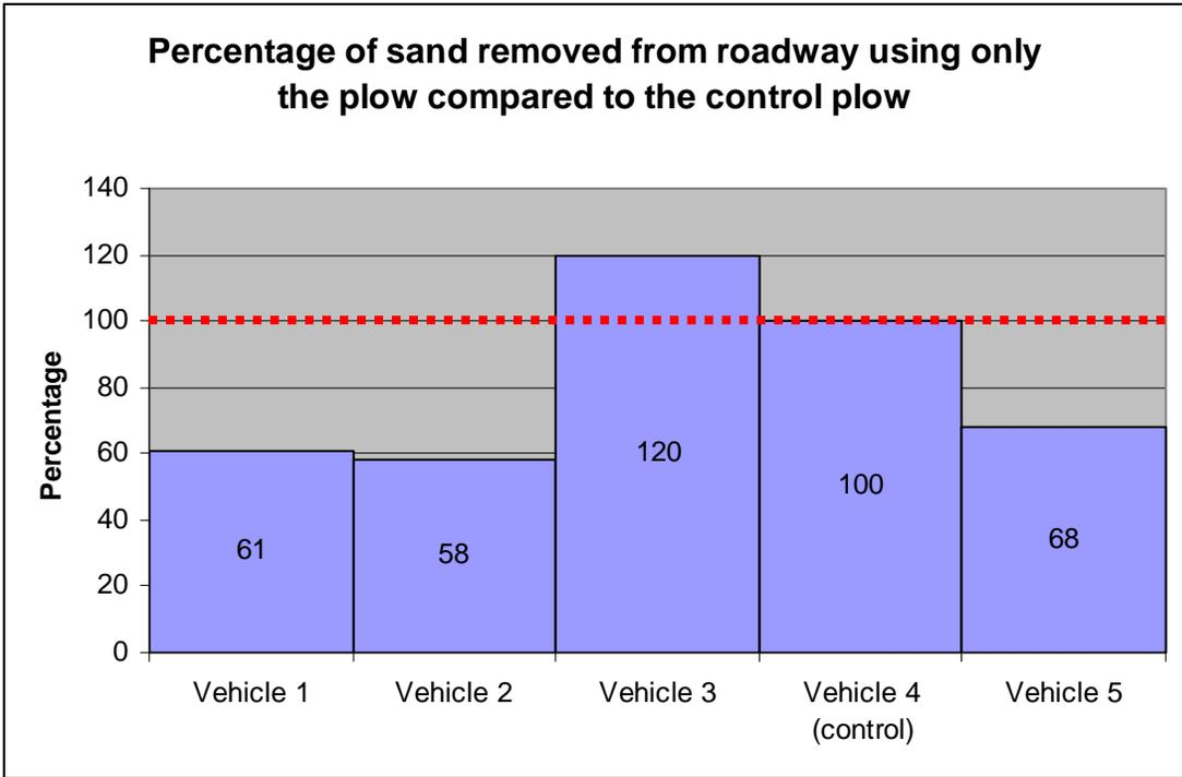
Figure 23. Plow only on even surface
