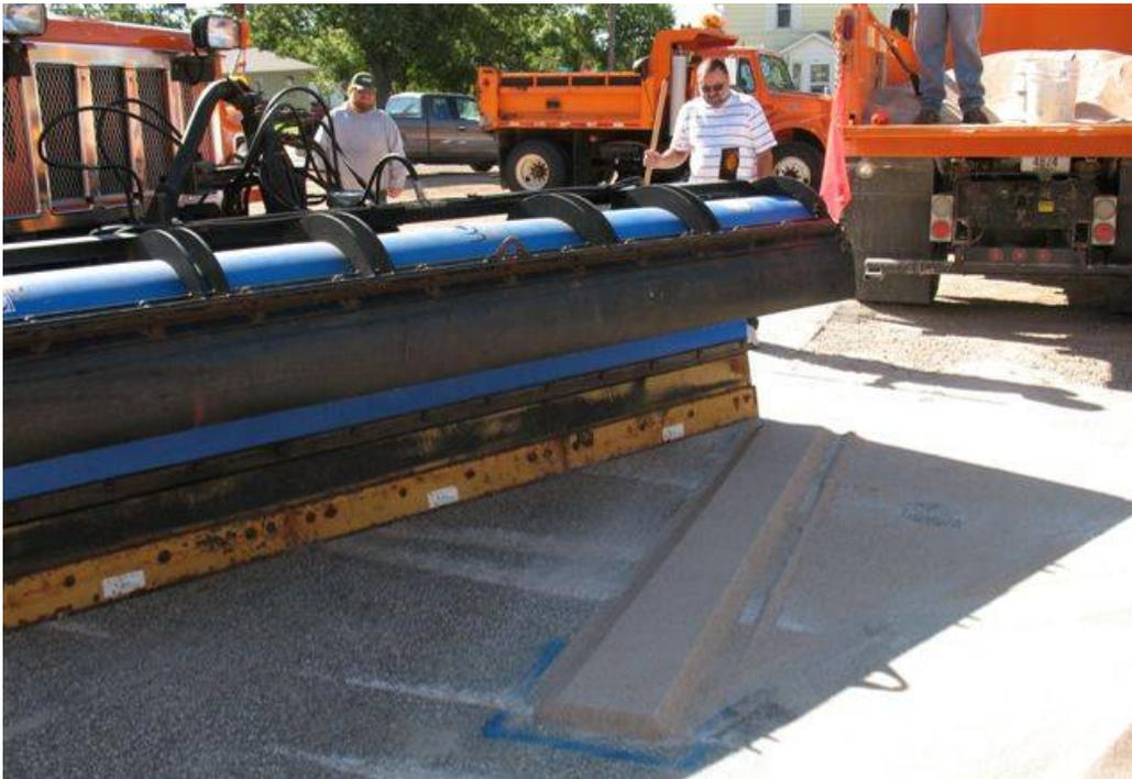
**Figure 6** Wausau down pressure plow
