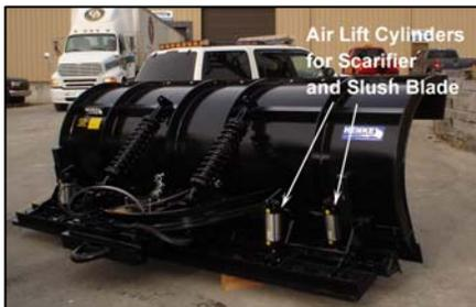
The scarifying and squeegee blades could be operated with hydraulic or air cylinders. For the Ohio DOT prototype, two air circuits were used to operate the additional blades—one to control the squeegee blade, and one to control the scarifying blade. No additional capacity was required
