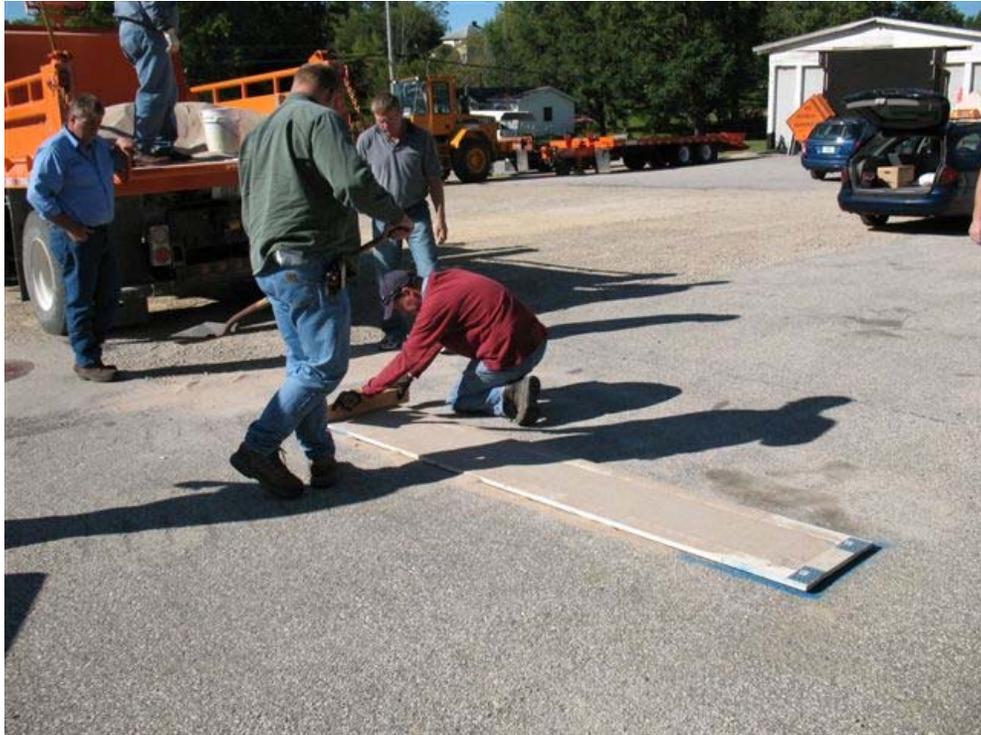
**Figure 13 Striking-off the top of the frame to make sure the same amount of sand was in the test area for each run**
