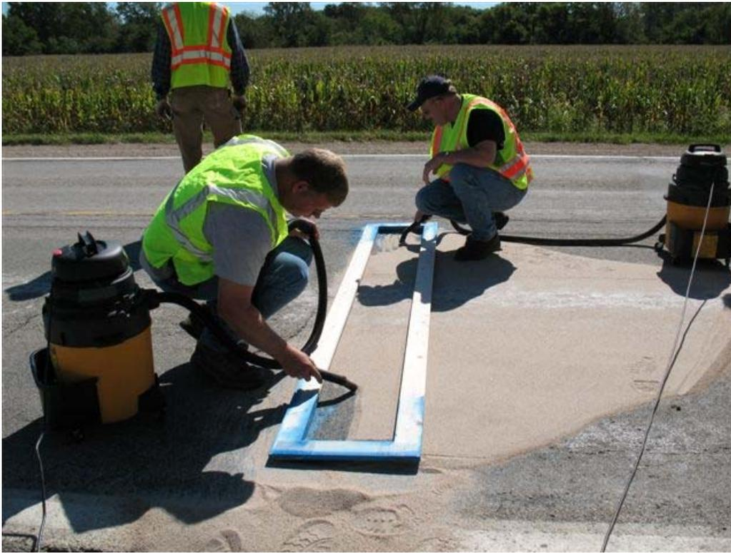
Figure 22 Collecting sand after plow passes through test area
