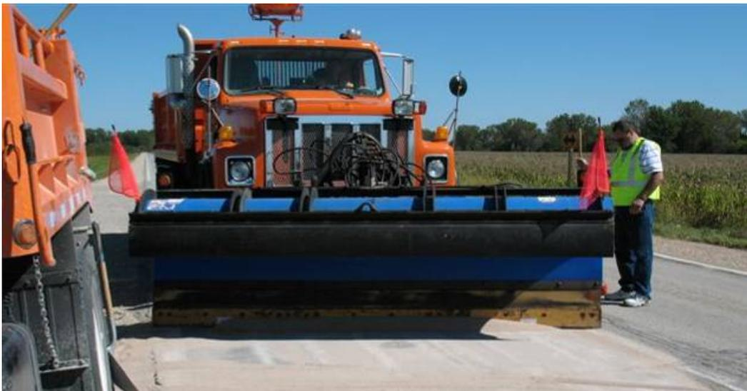
**Figure 7** Wausau down pressure plow on road test area
