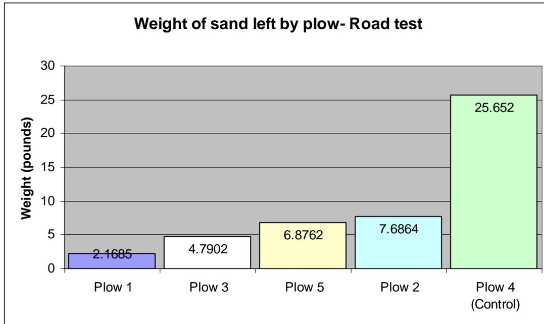
Figure 27. Weight of sand left behind each plow during road test
