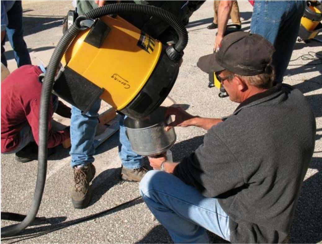
**Figure 19 Capturing sand for weighing**
