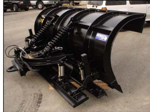
*The Henke Manufacturing prototype featured a custom-built flexible cutting edge, an Olofsfors scarifying blade and a squeegee blade.*
