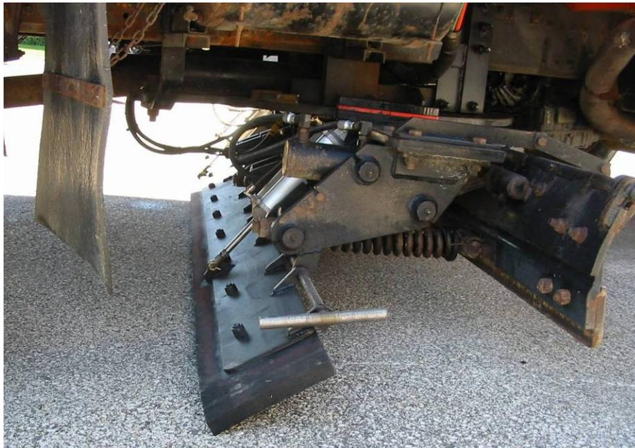
**Figure 10 Squeegee blade in contact with road surface to remove slush and liquids**
