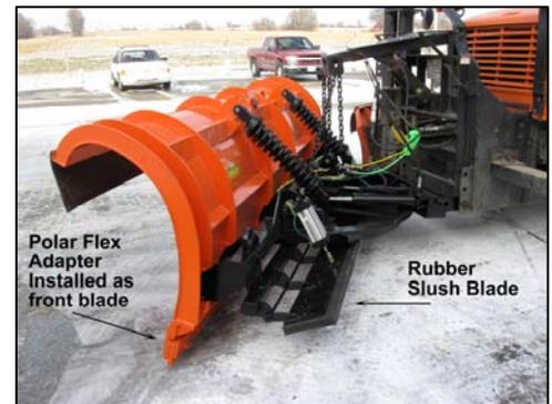
Air lines were run to the front of the truck to control the squeegee, and Iowa DOT installed electronic switches and relay valves. Consideration was given to how high to mount the plow and placement of the holes to attach it.
