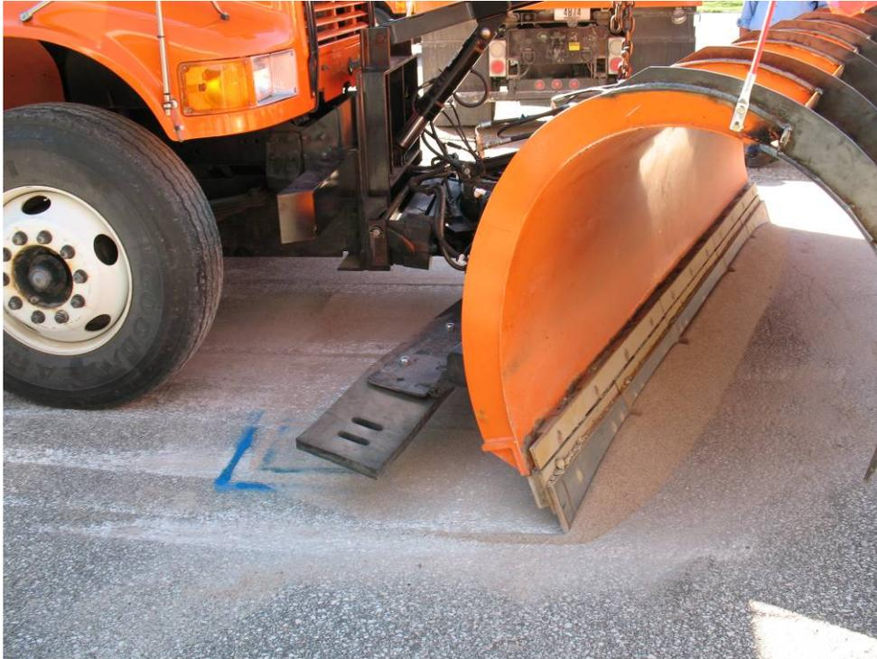
**Figure 15 Test plow runs through sand with squeegee blade activated**
