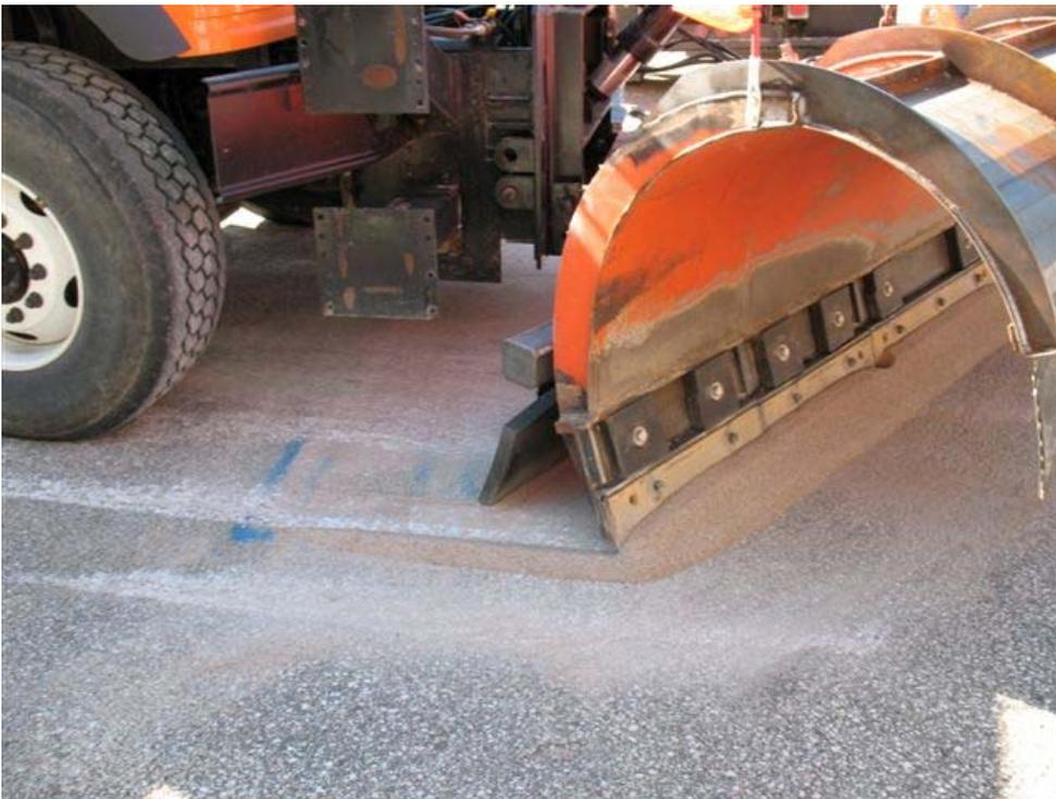
**Figure 16 Plow and squeegee blade clear sand from test area on second pass**
