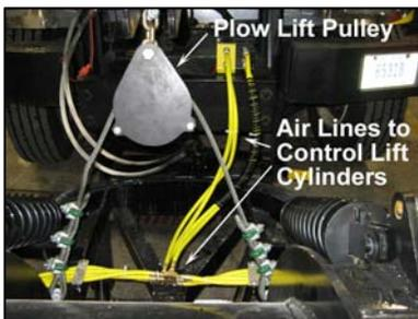
The scarifying and squeegee blades could be operated with hydraulic or air cylinders. For the Indiana DOT prototype, two air circuits were used to operate the additional blades—one to control the squeegee blade, and one to control the scarifying blade. No additional capacity was required for the truck's air system
