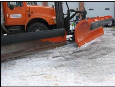
Air rather than hydraulics were used to operate Flink's multiple blades. With air, the operator could adjust the pressure setting, modifying the down pressure coming from the cylinder holding the blade on the pavement surface. This adjustment is harder to make with hydraulics. Flink representatives commented that a retrofit was made easier by tapping into air lines already present on the truck, which has air compressors for air brakes and air suspension.
