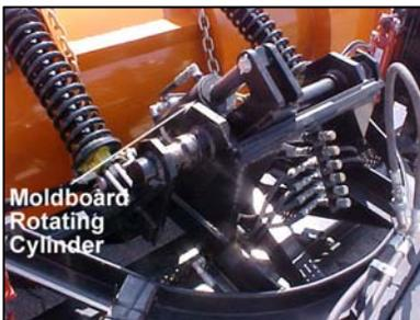
The ABAS flexible-edge system uses two- and three-foot blade sections. Unique among the project’s prototypes, the Monroe multiple-blade plow included a rotating moldboard that allowed for differences in the attack angle of the cutting blade, which was helpful in peeling up hardpack. Adjustments were available up to 25 to 30 degrees that move the cutting blade left and right and forward and back. The operator hydraulically activated the cutting edge attack angle by tilting the moldboard.
