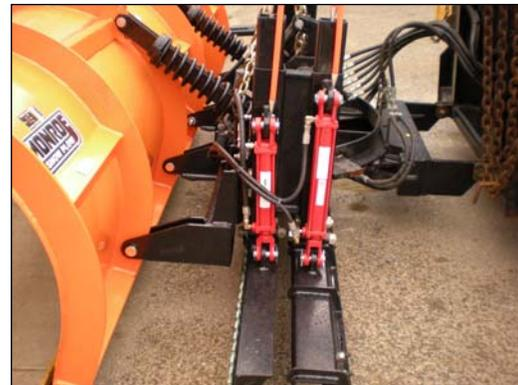
*Three blades are used on Monroe Truck Equipment's prototype: the ABAS flexible blade system, an Olofsfors scarifying blade and a squeegee blade.*
