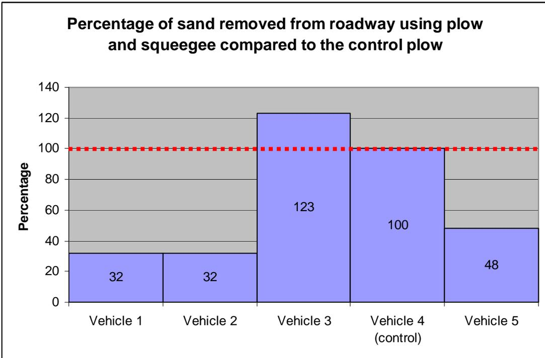
Figure 24 Plow and squeegee on an even surface
