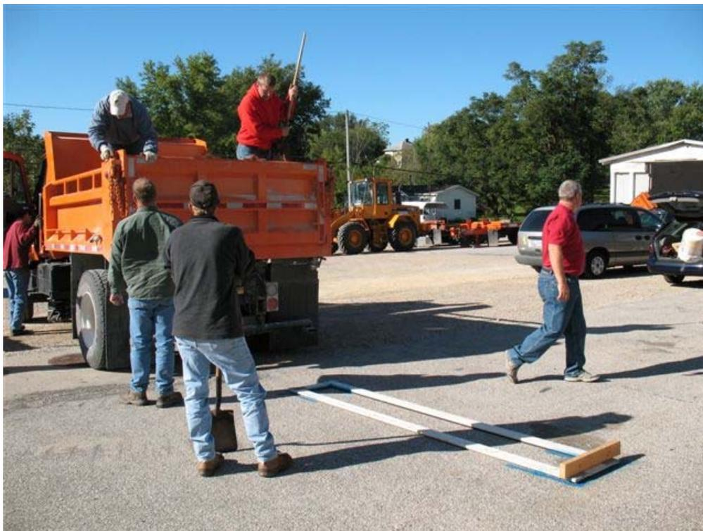
**Figure 12** Filling frame with sandblast sand
