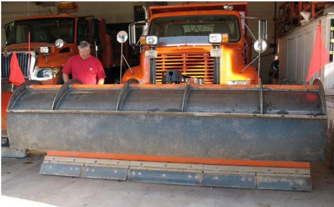
**Figure 5 Active Adaptor System with rebar under blades to show ability to adjust to roadway contours**
