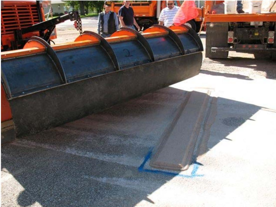
**Figure 3 Plow with Active Adapter system**
