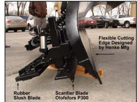
The prototype plow was mounted to a 2007 International multipurpose dump truck. Approximate total weight of the prototype plow is 2,750 lbs.
