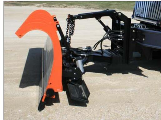
*The prototype developed by Henderson Products Inc. included two blades: a PolarFlex cutting blade and rubber squeegee blade.*
