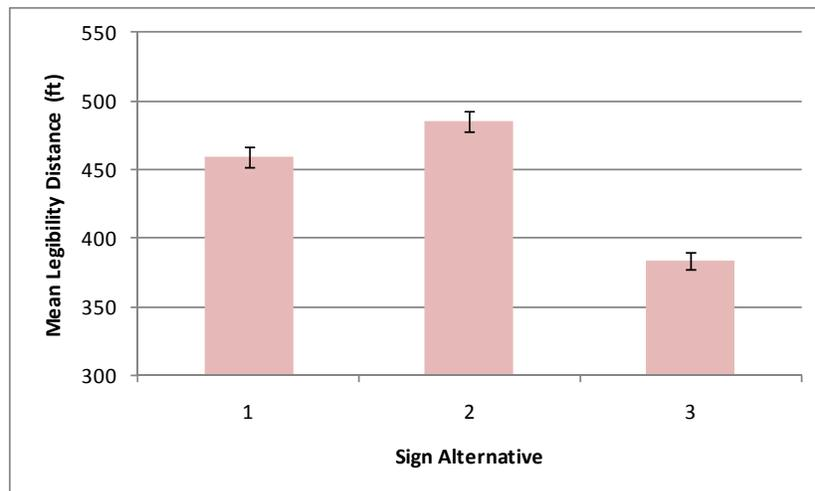
**Figure 7: Mean Distances for Flagger Ahead Signs**
