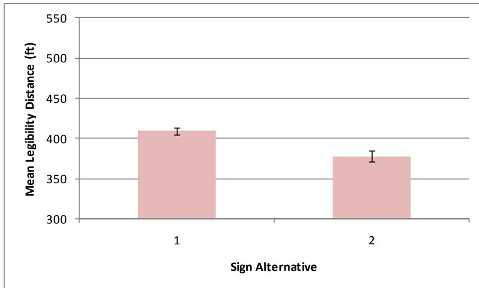
**Figure 12: Mean Distances for Uneven Lanes Signs**
