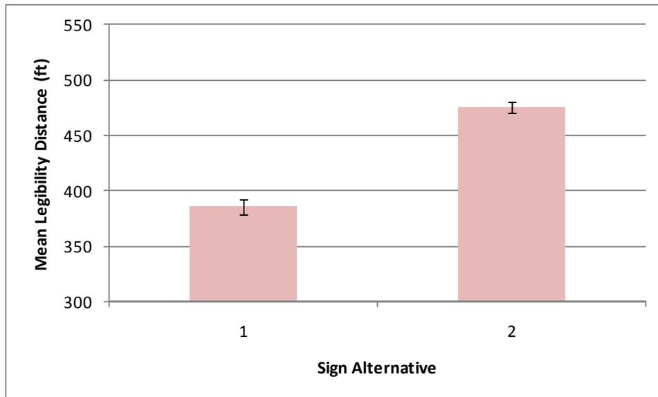
**Figure 4: Mean Distances for Do Not Pass Signs**
