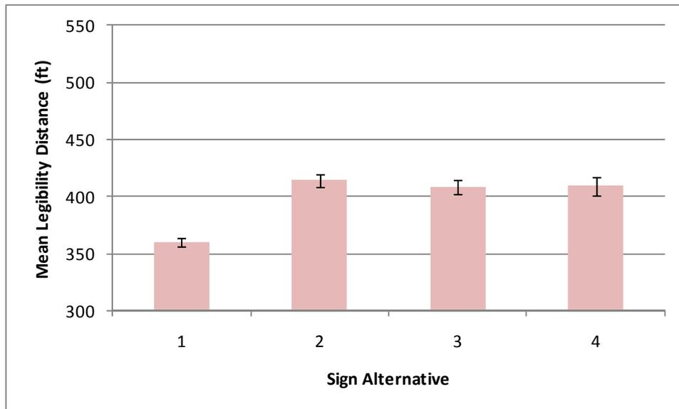
**Figure 10: Mean Distances for Low Shoulder Warning Signs**
