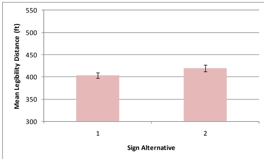
**Figure 8: Mean Distances for Maximum Width Signs**
