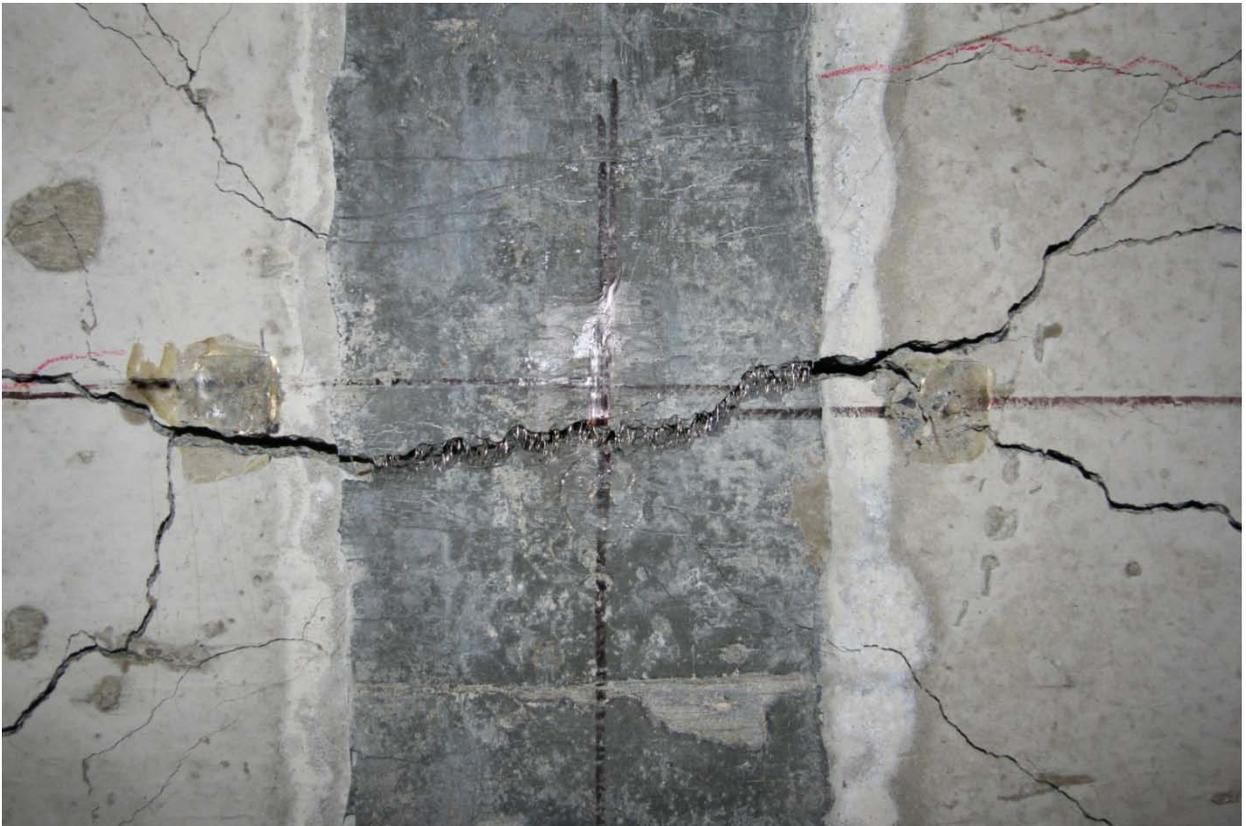
**Figure 30. Photograph. Underside of panel 8H at midspan centerline location after flexural failure.**
