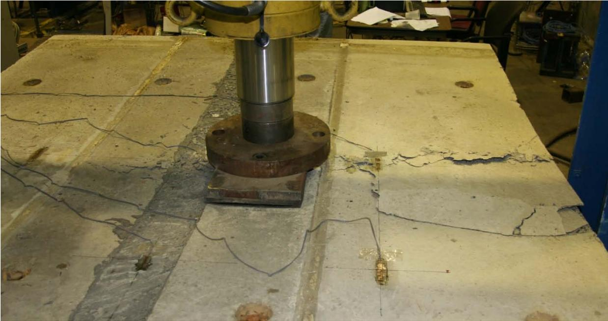
**Figure 55. Photograph. Top of panel 8B after flexural failure.**
