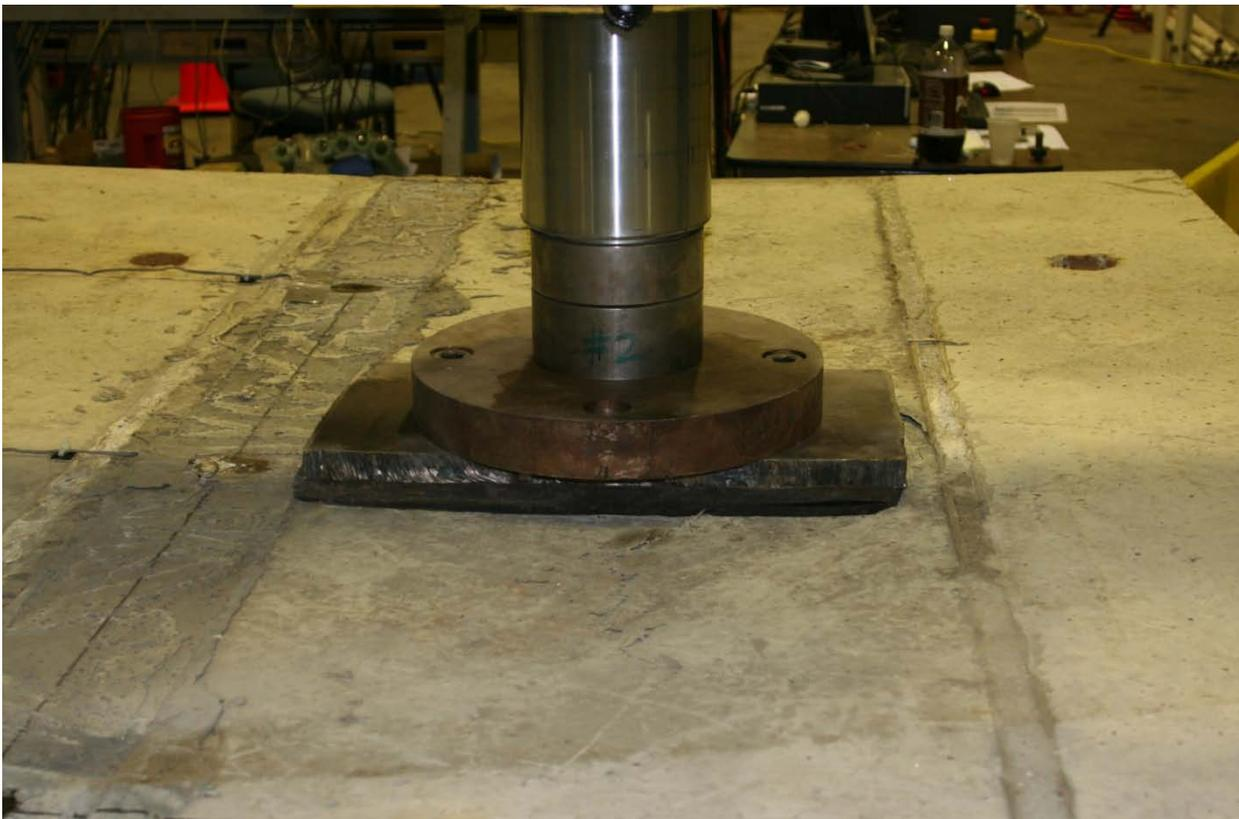
**Figure 71. Photograph. Top of panel 6H after flexural failure.**
