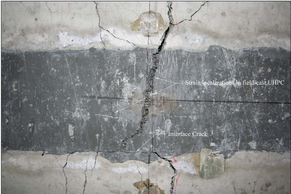
**Figure 56. Photograph. Underside of panel 8B at midspan centerline location after flexural failure.**
