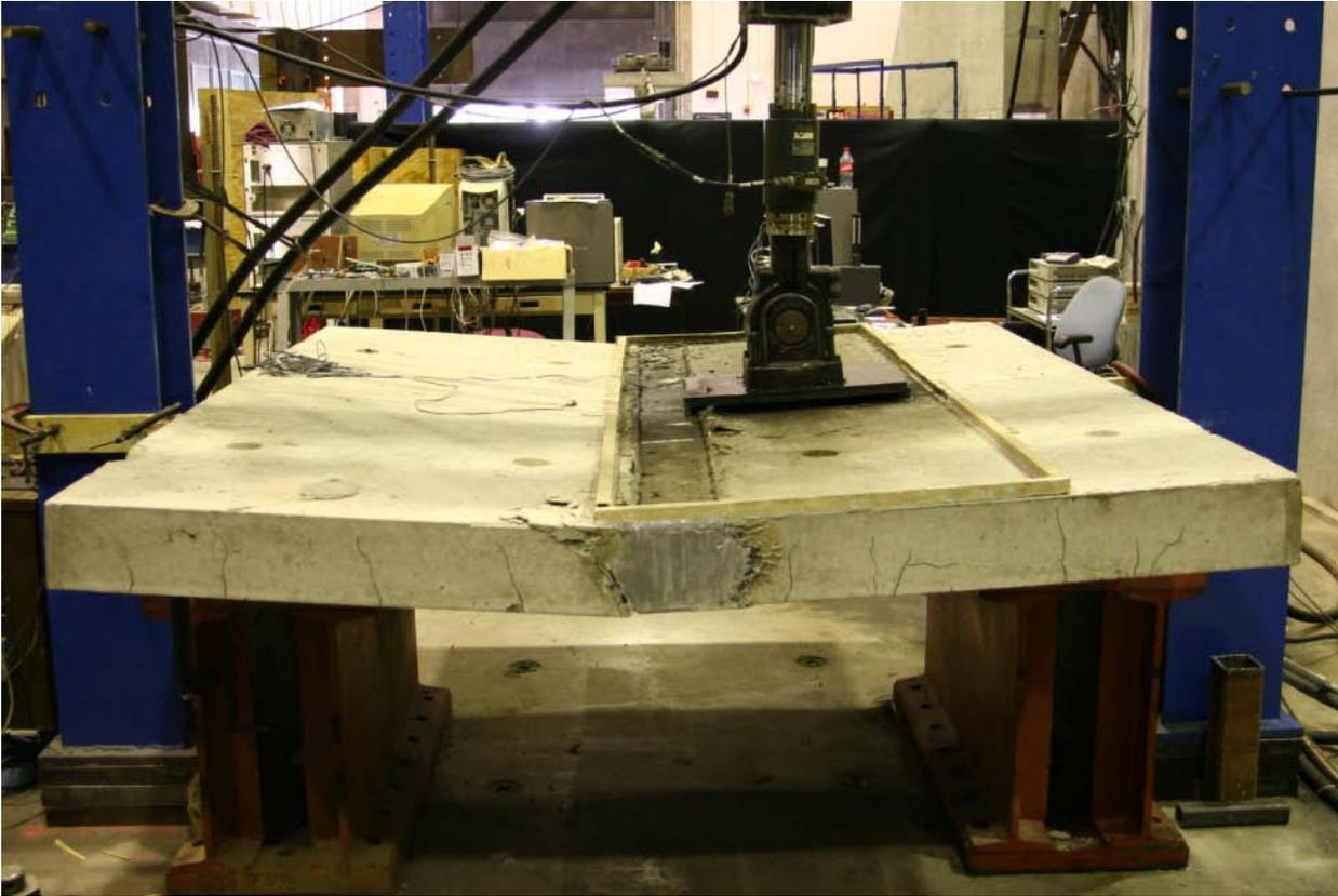
**Figure 77. Photograph. East side and top of panel 6B after the conclusion of cyclic loading.**
