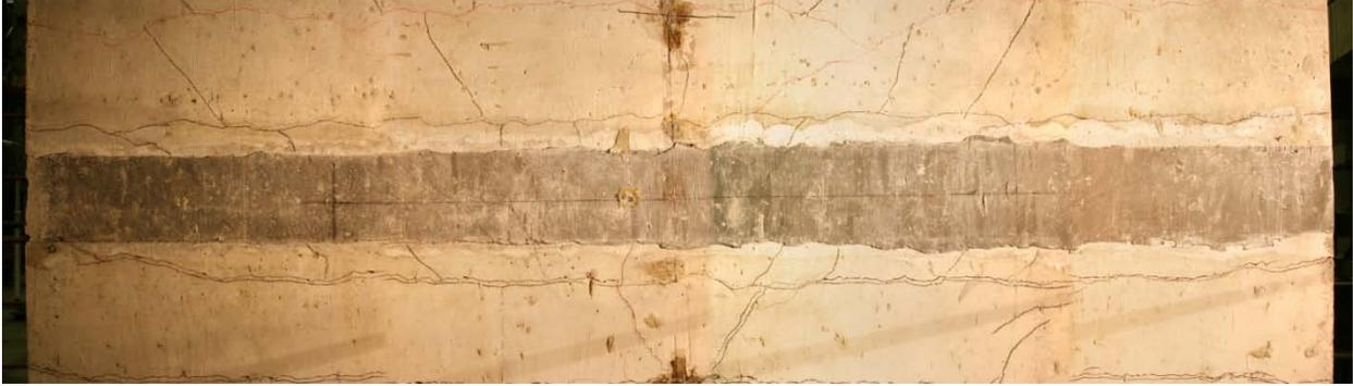
**Figure 72. Photograph. Underside of panel 6H along midspan after failure.**
