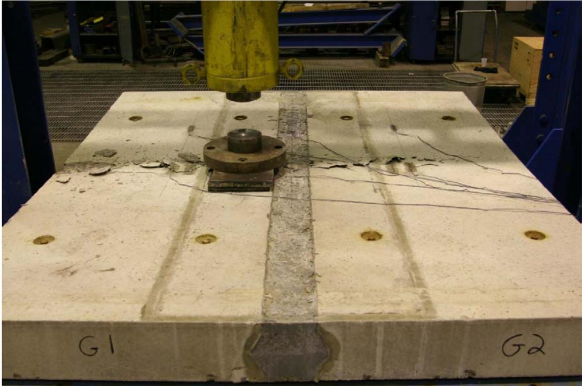
**Figure 46. Photograph. Top of panel 8G after flexural failure.**
