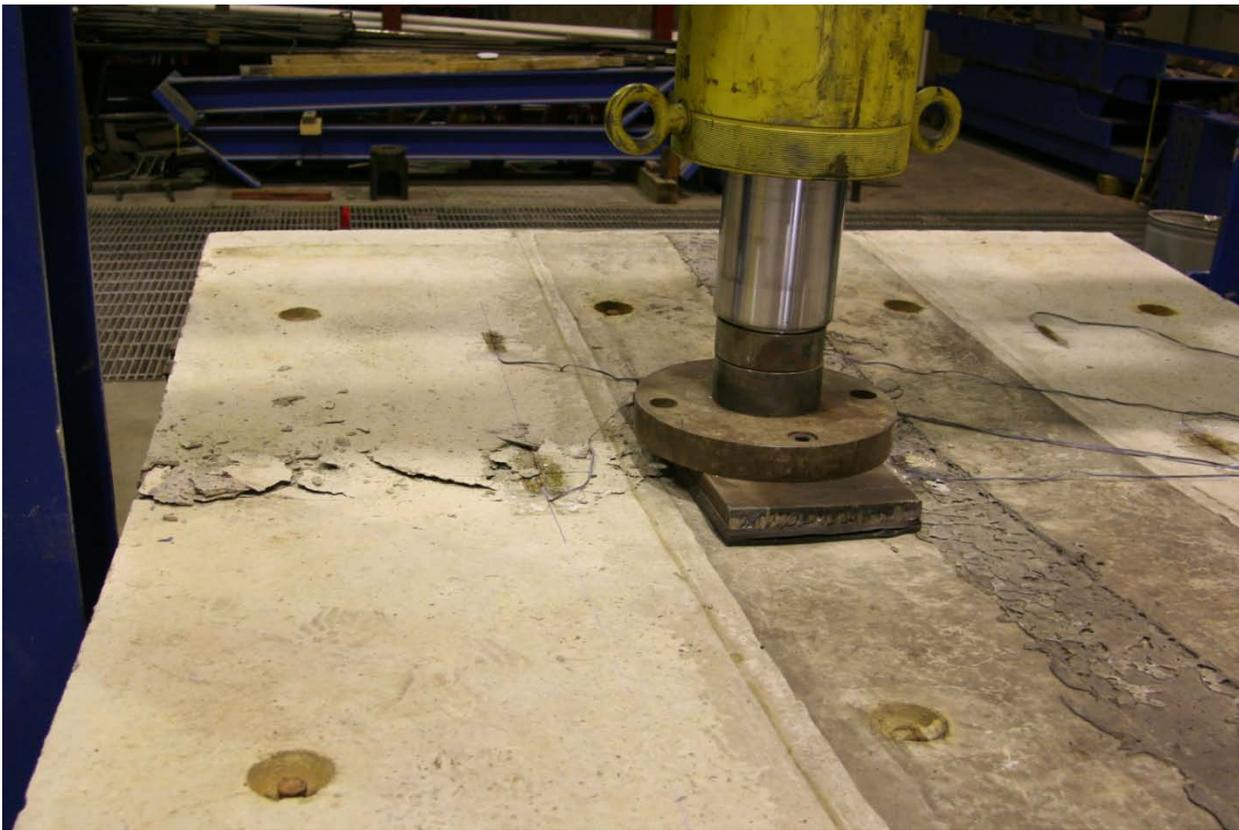
**Figure 37. Photograph. Top of panel 8E after flexural failure.**
