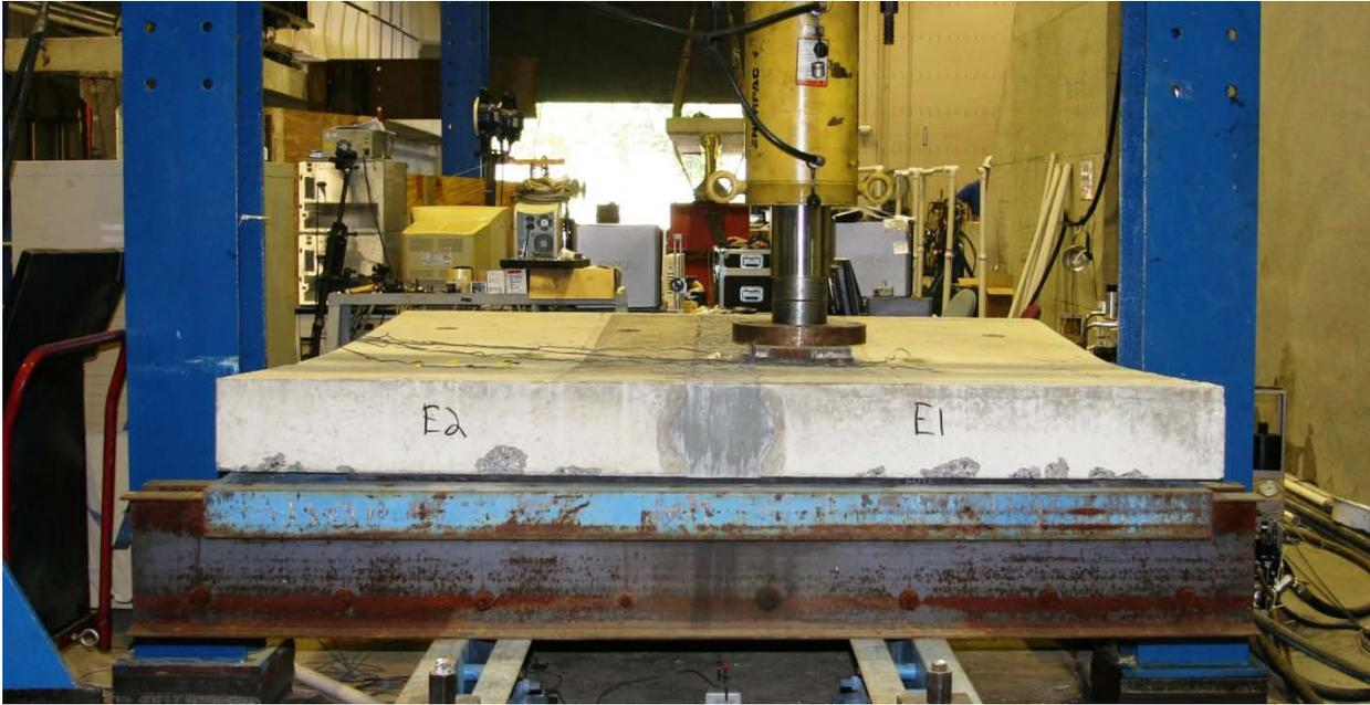
**Figure 36. Photograph. East side and top of panel 8E after 53 mm (2.1 inch) of midspan centerline deflection.**
