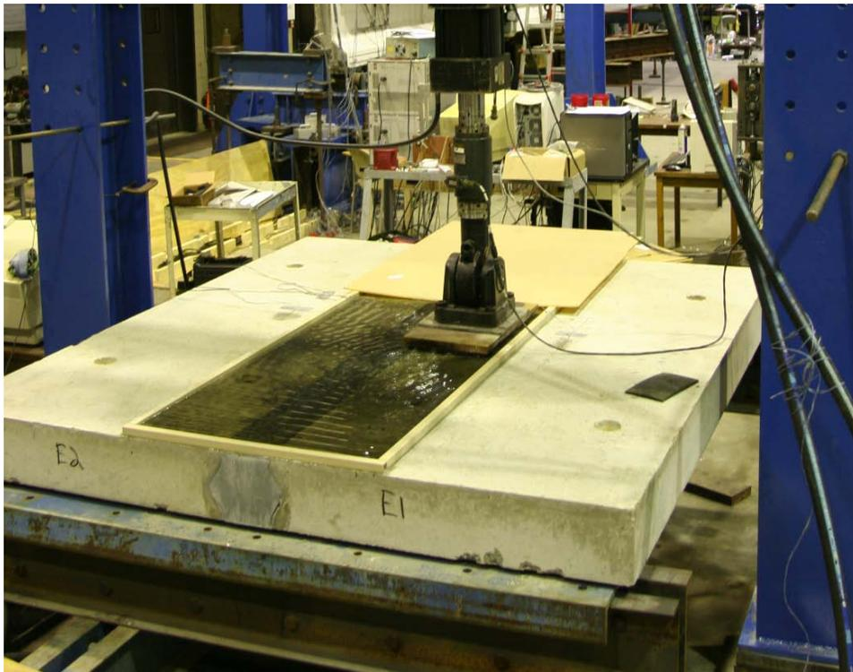
**Figure 17. Photograph. Oblique view of cyclic test setup for panels 8H, 8E, 8G, and 8B.**
