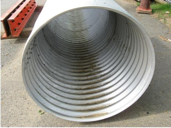
Figure 2: CMP Lateral Cross Section View
