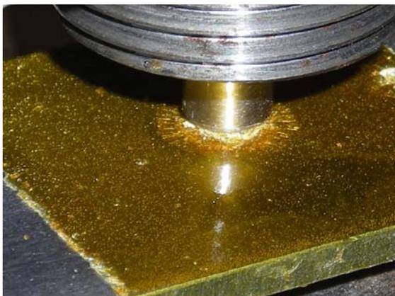
Fig. 12. Close view of the brittle coating undergoing cracking while the PICK tool is tightened in preparation for operation
