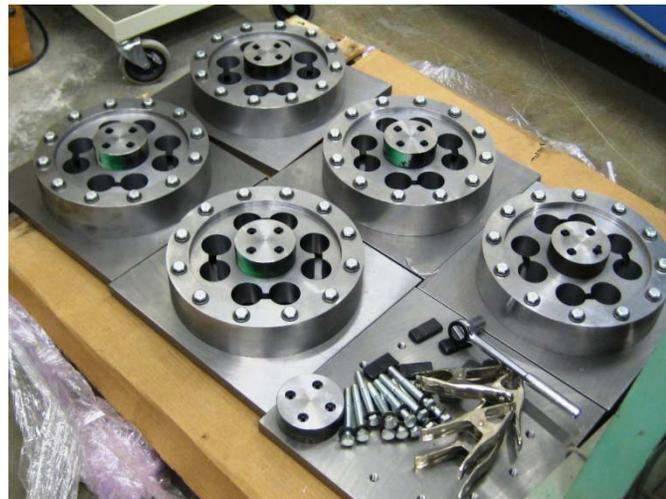
Fig. 3. As-fabricated load cells for the 30' bridge test set-up
