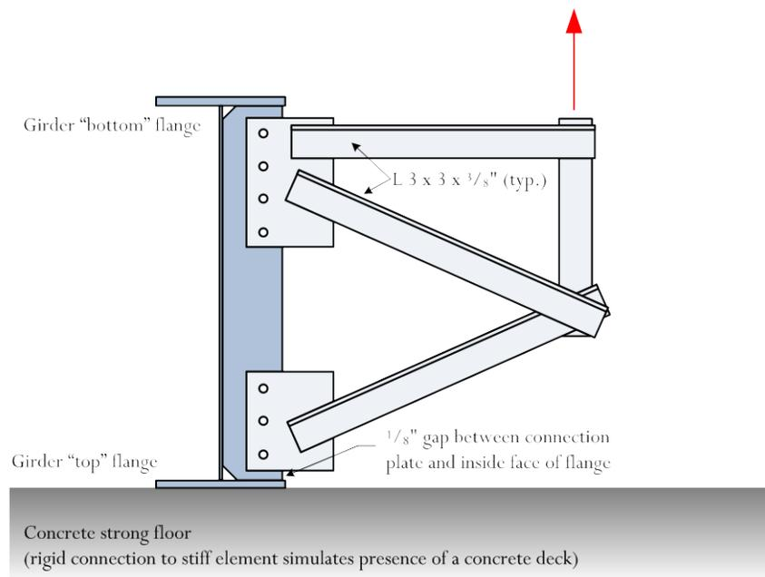
**Fig. 4. Cross-section schematic of the test set-up for the 9' girder specimens**
