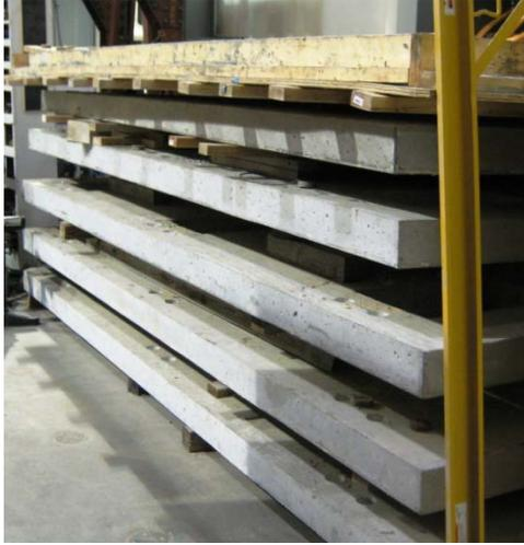
Fig. 1. Cast concrete deck slabs for the 30' bridge specimens
