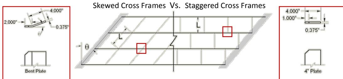
Fig. 15. Cross-frame layouts and connection stiffener geometries for bridge analyses
