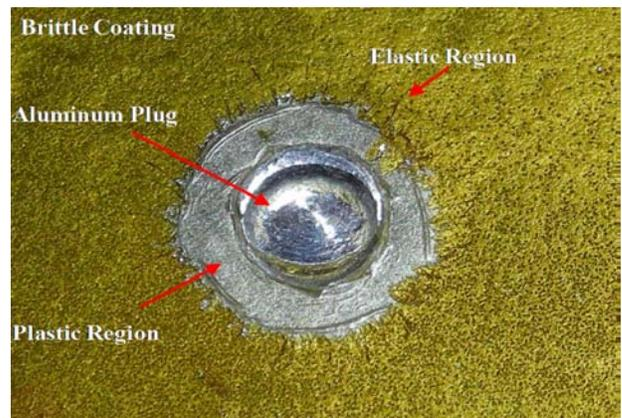
Fig. 13. Close view of the PICK-treated hole with brittle coating flaked-off in region of plasticity
