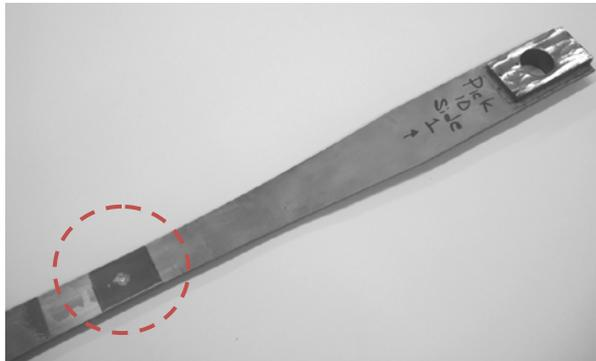
Fig. 11. View of the specimen with brittle coating applied around hole (circled region)
