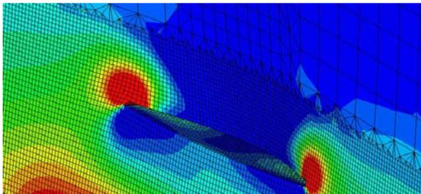
Fig. 8. View of the back of the web, showing the crack opening under distortion-induced fatigue
