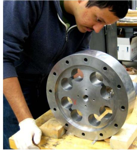
Fig. 2. Strain-gaging steel load cells for the 30' bridge test set-up
