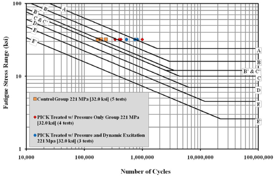
Fig. 10. S-N diagram showing results for untreated, static pressure-treated, and statically and dynamically treated specimens. All specimens were fatigue tested at 32 ksi, and data points refer to crack initiation.
