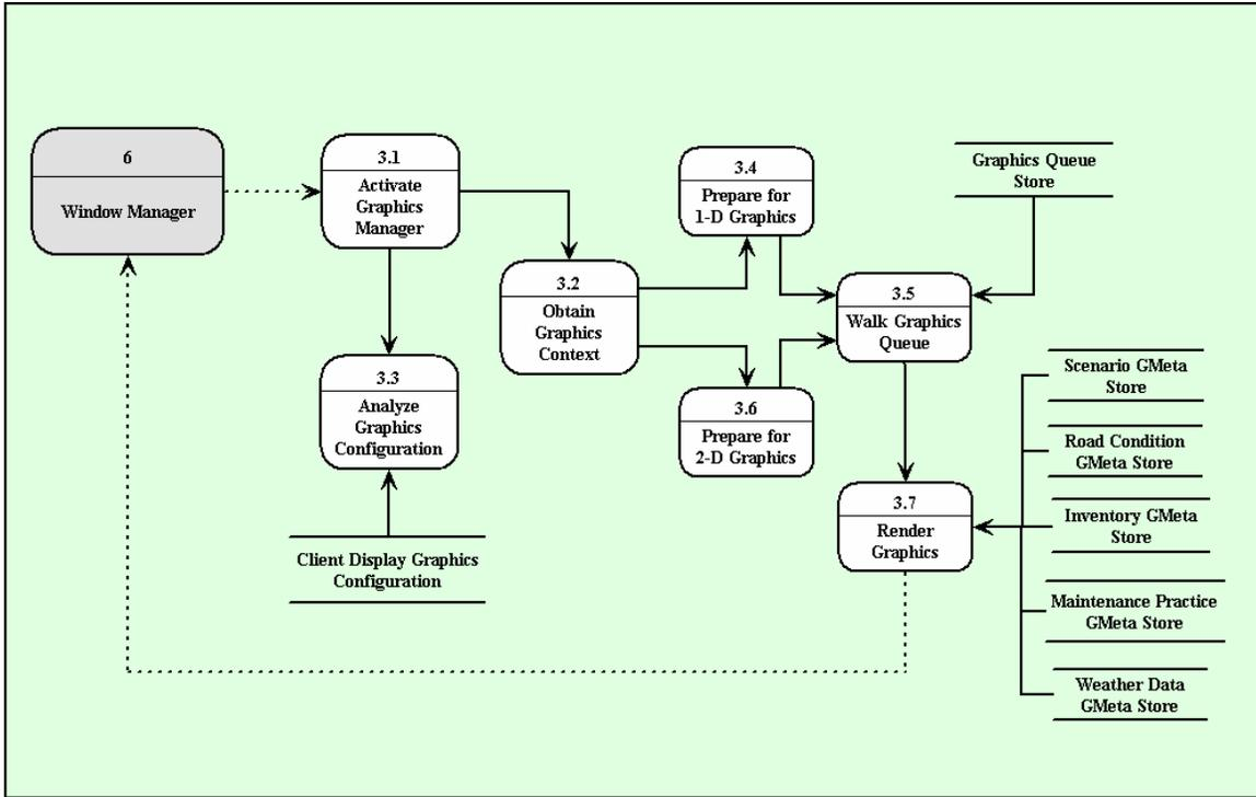
Figure B-5 Pooled Fund MDSS Level 2 Data Flow Diagram for the Graphics Generator
