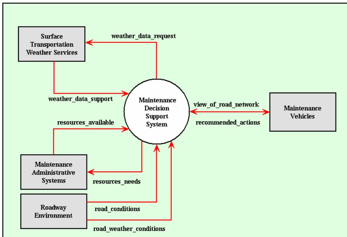
**Figure 7-6 Pooled Fund MDSS Context Diagram, Adapted from the National ITS Architecture**
