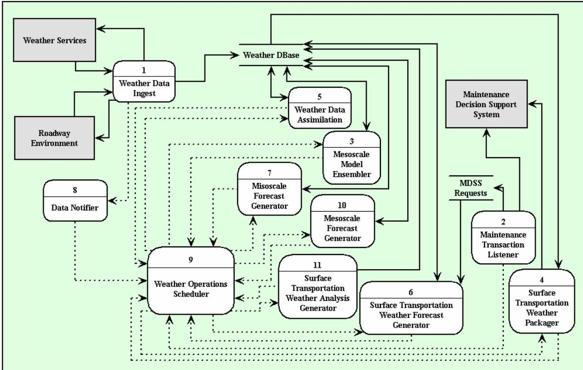
Figure B-13 Pooled Fund MDSS STWx Level 1 Data Flow Diagram
