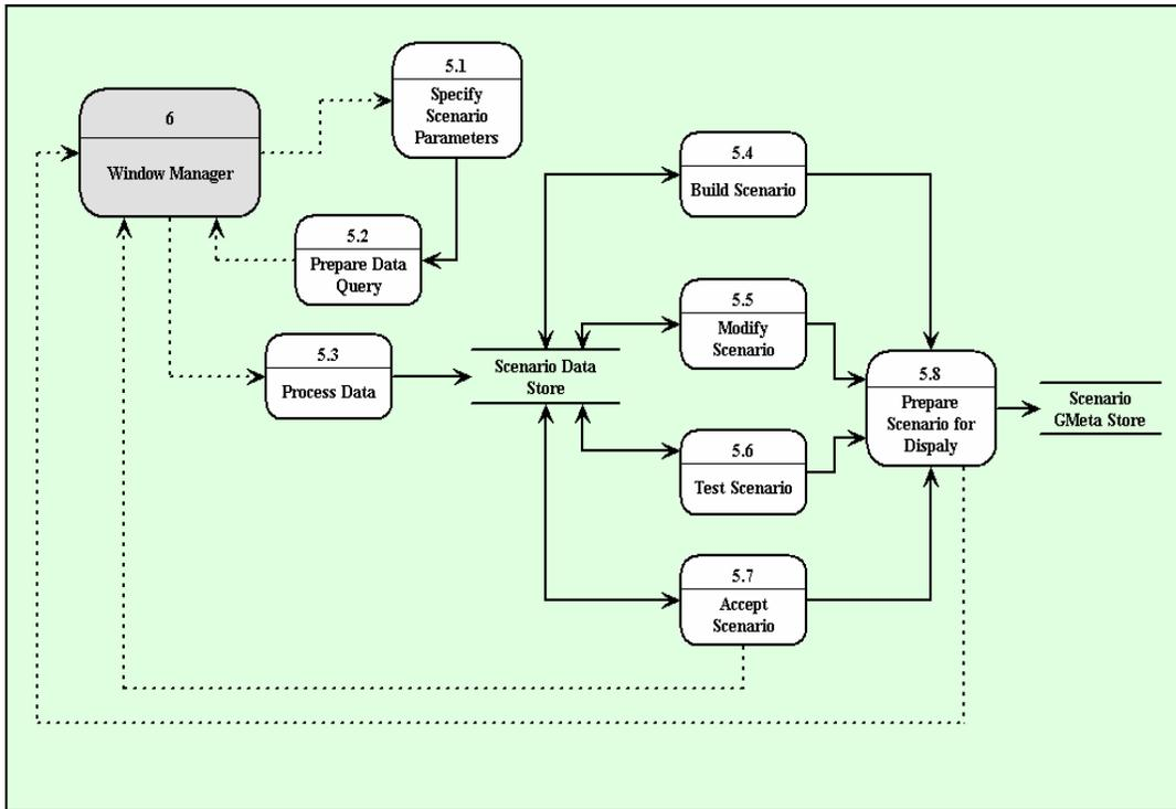
**Figure B-25 Pooled Fund MDSS Level 2 Scenario Generator Data Flow Diagram**
