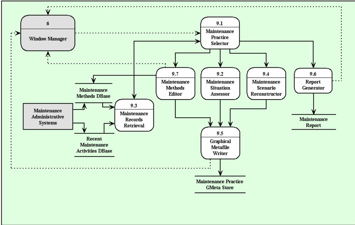
Figure B-11 Pooled Fund MDSS Level 2 Diagram for the Maintenance Practice Evaluator Process
