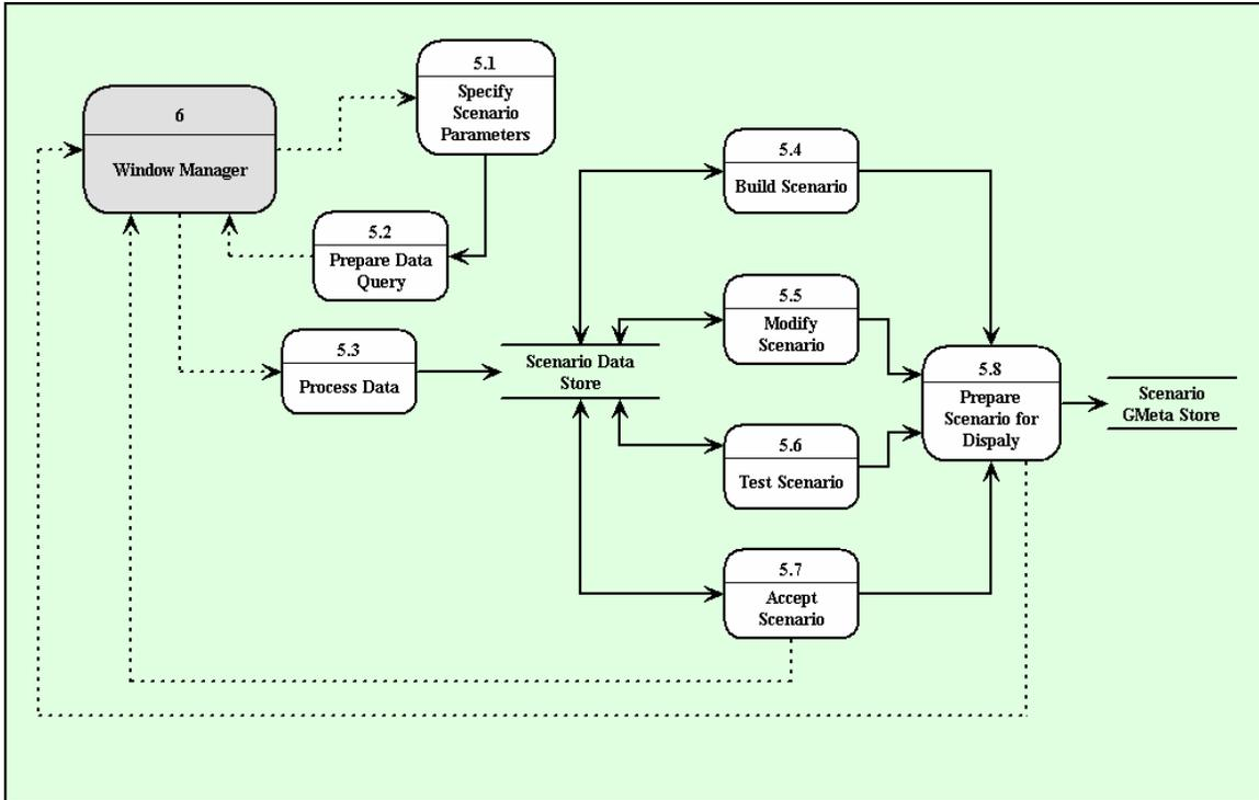
Figure B-7 Pooled Fund MDSS Level 2 Data Flow Diagram for the Scenario Generator Process
