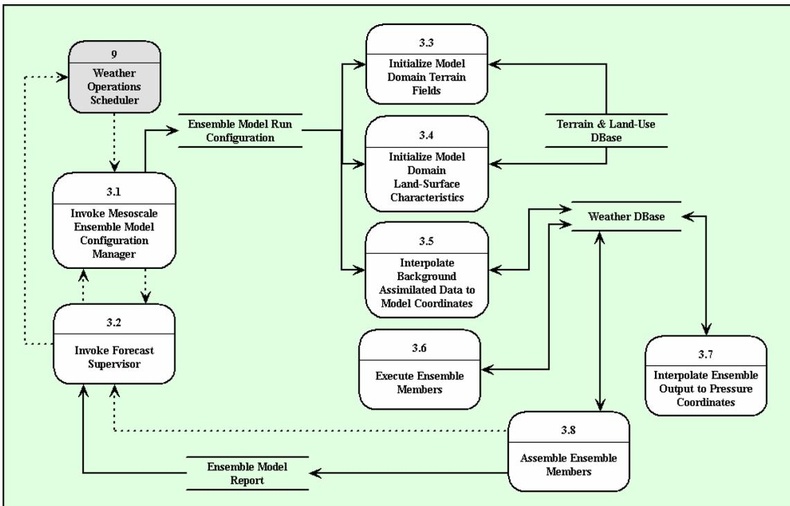
Figure B-16 Pooled Fund MDSS STWx Level 2 Data Flow Diagram for the Mesoscale Model Ensembler
