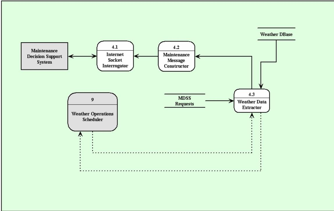
Figure B-17 Pooled Fund MDSS STWx Level 2 Data Flow Diagram for the Surface Transportation Weather Packager Process
