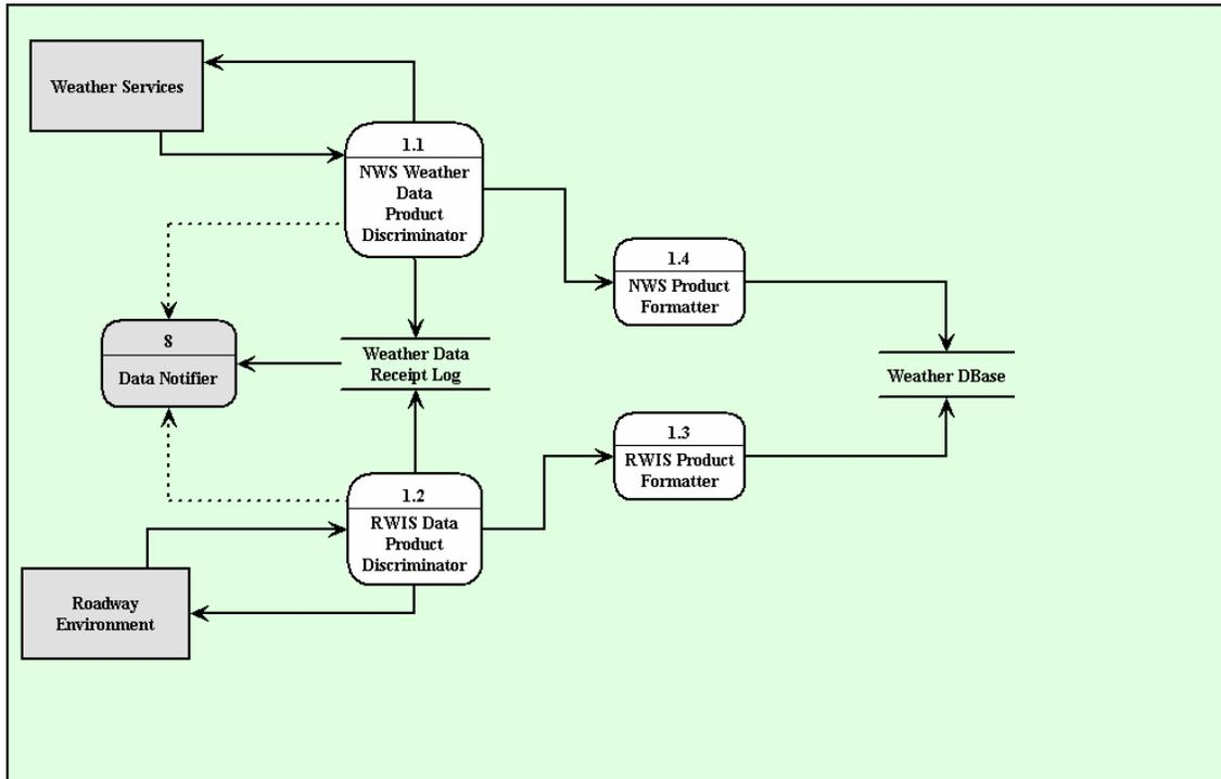
Figure B-14 Pooled Fund MDSS STWx Level 2 Data Flow Diagram for the Weather Data Ingest Process
