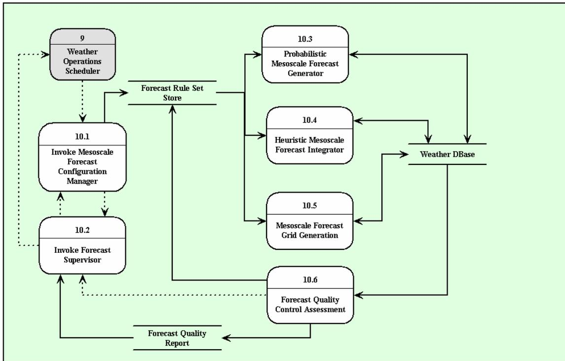
Figure B-23 Pooled Fund MDSS STWx Level 2 Data Flow Diagram for the Mesoscale Forecast Generator Process
