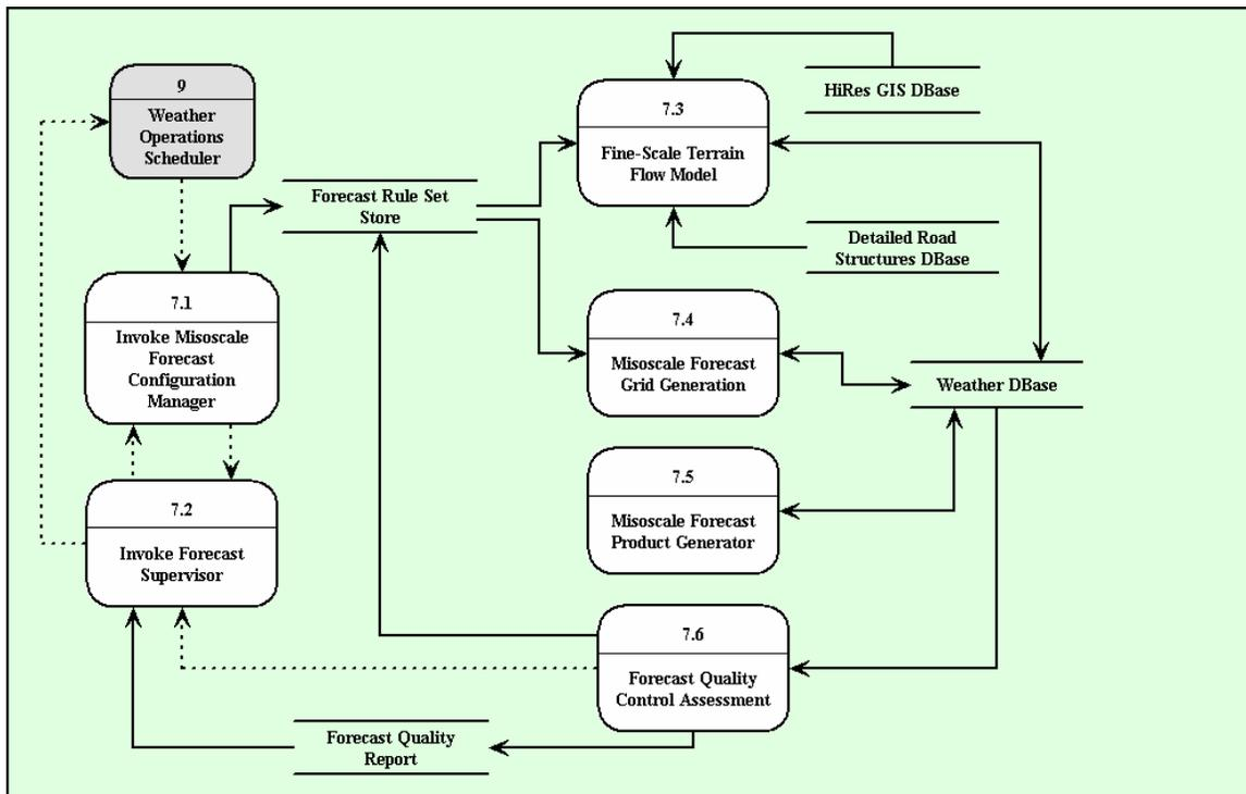
**Figure B-20 Pooled Fund MDSS STWx Level 2 Data Flow Diagram for the Misoscale Forecast Generator Process**
