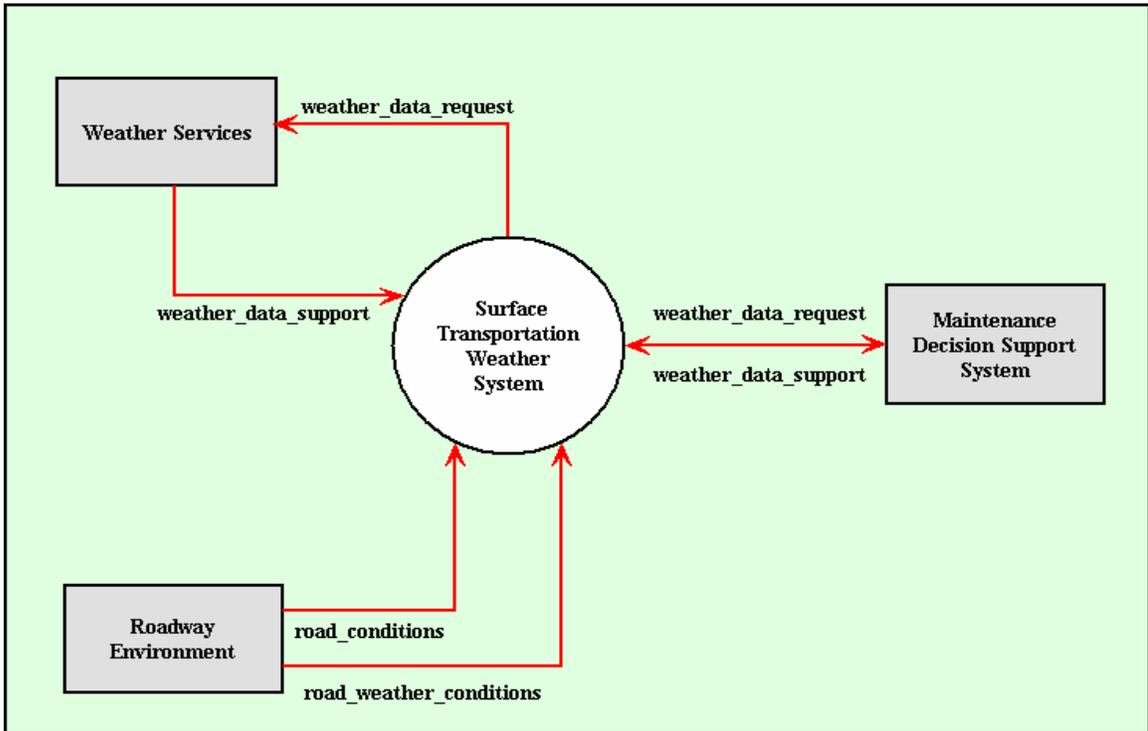
Figure B-12 Pooled Fund MDSS Context Diagram for the Surface Transportation Weather System (STWx)
