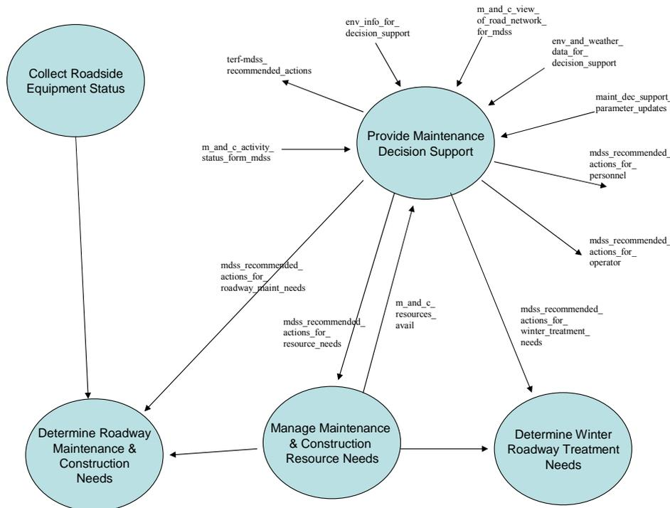
**Figure 7-5 Data Flows Associated with the “Provide Maintenance Decision Support” Process Specification from the “Determine Maintenance and Construction Needs” Logical Architecture Process of the National ITS Architecture**
