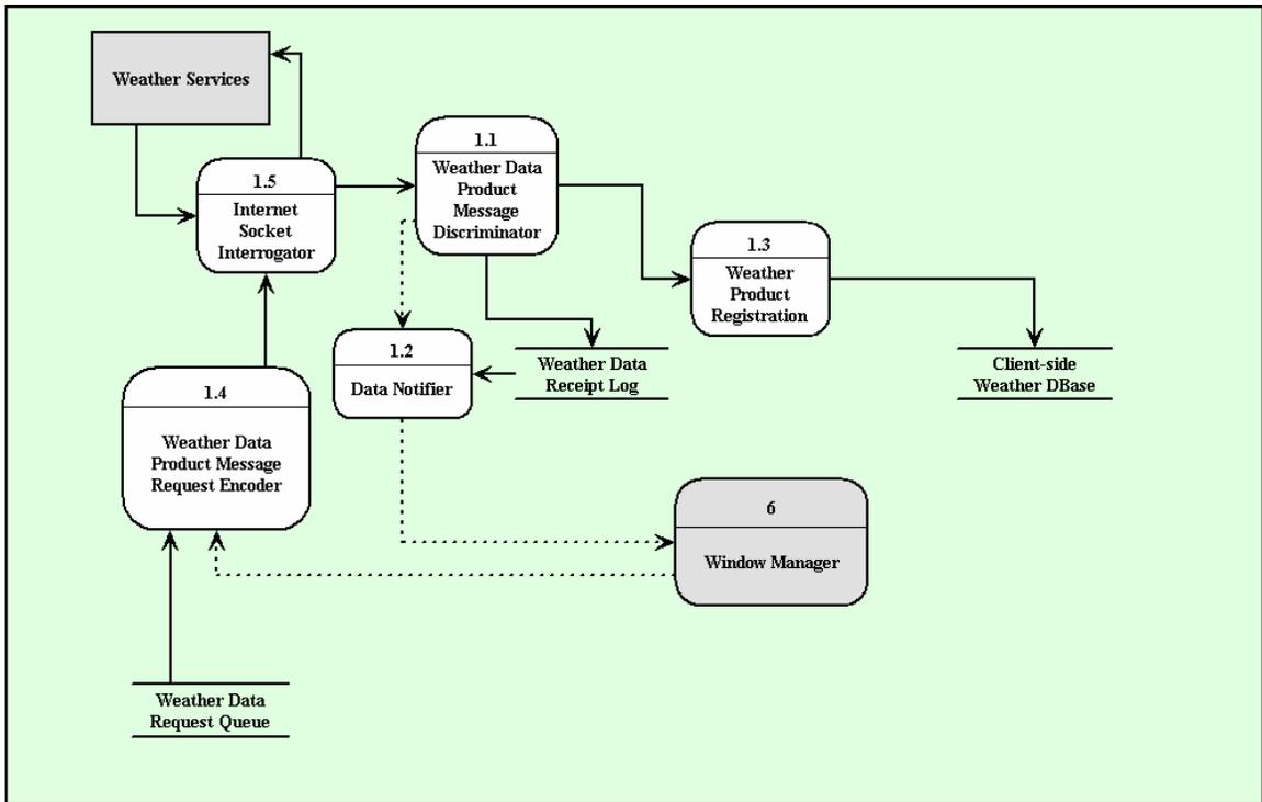
Figure B-3 Pooled Fund MDSS Level 2 Data Flow Diagram for the Weather Data Action Listener Process
