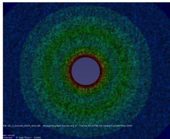
**Fig. 12.** Von Mises residual stress fields for 3% expansion of crack-stop hole
