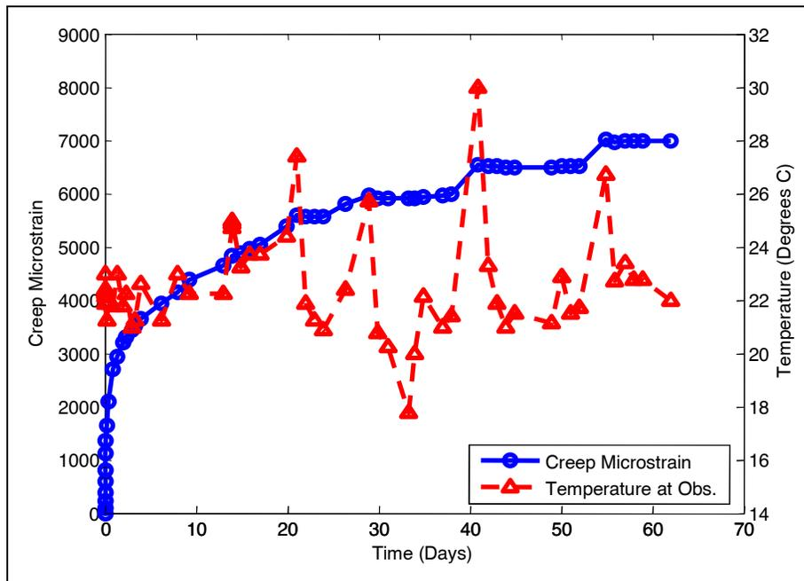
Figure C5. Upper load creep strains and temperatures.
