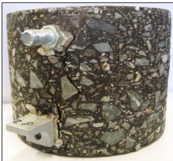
Figure C9. Typical asphalt core specimen failure.
