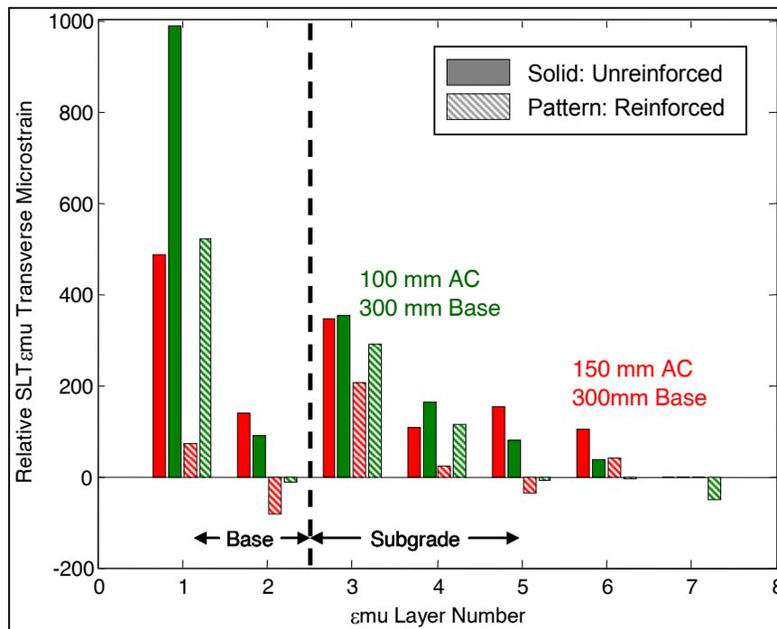
Figure 45. Average of SLT transverse elastic  $\epsilon_{mu}$  strains by  $\epsilon_{mu}$  layer for Test Sections 1 through 4 under a 48.9 kN (11 K) wheel load centered over the vertical  $\epsilon_{mu}$  stack. Matching unreinforced and reinforced test sections are shown in the same color: 100 mm AC/ 300 mm base is green and 150 mm AC/ 300 mm base is red.
