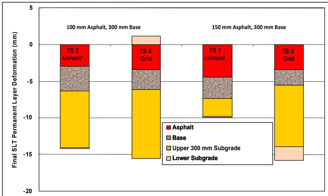
Figure 39. Permanent vertical deformations by individual emu layer for Test Sections 1-4 at the last set of SLTs (data has been adjusted according to the procedure outlined in this section).
