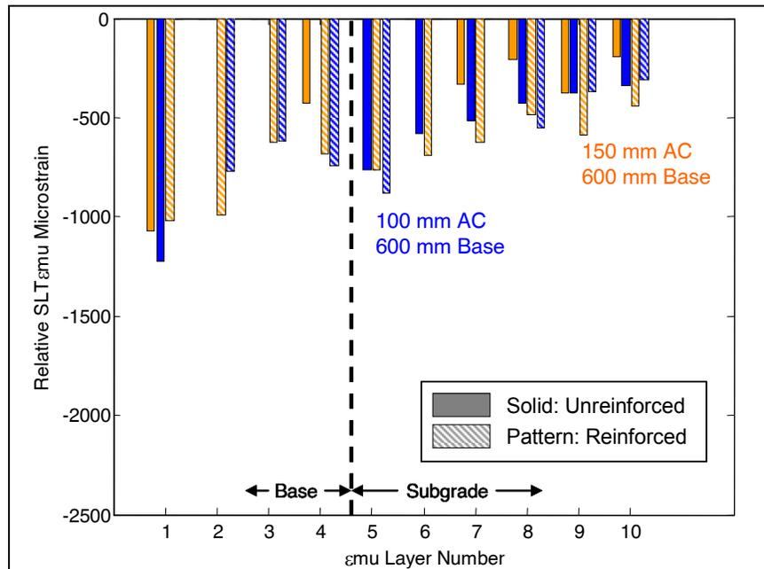
Figure 44. Average of SLT vertical elastic  $\epsilon_{mu}$  strains by  $\epsilon_{mu}$  layer for Test Sections 5 through 8 under a 48.9 kN (11 K) wheel load centered over the longitudinal  $\epsilon_{mu}$  stack. Matching unreinforced and reinforced test sections are shown in the same color: 100 mm AC/ 600 mm base is blue and 150 mm AC/ 600 mm base is gold.
