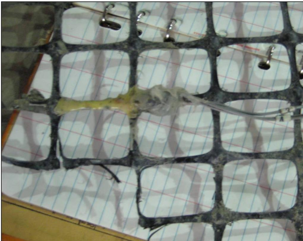
Figure B26. Close-up of Geogrid strain gages removed from TS 7 by the excavator.
