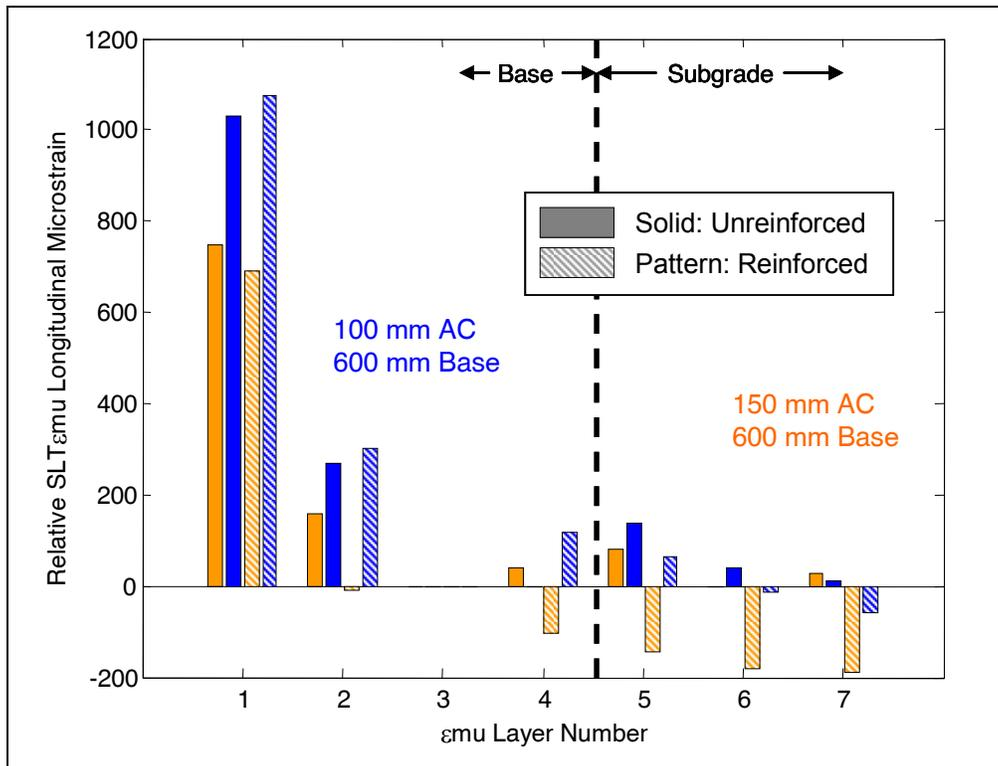
Figure 48. Average of SLT longitudinal elastic  $\epsilon_{mu}$  strains by  $\epsilon_{mu}$  layer for Test Sections 5 through 8 under a 48.9 kN (11 K) wheel load centered over the vertical  $\epsilon_{mu}$  stack. Matching unreinforced and reinforced test sections are shown in the same color: 100 mm AC/ 600 mm base is blue and 150 mm AC/ 600 mm base is gold.
