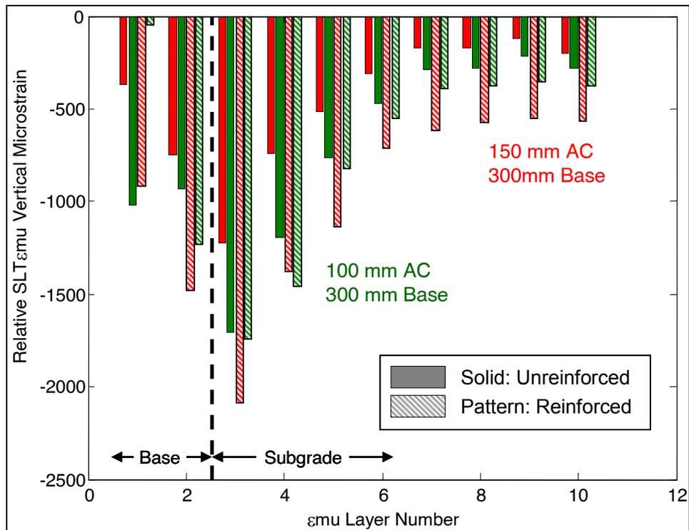
Figure 43. Average of SLT vertical elastic  $\epsilon_{\mu}$  strains by  $\epsilon_{\mu}$  layer for Test Sections 1 through 4 under a 48.9 kN (11 K) wheel load centered over the longitudinal  $\epsilon_{\mu}$  stack. Matching unreinforced and reinforced test sections are shown in the same color: 100 mm AC/ 300 mm base is green and 150 mm AC/ 300 mm base is red.
