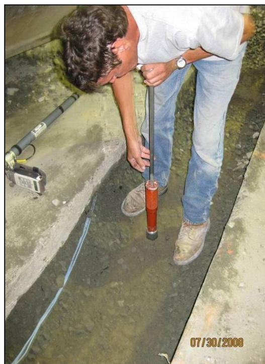
Figure B14. Drive cylinder used on surface of subgrade to determine moisture and density.
