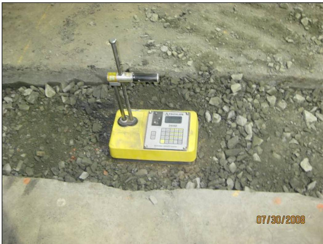
Figure B12. Soil moisture and density measurements taken with the Troxler nuclear gage.
