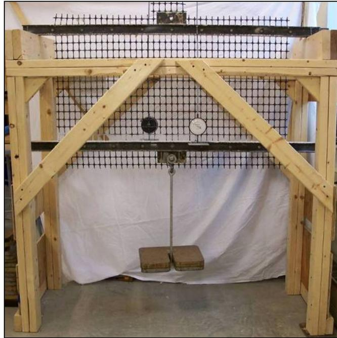
Figure C1. Photo of Geogrid creep test setup.
