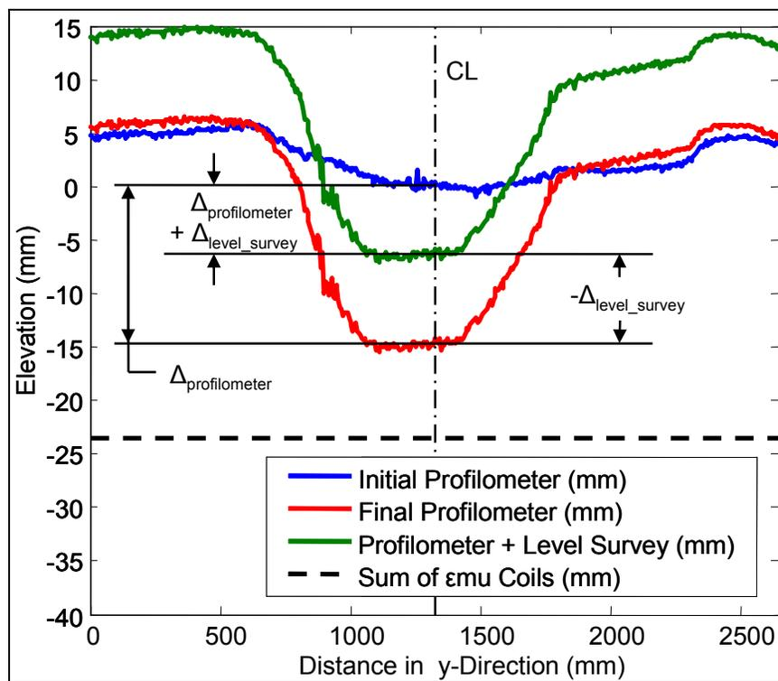
Figure 32. Example of deformation measurements for Test Section 2.
