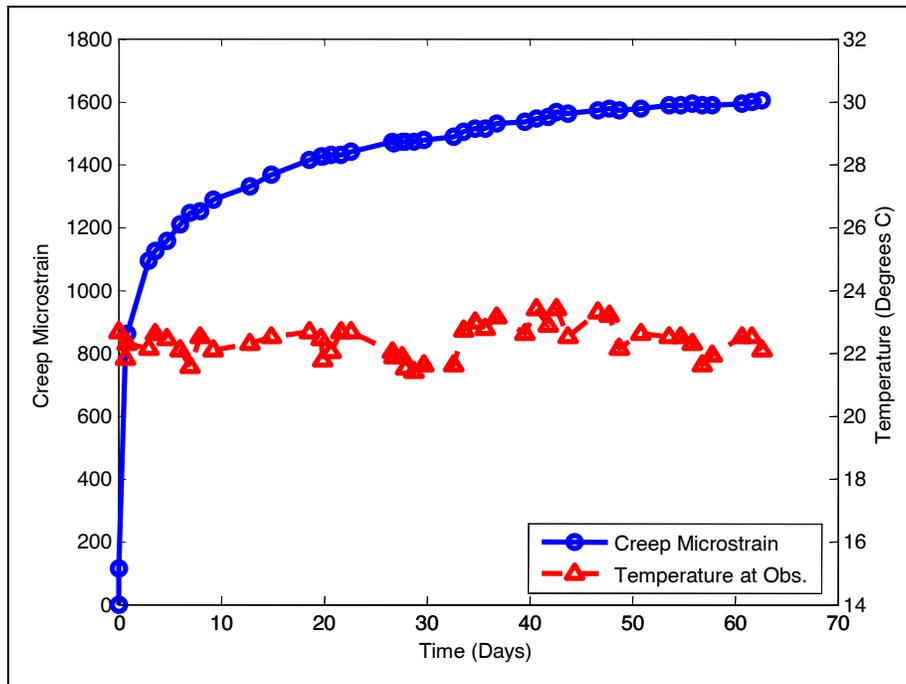
Figure C4. Lower load creep strains and temperatures.
