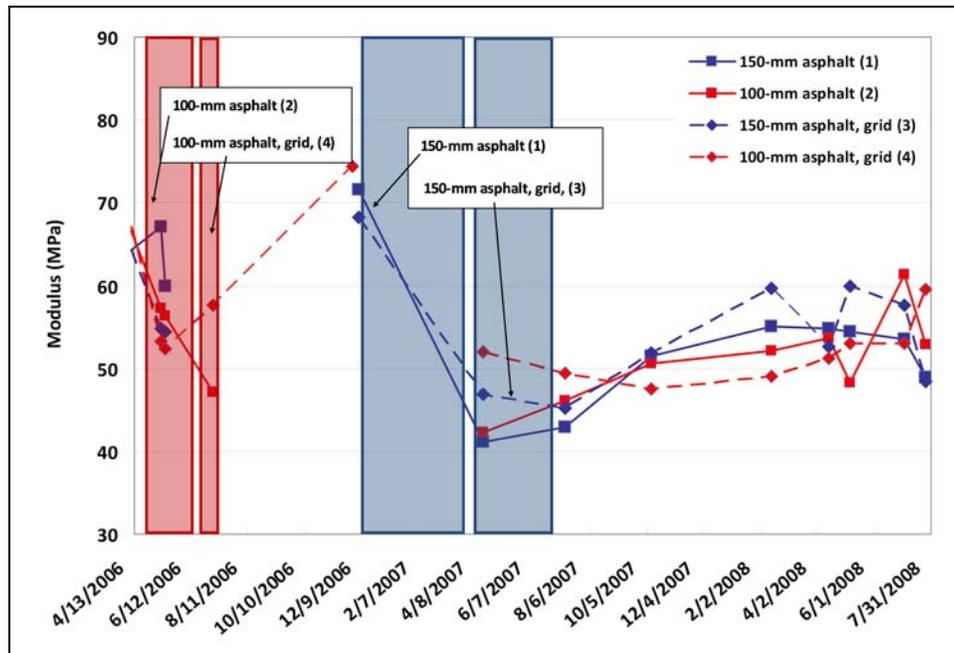
Figure 14. Estimated subgrade modulus values for Test Sections 1-4 with a base layer thickness of 300 mm for the trafficking phase of the test program. The shaded portions of the figure indicate when trafficking was conducted. Labels indicate which test section was trafficked.
