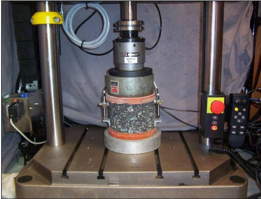
Figure C8. Asphalt core testing setup.
