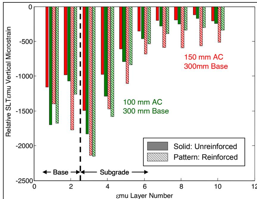
Figure 41. Average of SLT vertical elastic  $\epsilon$ mu strains by  $\epsilon$ mu layer for Test Sections 1 through 4 under a 48.9 kN (11 K) wheel load centered over the vertical  $\epsilon$ mu stack. Matching unreinforced and reinforced test sections are shown in the same color: 100 mm AC/ 300 mm base is green and 150 mm AC/ 300 mm base is red.
