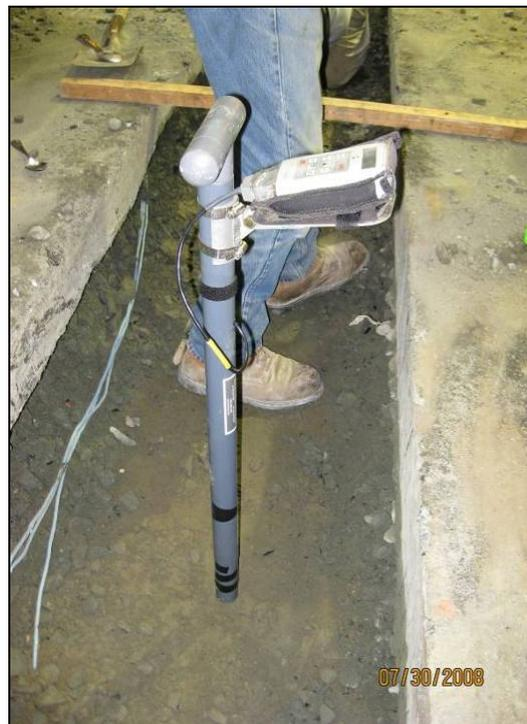
Figure B13. Dynamax ML2 probe used to take volumetric moisture content readings on the subgrade.
