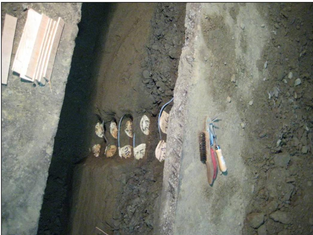
Figure B32. Exposed emu coils in TS 2.
