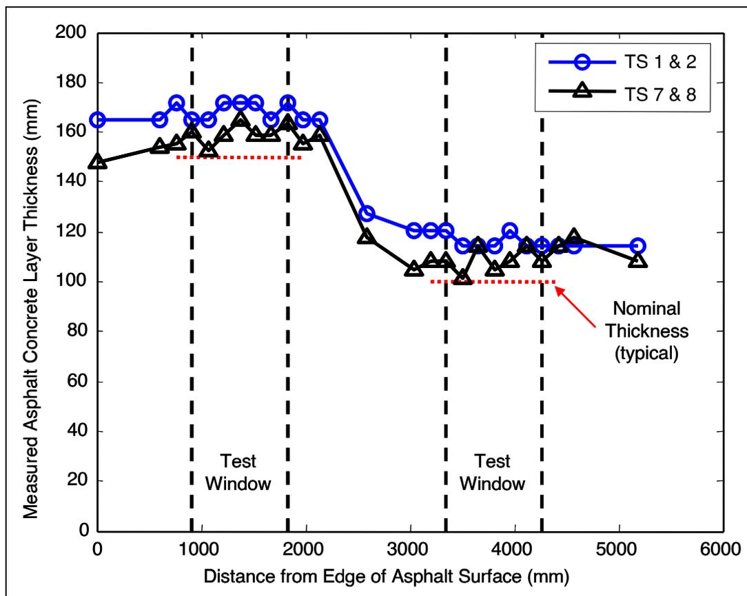
Figure B34. Measured and nominal AC layer thickness profiles for TS 1, 2, 7, and 8.
