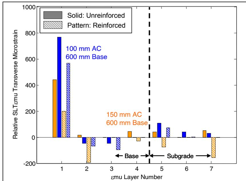
Figure 46. Average of SLT transverse elastic  $\epsilon_{\mu}$  strains by  $\epsilon_{\mu}$  layer for Test Sections 5 through 8 under a 48.9 kN (11 K) wheel load centered over the vertical  $\epsilon_{\mu}$  stack. Matching unreinforced and reinforced test sections are shown in the same color: 100 mm AC/ 600 mm base is blue and 150 mm AC/ 600 mm base is gold.
