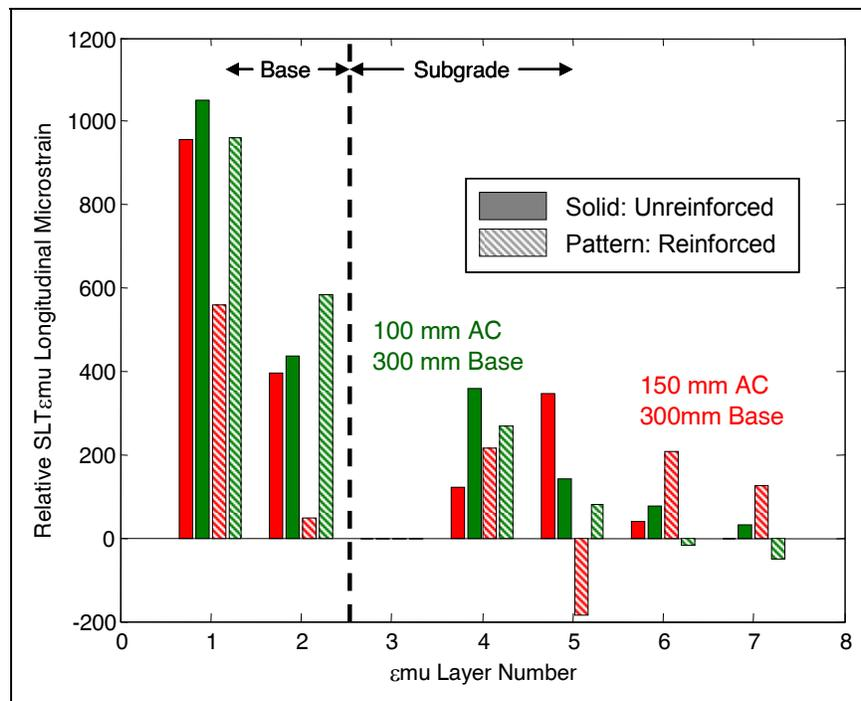
Figure 47. Average of SLT longitudinal elastic  $\epsilon_{\mu}$  strains by  $\epsilon_{\mu}$  layer for Test Sections 1 through 4 under a 48.9 kN (11 K) wheel load centered over the vertical  $\epsilon_{\mu}$  stack. Matching unreinforced and reinforced test sections are shown in the same color: 100 mm AC/ 300 mm base is green and 150 mm AC/ 300 mm base is red.
