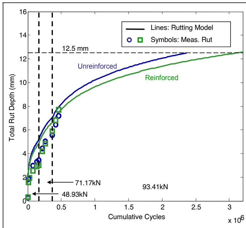
Figure 76. Rutting model predictions and measured surface rut depths for test sections 5 and 7 (data from Test Sections 5 and 7 not used for calibration).
