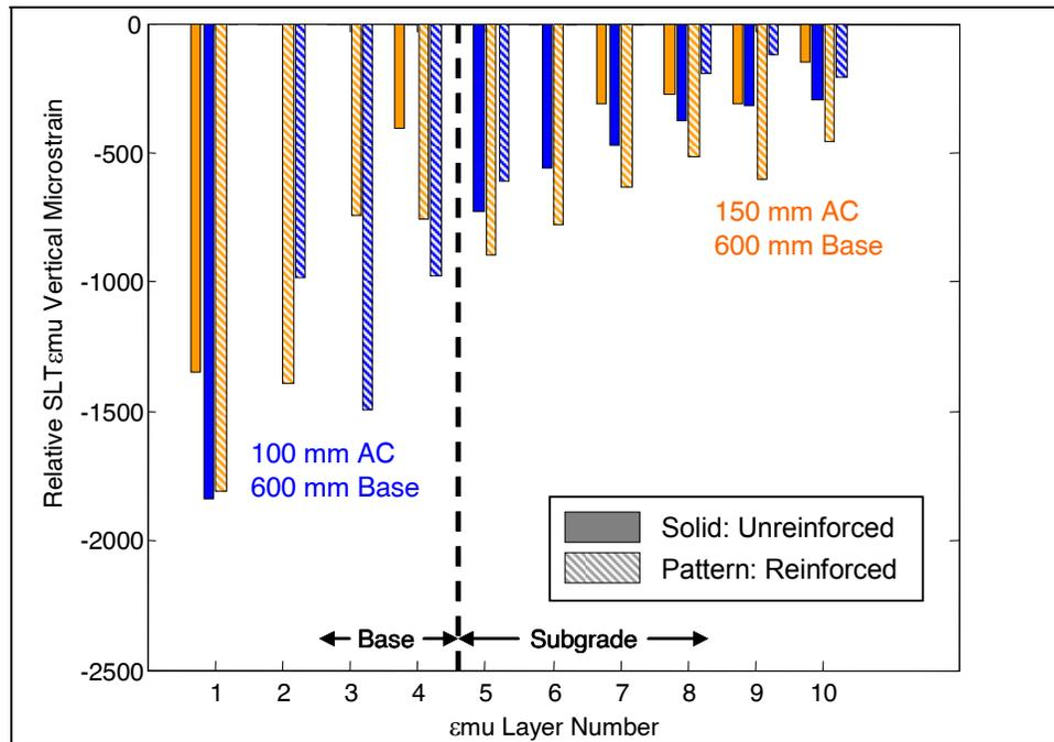
Figure 42. Average of SLT vertical elastic  $\epsilon_{\mu}$  strains by  $\epsilon_{\mu}$  layer for Test Sections 5 through 8 under a 48.9 kN (11 K) wheel load centered over the vertical  $\epsilon_{\mu}$  stack. Matching unreinforced and reinforced test sections are shown in the same color: 100 mm AC/ 600 mm base is blue and 150 mm AC/ 600 mm base is gold.
