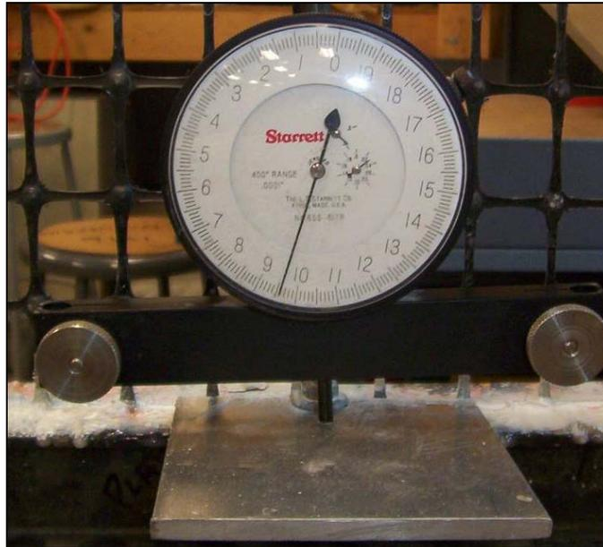
Figure C2. Close-up of dial gage used in creep test.
