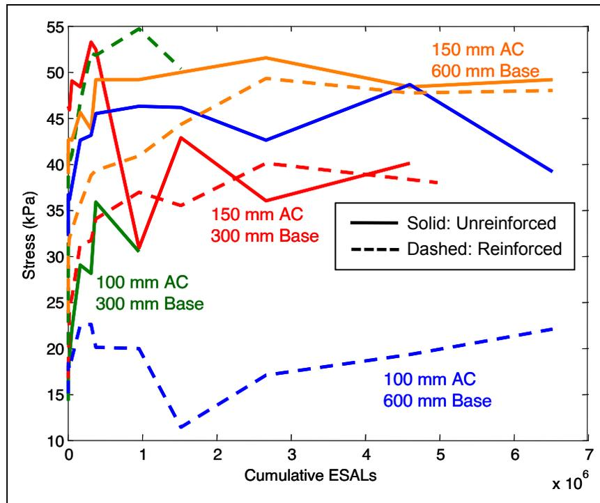
Figure 67. Vertical Geokon stresses near the top of the subgrade layer as a function of cumulative ESALs measured in an unloaded condition.
