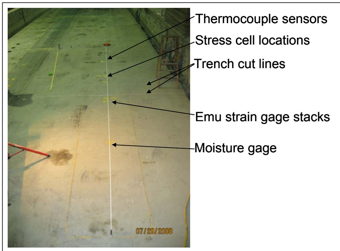
Figure B1. Test Section 1 surface condition.
