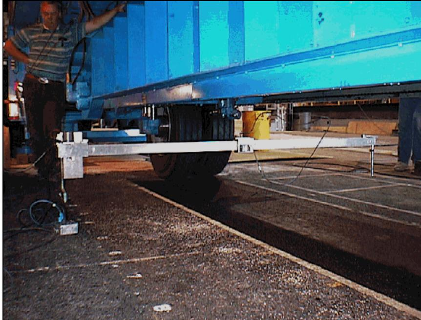
Figure 7: Surface deformation laser profilometer measurement device.
