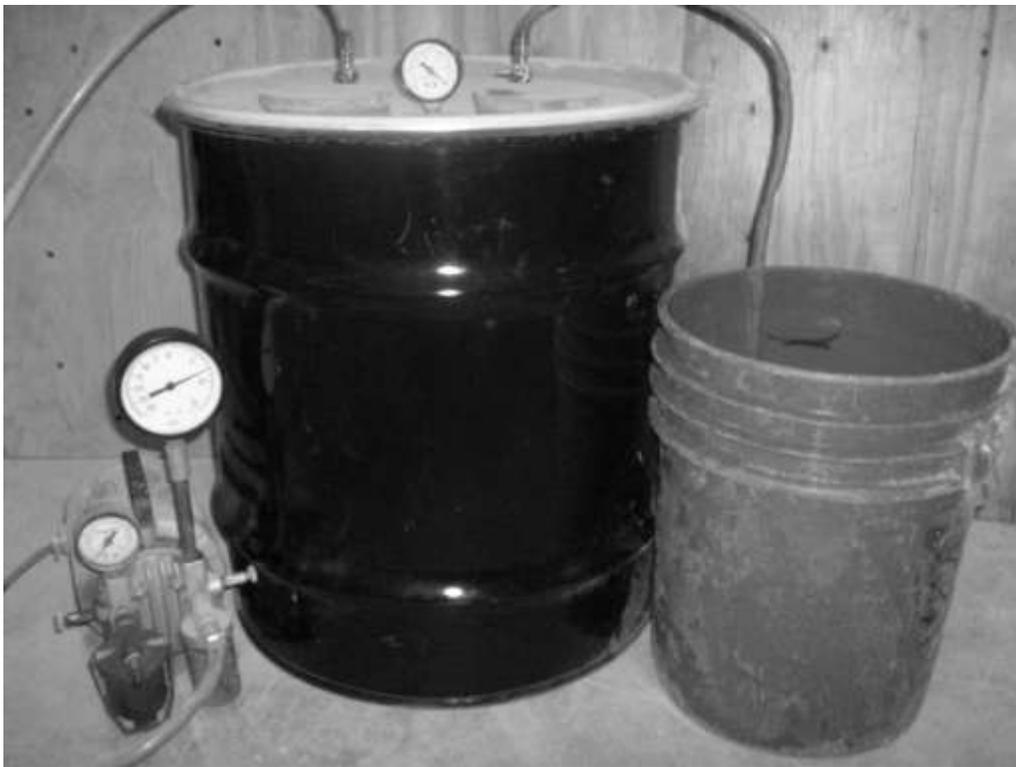
**Figure 2-4: Vacuum Saturation Equipment**
