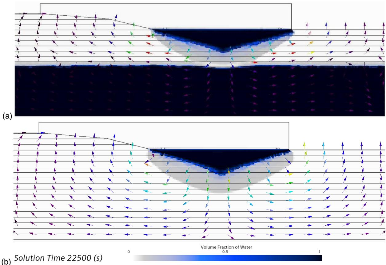
**Figure 2. Water extent after 6.25 hours of simulated time in the model (a) with underground water table close to the ditch bottom and (b) with no water table in its vicinity. Initial moisture content in the ground is zero.**
