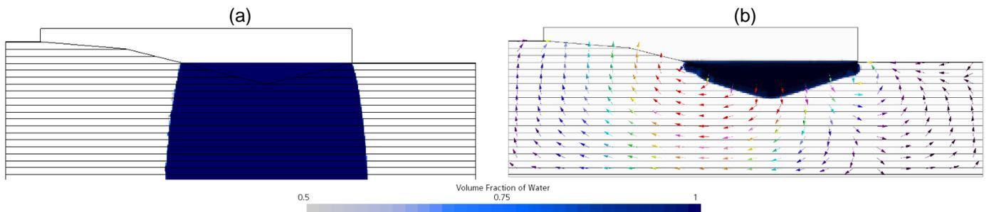
**Figure 4. Water extent at 1 hour of simulated time in the model with (a) 40% porosity, and (b) 5% porosity.**
