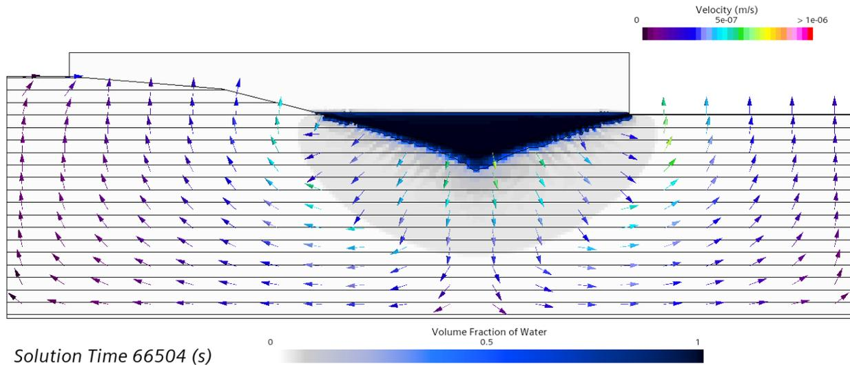
**Figure 3. Water extent at ~18.5 hours of simulated time in the model without the water table.**
