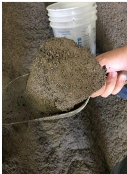
Figure 2.9: A Dense Clump of LWA Observed in the Stockpile for MN-IC-LC-HPC-5
