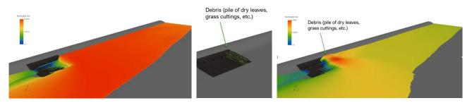
Figure 4. Comparison of flow pattern for an unobstructed (left) and partially clogged (right) grate, for example conditions of longitudinal grade 0.01 ft/ft and upstream flow spread 4 ft.
