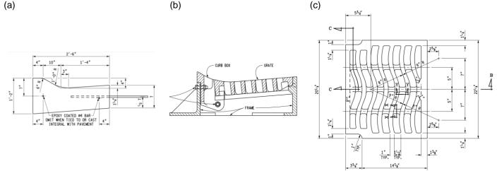
**Figure 1. Standard drawings** TPF – 5(446) Q3 2023 Report The computational domain for the on-grade condition is shown in Figure 2. It covers a section of a roadway pavement, curb and gutter and the cover C with a catch basin underneath. The geometry was recreated based on the standard drawings provided by MDOT.
