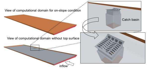
Figure 2. Computational domain for on-slope condition
