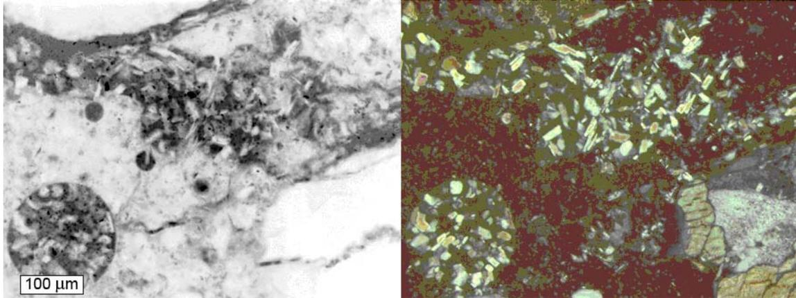
**Figure 5.101. Deteriorated 0.45 w/c straight portland cement concrete exposed to  $MgCl_2$  brine with blocky  $Ca(OH)_2$  crystals.
