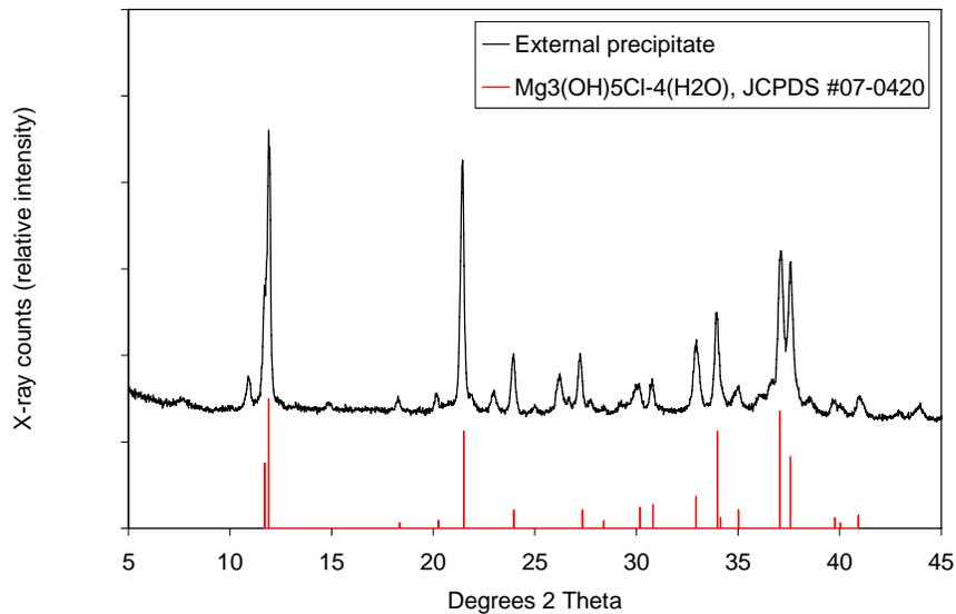
**Figure 5.78.** XRD pattern from the external precipitate collected from concrete exposed to MBAP solution for 500 days, with reference pattern for  $\text{Mg}_3(\text{OH})_5\text{Cl}\cdot 4\text{H}_2\text{O}$ .
