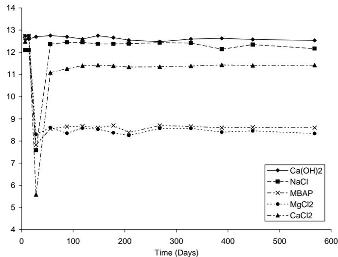
**Figure 5.33. Measured pH change during deicer exposure period.**
