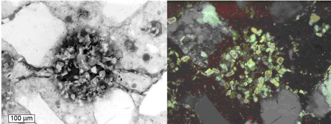
**Figure 5.93. Deteriorated portion from 0.45 w/c straight portland cement concrete exposed to  $\text{CaCl}_2$  brine with blocky  $\text{Ca(OH)}_2$  crystals.
