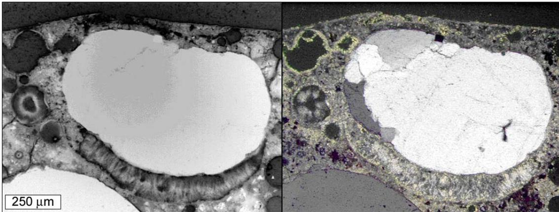
**Figure 5.12. Brucite, (magnesium hydroxide) crystals in air void and seam beneath sand grain near exterior in cylinder immersed in  $MgCl_2$  solution.
