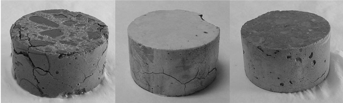
**Figure 5.50. Photographs of 4 inch [100 mm] diameter 0.45 w/c ordinary portland cement (OPC) concrete specimens after 500 days in high concentration brines. From left to right:  $\text{CaCl}_2$ ,  $\text{MgCl}_2$ , and MBAP brines.**
