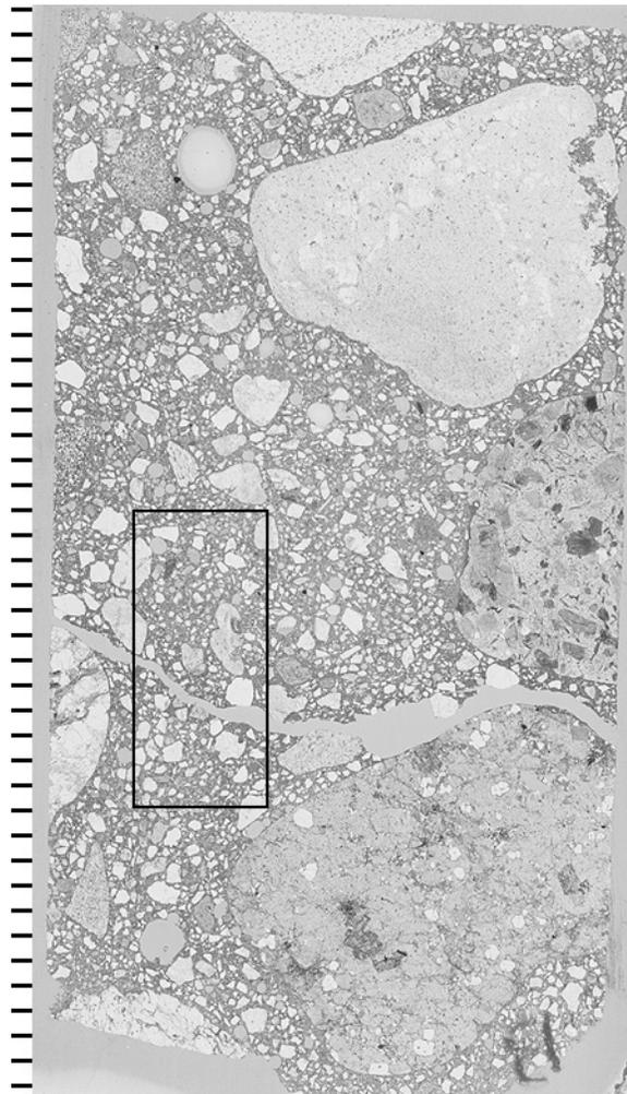
**Figure 4.39. Transmitted light scanned image of thin section to show location of elemental maps shown in Figure 4.41. The large crack, sub-parallel to the pavement surface, is at a depth of about 40 mm, (tic marks every mm).**
