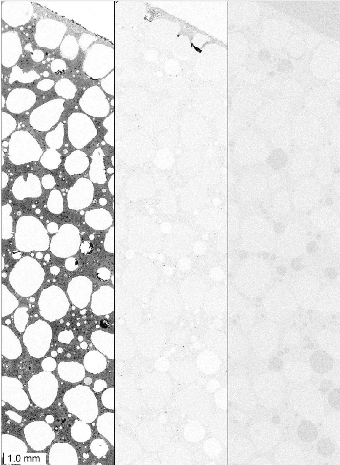
**Figure 5.22. Elemental maps, from left to right: calcium, magnesium, and chlorine. The elemental maps were collected from a thin section prepared from a cylinder immersed in calcium magnesium acetate solution. Darker areas indicate a higher concentration.**
