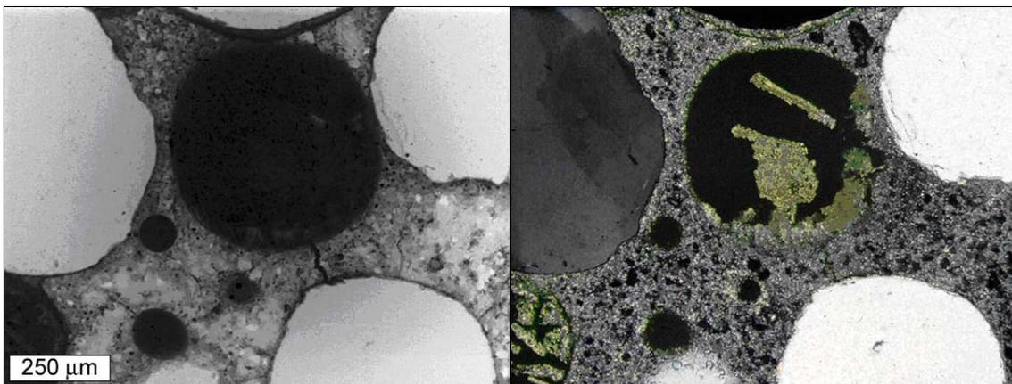
**Figure 5.10. Remnant calcium oxychloride crystals that are pseudomorphs of secondary calcium hydroxide crystals formed in an air void from  $MgCl_2$  solution immersed sample. From left to right, epifluorescent and crossed polars.**
