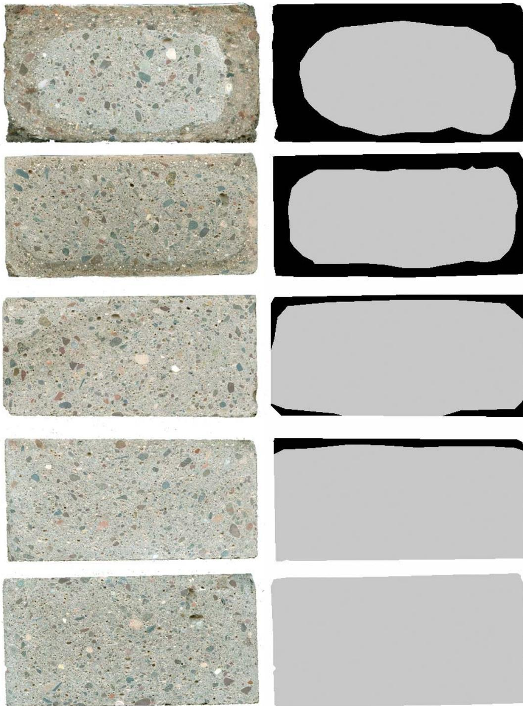
**Figure 5.53. Visible alteration on saw-cut plane through 0.45 w/c mortar specimens. From top to bottom: CaCl<sub>2</sub>, MgCl<sub>2</sub>, MBAP, NaCl & CMA high concentration brines at 500 days.**
