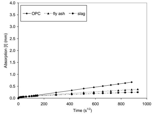
Figure 5.45. Sorptivity - concrete  $w/cm$  - 0.45 -  $MgCl_2$
