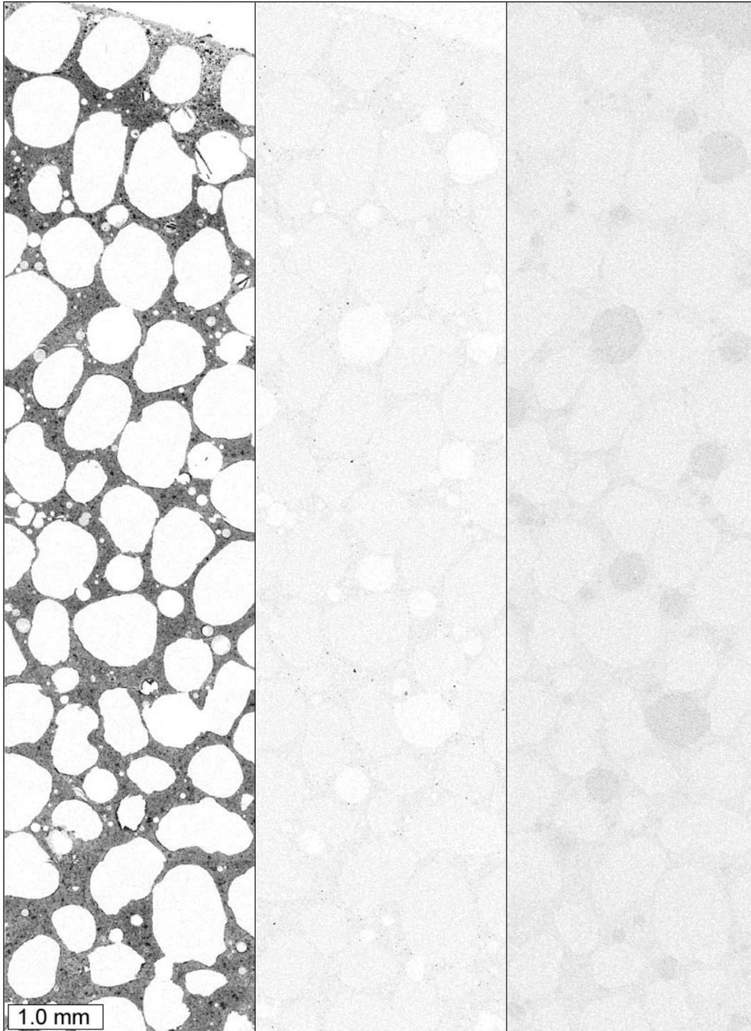
**Figure 5.24. Elemental maps, from left to right: calcium, magnesium, and chlorine. The elemental maps were collected from a thin section prepared from a cylinder immersed in limewater. Darker areas in elemental maps indicate a higher concentration.**
