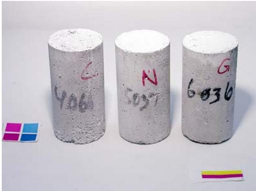
**Figure 5.25. Cylinders exposed to 3%  $\text{CaCl}_2$  solution after 56 days of constant low temperature test.**
