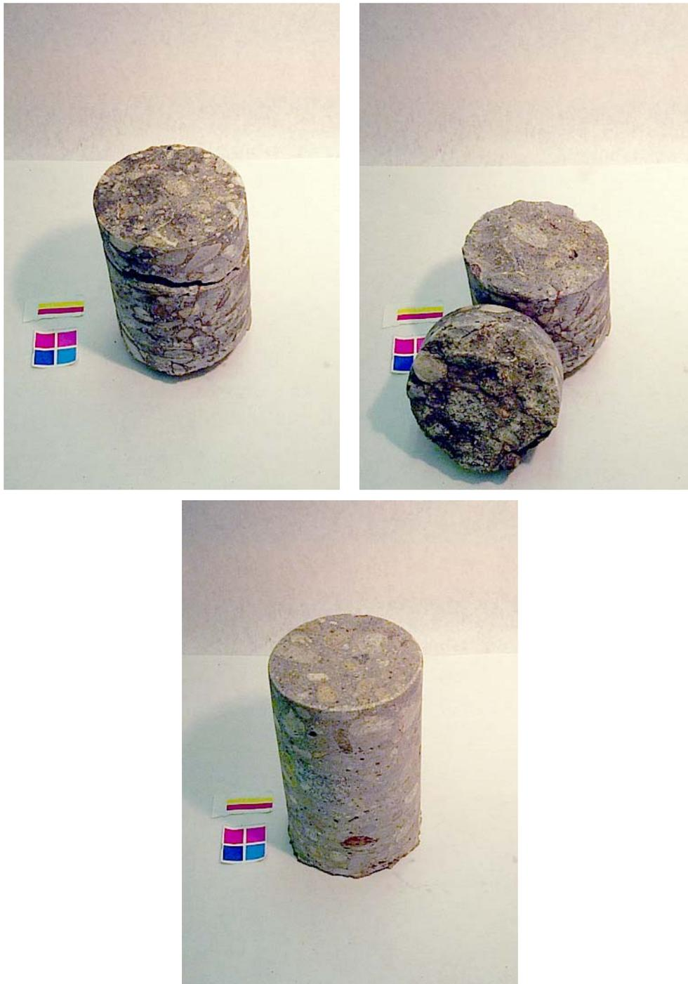
**Figure 4.29. Cores retrieved from site, core T-1 (top), core T-2 (bottom).**
