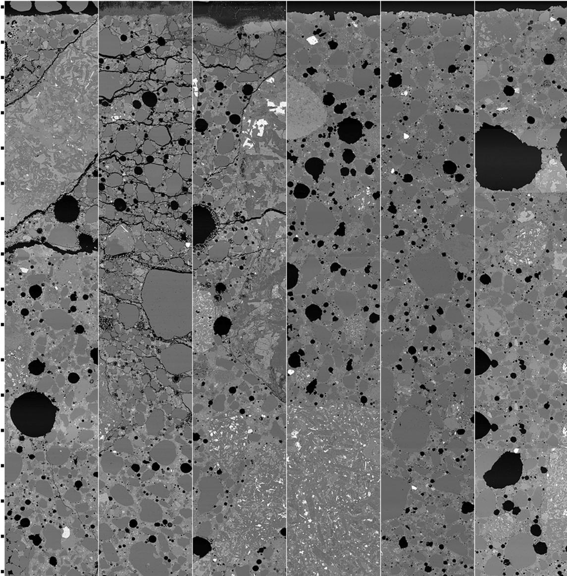
**Figure 5.107. BSE images from 0.45 w/c concrete specimens exposed to high concentration brines and the limewater control after 500 days. From left to right, CaCl<sub>2</sub>, MgCl<sub>2</sub>, MBAP, NaCl, CMA, and limewater.**
