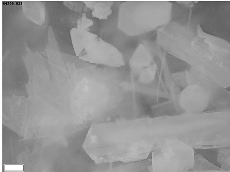
**Figure 5.70.  $\text{CaCl}_2 \cdot \text{Ca}(\text{OH})_2 \cdot 2\text{H}_2\text{O}$  crystals before, (top) and after immersion in distilled water in atmospheric equilibrium with  $\text{CO}_2$  at room temperature and subsequent alteration.
