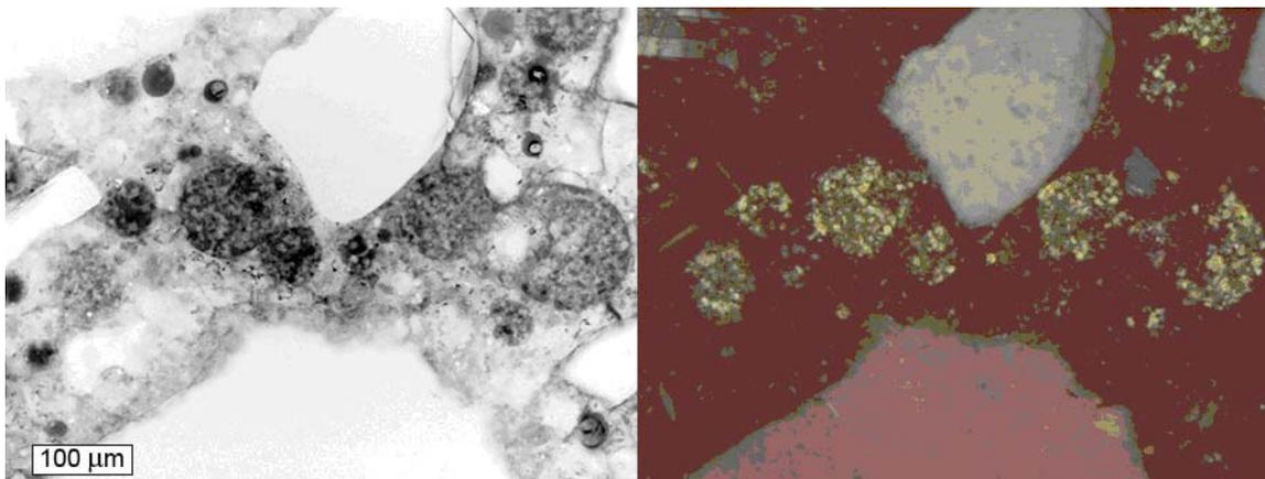
**Figure 5.102. Secondary blocky  $Ca(OH)_2$  crystals in air voids of 0.45 w/cm fly ash concrete exposed to  $MgCl_2$ .
