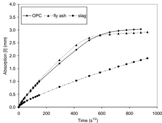
Figure 5.48. Sorptivity - concrete  $w/cm$  - 0.55 - water
