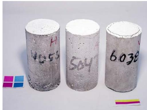
**Figure 5.28. Cylinders exposed to 14%  $\text{CaCl}_2$  solution after 56 days of constant low temperature test.**
