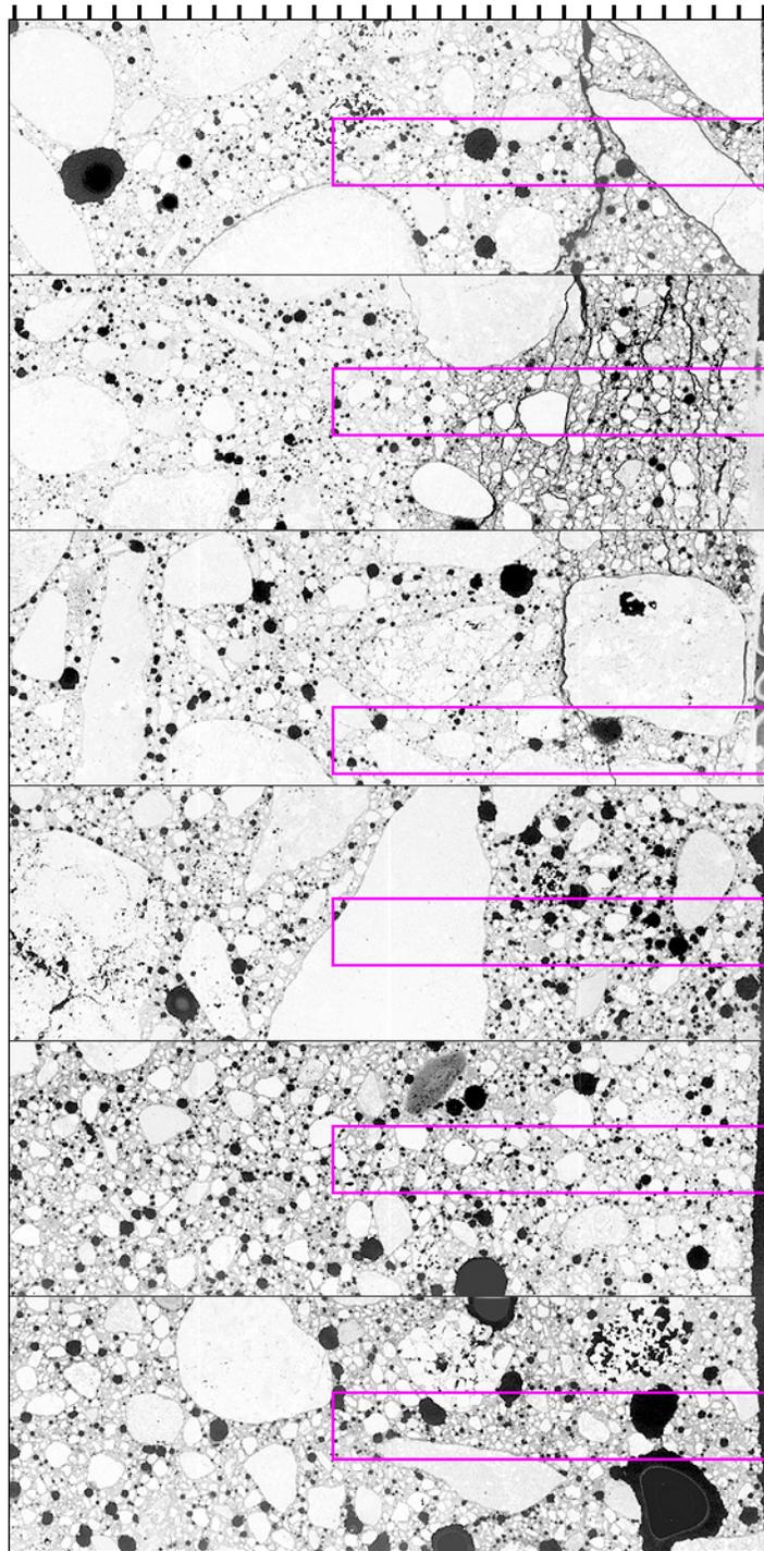
**Figure 5.80. Epifluorescent thin section views of the 0.45 w/c concrete specimens immersed in solution for 500 days, exterior surfaces to the right. From top to bottom: CaCl<sub>2</sub>, MgCl<sub>2</sub>, MBAP, NaCl, CMA, and limewater, tic marks every mm. Pink boxes highlight close-up regions shown in Figure 5.81.**
