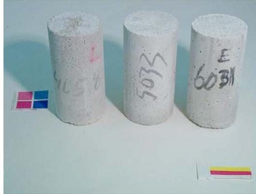
Figure 5.5. Control cylinders exposed to limewater solution after 84 days of constant low temperature test. From left to right: 0.40, 0.50, and 0.60 w/c mortar cylinders.
