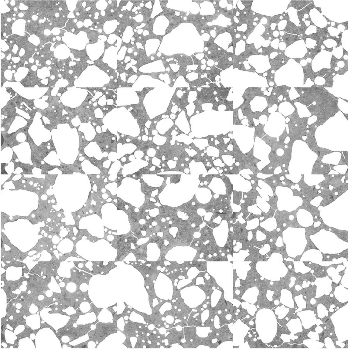
**Figure 4.12. Mosaic of 12 frames collected from thin section prepared from billet cut from top portion of core SD-1 after masking out air voids, fine aggregate, and micro-cracks to isolate cement paste (each individual frame measures 2.612 x 1.959 mm).**
