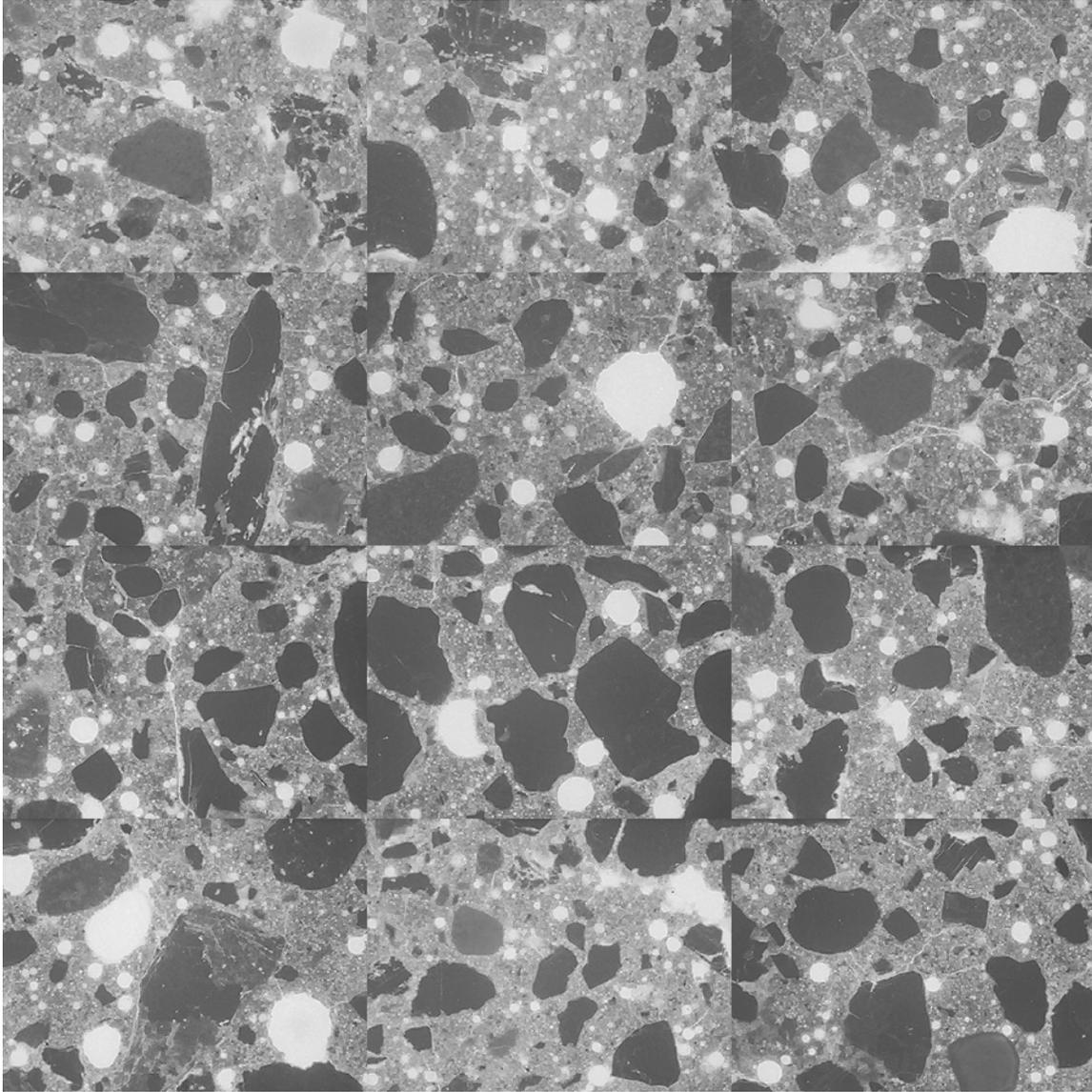
**Figure 4.13. Mosaic of 12 frames collected from thin section prepared from a second billet cut from top portion of core SD-1 (each individual frame measures 2.612 x 1.959 mm). These frames were not masked and used for *w/c* determination, but recorded as visual check against the first section prepared from core SD-1.**
