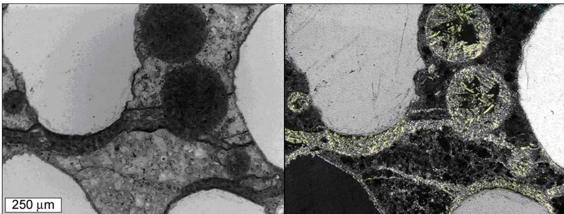
**Figure 5.9. Cracks and air voids filled with remnant calcium oxychloride crystals in  $CaCl_2$  solution immersed sample. From left to right, epifluorescent and crossed polars.**
