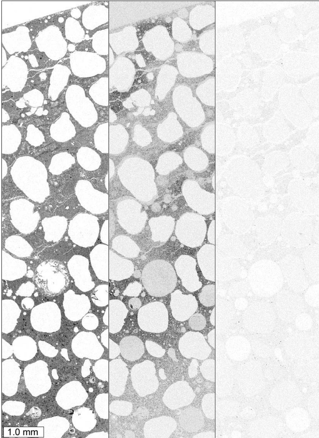
**Figure 5.18. Elemental maps, from left to right: calcium, chloride, and magnesium. The elemental maps were collected from a thin section prepared from a cylinder immersed in calcium chloride solution. Darker areas indicate a higher concentration.**
