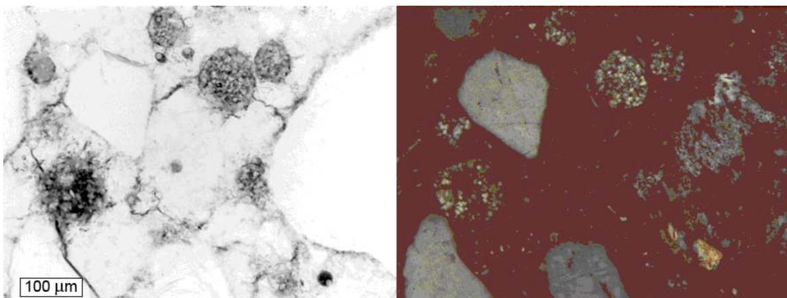
**Figure 5.103. Deteriorated 0.45 w/cm GGBFS concrete exposed to  $MgCl_2$  brine with blocky  $Ca(OH)_2$  crystals in air voids. From left to right: epifluorescent and crossed polars.**
