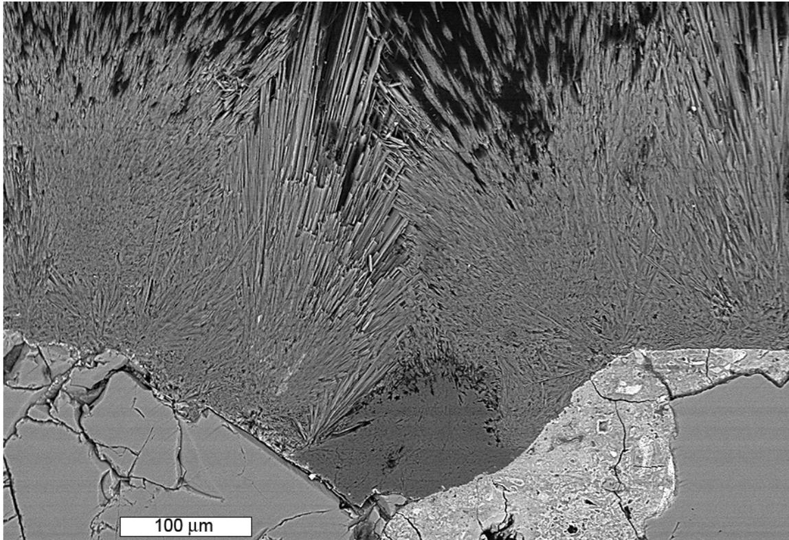
**Figure 5.111. BSE image of magnesium chloride hydroxide hydrate (lighter) and brucite (darker) crystals at surface of 0.45 w/c concrete specimen exposed to  $MgCl_2$  brine.**
