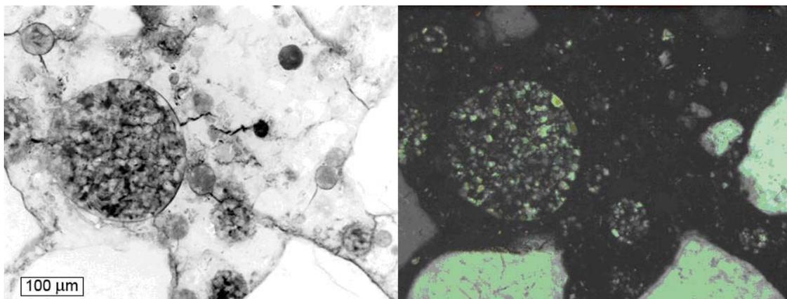
**Figure 5.94. Deteriorated portion from 0.45 w/cm fly ash concrete exposed to  $\text{CaCl}_2$  brine with blocky  $\text{Ca(OH)}_2$  crystals.
