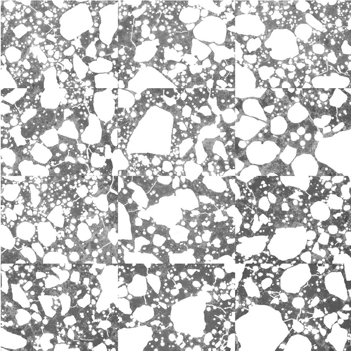
**Figure 4.20. Mosaic of 12 frames collected from thin section prepared from billet cut from top portion of core SD-5 after masking out air voids, fine aggregate, and micro-cracks to isolate cement paste (each individual frame measures 2.612 x 1.959 mm).**
