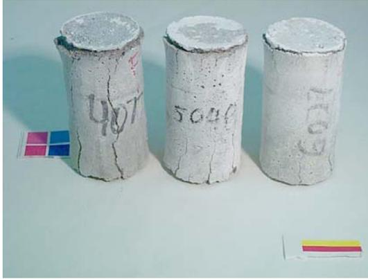
Figure 5.3. Cylinders exposed to  $\text{CaCl}_2$  solution after 84 days of constant low temperature test. From left to right: 0.40, 0.50, and 0.60 w/c mortar cylinders.
