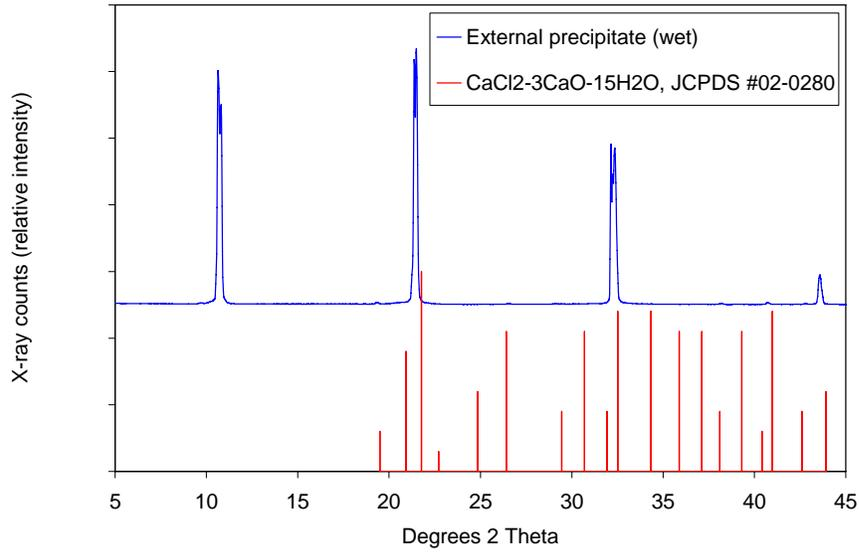
**Figure 5.67.** XRD pattern from the wet precipitate collected from the exterior of concrete exposed to  $\text{CaCl}_2$  brine for 500 days compared to  $3\text{CaO}\cdot\text{CaCl}_2\cdot 15\text{H}_2\text{O}$  reference peaks.
