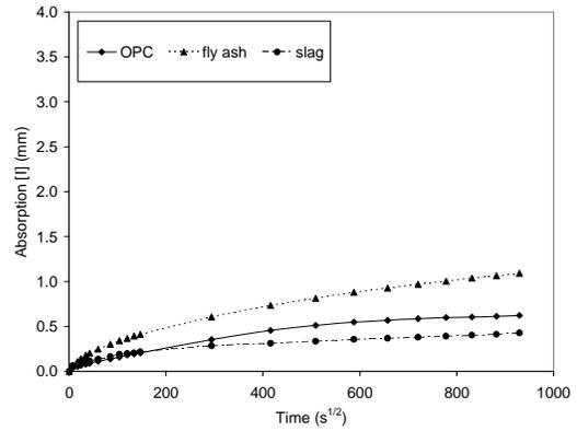
Figure 5.43. Sorptivity - concrete  $w/cm$  - 0.45 -  $CaCl_2$
