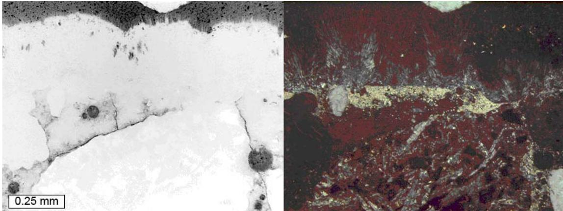
**Figure 5.104. Fibrous crystals at surface of 0.45 w/c straight portland cement concrete exposed to  $MgCl_2$  brine.**
