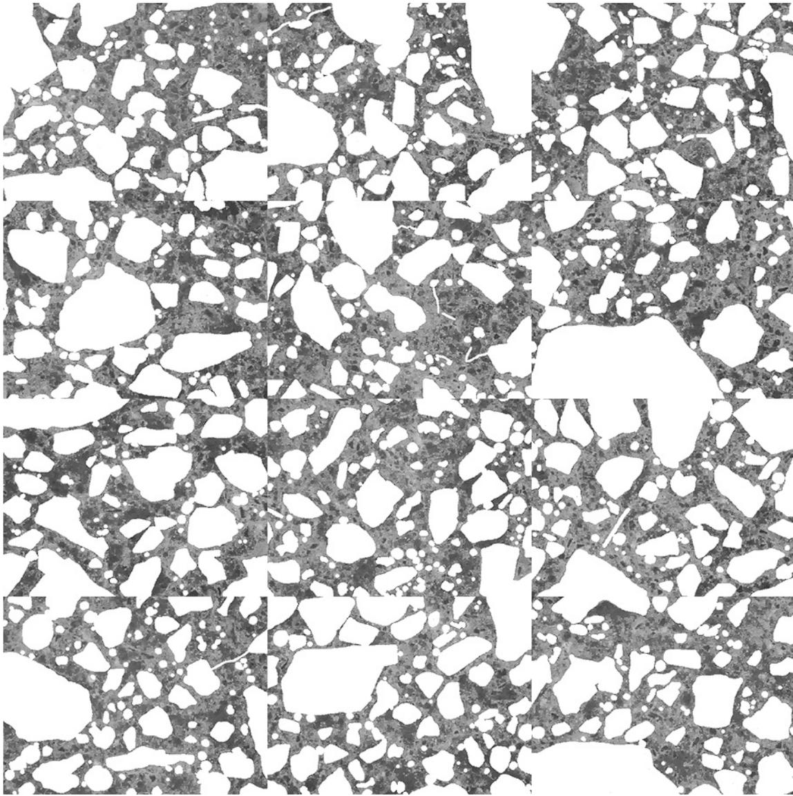
**Figure 4.34. Mosaic of 12 frames collected from thin section prepared from billet cut from top portion of core T-2 after masking out air voids, fine aggregate, and micro-cracks to isolate cement paste (each individual frame measures 2.612 x 1.959 mm).**
