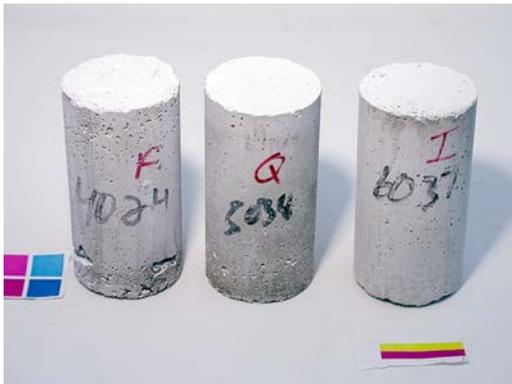
**Figure 5.27. Cylinders exposed to 10%  $\text{CaCl}_2$  solution after 56 days of constant low temperature test.**
