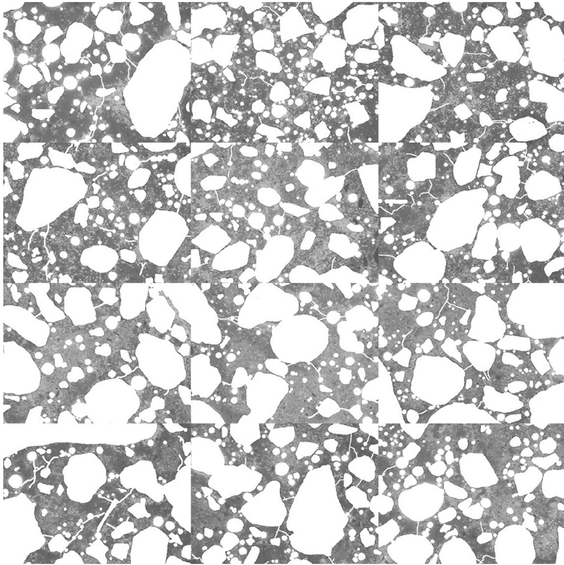
**Figure 4.17. Mosaic of 12 frames collected from thin section prepared from billet cut from top portion of core SD-4 after masking out air voids, fine aggregate, and micro-cracks to isolate cement paste (each individual frame measures 2.612 x 1.959 mm).**
