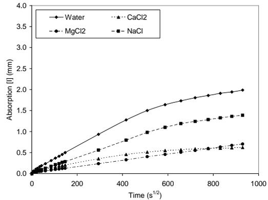
**Figure 5.37. Sorptivity of portland cement concrete - w/c - 0.45**
