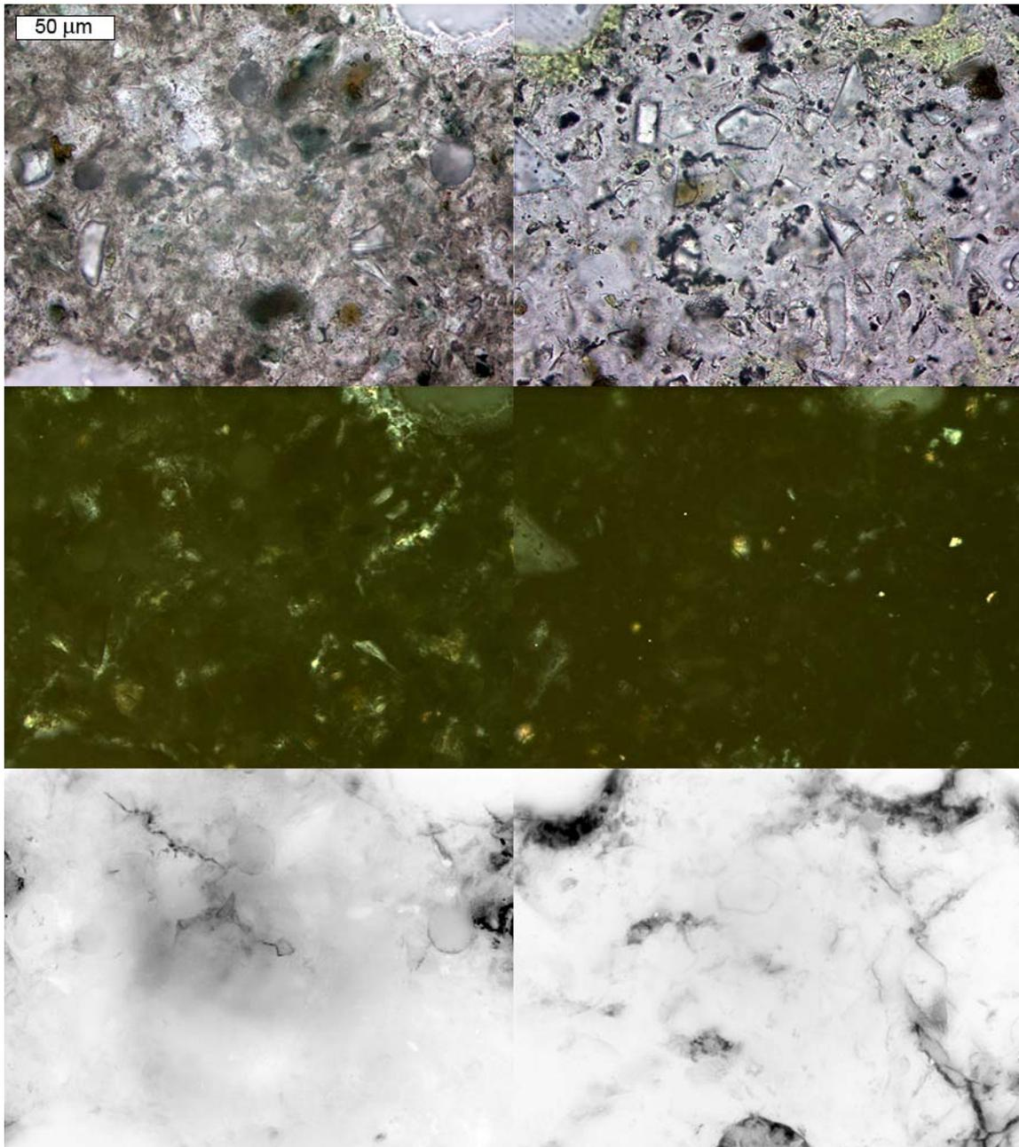
**Figure 5.100. Regions of cement paste in 0.45 w/cm GGBFS concrete exposed to MgCl<sub>2</sub> brine where Ca(OH)<sub>2</sub> is depleted, (right) and still present, (left). From top to bottom: transmitted light, crossed polars, and epifluorescent mode images.**
