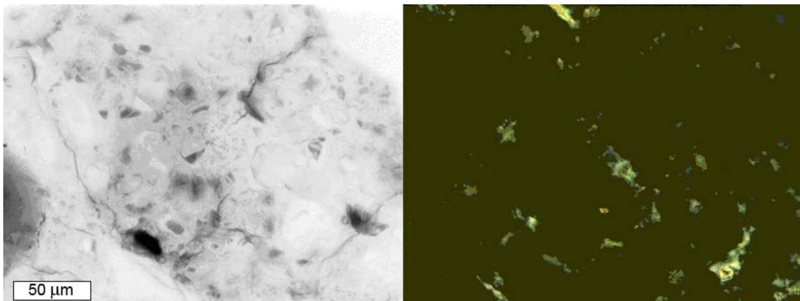
**Figure 5.106. Cement paste just below surface, 0.45 w/c straight portland cement concrete, silane-sealed, exposed to  $MgCl_2$  brine.**
