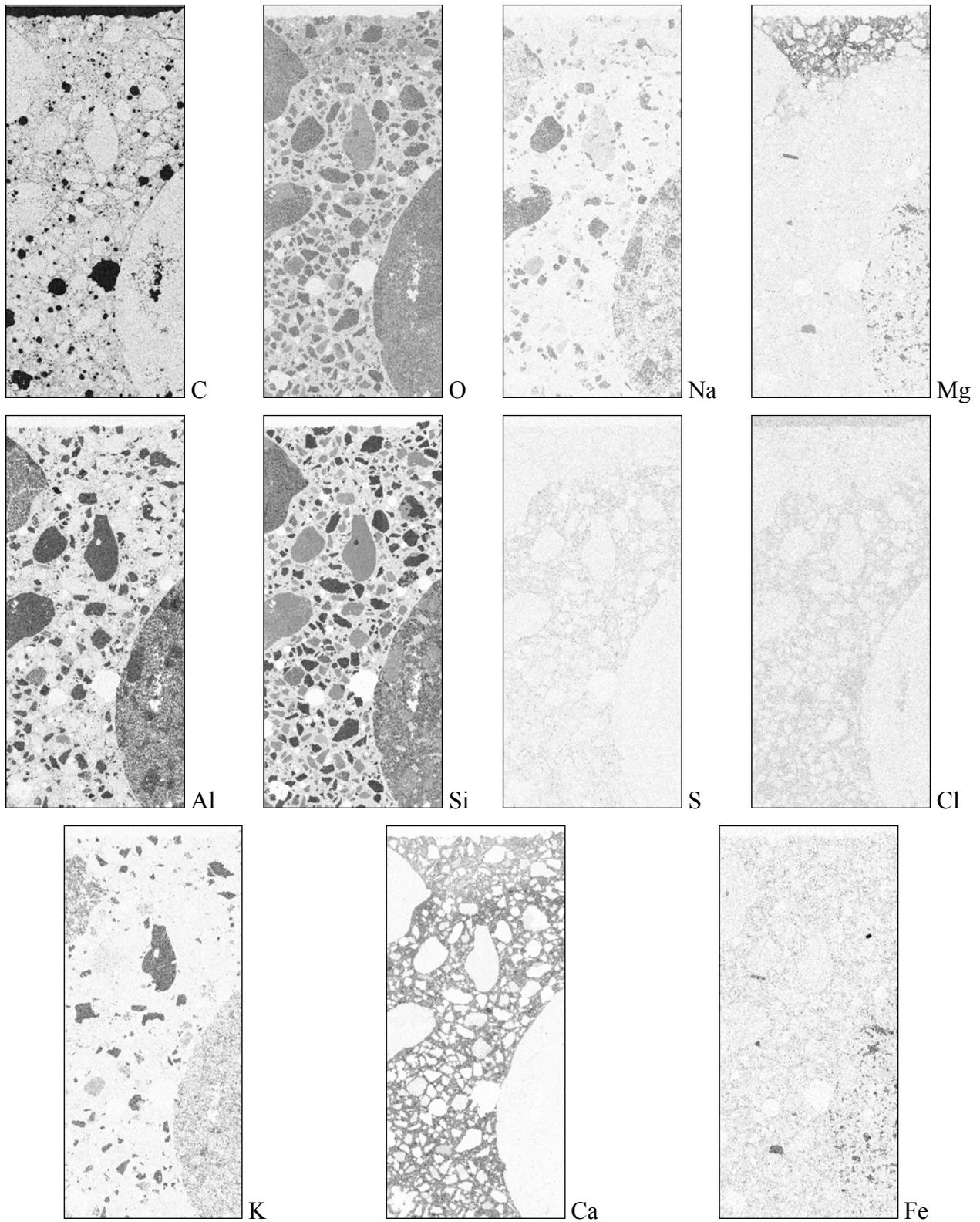
Figure 4.40. Elemental maps from pavement surface, darker regions indicate higher concentrations.
