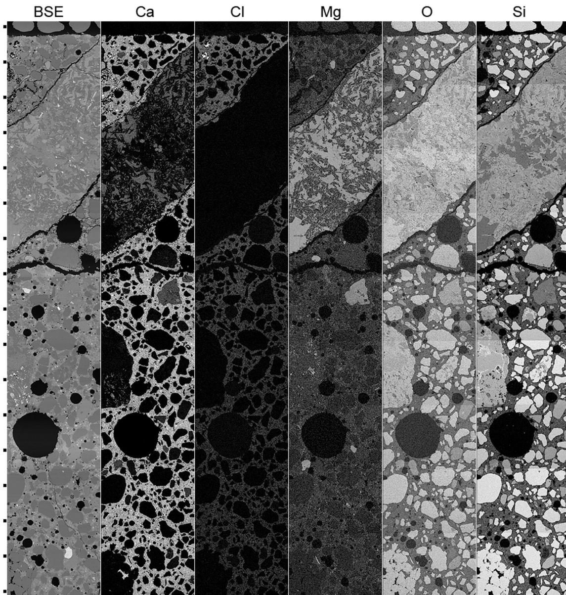
**Figure 5.108. Elemental maps collected from 0.45 w/c concrete specimen immersed in  $\text{CaCl}_2$  brine at 500 days. Brighter regions correspond to higher counts for characteristic elemental X-rays.**
