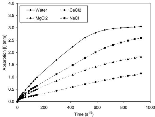
**Figure 5.36. Sorptivity of portland cement concrete - w/c - 0.55**
