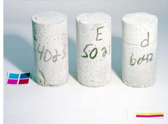
Figure 5.4. Cylinders exposed to CMA solution after 84 days of constant low temperature test. From left to right: 0.40, 0.50, and 0.60 w/c mortar cylinders.
