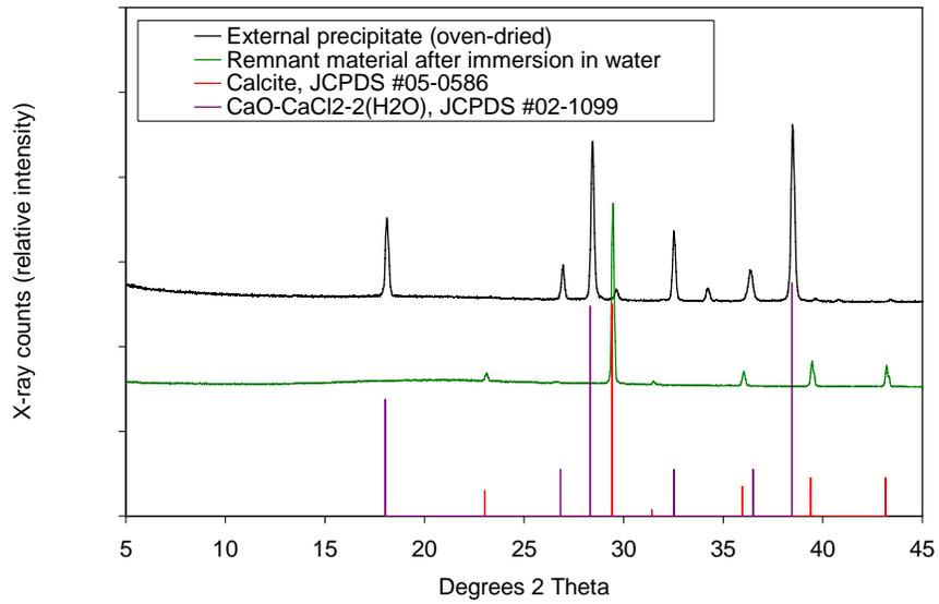
**Figure 5.71. XRD patterns from oven-dried external precipitate crystals, and the resultant remnant material after immersion in room temperature water, as compared to a reference patterns for calcite and  $\text{CaCl}_2 \cdot \text{Ca}(\text{OH})_2 \cdot 2\text{H}_2\text{O}$ .**
