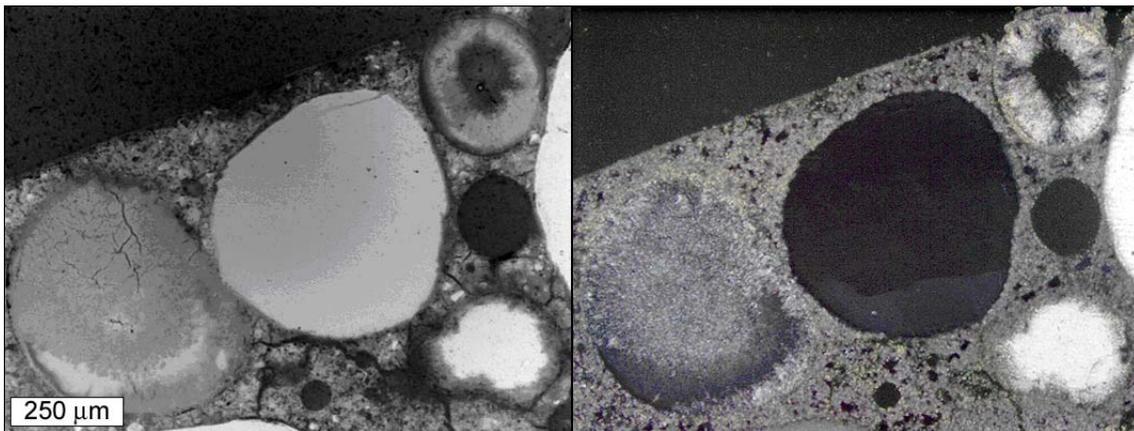
**Figure 5.13. Magnesium chloride hydrate crystals in air voids near exterior in thin section prepared from cylinder immersed in  $MgCl_2$  solution.
