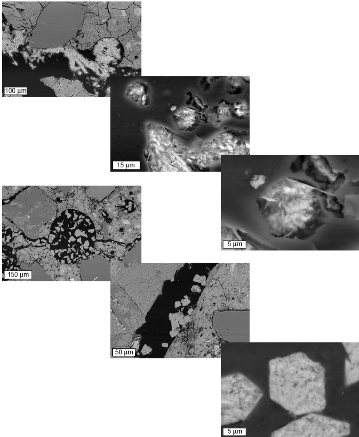
**Figure 5.112. BSE images comparing bladed crystals observed near the top of the specimen exposed to  $\text{CaCl}_2$  brine, (upper images) to secondary blocky calcium hydroxide crystals observed at depth (lower images).**
