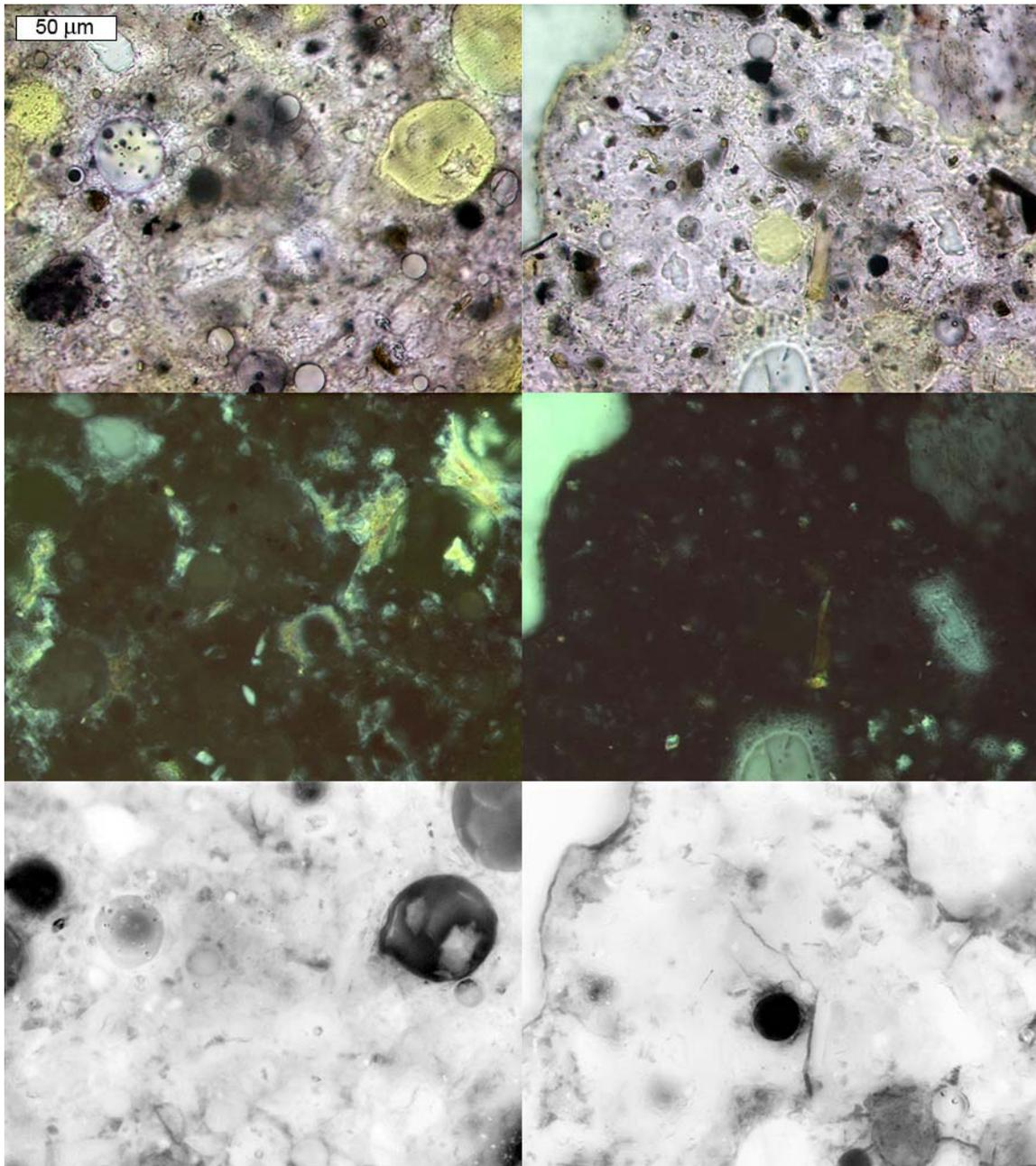
**Figure 5.91. Regions of cement paste in 0.45 *w/cm* fly ash concrete exposed to  $\text{CaCl}_2$  brine where  $\text{Ca(OH)}_2$  is depleted, (right) and still present, (left).
