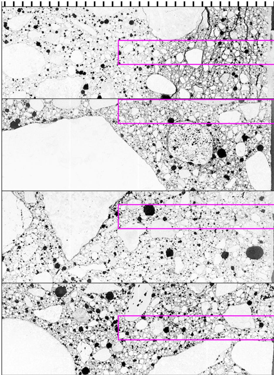
Figure 5.96. Epifluorescent thin section views of 0.45 *w/cm* concrete specimens, and a 0.55 *w/c* concrete silane-sealed specimen, all immersed in  $MgCl_2$  solution for 500 days, exterior surfaces to the right.
