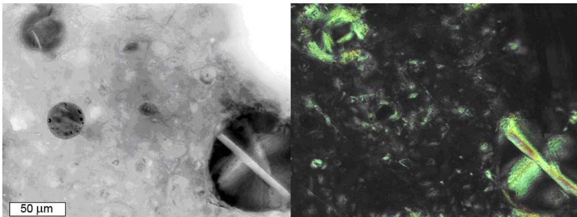
**Figure 5.87.** Cement paste just below the surface from 0.45 w/c straight portland cement concrete exposed to limewater.  $\text{Ca}(\text{OH})_2$  deposits in air voids. From left to right: epifluorescent and crossed polars.
