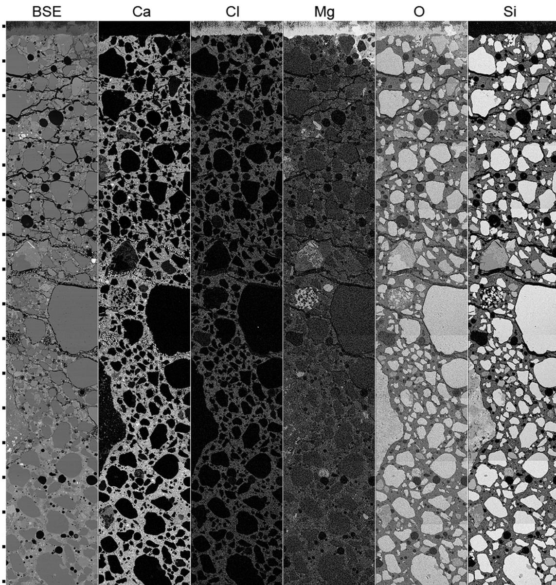
**Figure 5.109. Elemental maps collected from 0.45 w/c concrete specimen immersed in  $MgCl_2$  brine at 500 days. Brighter regions correspond to higher counts for characteristic elemental X-rays.**
