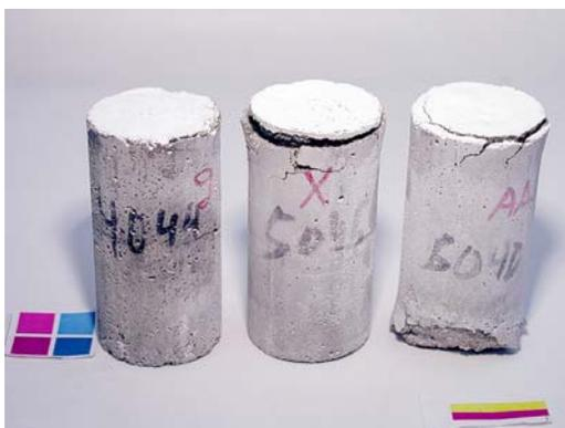
**Figure 5.29. Cylinders exposed to 17%  $\text{CaCl}_2$  solution after 56 days of constant low temperature test. From left to right: 0.40, 0.50, and 0.60 w/c.**
