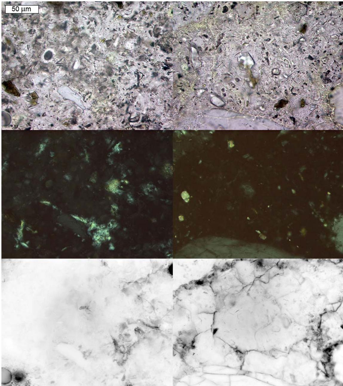
**Figure 5.92. Regions of cement paste in 0.45 *w/cm* GGBFS concrete exposed to  $\text{CaCl}_2$  brine where  $\text{Ca(OH)}_2$  is depleted, (right) and still present, (left). From top to bottom: transmitted light, crossed polars, and epifluorescent mode images.**
