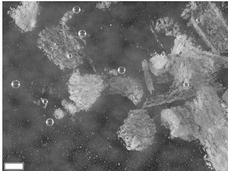
**Figure 5.72. Fresh calcium oxochloride crystals before, (top) and after immersion in a sealed container of hot  $\text{CaCl}_2$  brine. (Bottom) scale bar = 1 mm.**
