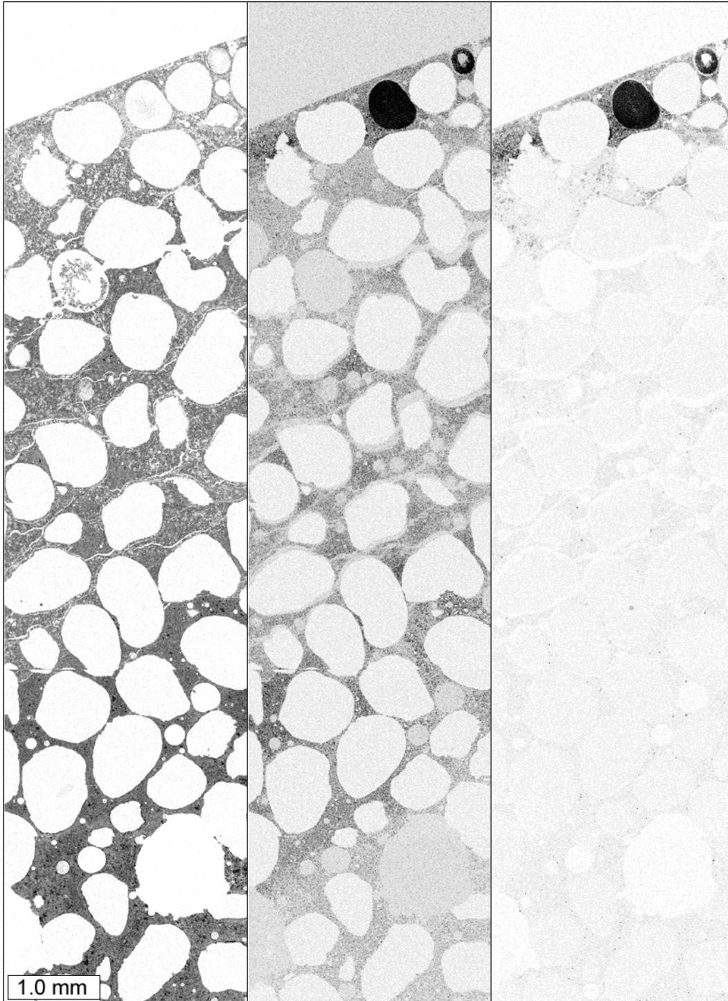
**Figure 5.16. Elemental maps, from left to right: calcium, chlorine, and magnesium. The elemental maps were collected from a thin section prepared from a cylinder immersed in magnesium chloride solution. Darker areas indicate a higher concentration.**
