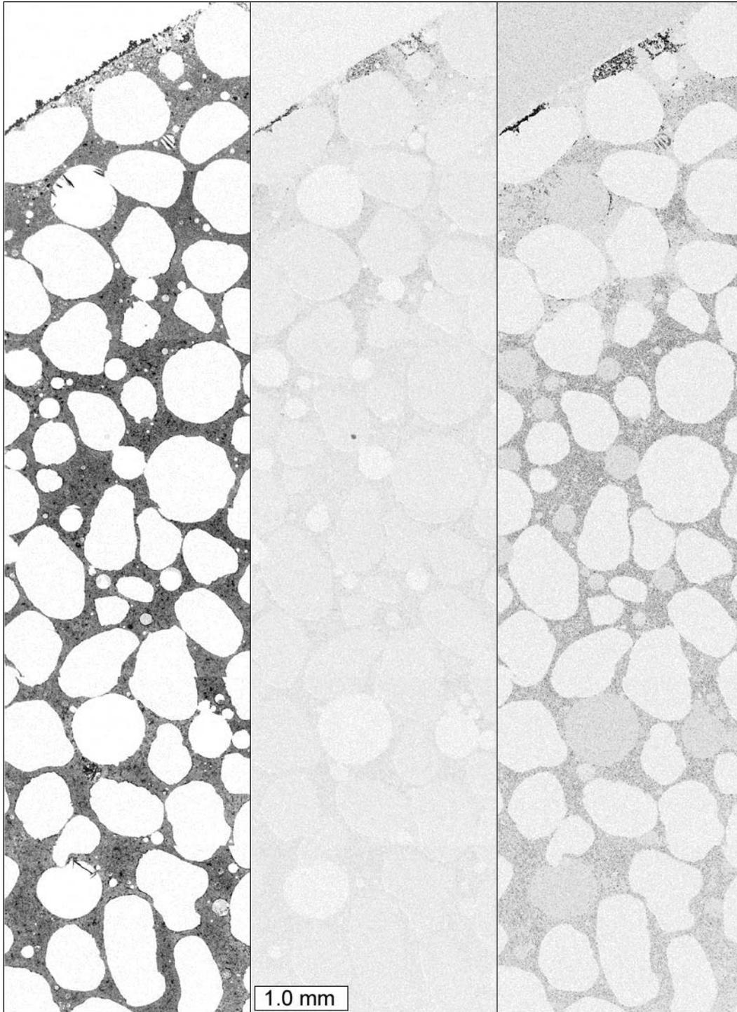
**Figure 5.20. Elemental maps, from left to right: calcium, sodium, and chlorine. The elemental maps were collected from a thin section prepared from a cylinder immersed in sodium chloride solution. Darker areas indicate a higher concentration.**
