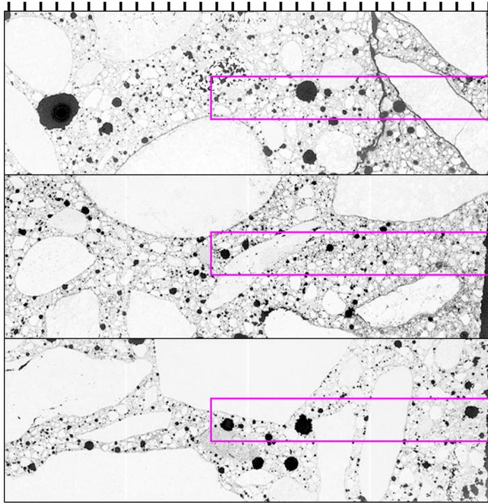
**Figure 5.88. Epifluorescent thin section views of the 0.45 *w/cm* concrete specimens immersed in  $\text{CaCl}_2$  solution for 500 days, exterior surfaces to the right. From top to bottom: straight portland cement concrete, supplementary fly ash concrete, and supplementary GGBFS concrete, tic marks every mm. Pink boxes highlight close-up regions shown in Figure 5.89.**
