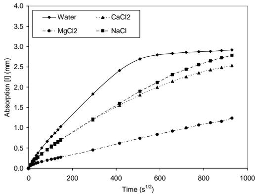
Figure 5.38. Sorptivity - fly ash concrete -  $w/cm$  - 0.55
