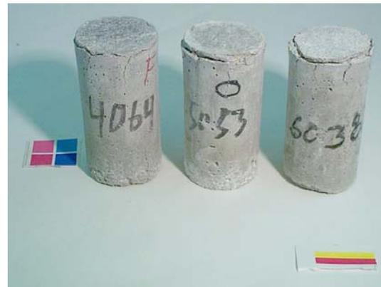
Figure 5.2. Cylinders exposed to MgCl<sub>2</sub> solution after 84 days of constant low temperature test. From left to right: 0.40, 0.50, and 0.60 w/c mortar cylinders.
