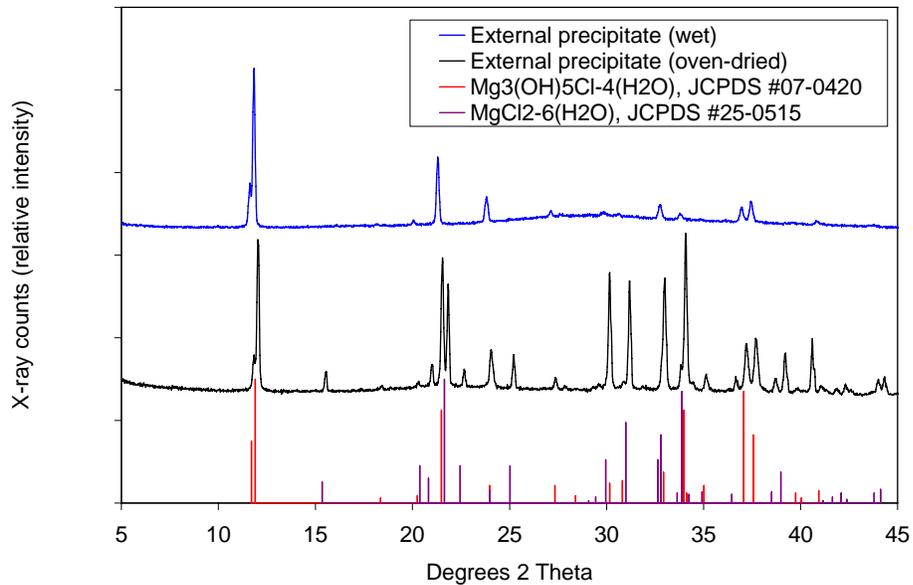
**Figure 5.76. XRD patterns from the wet and oven dried external precipitate collected from concrete exposed to  $\text{MgCl}_2$  brine for 500 days, with reference patterns for  $\text{Mg}_3(\text{OH})_5\text{Cl}\cdot 4\text{H}_2\text{O}$  and  $\text{MgCl}_2\cdot 6\text{H}_2\text{O}$ .**
