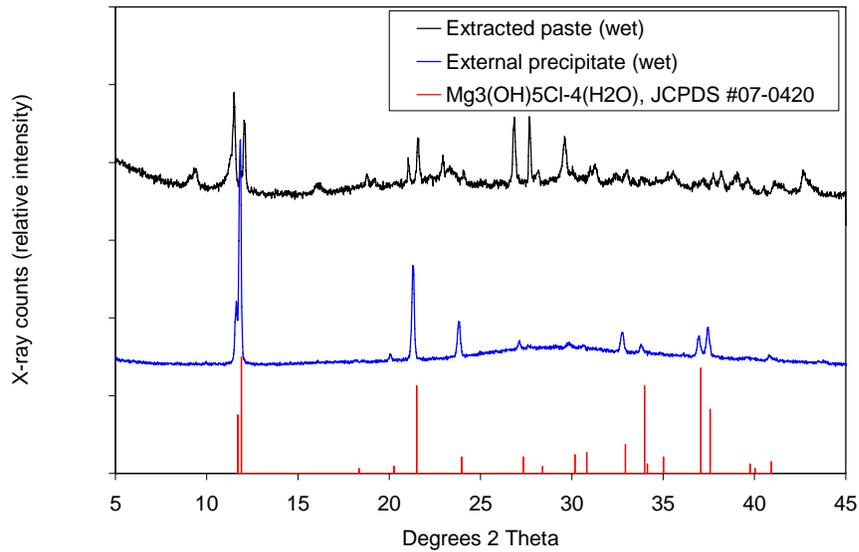
**Figure 5.75. XRD patterns from the wet extracted paste and wet external precipitate collected from concrete exposed to  $\text{MgCl}_2$  brine for 500 days, with reference pattern for  $\text{Mg}_3(\text{OH})_5\text{Cl}\cdot 4\text{H}_2\text{O}$ .**
