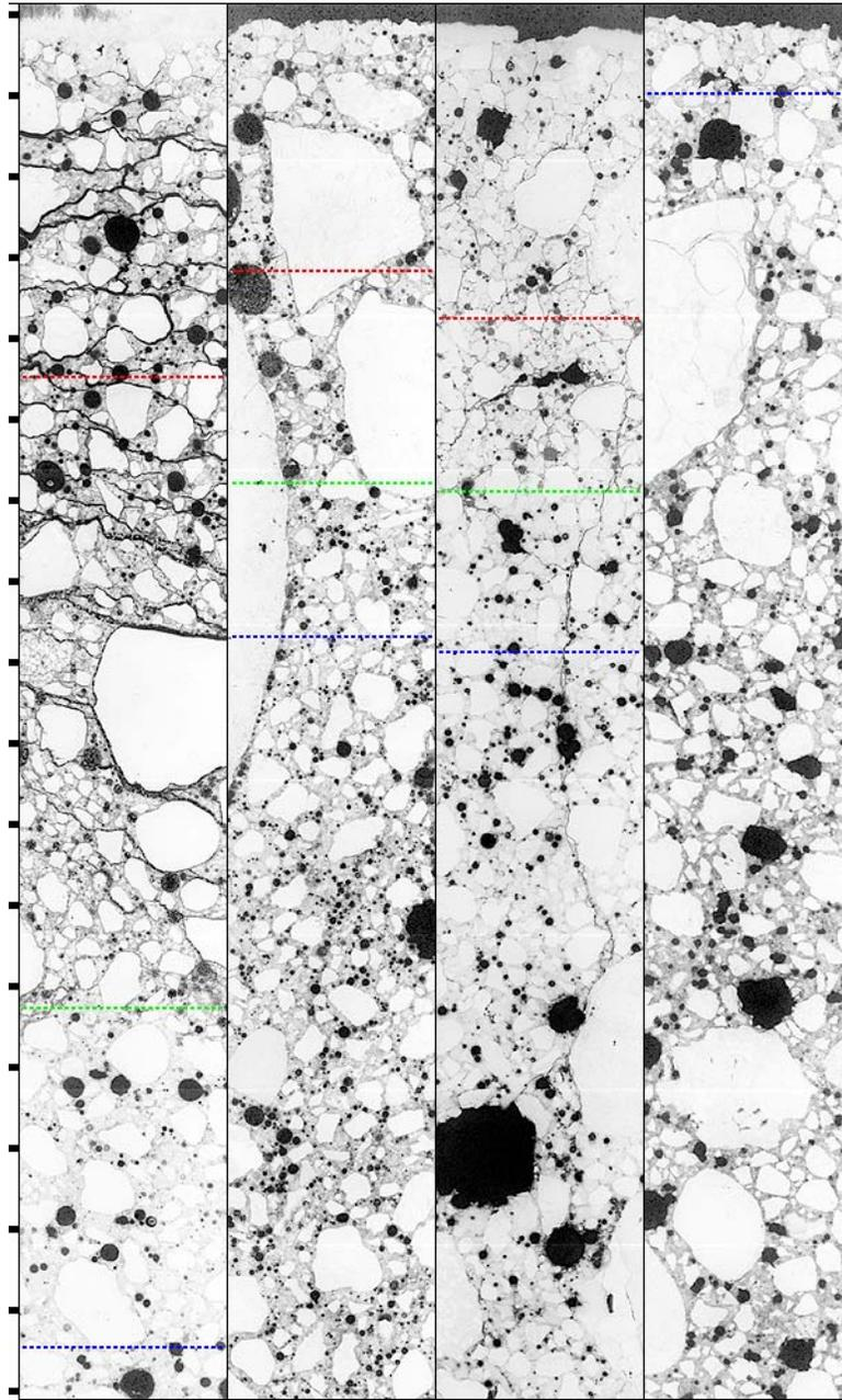
**Figure 5.97. Close-up views of regions outlined in pink in Figure 5.96, but with exterior surfaces oriented towards the top. Cross-sectional epifluorescent mode images of 0.45 w/cm concrete specimens, and a 0.55 w/c concrete specimen after 500 days of immersion in  $MgCl_2$  solution.**
