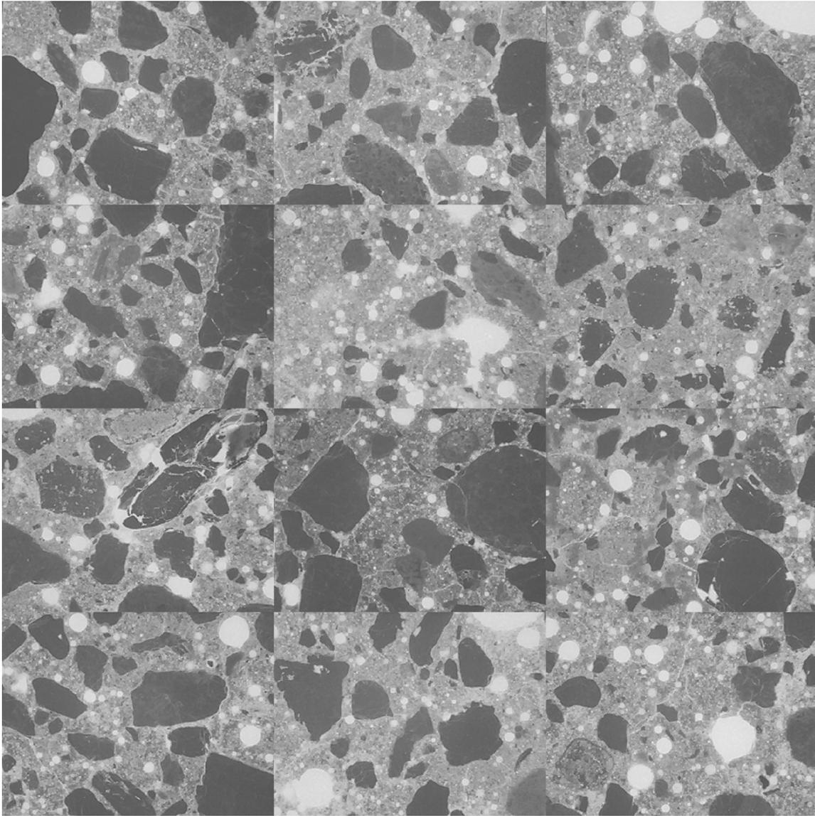
**Figure 4.18. Mosaic of 12 frames collected from thin section prepared from a second billet cut from top portion of core SD-4 (each individual frame measures 2.612 x 1.959 mm). These frames were not masked and used for *w/c* determination, but recorded as visual check against the first section prepared from core SD-4.**
