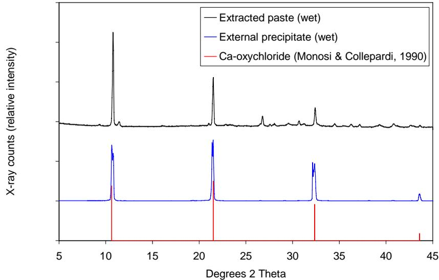
**Figure 5.66. XRD patterns from the wet extracted paste and the wet exterior precipitate collected from concrete exposed to  $CaCl_2$  brine for 500 days compared to the reference 8.34, 4.13, 2.76 angstrom peaks for Monosi and Collepardi's calcium oxychloride phase.**
