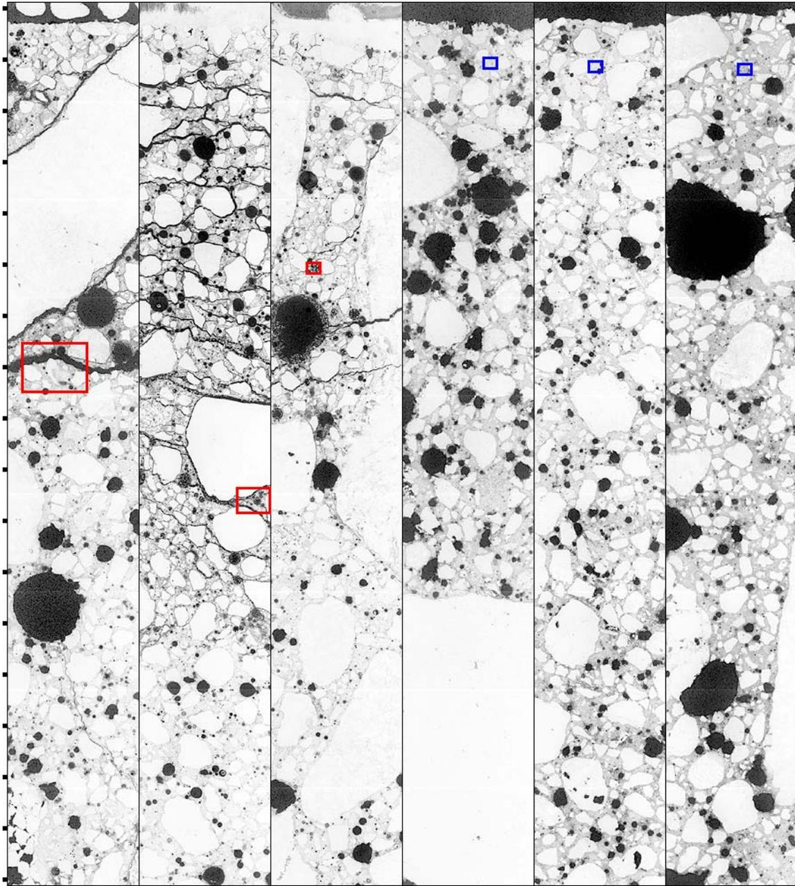
**Figure 5.81. Close-up views of regions outlined in pink in Figure 5.183, but with exterior surfaces oriented towards the top. Cross-sectional epifluorescent mode images of the 0.45 w/c concrete specimens after 500 days of immersion in solution.**
