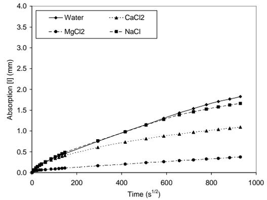
Figure 5.39. Sorptivity - fly ash concrete -  $w/cm$  - 0.45
