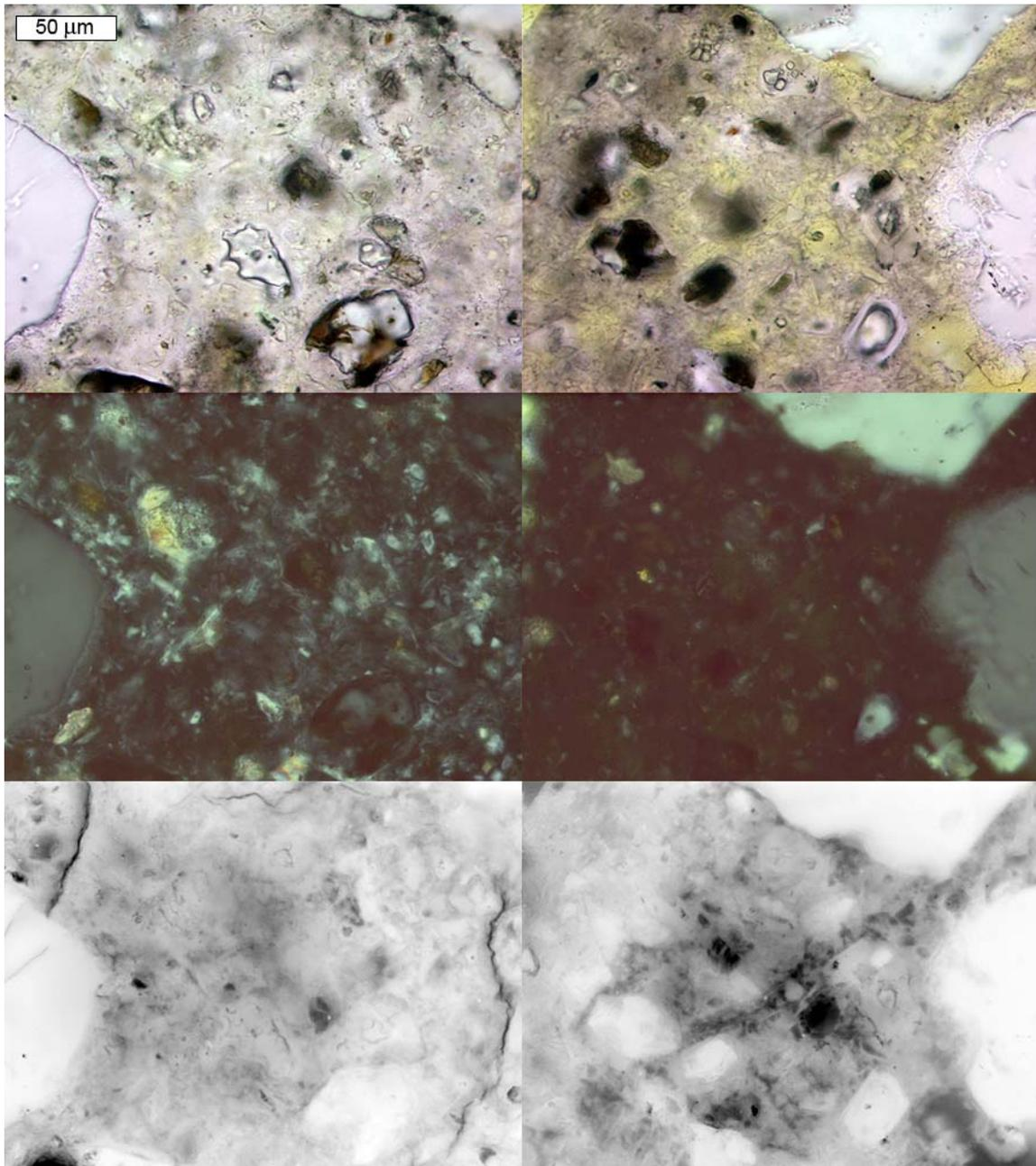
**Figure 5.90. Regions of cement paste in 0.45 w/c straight portland cement concrete exposed to  $\text{CaCl}_2$  brine where  $\text{Ca(OH)}_2$  is depleted, (right) and still present, (left). From top to bottom: transmitted light, crossed polars, and epifluorescent mode images.**
