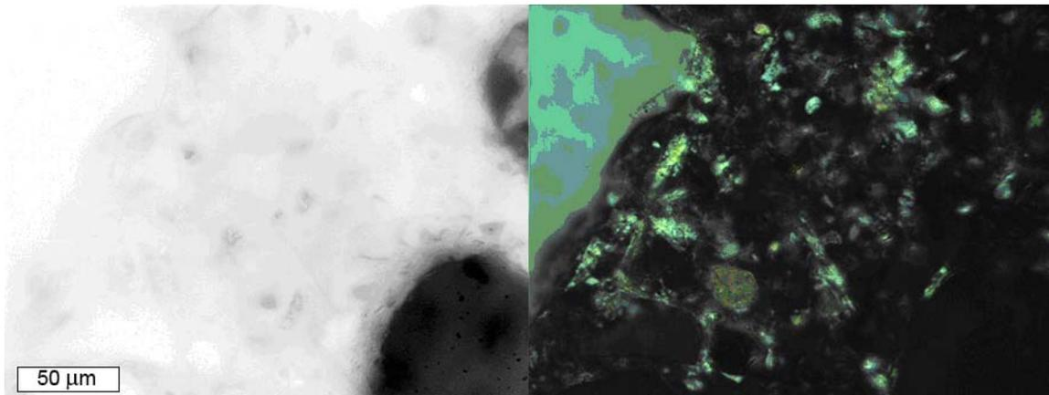
**Figure 5.86.** Cement paste just below the surface from 0.45 w/c straight portland cement concrete exposed to CMA brine. From left to right: epifluorescent and crossed polars.
