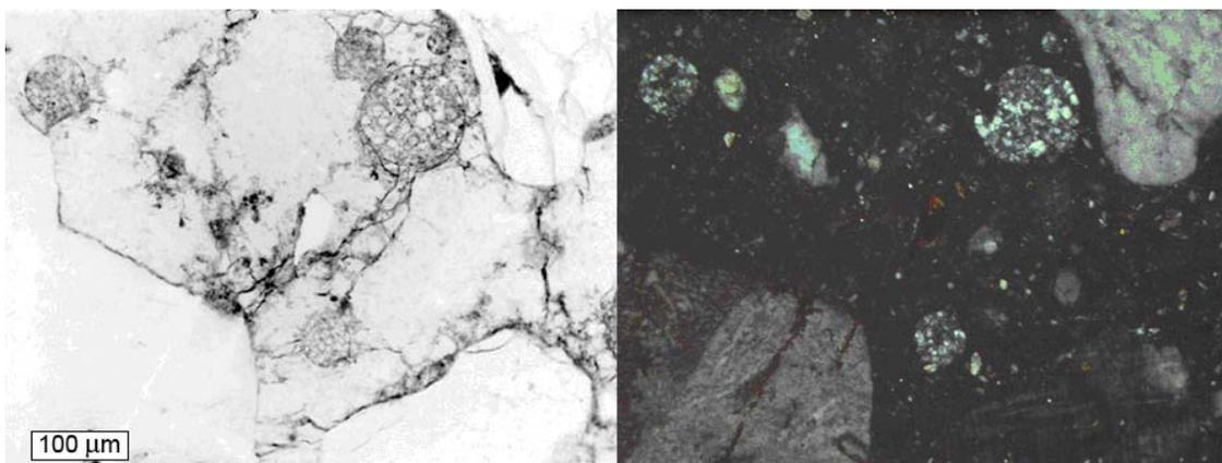
**Figure 5.95. Secondary blocky calcium hydroxide crystals in air voids of 0.45 w/cm GGBFS concrete exposed to  $\text{CaCl}_2$ .
