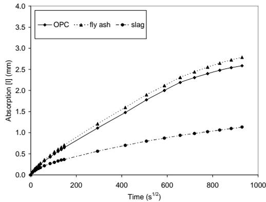
Figure 5.46. Sorptivity - concrete  $w/cm$  - 0.55 -  $NaCl$
