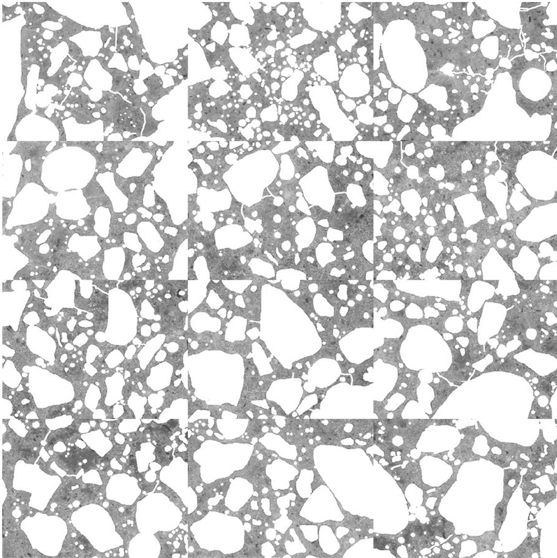
**Figure 4.15. Mosaic of 12 frames collected from thin section prepared from billet cut from top portion of core SD-7 after masking out air voids, fine aggregate, and micro-cracks to isolate cement paste (each individual frame measures 2.612 x 1.959 mm).**
