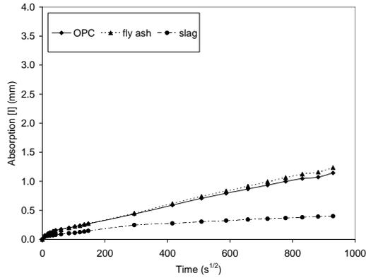
Figure 5.44. Sorptivity - concrete  $w/cm$  - 0.55 -  $MgCl_2$
