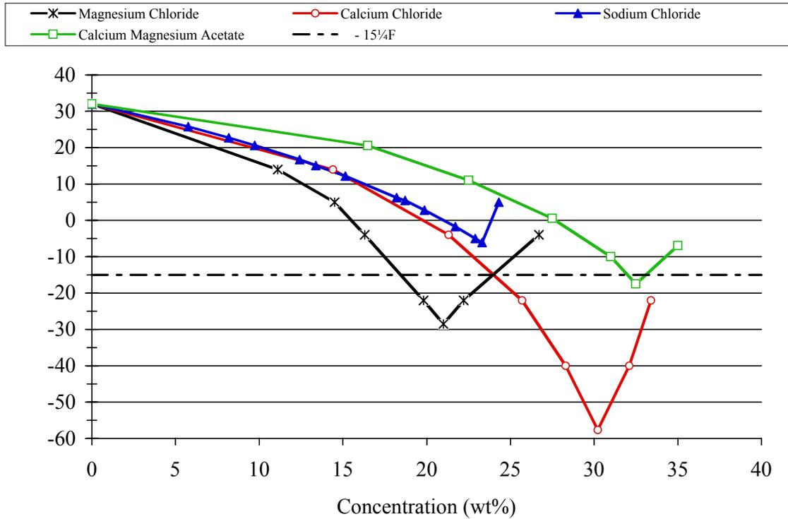
**Figure 3.1. The partial phase diagrams for the deicer solutions tested showing the eutectic points for each solution. The temperature  $-15^{\circ}\text{F}$  [ $-26^{\circ}\text{C}$ ] is shown as a dotted horizontal line.**
