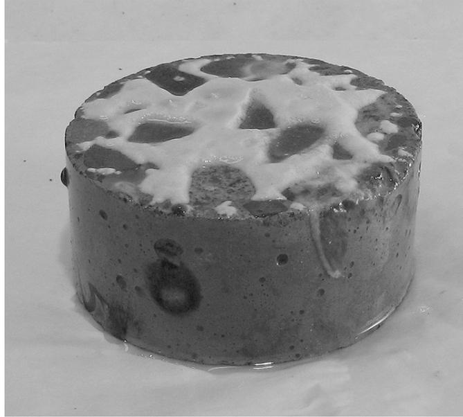
**Figure 5.52. White precipitate on exterior of 4 inch [100 mm] diameter concrete specimen after 500 days immersion in low-concentration CMA solution.**
