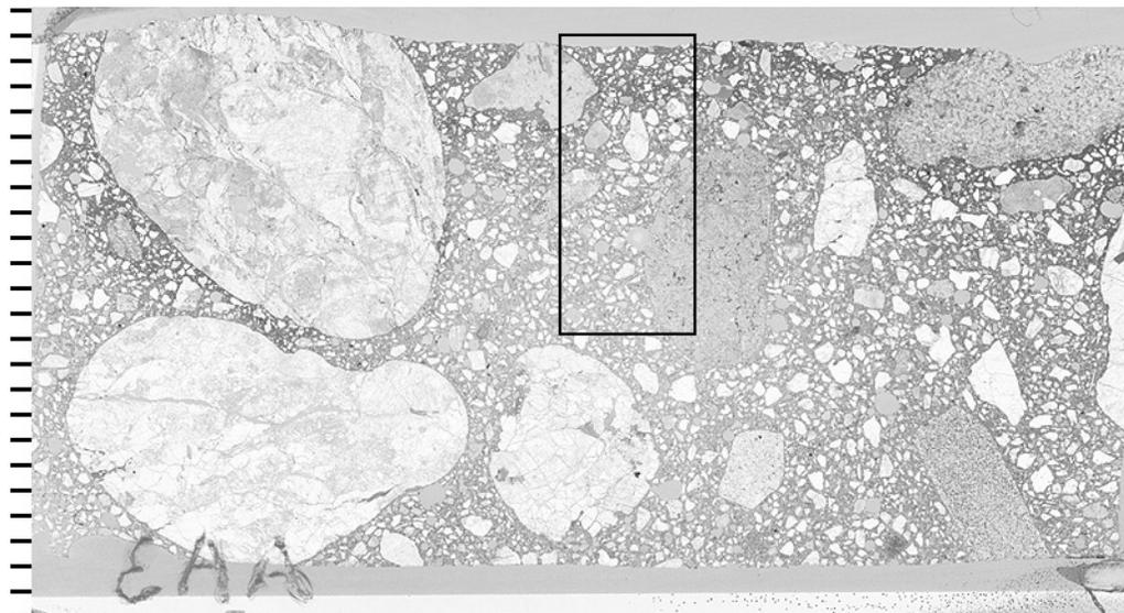
**Figure 4.38. Transmitted light scanned image of thin section to show location of elemental maps shown in Figure 4.40. The top of the thin section represents the wear surface of the pavement, (tic marks every mm).**
