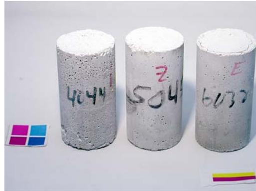
**Figure 5.26. Cylinders exposed to 7%  $\text{CaCl}_2$  solution after 56 days of constant low temperature test.**
