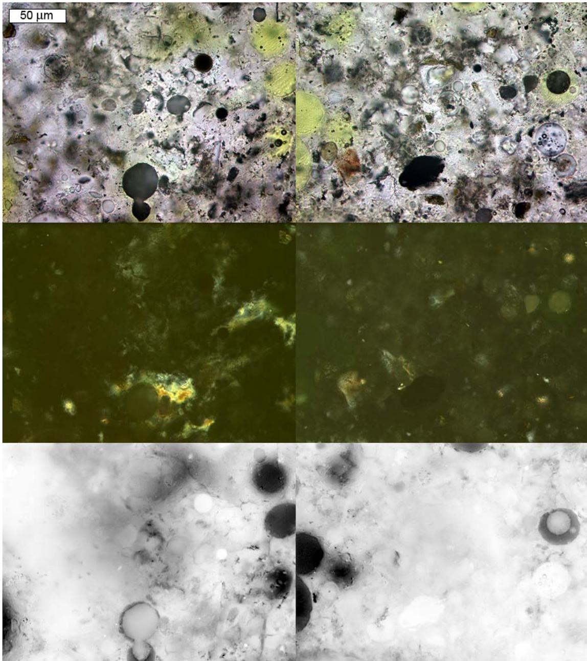
Figure 5.99. Regions of cement paste in 0.45 *w/cm* fly ash concrete exposed to  $\text{MgCl}_2$  brine where  $\text{Ca(OH)}_2$  is depleted, (right) and still present, (left).
