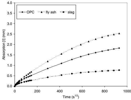
Figure 5.42. Sorptivity - concrete  $w/cm$  - 0.55 -  $CaCl_2$
