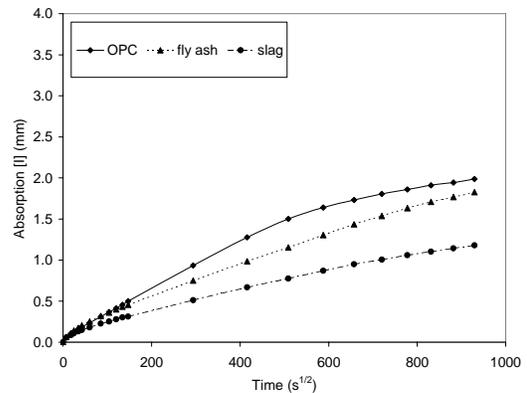
Figure 5.49. Sorptivity - concrete  $w/cm$  - 0.45 - water
