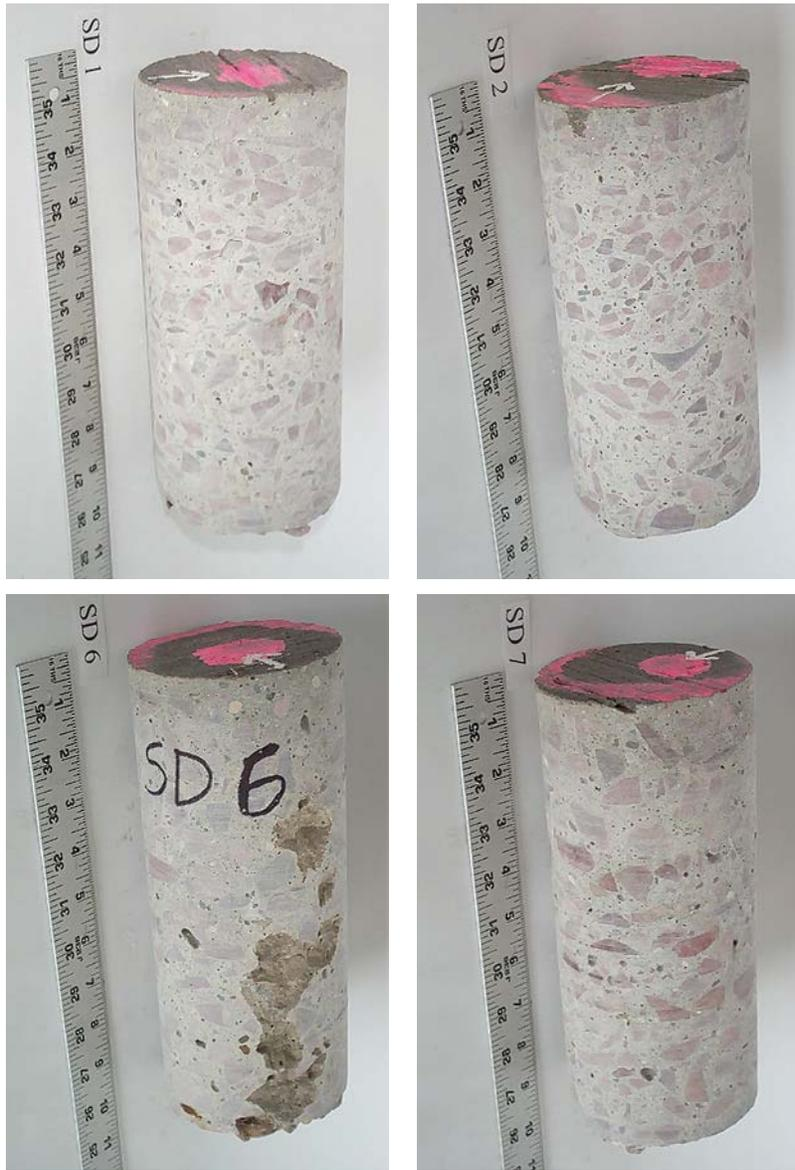
Figure 4.4. Cores taken at joint.
