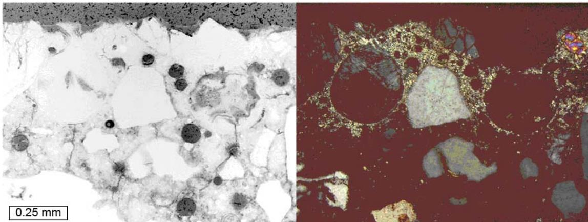
**Figure 5.105. Fibrous crystals in voids near surface of 0.45 w/c straight portland cement concrete exposed to  $MgCl_2$  brine.**
