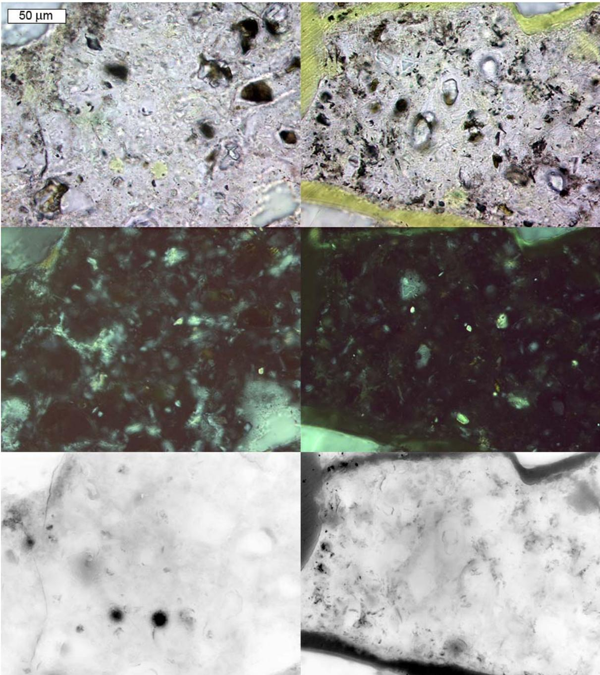
**Figure 5.98. Regions of cement paste in 0.45 w/c straight portland cement concrete exposed to  $MgCl_2$  brine where  $Ca(OH)_2$  is depleted, (right) and still present, (left).
