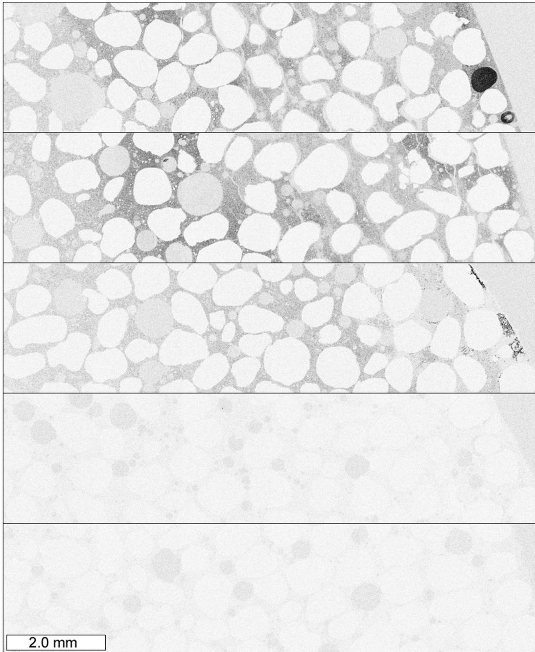
**Figure 5.14. Elemental map for chlorine collected from thin sections prepared from mortar cylinders immersed in chemical solutions.**
