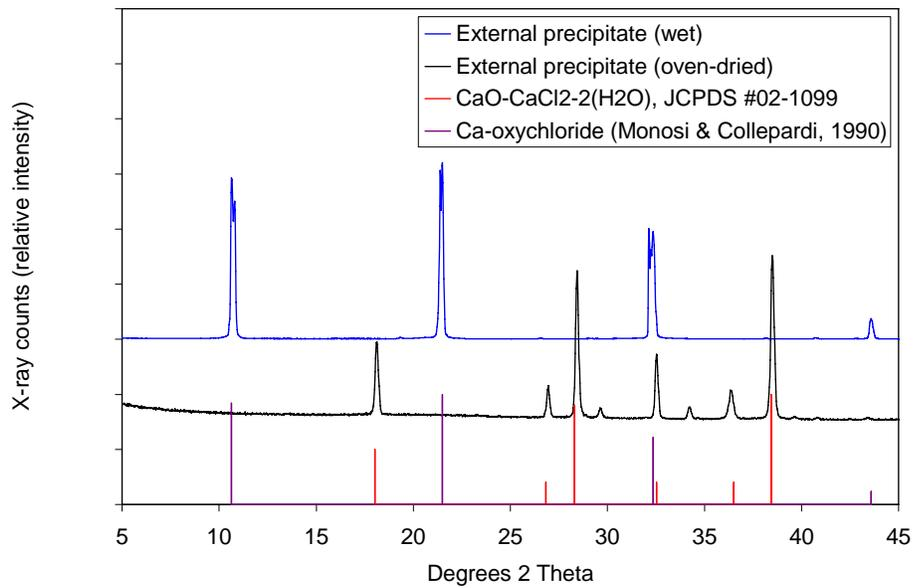
**Figure 5.68.** XRD patterns from the wet and oven-dried external precipitate collected from concrete exposed to  $\text{CaCl}_2$  brine for 500 days compared to reference patterns for calcium oxychloride and  $\text{CaCl}_2\cdot\text{Ca}(\text{OH})_2\cdot 2\text{H}_2\text{O}$ .
