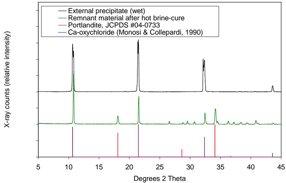
**Figure 5.73. XRD patterns from wet external precipitate, and the resultant remnant material after curing in hot  $\text{CaCl}_2$  brine, with reference patterns for calcium oxychloride and portlandite.**
