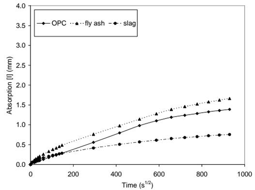
Figure 5.47. Sorptivity - concrete  $w/cm$  - 0.45 -  $NaCl$
