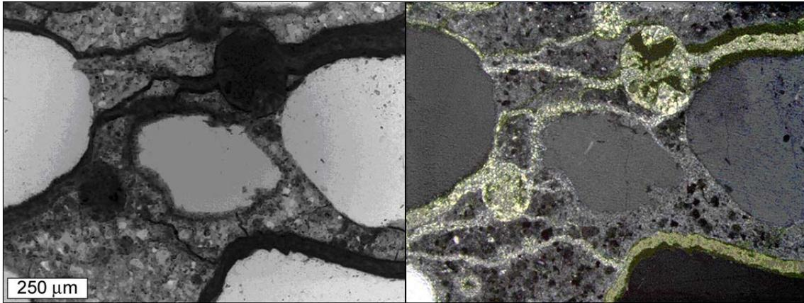
**Figure 5.8. Cracks and air voids filled with remnant calcium oxychloride crystals in  $MgCl_2$  solution immersed sample. From left to right, epifluorescent and crossed polars.**
