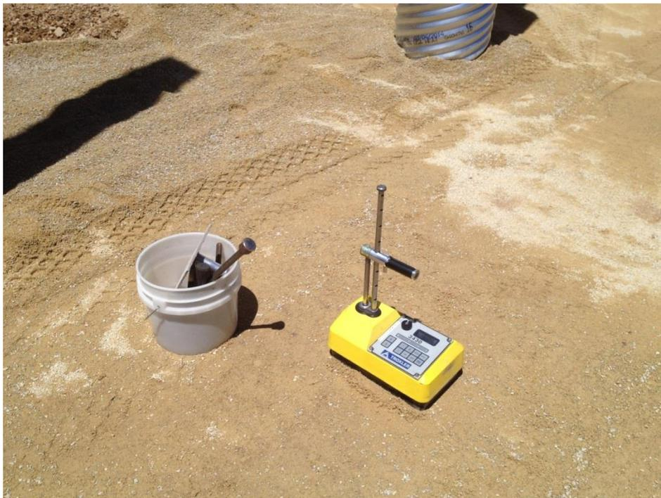
**Figure 3.11: In-place nuclear density gauge test.**
