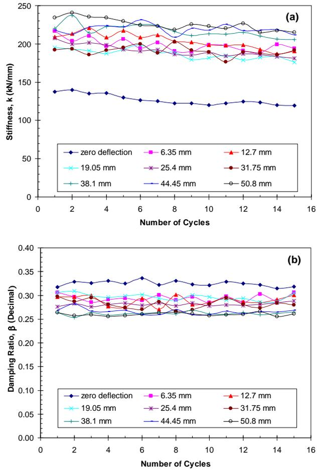
**Fig. 8. Plots of (a) dynamic stiffness and (b) damping ratio as a function of number of cycles at each initial deflection increment for the pile cap with a 0.91-m wide dense gravel zone.**
