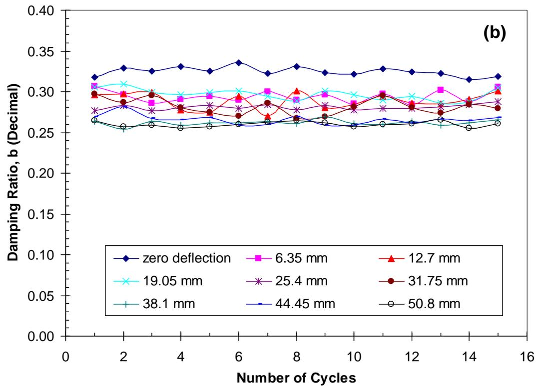
**Fig. 9.** Plots of (a) dynamic stiffness and (b) damping ratio as a function of number of cycles at each initial deflection increment for the pile cap with a 1.82-m wide dense gravel zone.
