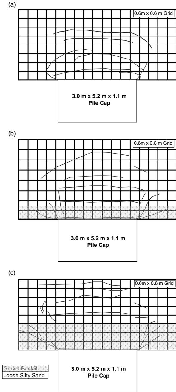
**Fig. 6. Plan view of crack patterns with backfills consisting of (a) loose silty sand, (b) 0.91-m wide dense gravel zone with loose silty sand, and (c) 1.82-m wide dense gravel and loose silty sand.**
