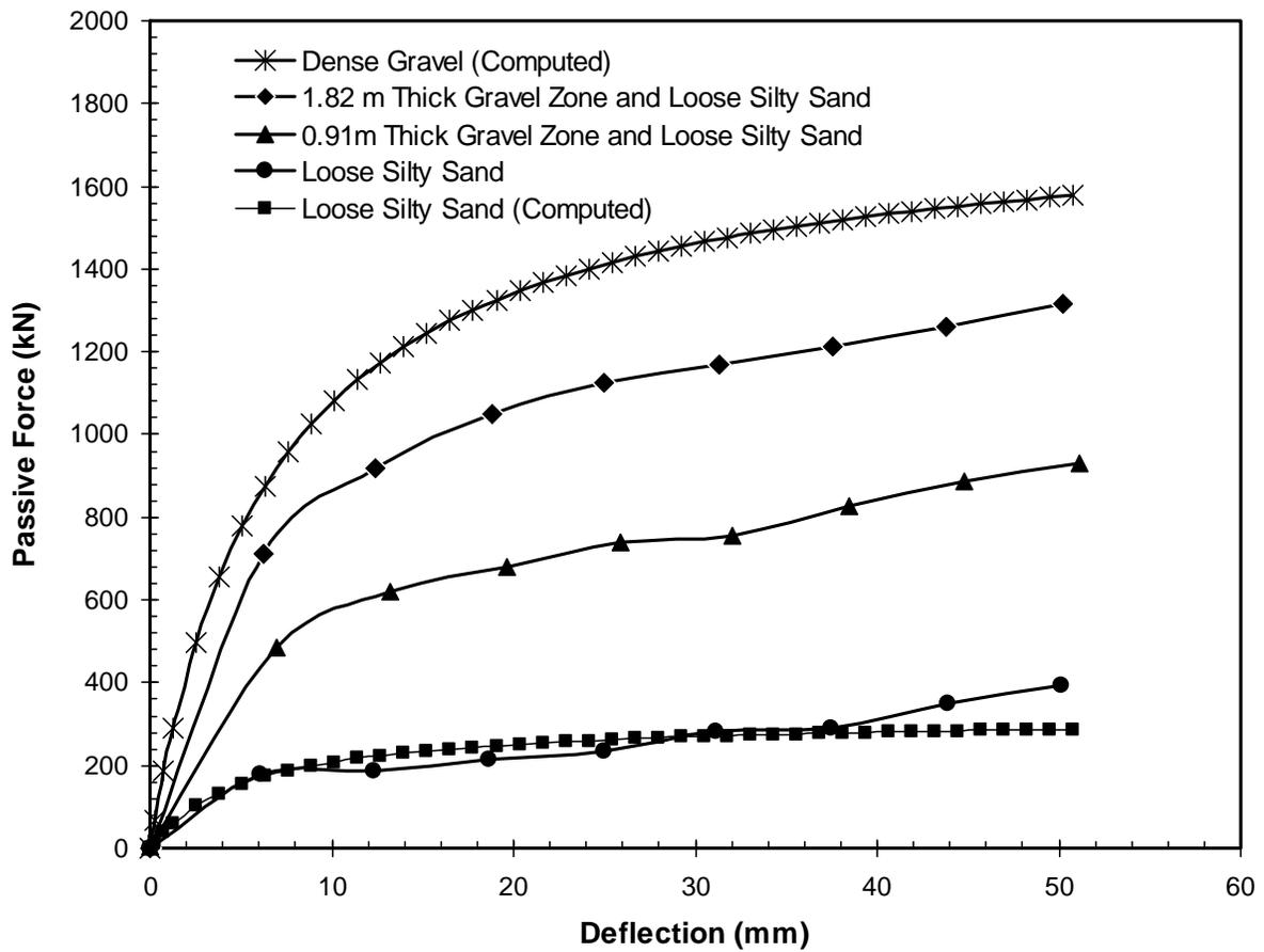
**Fig. 3. Measured passive force vs. deflection curves for a pile cap with loose silty sand backfill and with 0.91- and 1.82-m wide dense gravel zones with loose silty sand backfill. Computed curves for backfills entirely of loose silty sand and dense gravel are also shown.**
