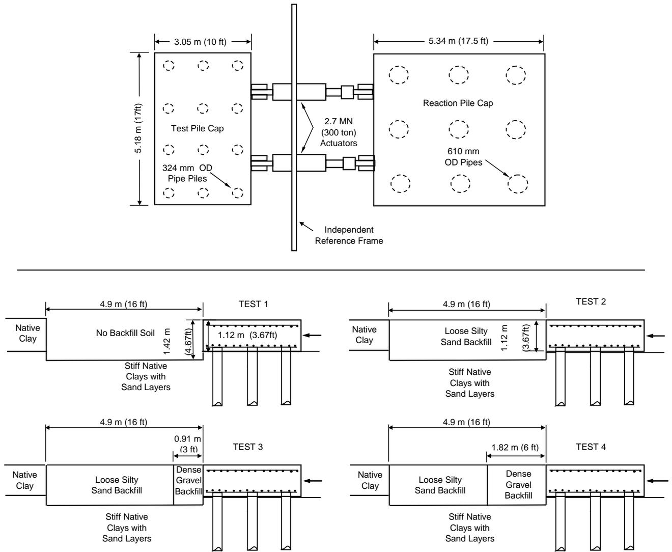
**Fig. 1. Plan and profile views of the test layout for the large-scale passive force tests.**
