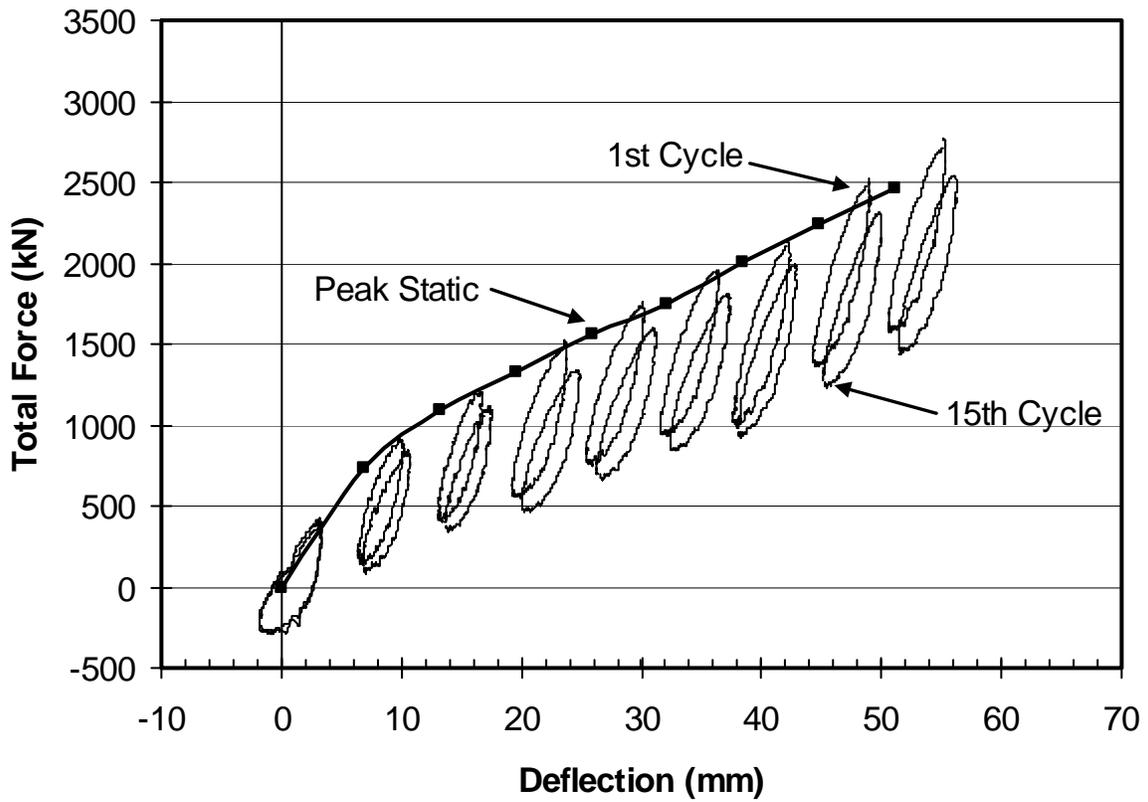
**Fig. 7. Plots of peak static load-deflection along with 1<sup>st</sup> and 15<sup>th</sup> load cycles at each deflection increment for tests involving 0.91-m wide gravel zone.**
