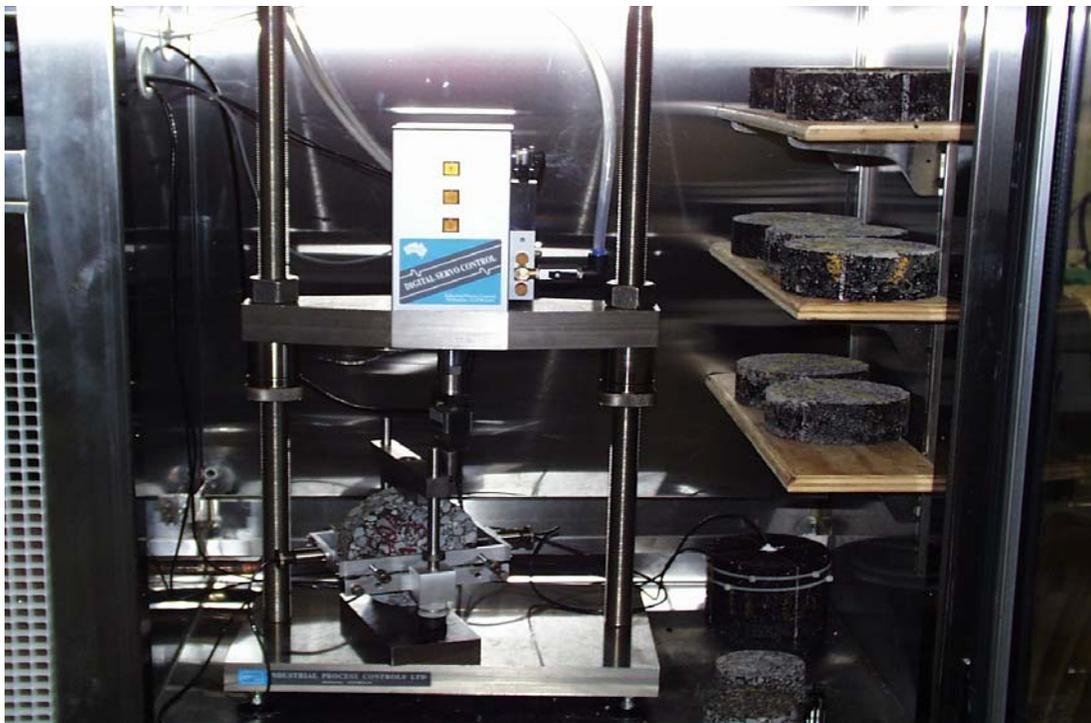
Figure 6-1 Resilient Modulus ( $M_R$ ) Test Device Utilized at the University of Illinois ATREL
