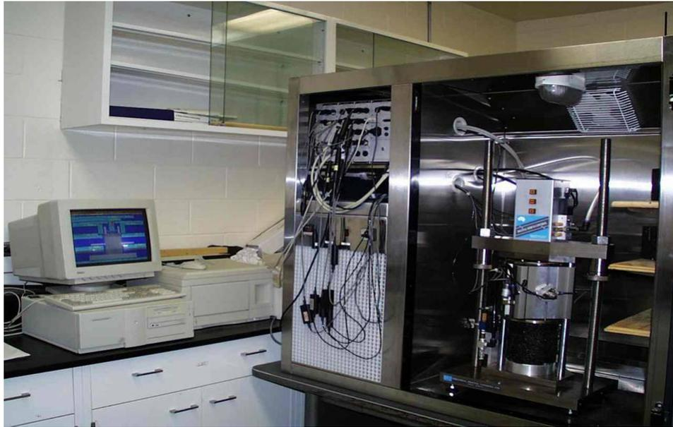
Figure 5-2 Repeated Load Triaxial Setup Used in Permanent Deformation Testing of Asphalt Specimens at ATREL
