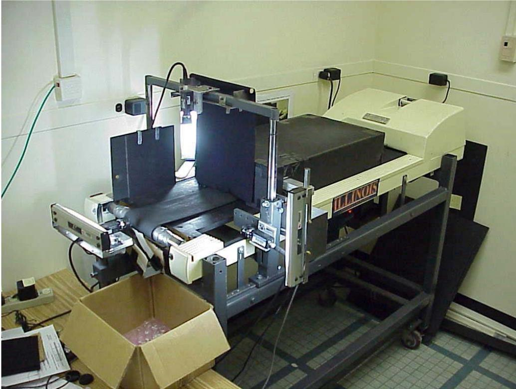
Figure 2-5 Photograph Showing the University of Illinois Aggregate Image Analyzer
