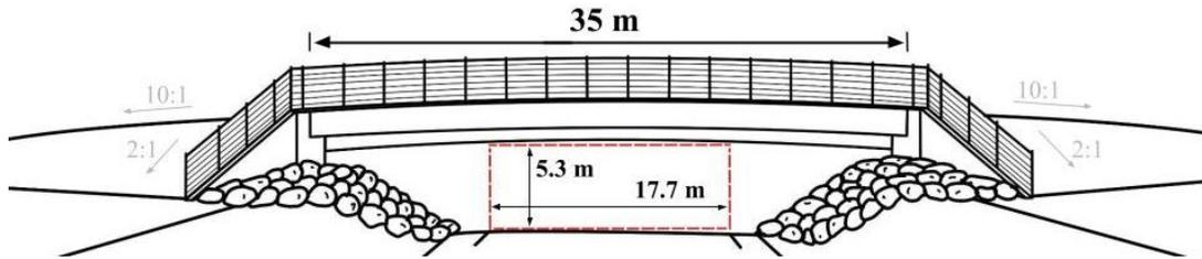
**Figure 9: Elevation view of the US-97 wildlife overpass.**
