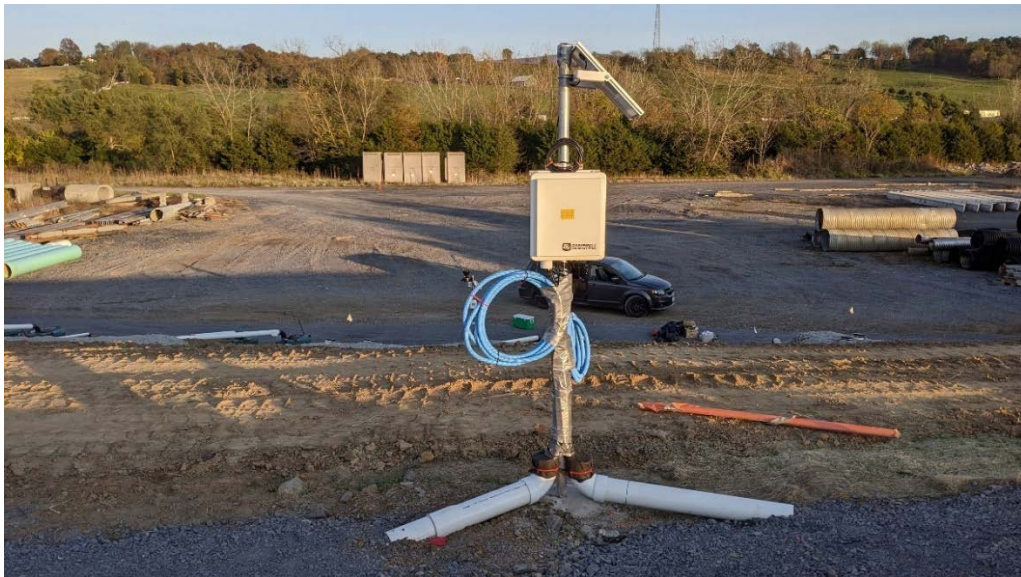
Figure 10. Data logger pole for all volumetric moisture content sensors
