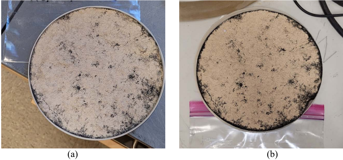
Figure 13. Appearance of the geotextile sample exhumed from unpaved RCA section after 9 months (a) before and (b) after permittivity test
