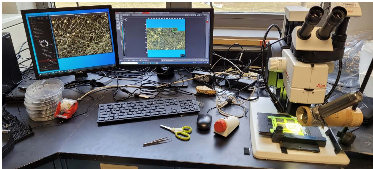
Figure 15. Leica M125 C microscope with a built-in 5 MP HD digital camera with a geotextile sample under analysis
