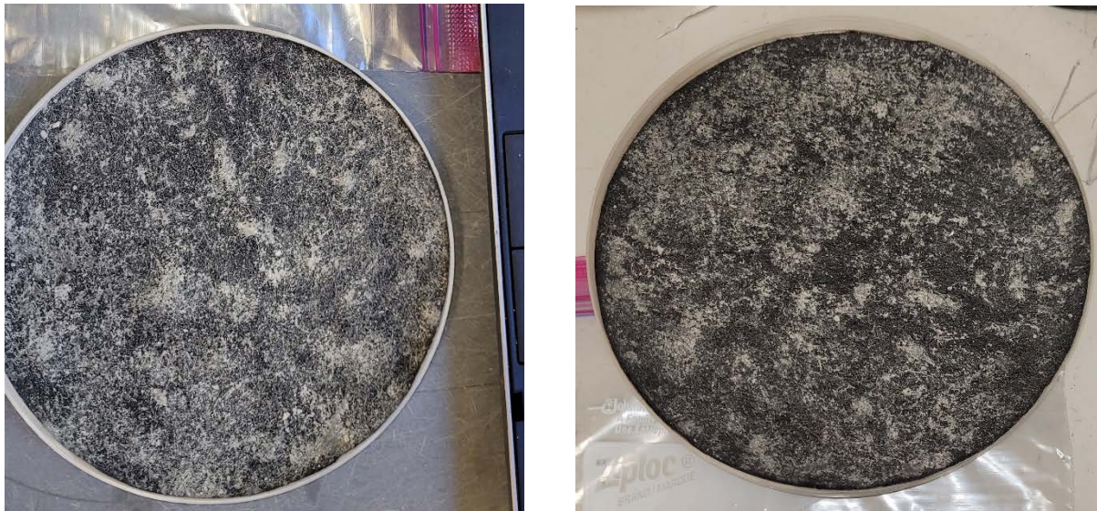
Figure 14. Geotextile sample exhumed from unpaved V.A. section after 9 months (a) before and (b) after permittivity test
