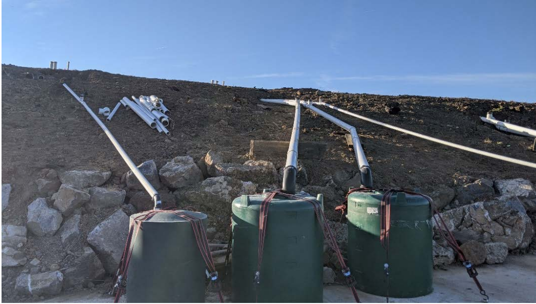
Figure 7. Collection tanks connected to underdrains (two 100-gallon tanks) for each side
