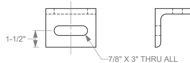
**10a.** Galvanize all components after fabrication is complete.
