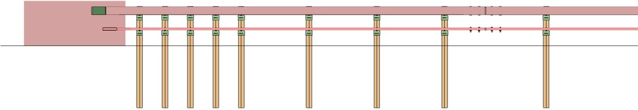
**Figure 1. Box Beam Transition to Concrete Parapet.**
