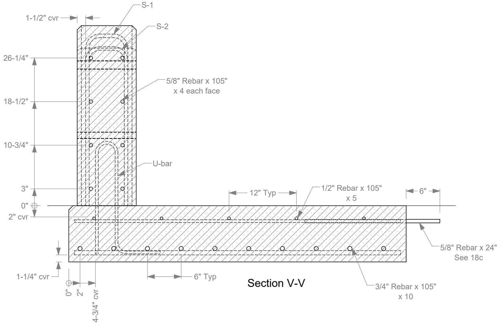
**18a.** Concrete is 4,000 psi. Rebar is Grade 60.
