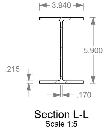
**9a.** Galvanize all components after fabrication is complete.
