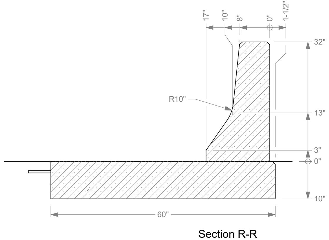
**16a.** Chamfer 1" (3/4" each way) edges of Parapet and Deck where shown.
