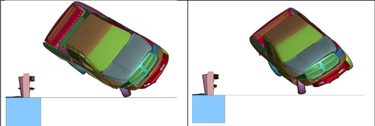
**Figure 3. HSS 6x2 (left) and HSS 4x3 (right) Pickup Truck at Maximum Roll Angle.**
