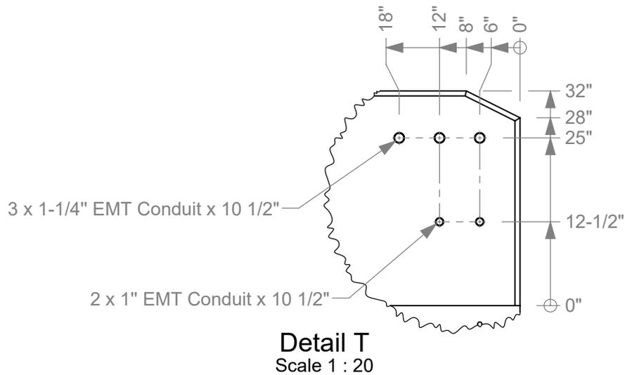
**15a.** Chamfer 1" (3/4" each way) edges of Parapet and Deck where shown.
