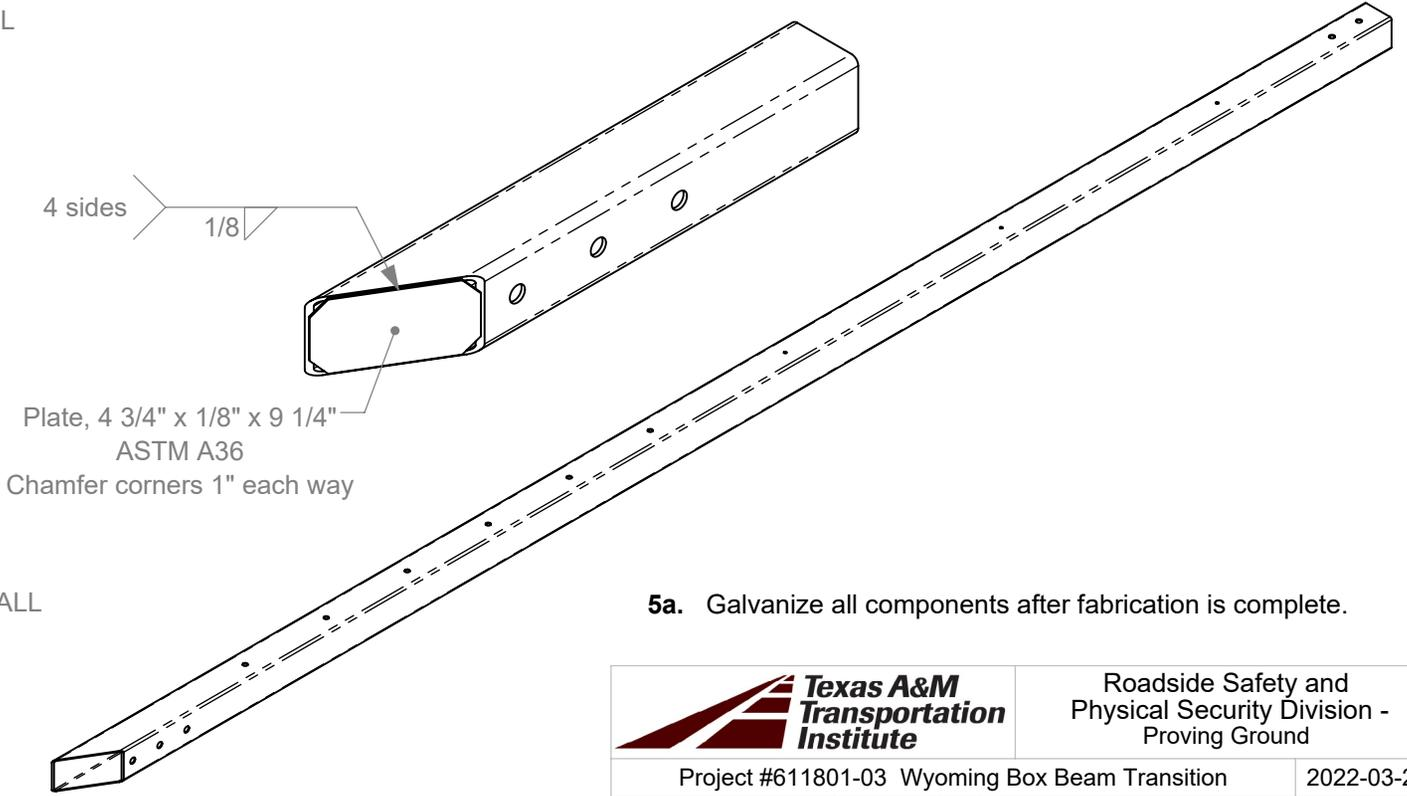
5a. Galvanize all components after fabrication is complete.
