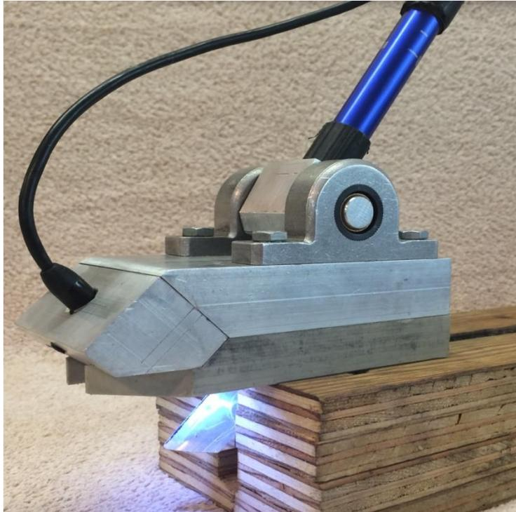
**Figure 25. Photo. Joint inspection assembly - (JIS-QC), production prototype.**
