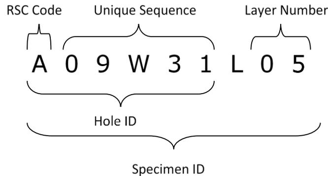
**Figure 13. Illustration. SPECIMEN ID Diagram.**
