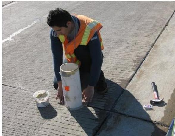
**Figure 29. Photo. Infiltration Testing**
