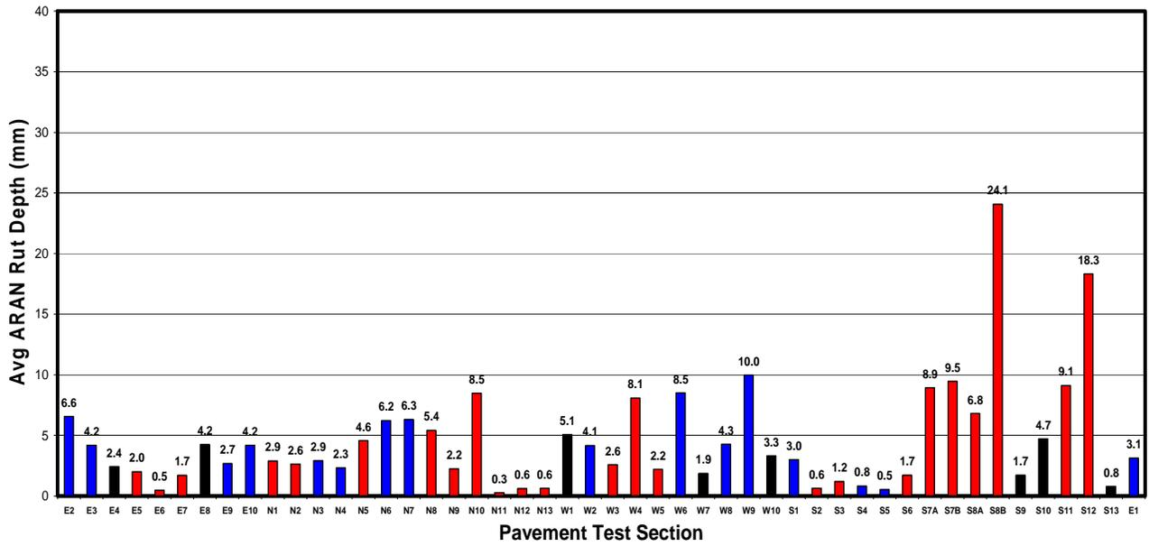
**Figure 2 Rutting Performance of Test Sections at the End of Reporting Period**
