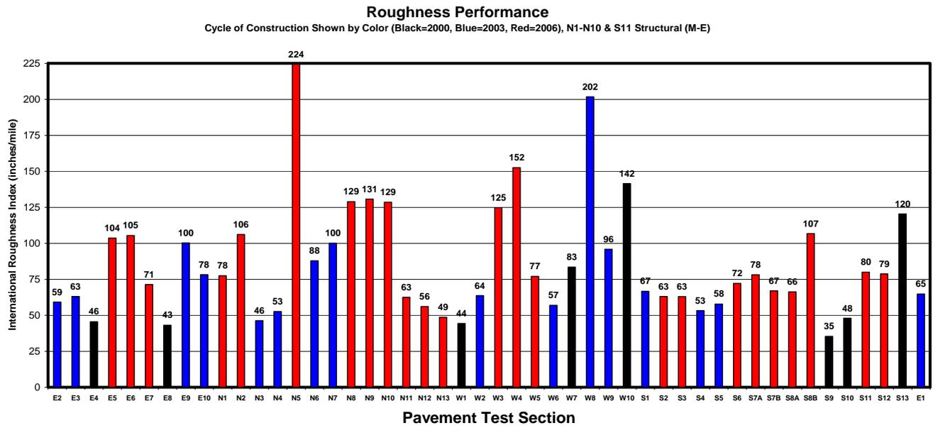
**Figure 3 IRI of Test Sections at the End of Reporting Period**
