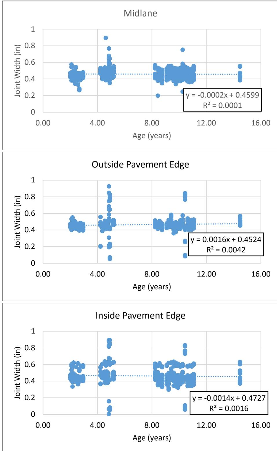
**Figure 20. Linear Regression of Joint Width Against Time for All Six Joints Measured on 040215.**
