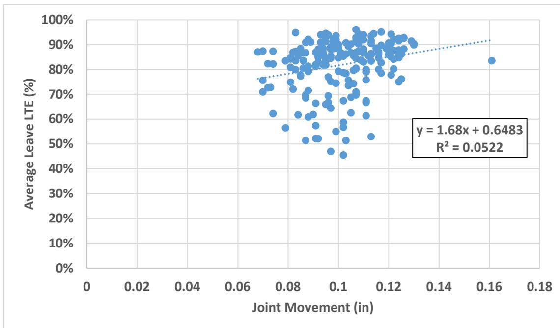
**Figure 12. Comparison of Average Load Transfer Efficiency on Approach (top) and Leave (bottom) Side of Joints to Predicted Joint Movement for all SPS-2 Sections.**
