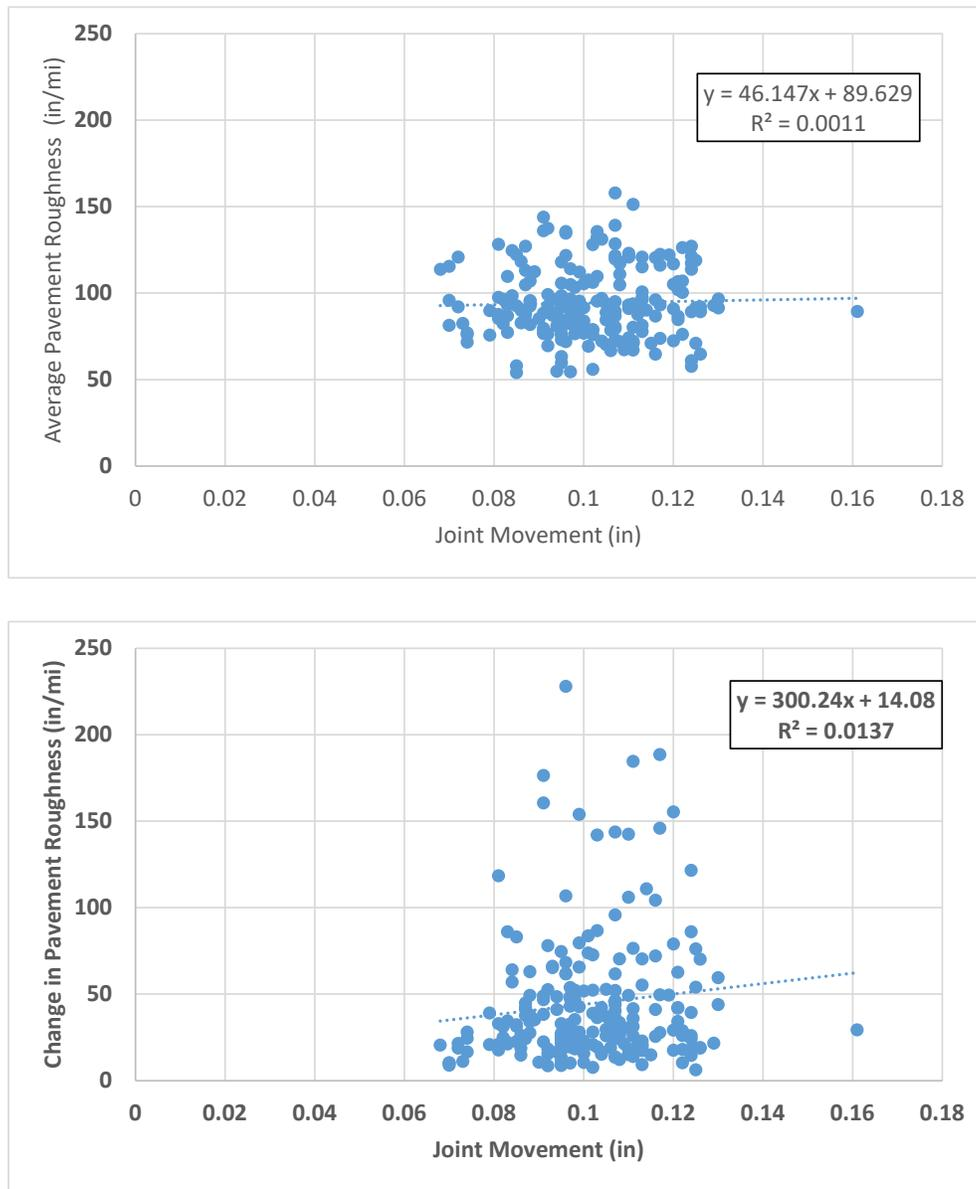
**Figure 16. Comparison of Average Pavement Roughness (top) and Lifetime Change in Pavement Roughness (bottom) to Predicted Joint Movement for all SPS-2 Sections.**
