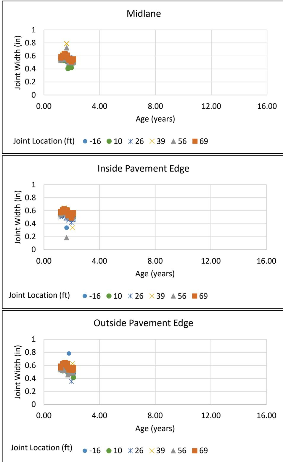
Figure 23. Summary of Joint Widths Over Time for Six Joints Measured on 320204.
