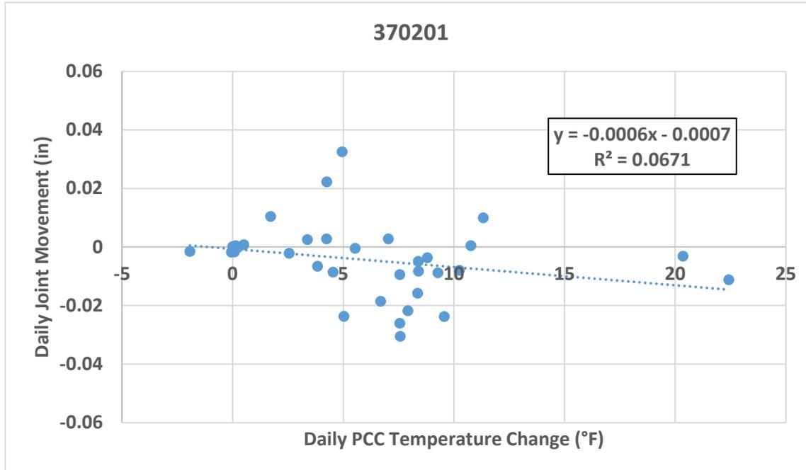
**Figure 10. Comparison of Average Daily Joint Movement to Average Daily Change in PCC Temperature for 370201.**
