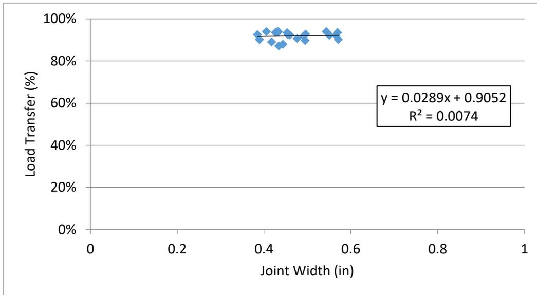
**Figure 26. LTE Versus Joint Width for Joints with 0.5 mil Difference in Deflection for 390204.**
