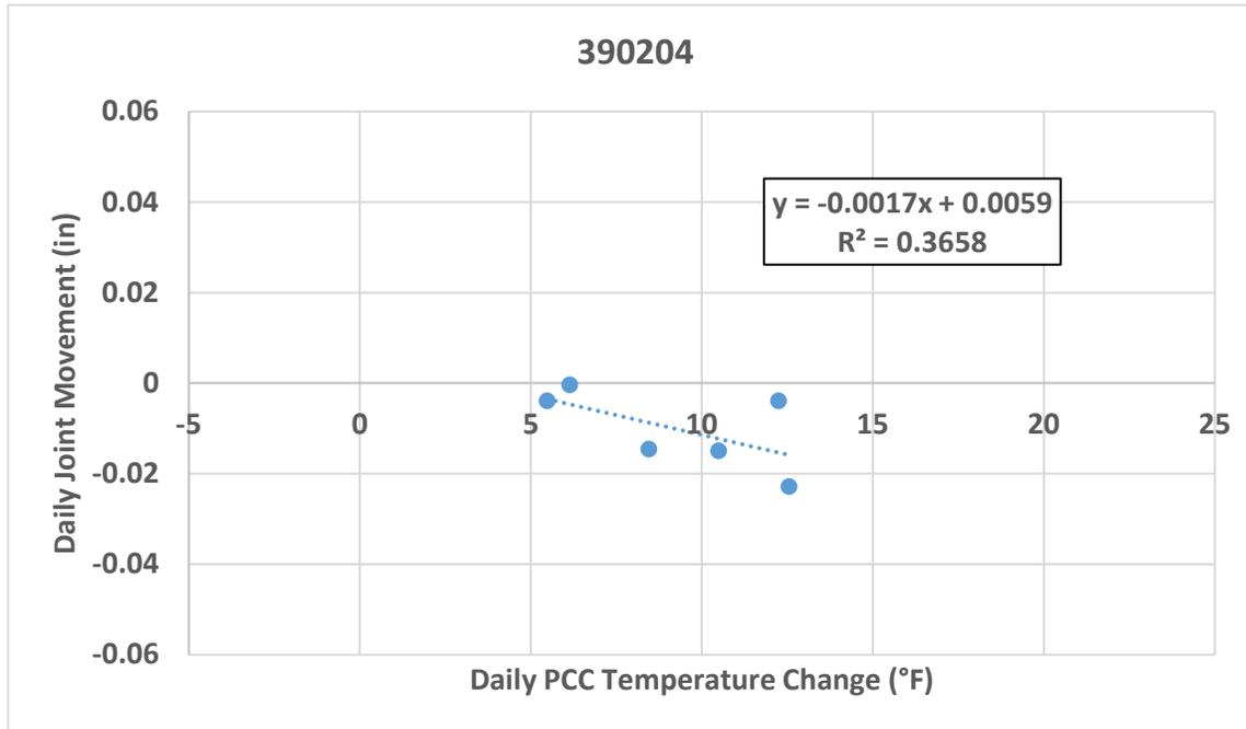
**Figure 11. Comparison of Average Daily Joint Movement to Average Daily Change in PCC Temperature for 390204.**
