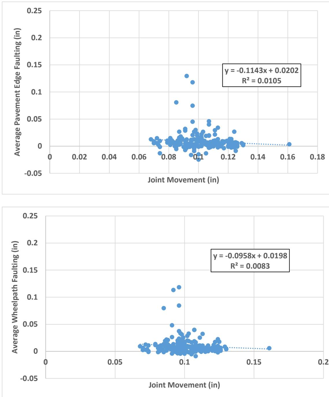
**Figure 14. Comparison of Average Faulting Measurements at Pavement Edge (top) and Outer Wheel-Path (bottom) to Predicted Joint Movement for all SPS-2 Sections.**
