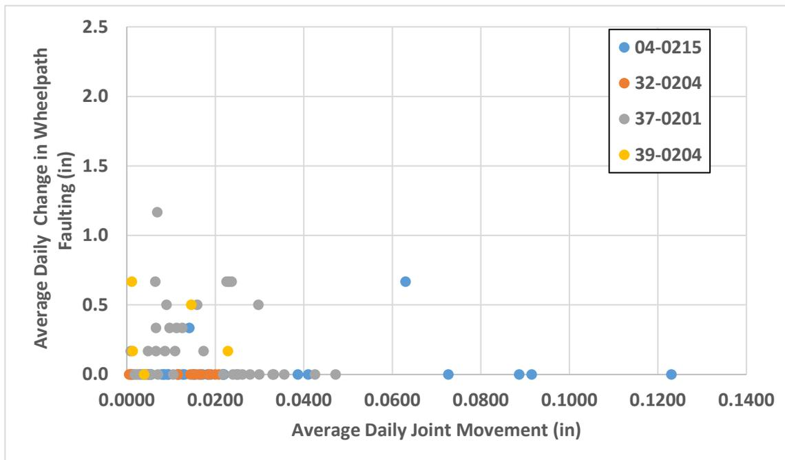
**Figure 7. Comparison of Average Daily Change in Pavement Edge (top) and Wheel-Path (bottom) Faulting Measurements Compared to Average Daily Joint Movement for SPS-2 SMP Sections.**
