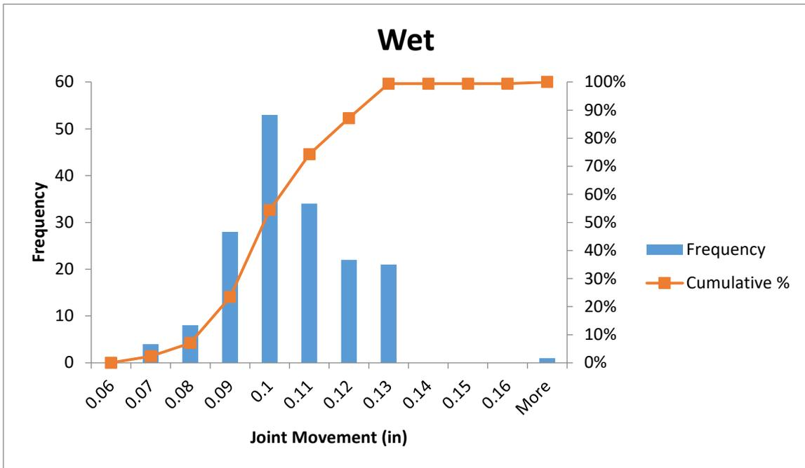
**Figure 1. Distribution of Estimated Joint Movement Values for all SPS-2 Sections for Dry (top) and Wet (bottom) Climates.**
