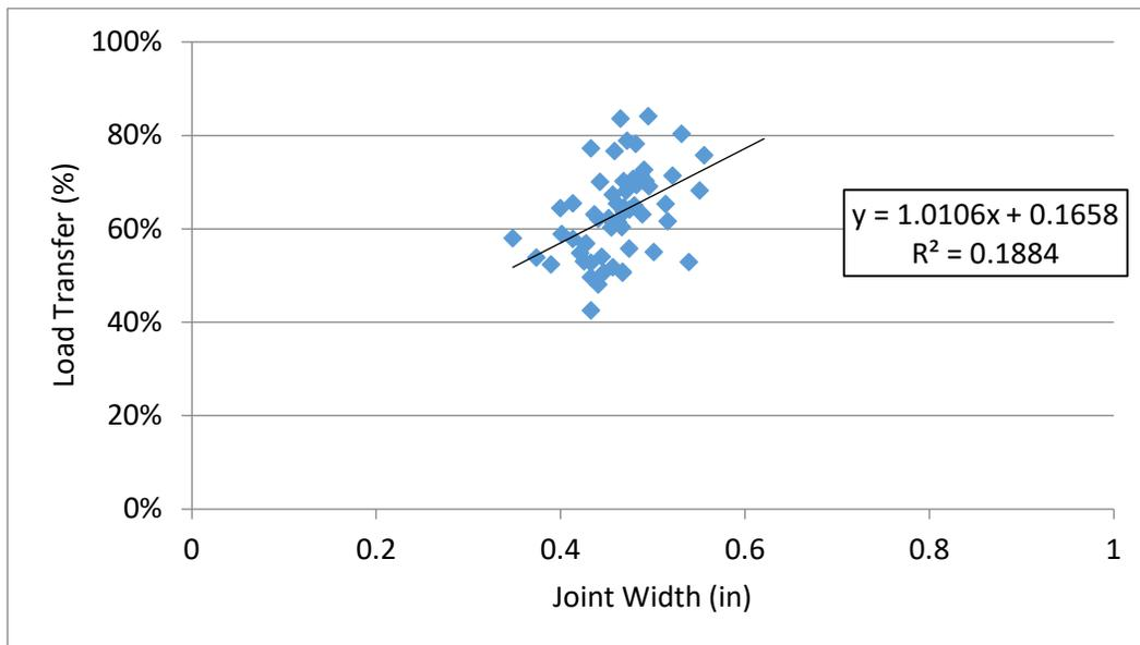
**Figure 18. LTE Versus Joint Width for Joints with More than 1.5 mils Difference in Deflection on 040215.**
