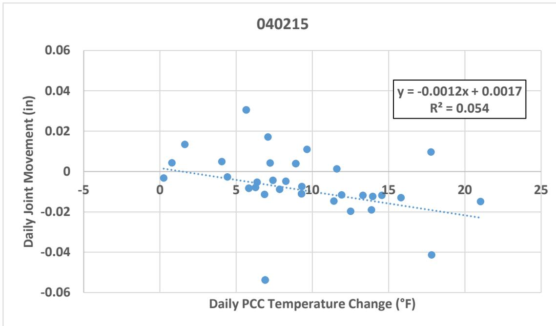
**Figure 8. Comparison of Average Daily Joint Movement to Average Daily Change in PCC Temperature for 040215.**
