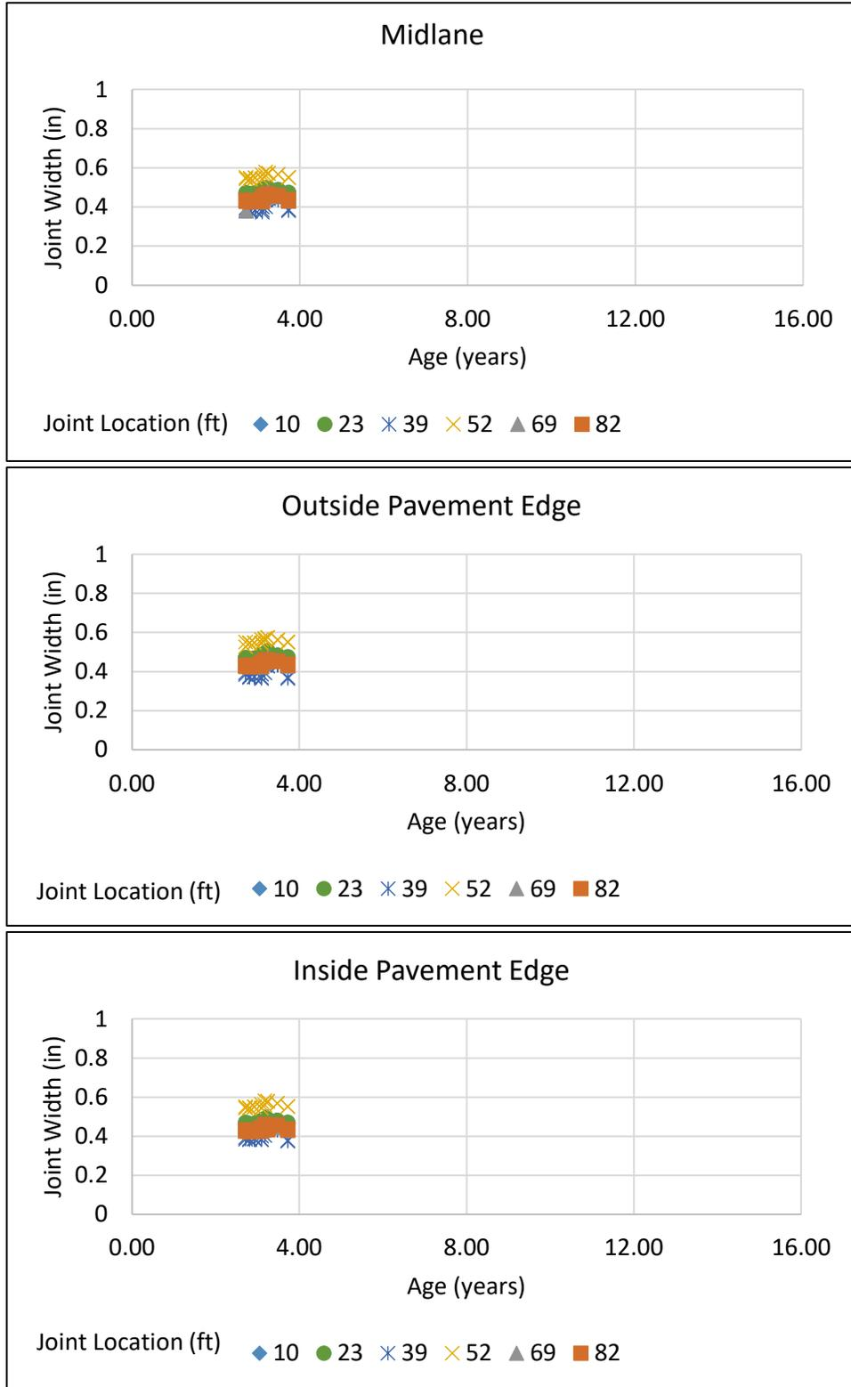
**Figure 27. Comparison of Joint Widths Over Time for Six Joints Measured on 390204.**
