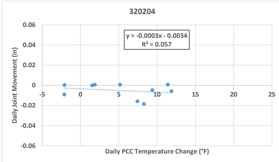
**Figure 9. Comparison of Average Daily Joint Movement to Average Daily Change in PCC Temperature for 320204.**
