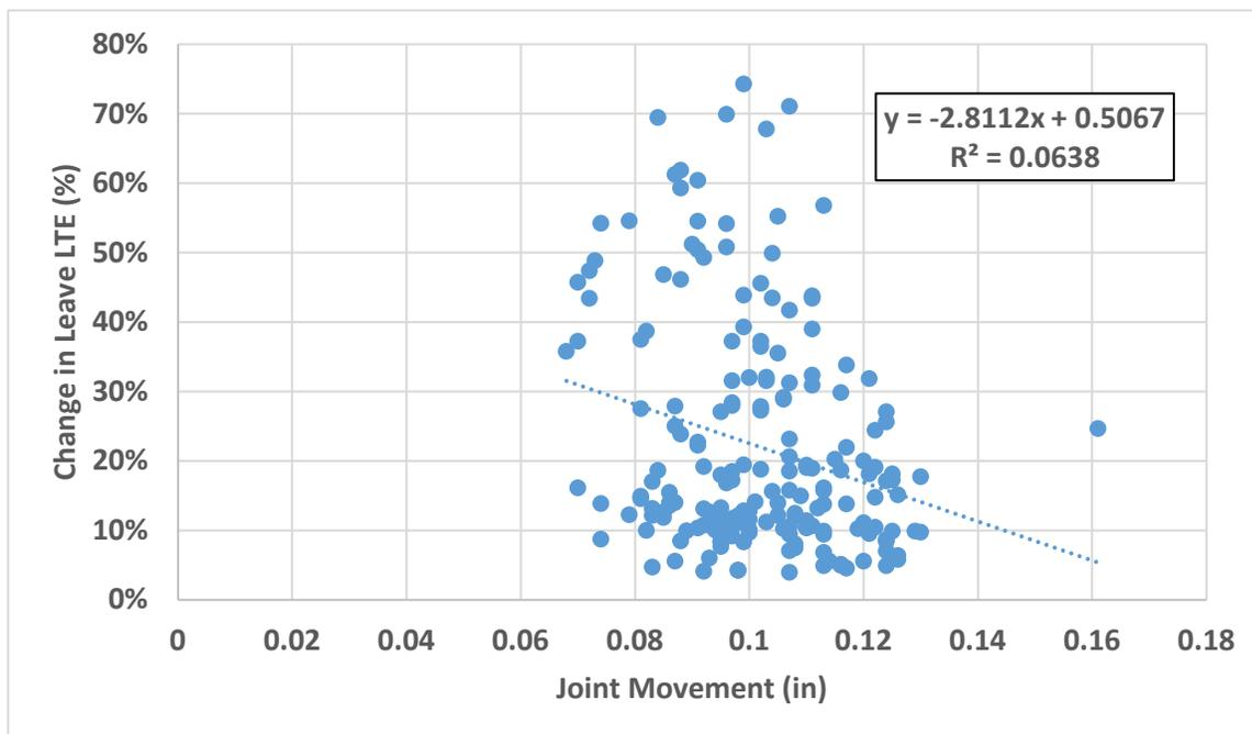
**Figure 13. Comparison of Lifetime Change in Load Transfer Efficiency on Approach (top) and Leave (bottom) Side of Joints to Predicted Joint Movement for all SPS-2 Sections.**
