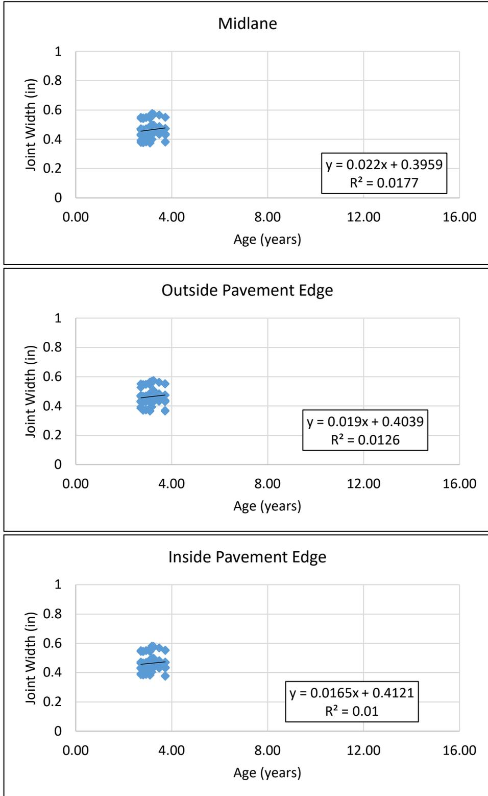
**Figure 28. Linear Regression of Joint Widths Against Time for Six Joints Measured on 390204.**
