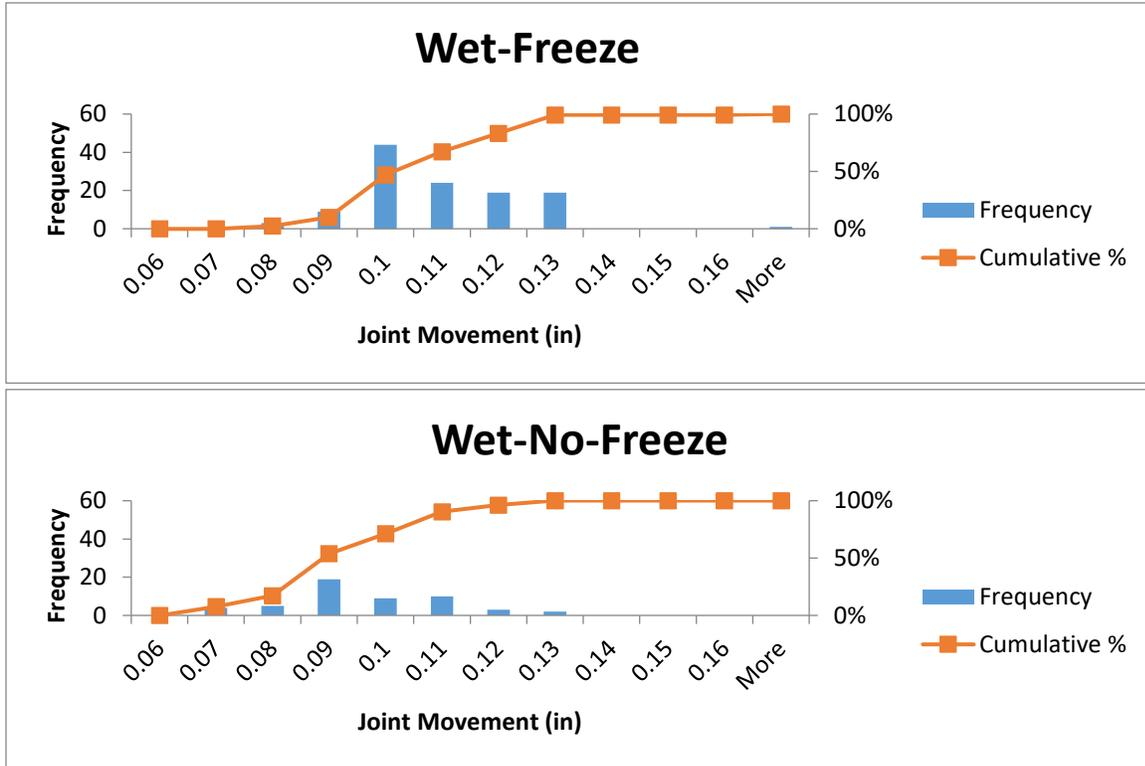
**Figure 3. Distribution of Estimated Joint Movement Values for all SPS-2 Sections Based on the Four LTPP Climatic Regions: Dry-Freeze (top), Dry-No-Freeze (2<sup>nd</sup> from top), Wet-Freeze (2<sup>nd</sup> from bottom), and Wet-No-Freeze (bottom).**
