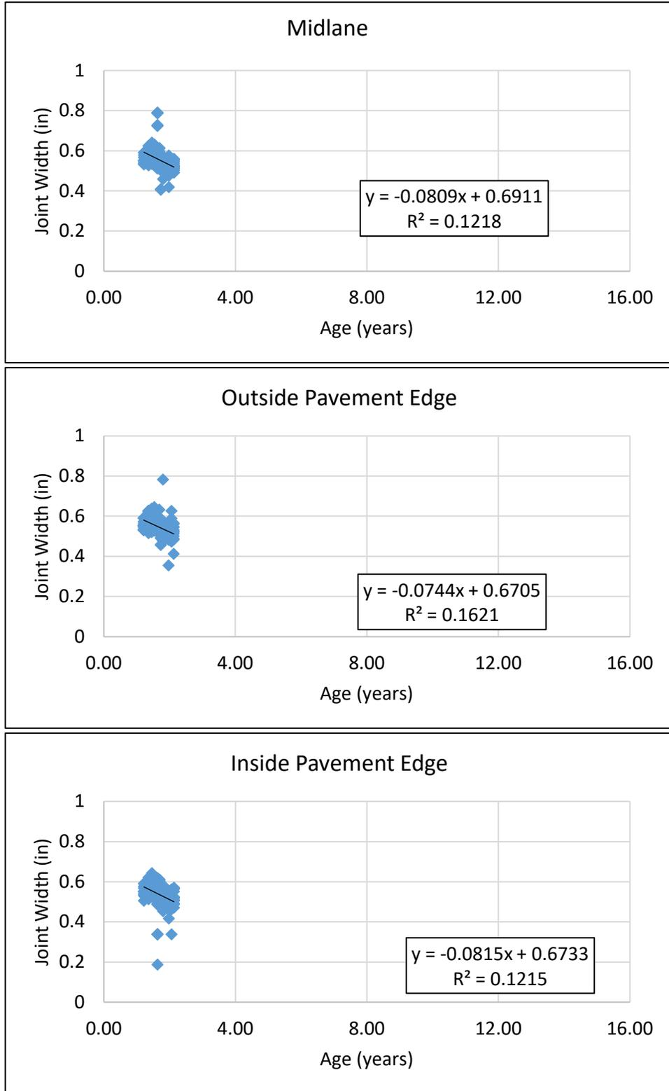
**Figure 24. Linear Regression of Joint Width Against Time for Six Joints Measured on 320204.**
