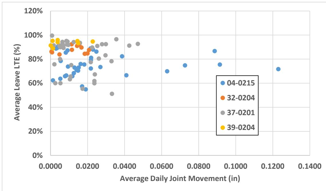
**Figure 4. Comparison of Daily Average LTE for Approach (top) and Leave (bottom) Side of Joints Compared to the Average Daily Joint Movement on the SPS-2 SMP Sections.**
