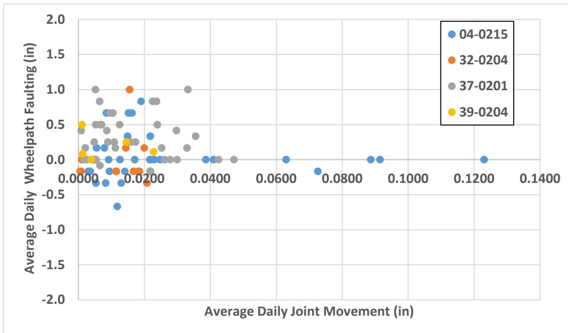
**Figure 6. Comparison of Average Daily Pavement Edge (top) and Wheel-Path (bottom) Faulting Measurements Compared to Average Daily Joint Movement for SPS-2 SMP Sections.**
