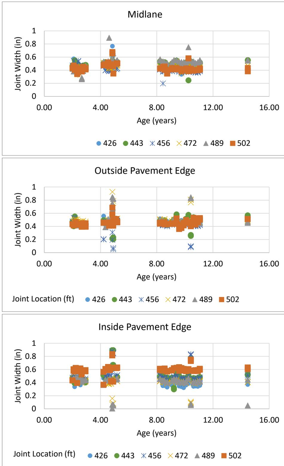
**Figure 19. Joint Width Changes Over Time for All Six Joints Measured on 042015.**
