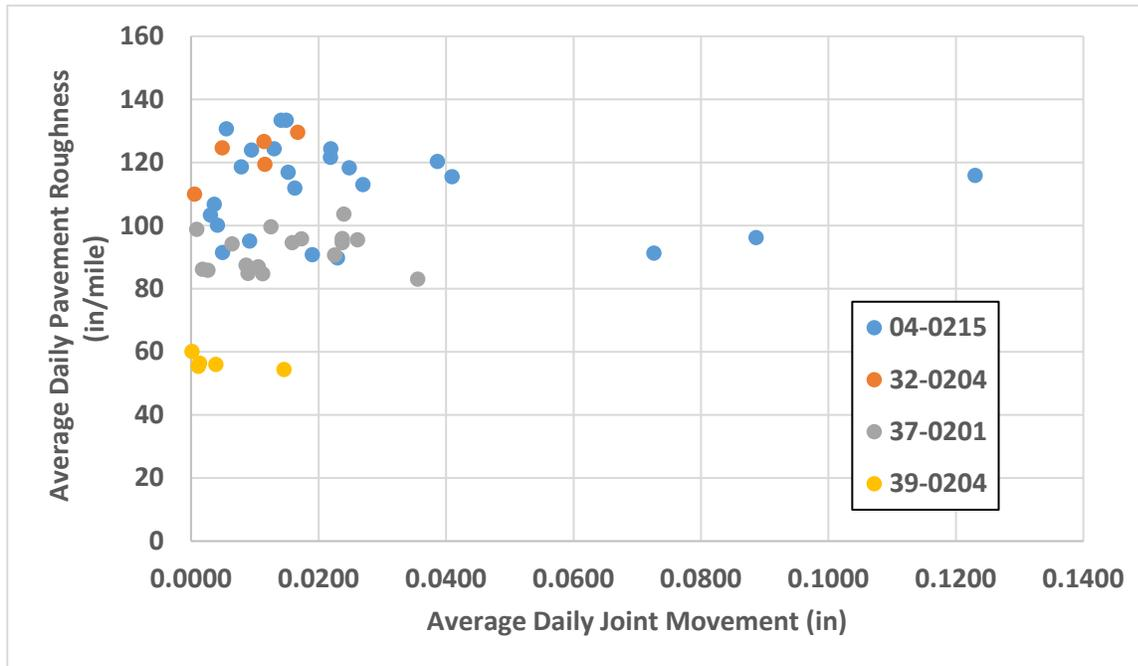
**Figure 5. Average Daily Pavement Roughness Values Compared to the Average Daily Joint Movement on the SPS-2 SMP Sections.**
