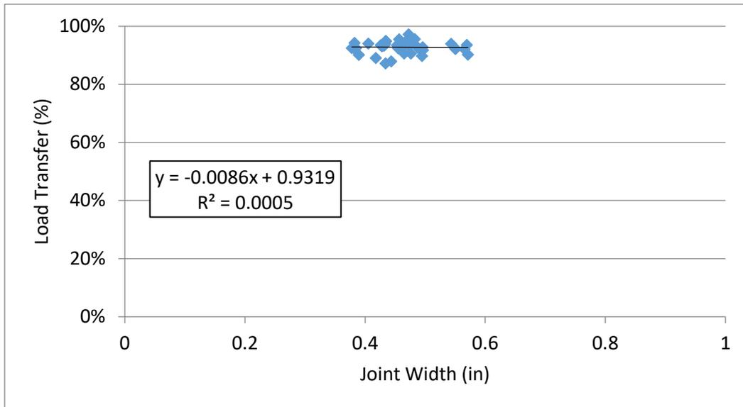
**Figure 25. LTE Versus Joint Widths for All Joints on 390204.**
