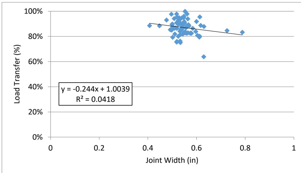
**Figure 21. LTE Versus Joint Opening Width for All Joints on 320204.**
