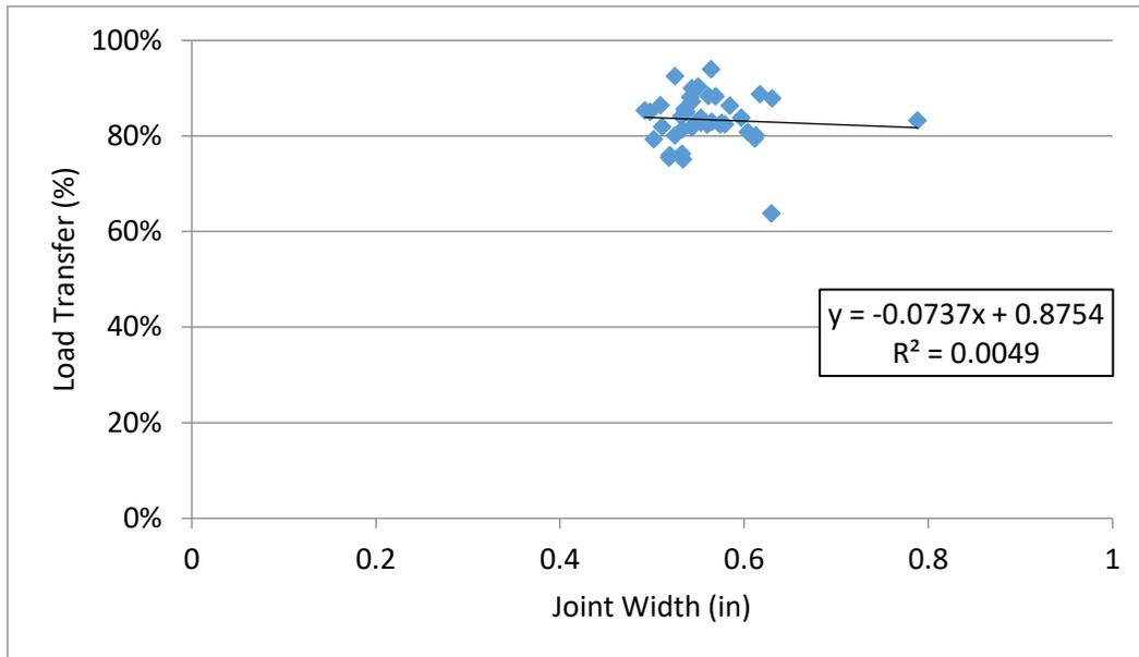
**Figure 22. LTE Versus Joint Opening Width for Joints with More than 0.5 mil Difference in Deflection for 320204.**
