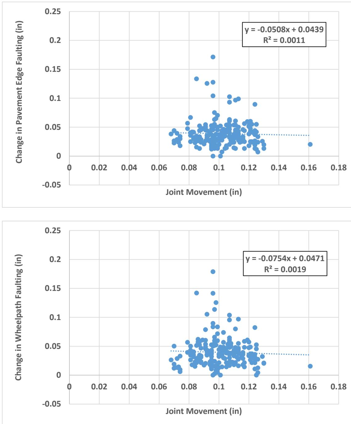
**Figure 15. Comparison of Lifetime Change in Faulting Measurements at Pavement Edge (top) and Outer Wheel-Path (bottom) to Predicted Joint Movement for all SPS-2 Sections.**
