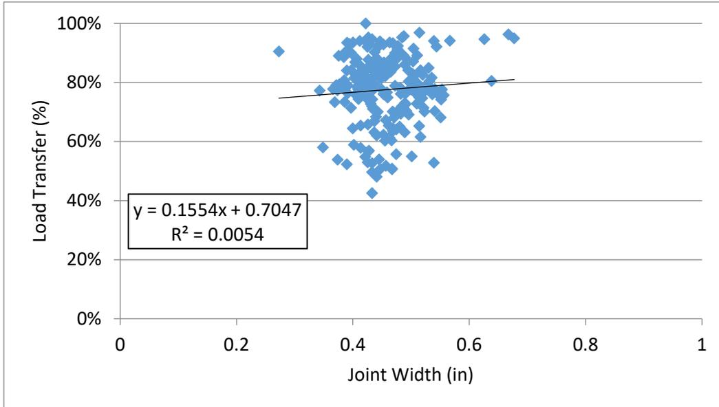
**Figure 17. LTE Versus Joint Width for all Joints on 040215.**
